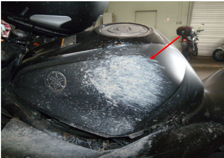
Photo 9 shows a closer view of the grazed petrol tank of the Motorcycle as a result of the accident (arrowed).
