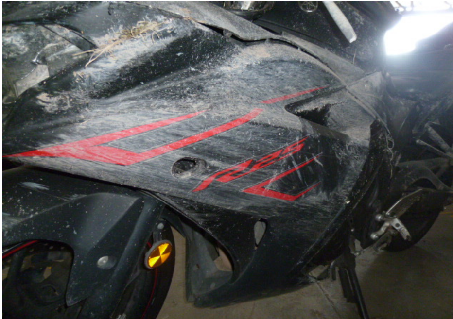
Photo 10 shows a closer view of the left cowling which was amongst the body parts of the Motorcycle that had sustained damage as a result of the accident.
