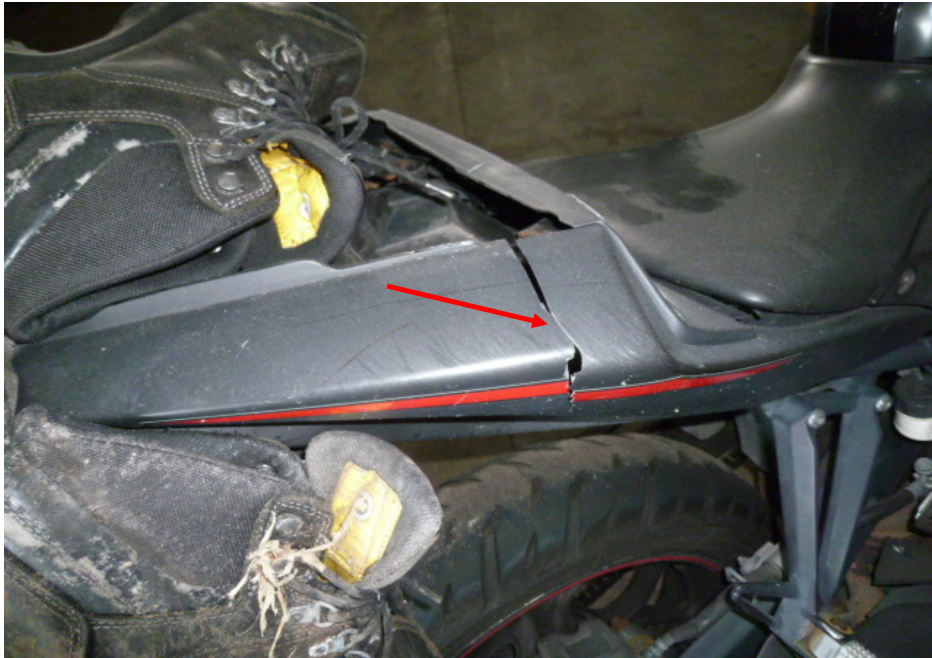
Photo 14 shows a closer view of the cracked right rear side cover of the Motorcycle as a result of the accident (arrowed).
