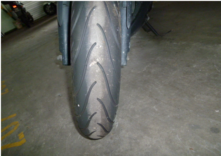
Photo 15 shows the front tyre of the Motorcycle at the time of our inspection. The front tyre was observed to be in serviceable condition with remaining tread depth of approximately 4mm. The pattern of the tread was also clearly visible. There was no tear, burst mark(s) and/or punctured hole(s) on the sidewalls as well as across the tread of the front tyre.
