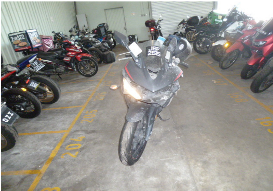
Photo 23 shows the front wheel of the Motorcycle turned towards its full right. Turning the Motorcycle's handle bar towards the right did not produce any abnormal free play and/or resistance. This would indicate that the steering system of the Motorcycle was in serviceable condition at the time of our inspection.
