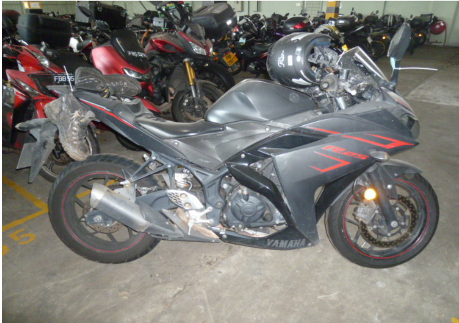
Photo 4 shows a general view of the right body of the Motorcycle at the time of our inspection. The Motorcycle was observed to have sustained damages all around. The body parts that were found to have been damaged include its front cowling, front mudguard, front wheel axle nut, side cowlings, left side mirror, clutch lever, left handlebar end, petrol tank, gear shift pedal, left front footrest, rear side covers and left rear signal lamp, amongst others.
