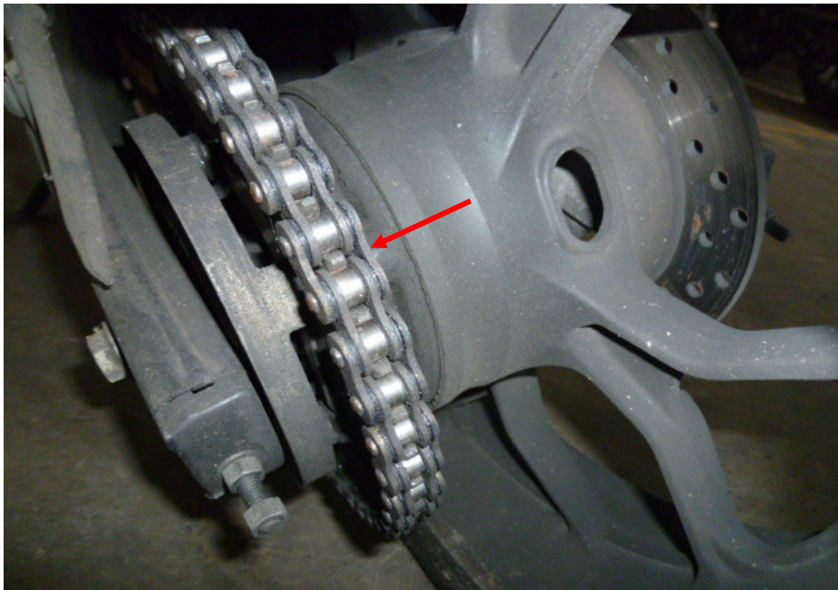
Photo 20 shows a closer view of the gear train (arrowed) of the Motorcycle, which was observed to be intact with no misalignment. It was also adequately lubricated for operating purposes.
