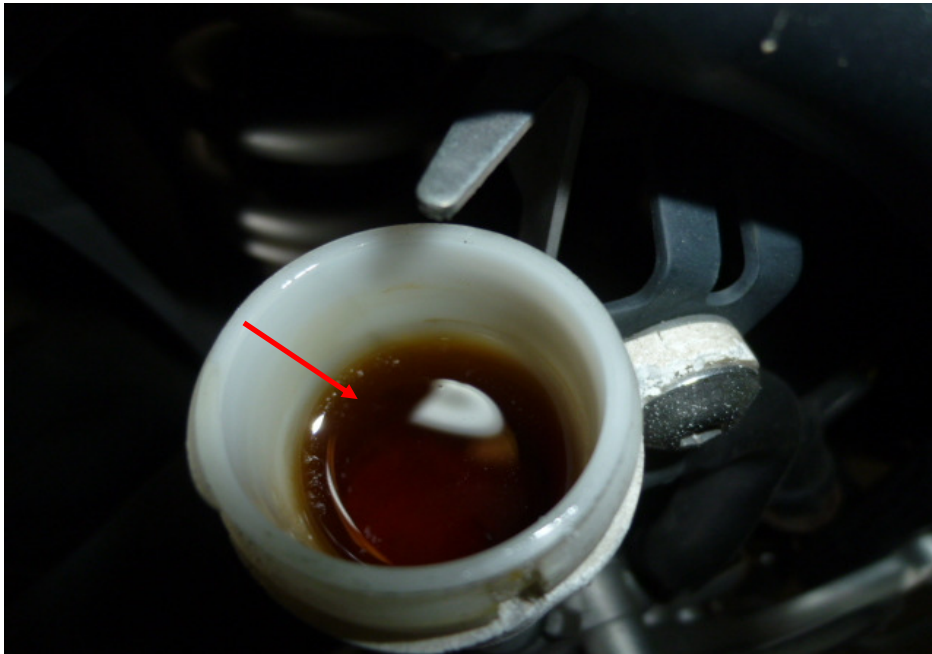
Photo 29 shows a close up view of the brake fluid reservoir for the rear brake of the Motorcycle. The rear brake fluid was observed to be of sufficient level for operational purposes. However it was found to be slightly contaminated (arrowed).
