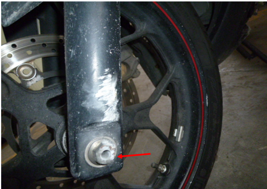
Photo 7 shows a closer view of the grazed front wheel axle nut (arrowed) of the Motorcycle as a result of the accident.
