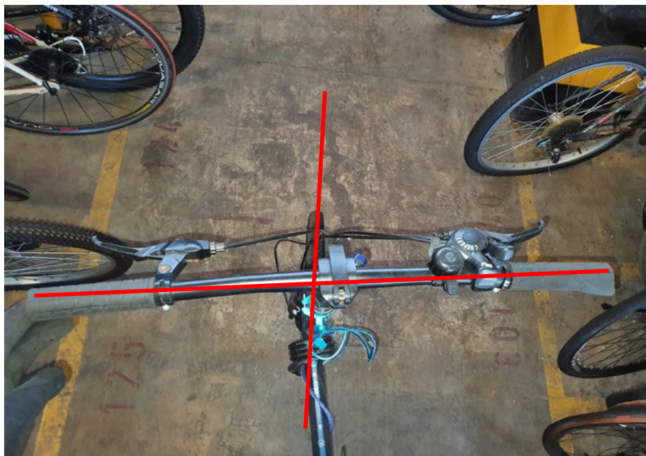
Photo 5 shows the frontal portion of the Bicycle (top view) at the time of our inspection. There was a misalignment of the handlebar & front tyre observed.
