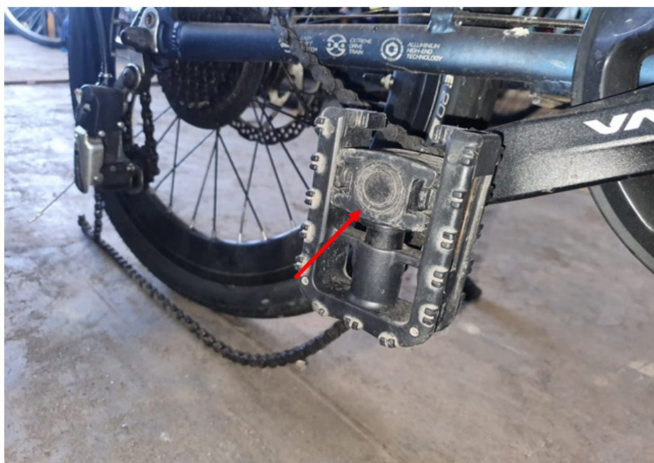
Photo 8 shows the grazed right pedal of the Bicycle at the time of our inspection (arrowed).
