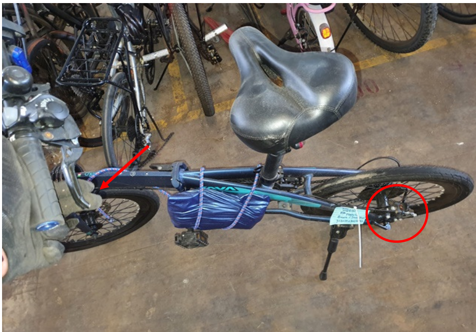
Photo 20 shows a static brake test conducted on the Bicycle's rear brake. There was some resistance felt upon pressing the right hand brake lever (arrowed). It also shows that the rear brake pads responded to the gripping action (circled) after depressing the right hand brake lever.
