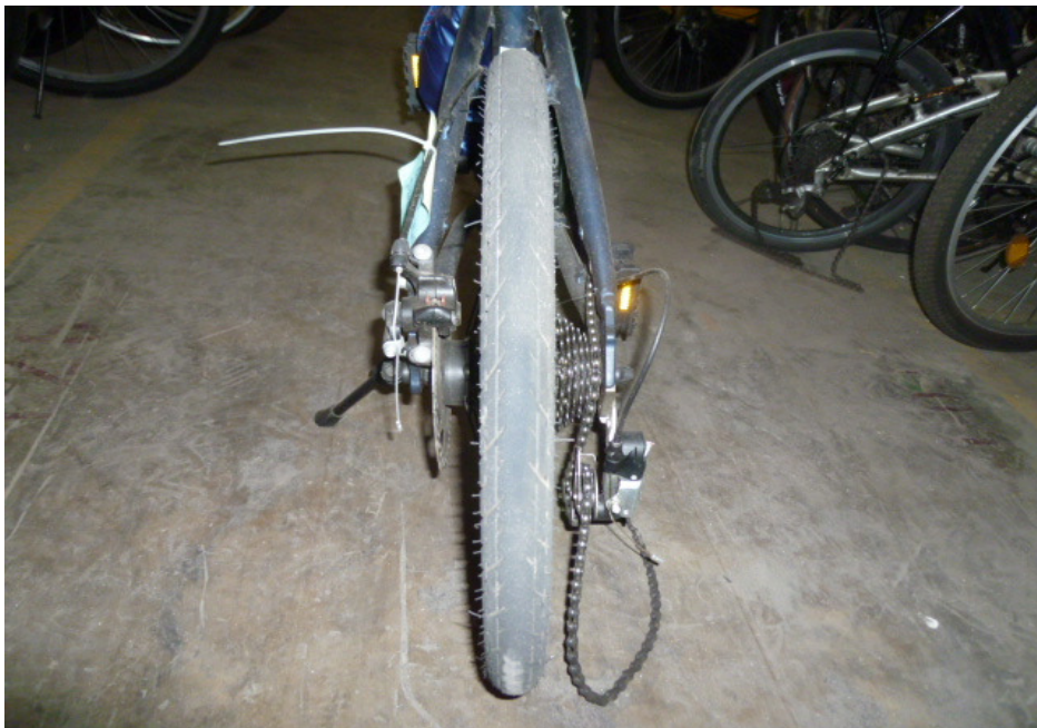
Photo 12 shows the rear tyre of the Bicycle. The rear tyre was observed to be in serviceable condition with remaining tread depth of approximately 3mm. The pattern of the tread was clearly visible. There was no tear, burst mark(s) and/or punctured hole(s) on the sidewalls as well as across the tread of the rear tyre. The rear tyre was also observed to be sufficiently inflated for vehicular operation.
