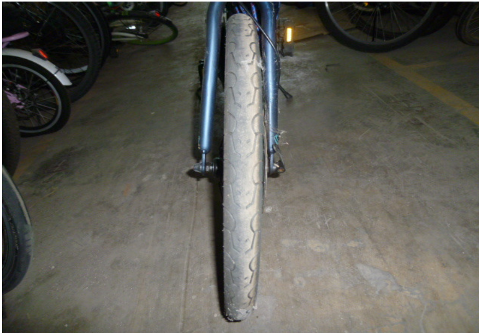
Photo 11 shows the front tyre of the Bicycle. The front tyre was observed to be in serviceable condition with remaining tread depth of approximately 3mm. There was no tear, burst mark(s) and/or punctured hole(s) on the sidewalls as well as across the tread of the front tyre. The front tyre was also observed to be sufficiently inflated for vehicular operation.
