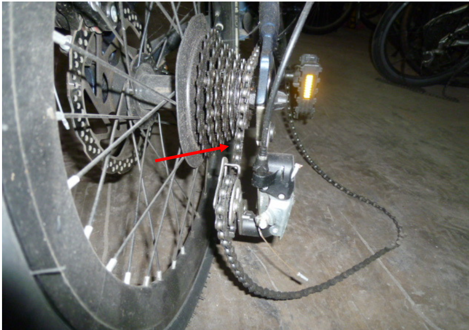
Photo 14 shows a close up view of the gear train of the Bicycle, which was observed to have sustained severe damages as a result of the accident (arrowed). No free play tension test can be conducted due to the extensive damages.
