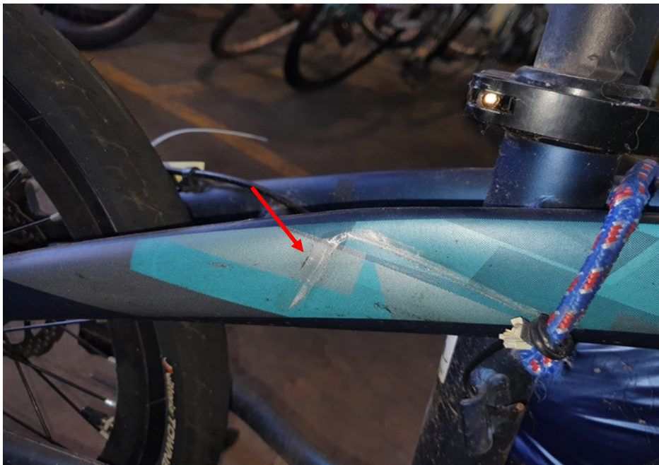
Photo 10 shows a close-up view of the deformed sub frame of the Bicycle as a result of the accident (arrowed).
