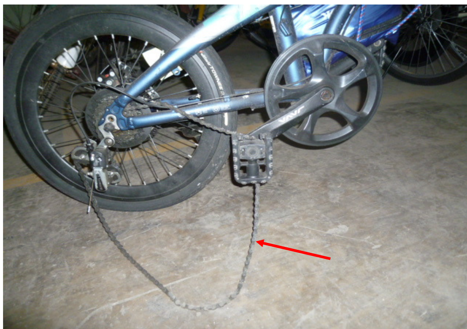
Photo 13 shows the general view of the gear train of the Bicycle which was found to be severely damaged as a result of the accident. The chain was also observed to be dislodged from the gear train most likely as a result of the accident (arrowed).
