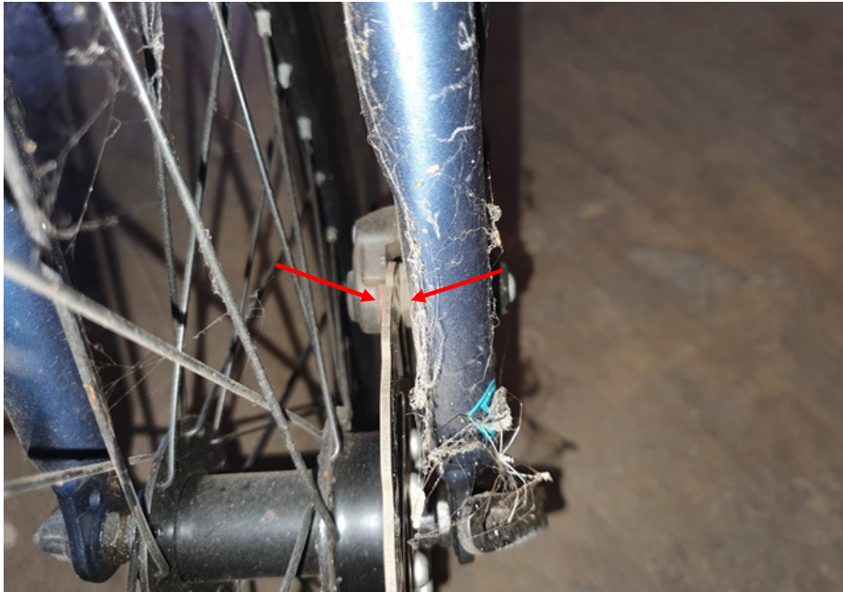
Photo 19 shows a close up view of the front brake pads responding to the gripping action. The front brake pads pressed against the front brake disc (arrowed) upon depressing the left hand brake lever. This had appeared to indicate that the front brake of the Bicycle was in serviceable condition.
