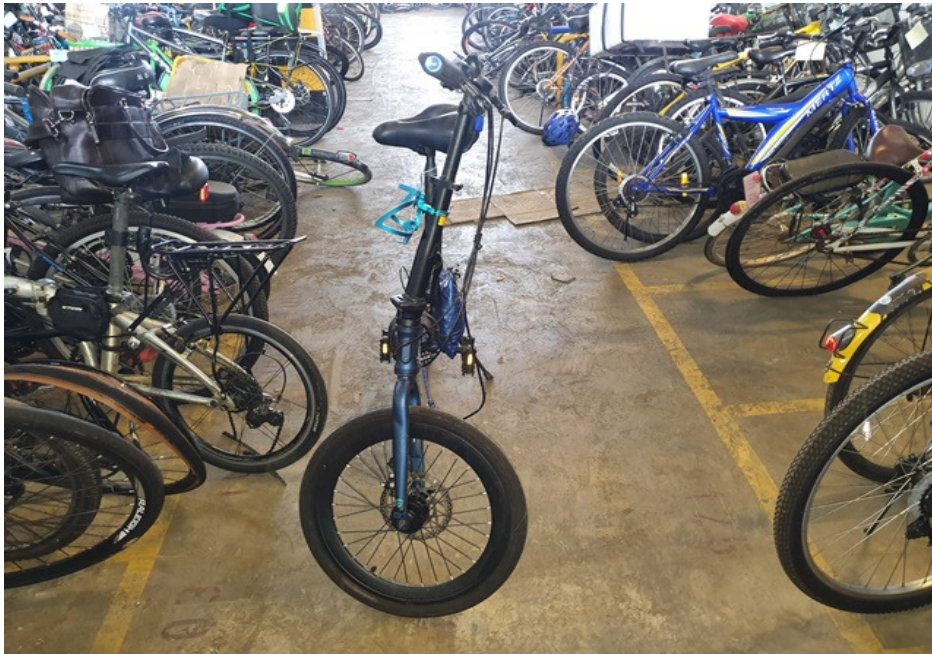
Photo 16 shows the front wheel of the Bicycle turned towards its full left. Turning the Bicycle's handle bar towards the left did not produce any abnormal free play and/or resistance. This would indicate that the steering system of the Bicycle was in serviceable condition at the time of our inspection.
