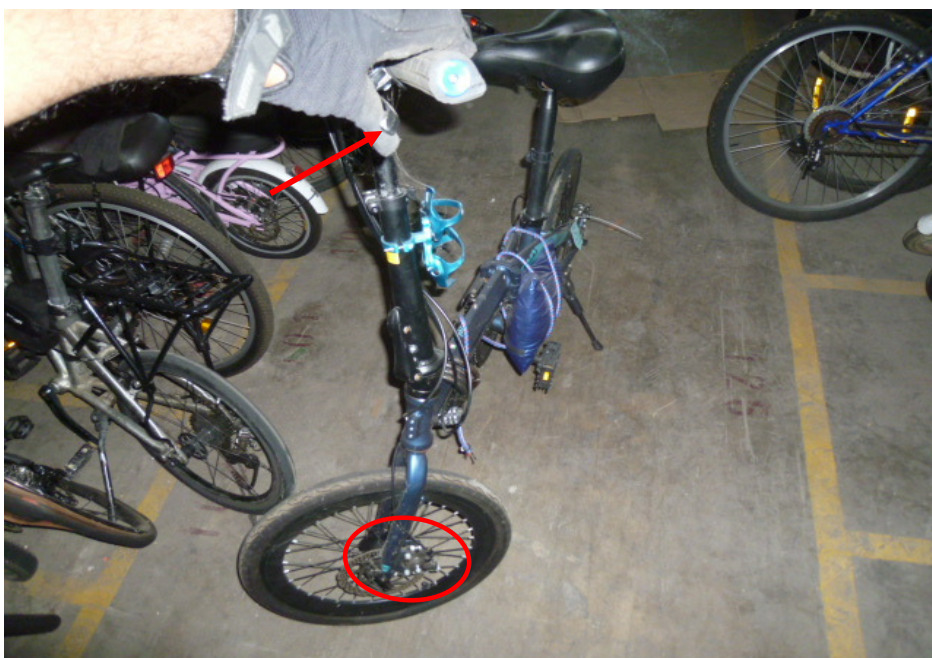
Photo 18 shows a static brake test conducted on the Bicycle's front brake. There was some resistance felt upon pressing the left hand brake lever (arrowed). It also shows that the front brake pads responded to the gripping action (circled) after depressing the left hand brake lever.
