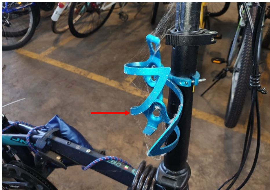
Photo 7 shows the deformed bottle holder (arrowed) of the Bicycle as a result of the accident.
