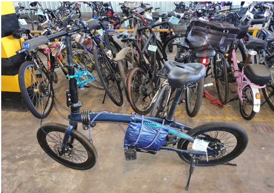
Photo 4 shows the left body of the Bicycle at the time of our inspection. The Bicycle had sustained damages all around. The body parts that were found to have been damaged include its left hand brake lever, right hand brake lever, handlebar grips, sub frame, bottle holder and right pedal, amongst others as a result of the accident.
