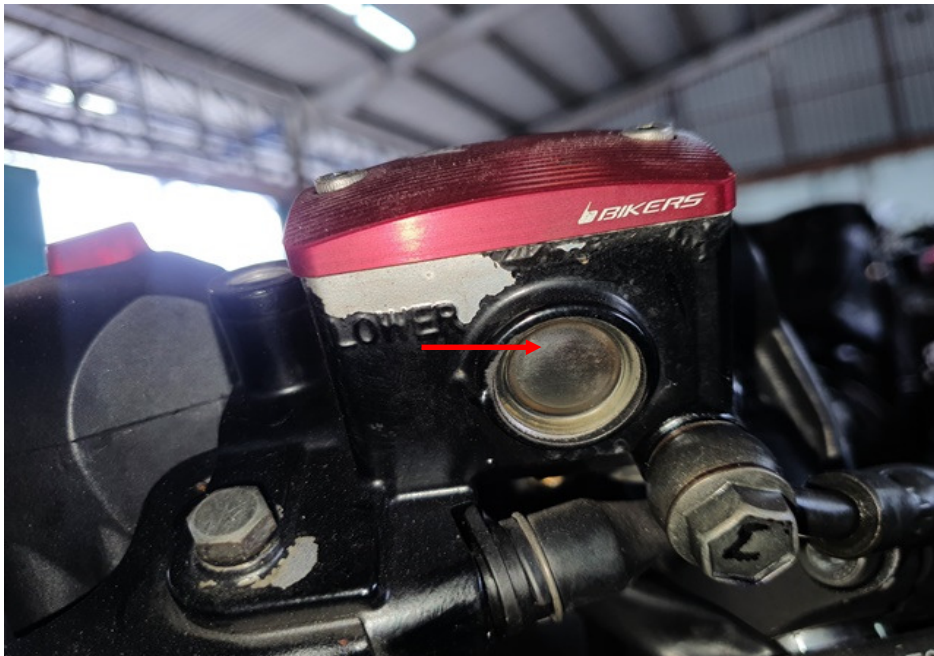
Photo 27 shows a close up view of the brake fluid reservoir for the front brake of the Motorcycle. The brake fluid was observed to be of sufficient level for operational purposes (arrowed).
