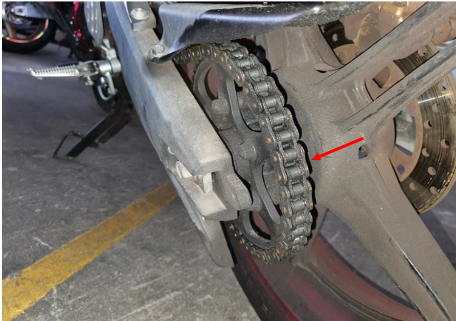
Photo 21 shows a closer view of the gear train (arrowed) of the Motorcycle, which was observed to be intact with no misalignment. It was also adequately lubricated for operating purposes.
