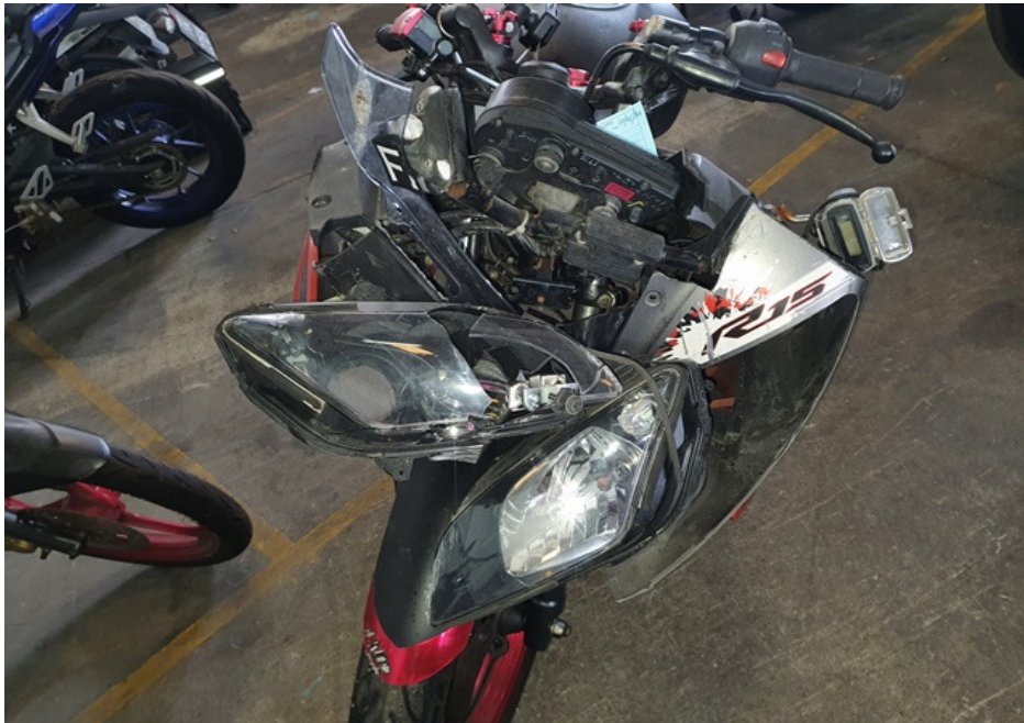
Photo 6 shows a close up view of the head cowl and headlight assembly which was amongst the body parts of the Motorcycle that had sustained damage as a result of the accident.
