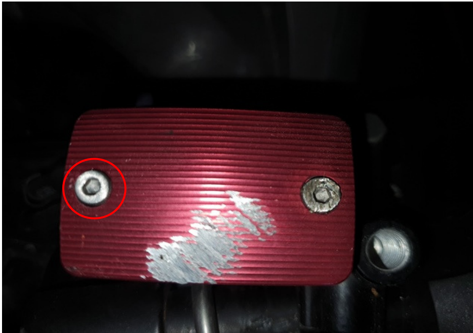
Photo 26 shows the brake fluid reservoir cover for the front brake of the Motorcycle. We were unable to examine whether the front brake fluid was without contamination due to the worn out screw (circled).
