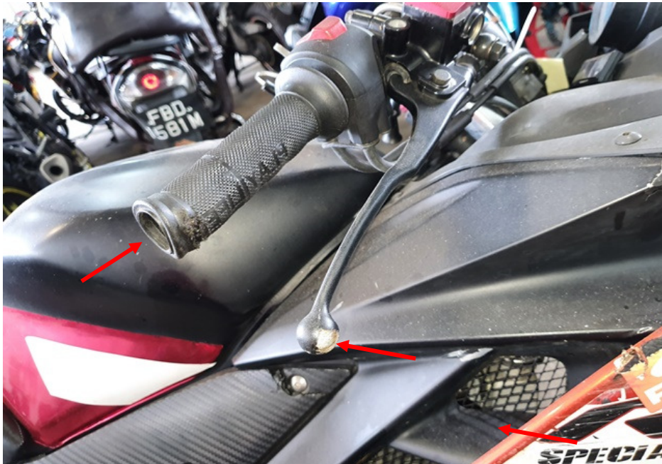
Photo 7 shows a closer view of right handlebar end and front brake lever (arrowed) which were amongst the body parts at the front body of the Motorcycle that had sustained damage as a result of the accident.
