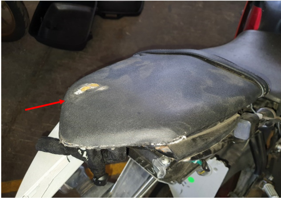
Photo 10 shows a closer view of the deformed pillion seat of the Motorcycle as a result of the accident (arrowed).
