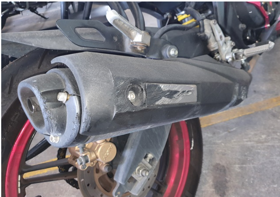
Photo 15 shows a closer view of the exhaust muffler heat shield of the Motorcycle that had sustained damages of grazing nature as a result of the accident.
