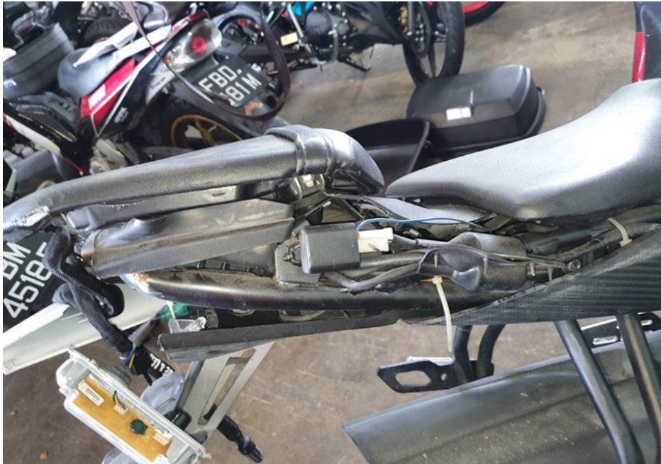
Photo 12 shows the missing right rear side cover of the Motorcycle as a result of the accident.
