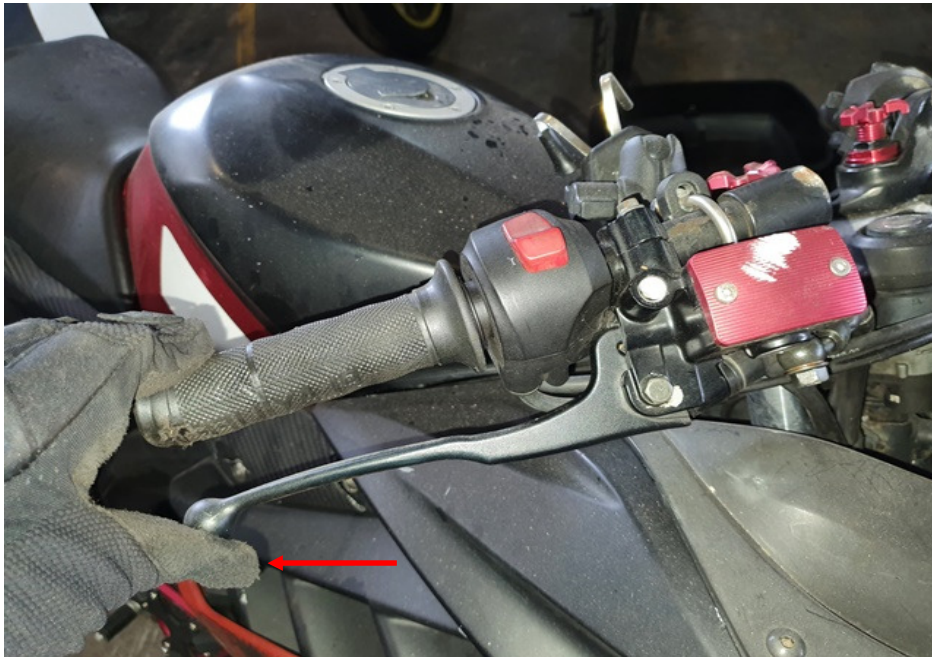
Photo 28 shows the front brake lever being depressed. There was some resistance felt (spongy like feel) upon pressing the front brake lever (arrowed). This would indicate that there is no leakage of pressure/vacuum in the front brake system.
