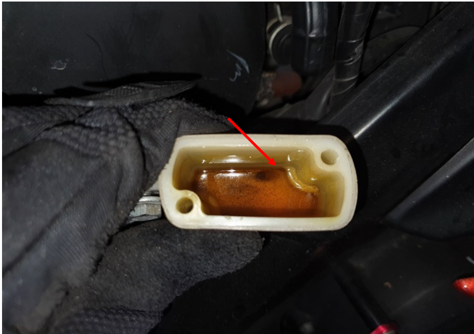
Photo 30 shows a close up view of the brake fluid reservoir for the rear brake of the Motorcycle. The brake fluid for the rear brake was found to be slightly contaminated. However it was observed not to be of sufficient level for operational purposes (arrowed).
