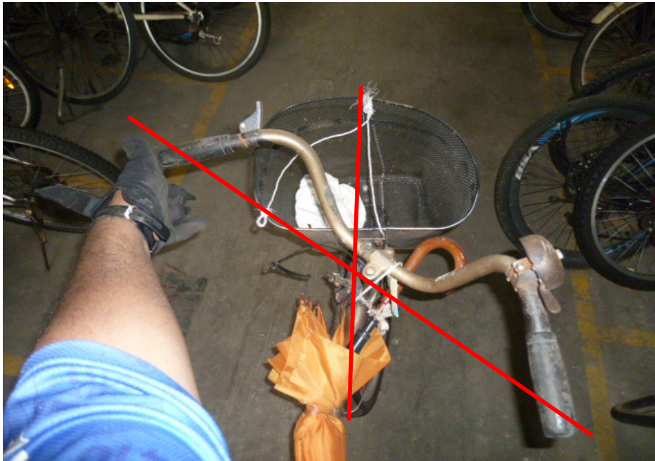
Photo 5 shows the frontal portion of the Bicycle (top view) at the time of our inspection. A misalignment of the handlebar & front tyre was observed.
