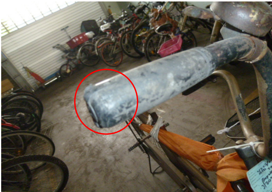
Photo 8 shows the damaged right handlebar grip of the Bicycle at the time of our inspection (circled).
