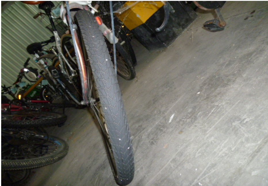
Photo 13 shows the front tyre of the Bicycle. The front tyre was observed to be in serviceable condition with remaining tread depth of approximately 3mm. There was no tear, burst mark(s) and/or punctured hole(s) on the sidewalls as well as across the tread of the front tyre. The front tyre was also observed to be sufficiently inflated for vehicular operation.
