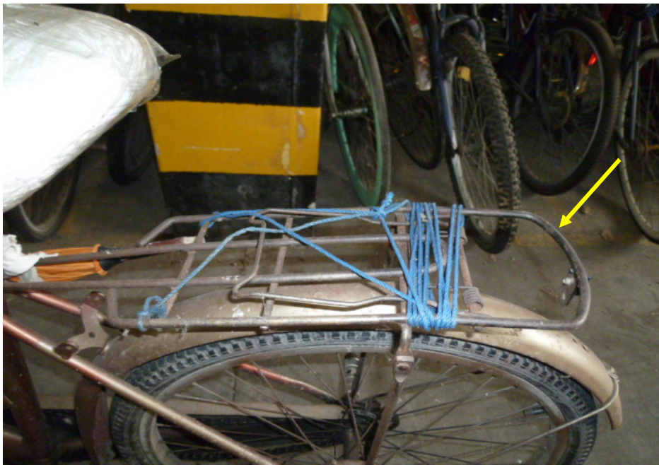
Photo 12 shows the deformed rack of the Bicycle as a result of the accident (arrowed).
