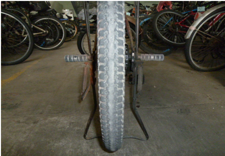
Photo 14 shows the rear tyre of the Bicycle. The rear tyre was observed to be in serviceable condition with remaining tread depth of approximately 3mm. The pattern of the tread was clearly visible. There was no tear, burst mark(s) and/or punctured hole(s) on the sidewalls as well as across the tread of the rear tyre. The rear tyre was also observed to be sufficiently inflated for vehicular operation.
