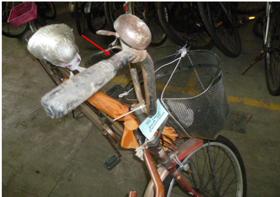
Photo 19 shows the right handlebar of the Bicycle. The right hand brake lever was observed to be missing as a result of the accident (arrowed). Hence a static brake test could not be conducted on the Bicycle's front braking system.
