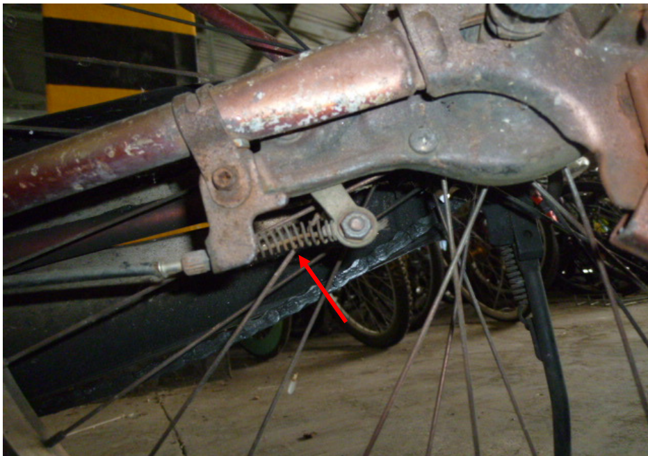
Photo 21 shows the rear wheel of the Bicycle. The type of brake system for the rear wheel was of a mechanical type, controlled by the left hand brake lever of the Bicycle. Our checks of the cable (arrowed), spring and drum which are all part of the components in the rear brake system of the Bicycle reveal all to be intact and without damage.
