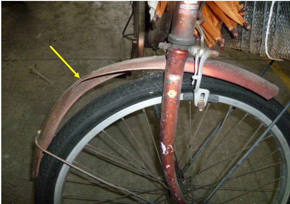
Photo 9 shows a close-up view of the deformed front mudguard of the Bicycle due to the accident (arrowed).
