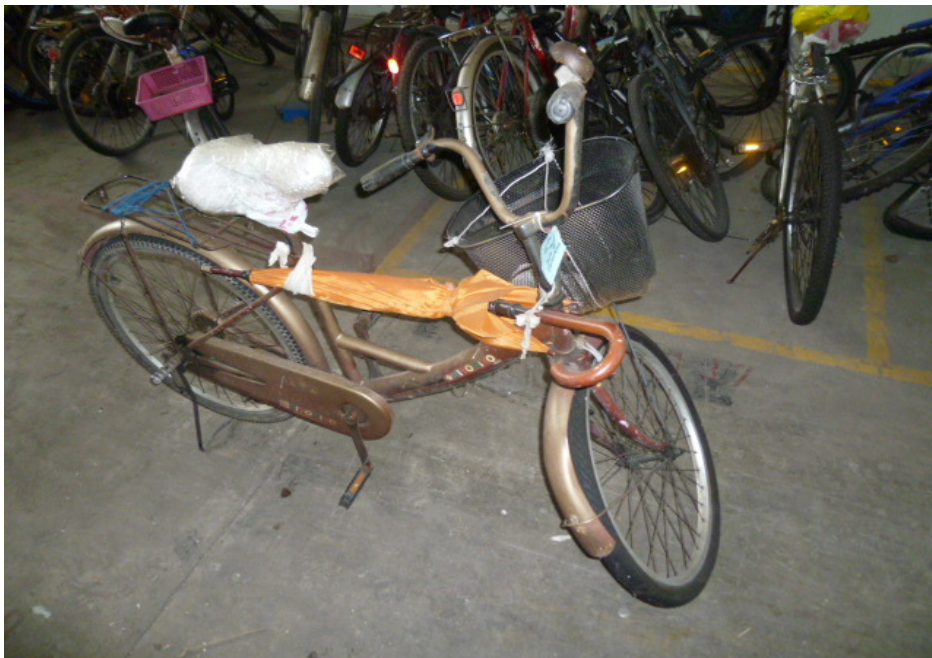
Photo 4 shows the right body of the Bicycle at the time of our inspection. The Bicycle had sustained damages all around. The body parts that were found to have been damaged include its handlebar, right handlebar grip, front basket, front fork assembly, front mudguard, left pedal, left pillion foot peg, braking components and rack, amongst others as a result of the accident.
