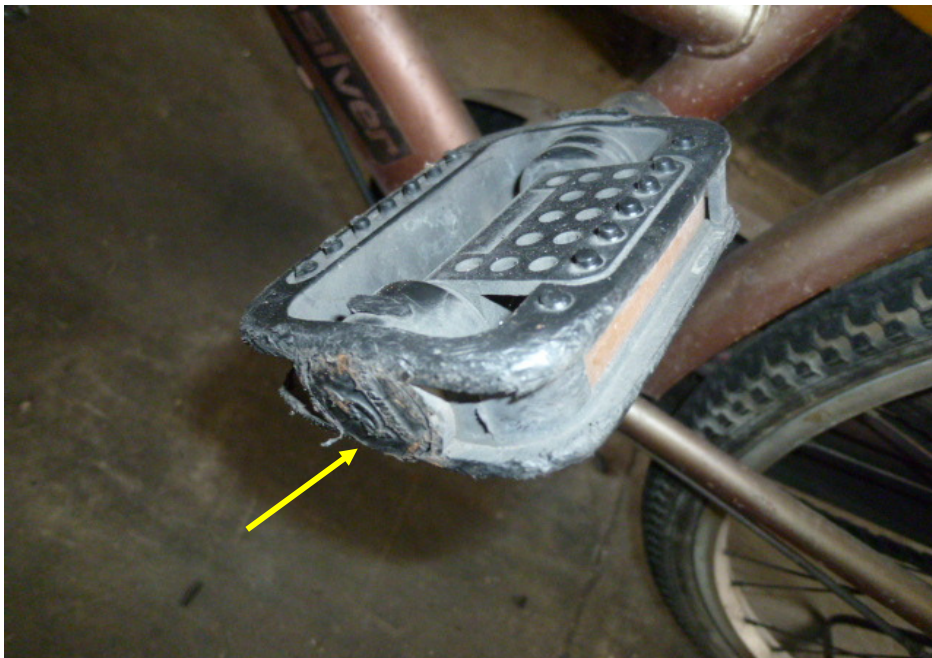
Photo 10 shows the left pedal of the Bicycle which had sustained damages of grazing nature as a result of the accident (arrowed).
