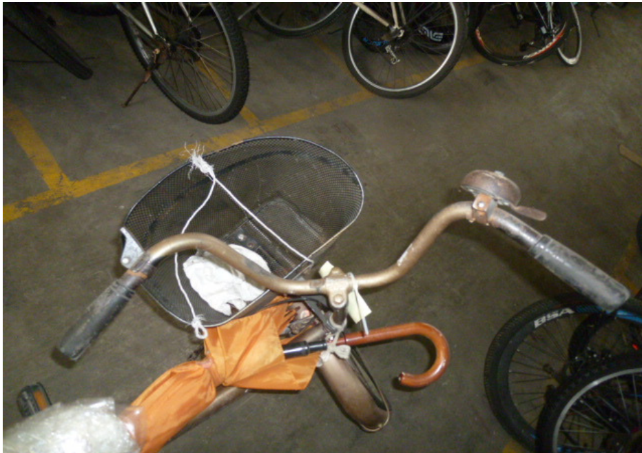
Photo 7 shows the deformed handlebar of the Bicycle at the time of our inspection.
