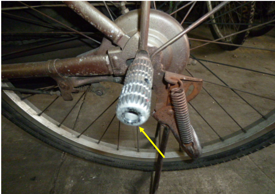
Photo 11 shows a close-up view of the left pillion foot peg of the Bicycle which had sustained damages of grazing nature as a result of the accident (arrowed).
