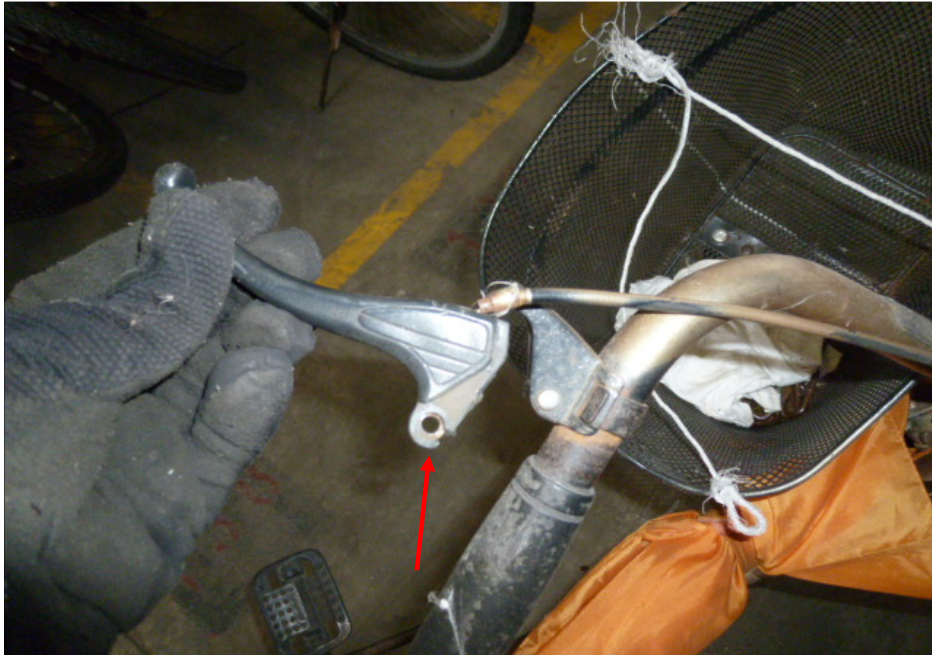
Photo 20 shows the left hand brake lever which was found to be broken due to the accident (arrowed). Hence a static brake test could not be conducted on the Bicycle's rear braking system.
