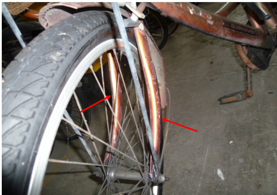
Photo 17 shows the front fork assembly of the Bicycle. The front forks of the Bicycle were found to be bent as a result of the accident (arrowed), hence causing the whole steering system to be out of alignment and rendering the Bicycle immobile for any static or operational tests.
