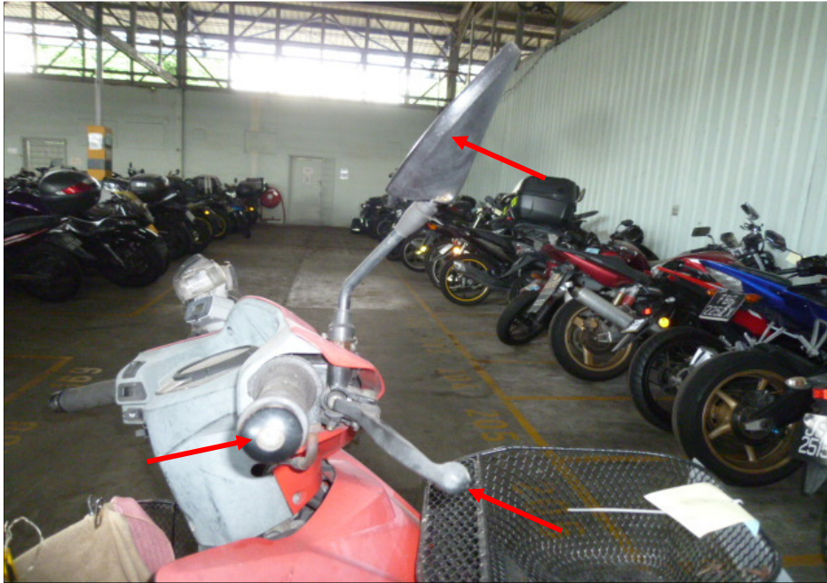
Photo 4 shows the right handlebar end, front brake lever and right side mirror (arrowed), which were amongst the body parts of the Motorcycle that had sustained damage as a result of the accident.
