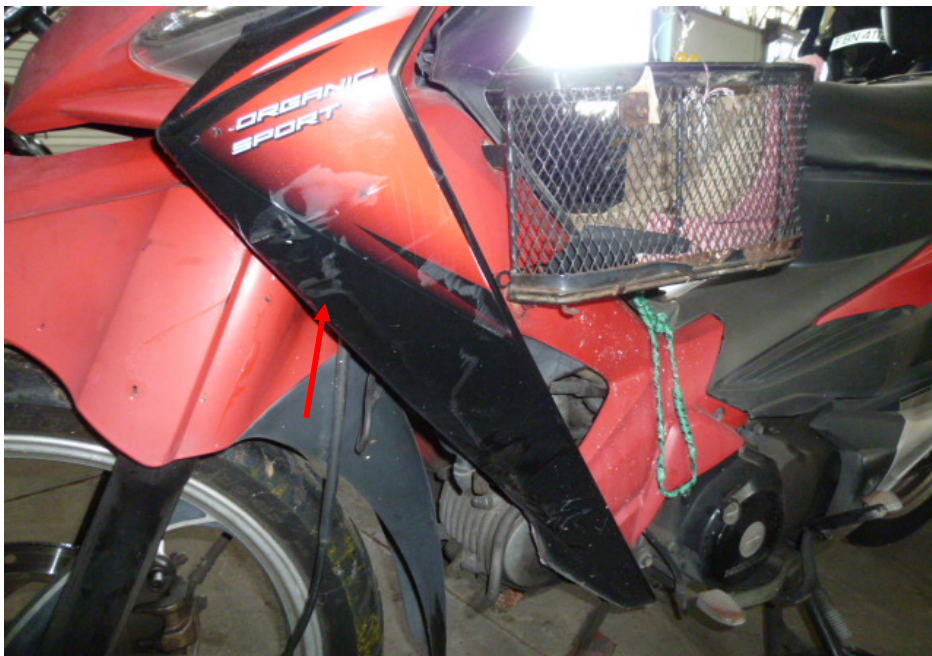
Photo 7 shows the left cowling (arrowed), which were amongst the body parts of the Motorcycle that had sustained damage as a result of the accident.
