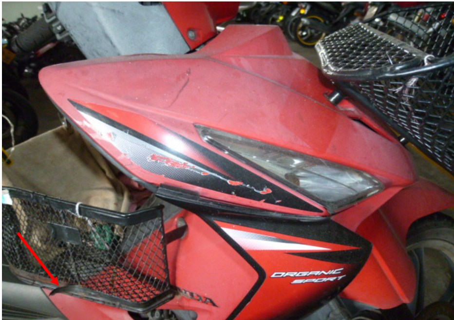
Photo 6 shows a closer view of the basket (arrowed) which was amongst the body parts of the Motorcycle that had sustained damage as a result of the accident.
