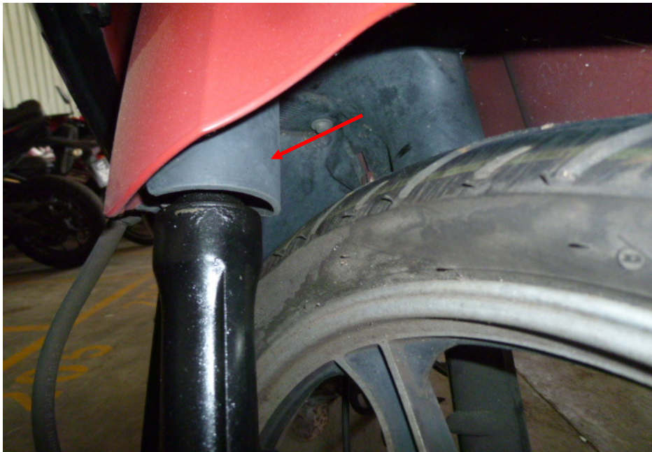
Photo 20 shows the right front fork (arrowed) of the Motorcycle. The right front fork and fork bracket of the Motorcycle were both found to be intact and undamaged. Turning the Motorcycle's handle bar towards the left and right did not produce any abnormal free play. The steering system of the Motorcycle was in serviceable condition at the time of our inspection.
