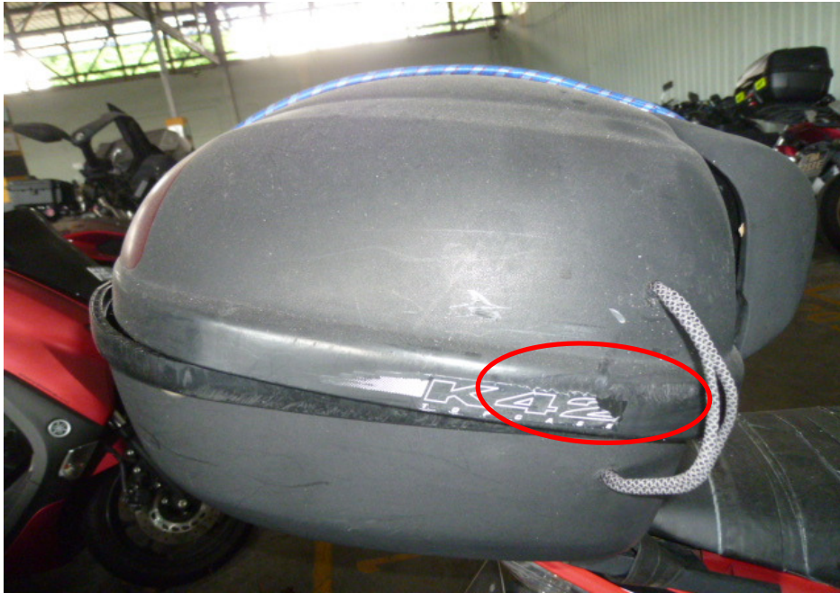
Photo 12 shows the top box of the Motorcycle that had sustained damage as a result of the accident (circled).
