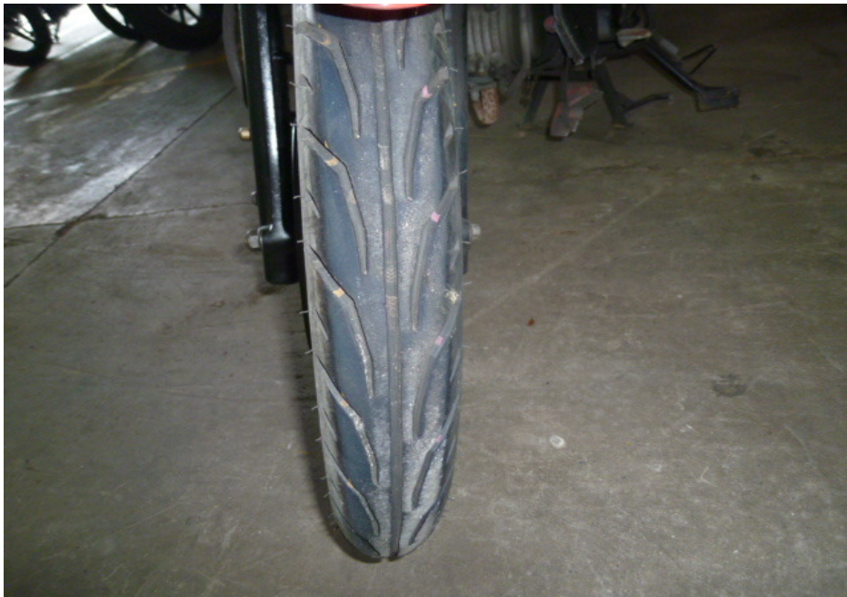
Photo 13 shows the front tyre of the Motorcycle at the time of our inspection. The front tyre was observed to be in serviceable condition with remaining tread depth of approximately 5mm. The pattern of the tread was also clearly visible. There was no tear, burst mark(s) and/or punctured hole(s) on the sidewalls as well as across the tread of the front tyre.
