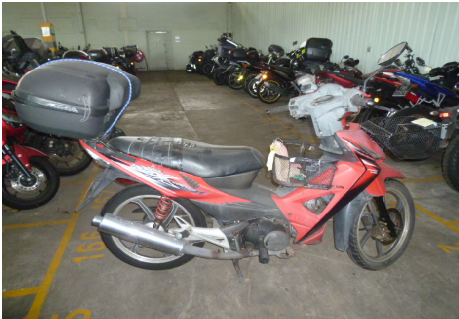
Photo 3 shows a general view of the right body of the Motorcycle at the time of our inspection. The Motorcycle was observed to have sustained damages all around. The body parts that were found to have been damaged include its front cowlings, side cowlings, side mirrors, handlebar ends, front brake lever, gear shift pedal, left front footrest and rear side covers, amongst others.
