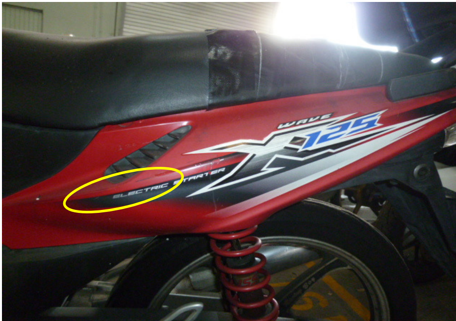
Photo 9 shows a closer view of the left rear side cover which was amongst the body parts of the Motorcycle that had sustained damages of grazing nature as a result of the accident (circled).
