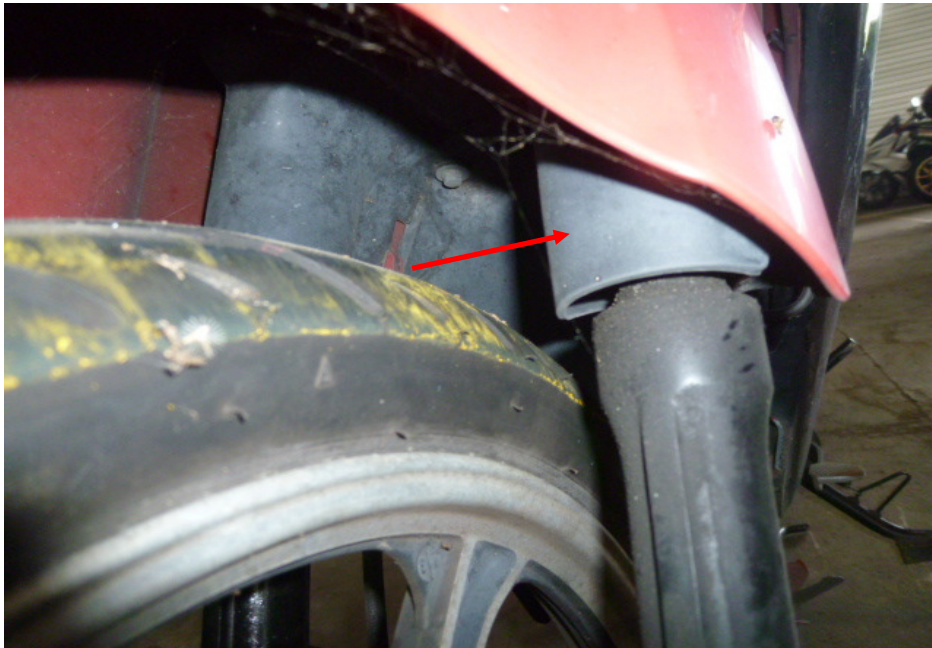
Photo 19 shows the left front fork (arrowed) of the Motorcycle. The left front fork and fork bracket of the Motorcycle were both found to be intact and undamaged. Turning the Motorcycle's handle bar towards the left and right did not produce any abnormal free play. The steering system of the Motorcycle was in serviceable condition at the time of our inspection.
