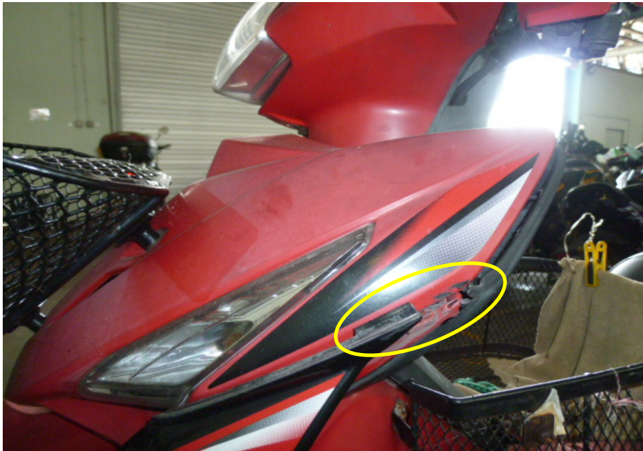
Photo 5 shows a closer view of the front cowling (circled) which was amongst the body parts of the Motorcycle that had sustained damage as a result of the accident.
