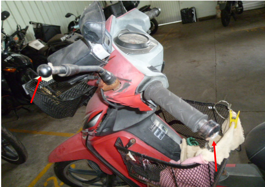
Photo 8 shows the left handlebar end and left side mirror (arrowed), which were amongst the body parts of the Motorcycle that had sustained damage as a result of the accident.
