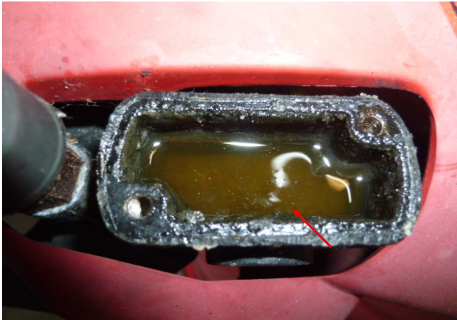
Photo 24 shows a close up view of the brake fluid reservoir for the front brake of the Motorcycle. The front brake fluid was observed to be of sufficient level for operational purposes. However it was found to be slightly contaminated (arrowed).
