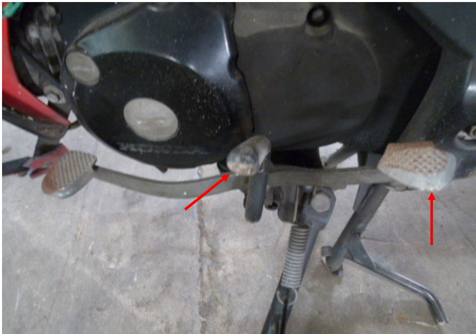
Photo 11 shows the grazed gear shift pedal and bent left front footrest of the Motorcycle as a result of the accident (arrowed).
