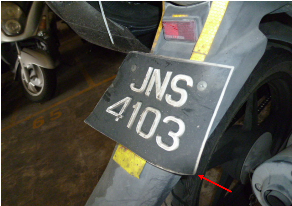
Photo 14 shows the dented rear number plate (arrowed) of the Motorcycle as a result of the accident.
