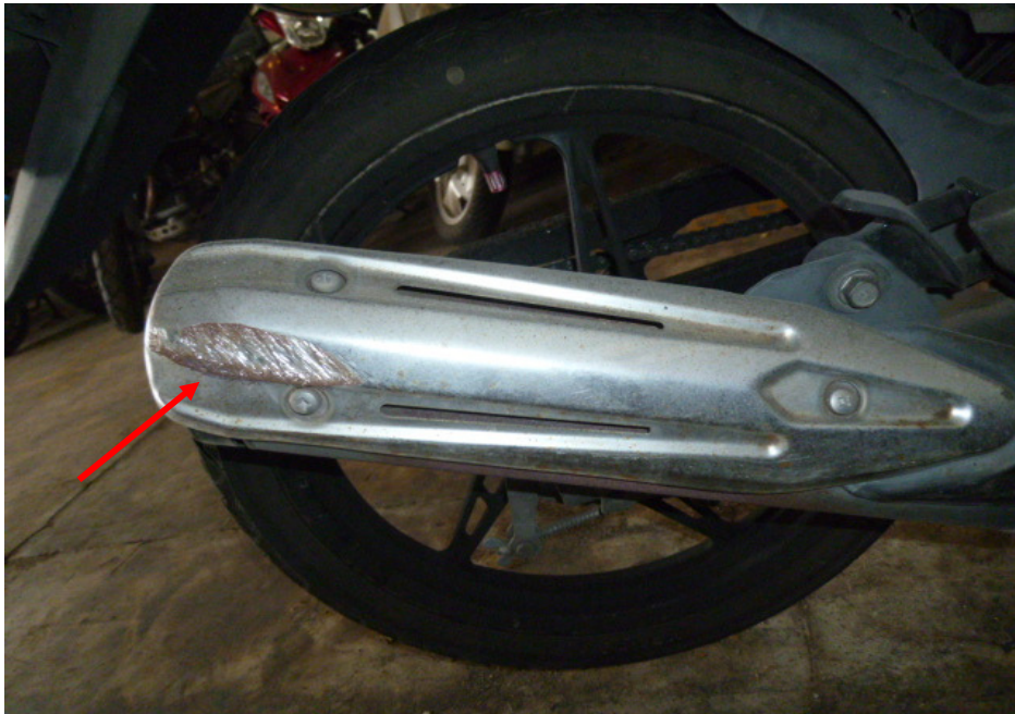
Photo 15 shows a closer view of the exhaust muffler heat shield which was amongst the body parts of the Motorcycle that had sustained damages of grazing nature as a result of the accident (arrowed).
