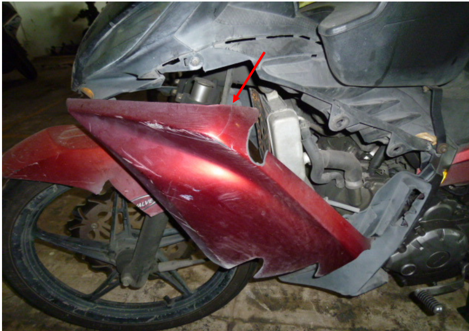
Photo 10 shows a closer view of the deformed left side cowling (arrowed) of the Motorcycle as a result of the accident.
