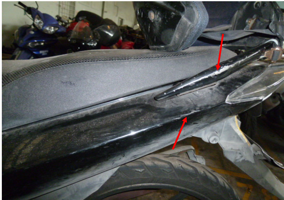
Photo 13 shows the grazed left pillion grab rail and left rear side cover (arrowed) of the Motorcycle as a result of the accident.
