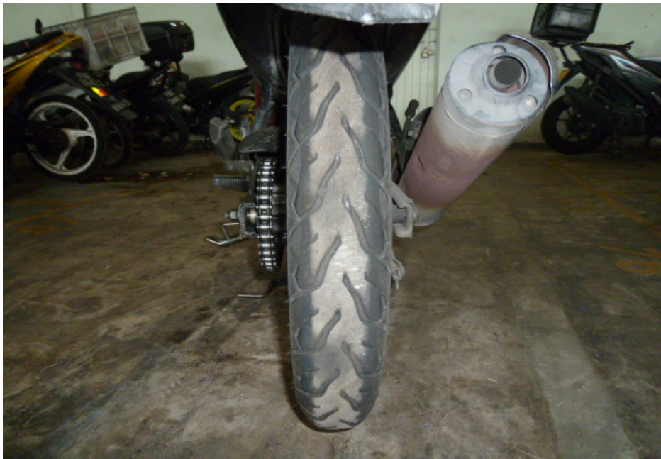
Photo 17 shows the condition of the Motorcycle's rear tyre. The rear tyre was observed to be in serviceable condition with remaining tread depth of approximately 3mm. The tyre was also observed to be sufficiently inflated for vehicular operation. We did not observe any tear, burst mark(s) and/or punctured hole(s) on the sidewalls as well as across the tread of the rear tyre.
