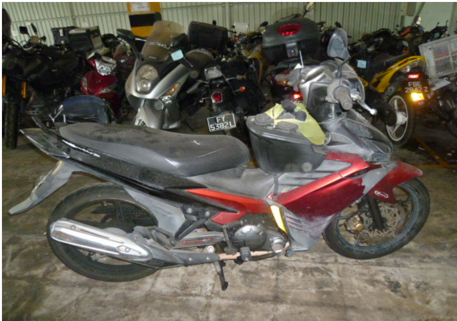
Photo 3 shows a general view of the right body of the Motorcycle at the time of our inspection. The Motorcycle was observed to have sustained damages all around. Amongst the body parts that were found to have been damaged include its head cowl, front mudguard, rear brake pedal, side cowlings, side mirrors, rear side covers, right front footrest and exhaust muffler heat shield, amongst others.
