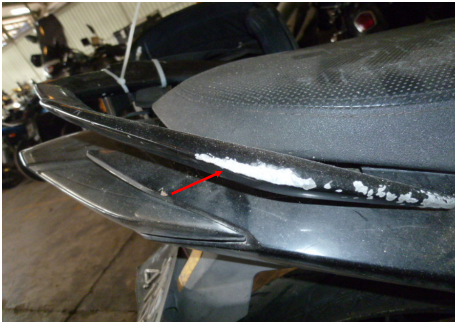
Photo 8 shows a closer view of the grazed right pillion grab rail (arrowed) of the Motorcycle as a result of the accident.
