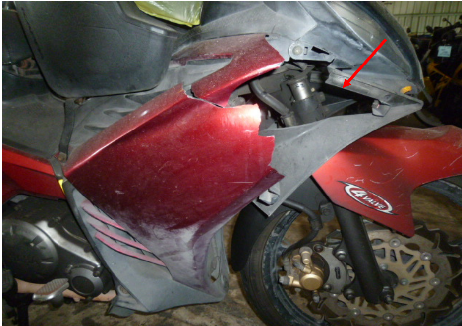
Photo 6 shows a closer view of the right cowling (arrowed) which was amongst the body parts of the Motorcycle that had sustained damage as a result of the accident.
