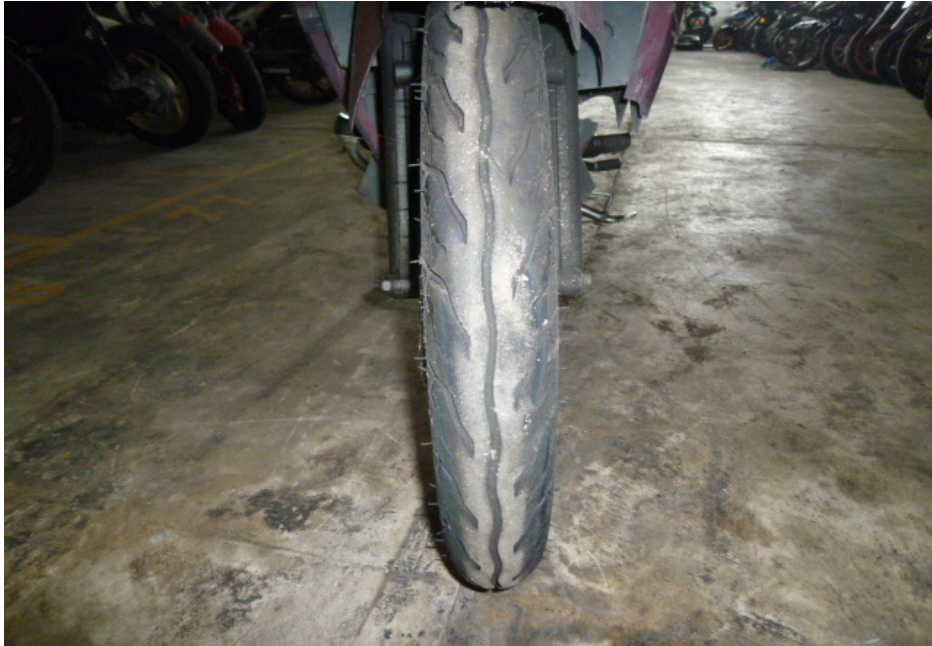
Photo 16 shows the front tyre of the Motorcycle at the time of our inspection. The front tyre was observed to be in serviceable condition with remaining tread depth of approximately 5mm. The pattern of the tread was also clearly visible. There was no tear, burst mark(s) and/or punctured hole(s) on the sidewalls as well as across the tread of the front tyre.
