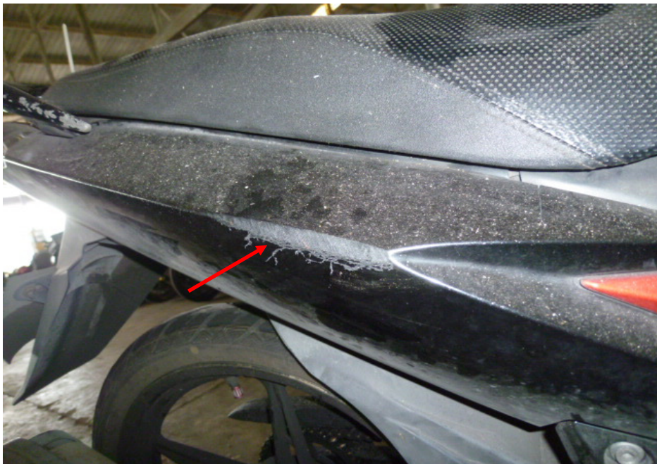
Photo 9 shows a closer view of the grazed right rear side cover (arrowed) of the Motorcycle as a result of the accident.
