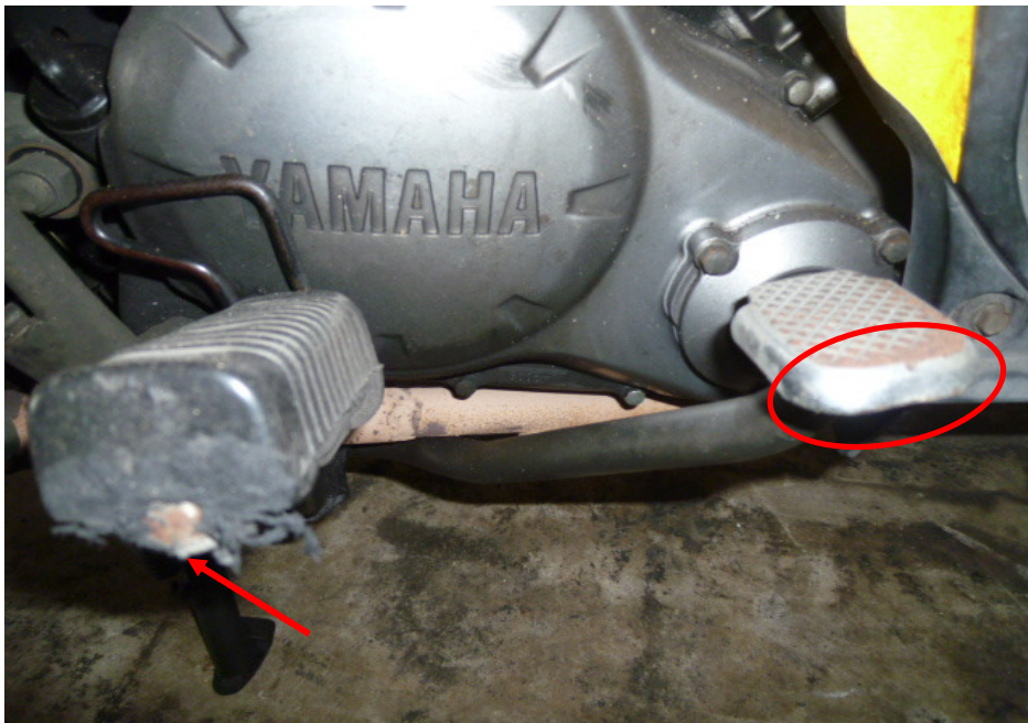
Photo 11 shows a closer view of the grazed rear brake pedal (circled) and right front footrest (arrowed) of the Motorcycle as a result of the accident.
