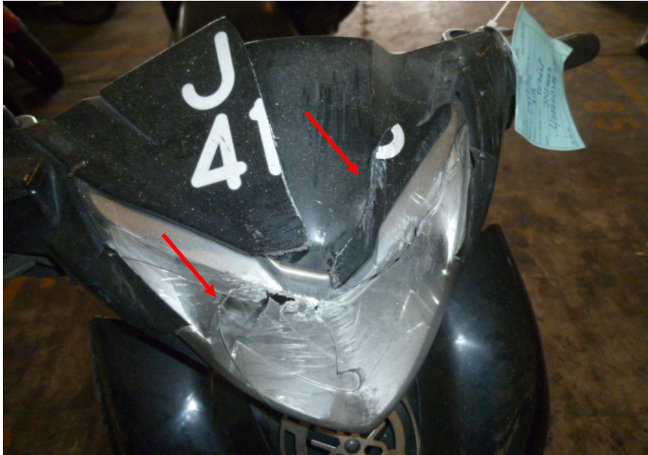
Photo 4 shows a closer view of the cracked head cowling and headlight assembly (arrowed) of the Motorcycle as a result of the accident.
