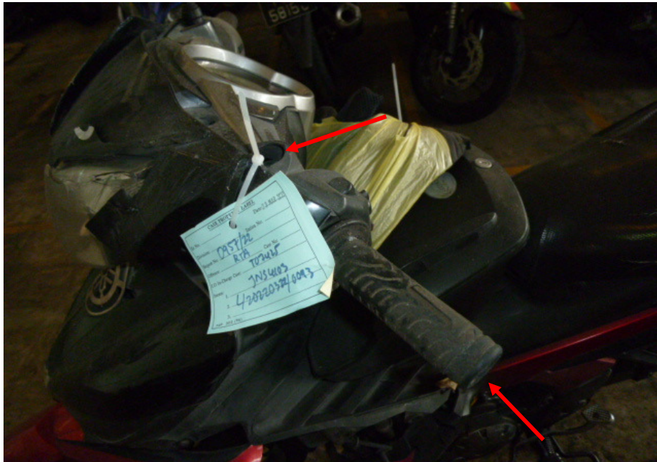
Photo 12 shows the left handlebar end and missing left side mirror (arrowed), which were amongst the body parts of the Motorcycle that had sustained damage as a result of the accident.
