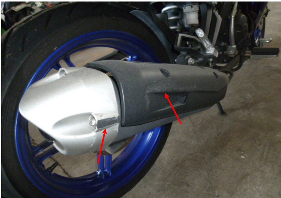
Photo 11 shows a closer view of the exhaust muffler heat shield which was amongst the body parts of the Motorcycle that had sustained damages of grazing nature as a result of the accident (arrowed).
