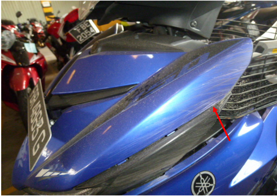
Photo 6 shows the front cowling (arrowed), which was amongst the body parts of the Motorcycle that had sustained damage as a result of the accident.
