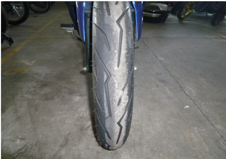
Photo 17 shows the front tyre of the Motorcycle at the time of our inspection. The front tyre was observed to be in serviceable condition with remaining tread depth of approximately 4mm. The pattern of the tread was also clearly visible. There was no tear, burst mark(s) and/or punctured hole(s) on the sidewalls as well as across the tread of the front tyre.
