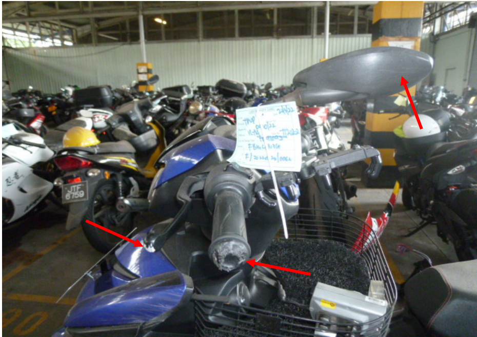
Photo 8 shows the left handlebar end, clutch lever and left side mirror (arrowed), which were amongst the body parts of the Motorcycle that had sustained damage as a result of the accident.
