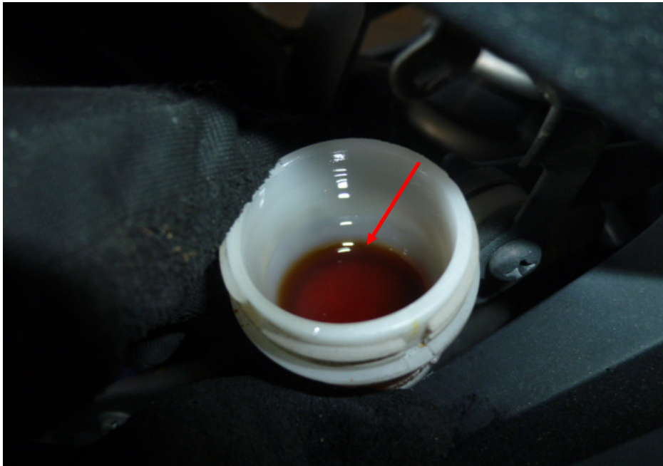
Photo 30 shows the brake fluid reservoir for the rear brake of the Motorcycle. The brake fluid was observed to be of sufficient level for operating purposes. However it was found to be slightly contaminated (arrowed).
