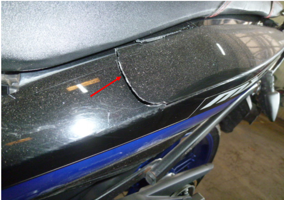
Photo 14 shows a closer view of the cracked left rear side cover of the Motorcycle as a result of the accident (arrowed).
