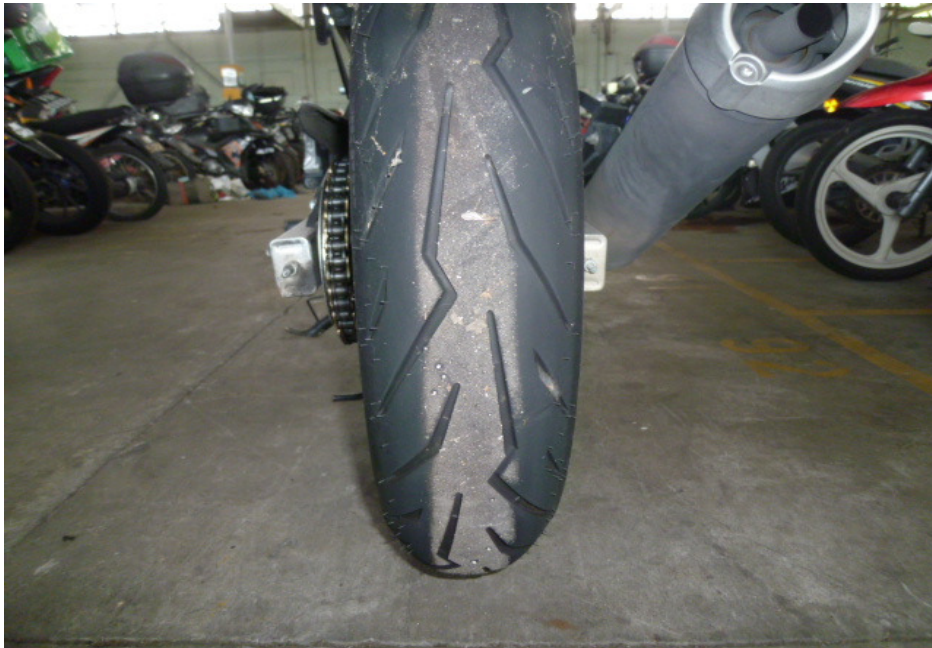
Photo 18 shows the condition of the Motorcycle's rear tyre. The rear tyre was observed to be in serviceable condition with remaining tread depth of approximately 5mm. The tyre was also observed to be sufficiently inflated for vehicular operation. We did not observe any tear, burst mark(s) and/or punctured hole(s) on the sidewalls as well as across the tread of the rear tyre.
