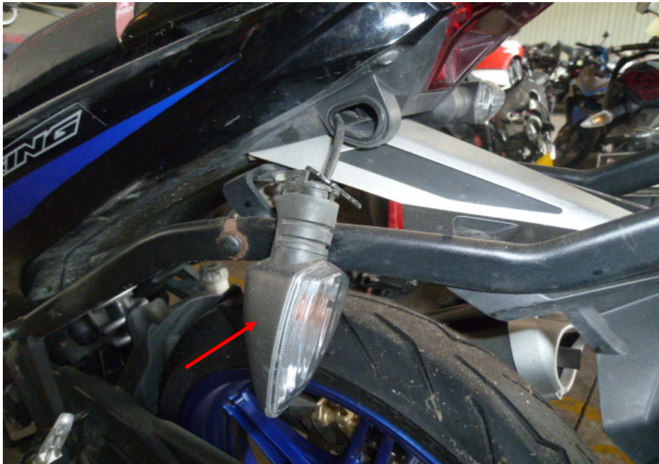
Photo 16 shows a closer view of the broken left signal lamp of the Motorcycle as a result of the accident (arrowed).
