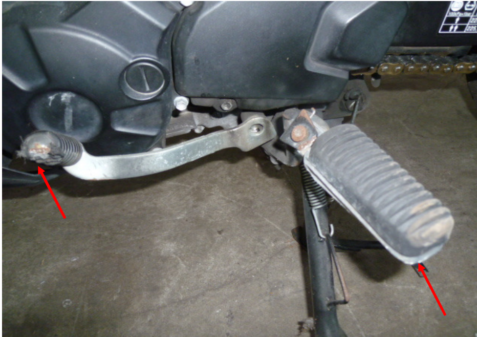
Photo 12 shows the bent gear shift pedal and left front footrest of the Motorcycle as a result of the accident (arrowed).
