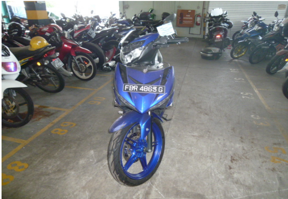
Photo 25 shows the front wheel of the Motorcycle turned towards its full right. Turning the Motorcycle's handle bar towards the right did not produce any abnormal free play and/or resistance. This would indicate that the steering system of the Motorcycle was in serviceable condition at the time of our inspection.
