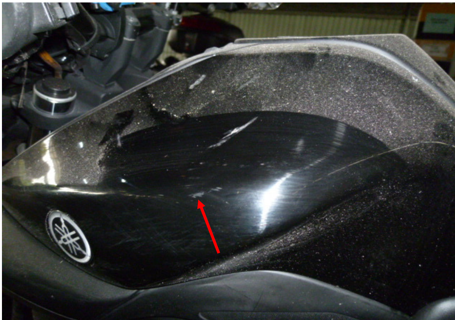
Photo 9 shows a closer view of the petrol tank of the Motorcycle as a result of the accident (arrowed).
