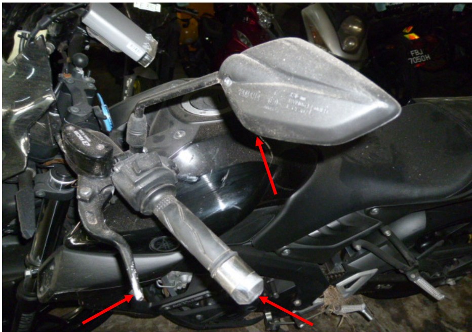
Photo 7 shows the left handlebar end, clutch lever and left side mirror (arrowed), which were amongst the body parts of the Motorcycle that had sustained damage as a result of the accident.
