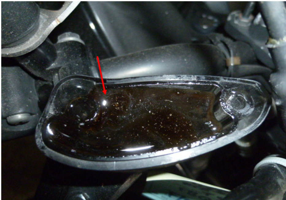
Photo 27 shows a close up view of the brake fluid reservoir for the front brake of the Motorcycle. The front brake fluid was observed to be of sufficient level for operational purposes. However it was found to be slightly contaminated (arrowed).
