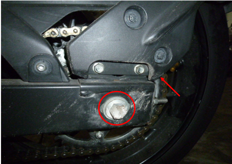
Photo 12 shows a closer view of the grazed rear sprocket nut (circled) and grazed rear wheel splash guard (arrowed) of the Motorcycle as a result of the accident.
