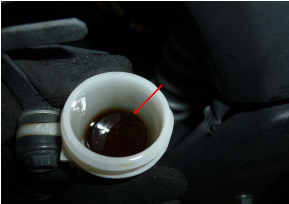
Photo 30 shows a close up view of the brake fluid reservoir for the rear brake of the Motorcycle. The rear brake fluid was observed to be of sufficient level for operational purposes. However it was found to be slightly contaminated (arrowed).
