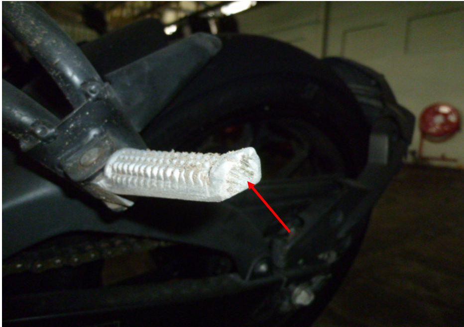
Photo 14 shows the grazed left pillion foot peg of the Motorcycle as a result of the accident (arrowed).
