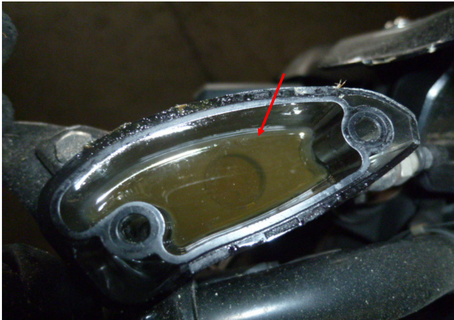
Photo 24 shows the hydraulic clutch fluid reservoir for the hydraulic clutch system of the Motorcycle. The hydraulic clutch fluid was observed to be of sufficient level for operational purposes. However it was found to be slightly contaminated (arrowed).
