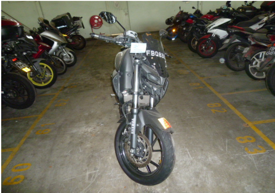
Photo 22 shows the front wheel of the Motorcycle turned towards its full left. Turning the Motorcycle's handle bar towards the left did not produce any abnormal free play and/or resistance. This would indicate that the steering system of the Motorcycle was in serviceable condition at the time of our inspection.
