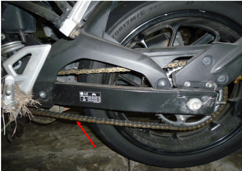
Photo 19 shows the general view of the gear chain (arrowed) of the Motorcycle, which was observed to be intact with no misalignment. It was also adequately lubricated for operating purposes. The gear chain rotates the rear wheel of the Motorcycle
