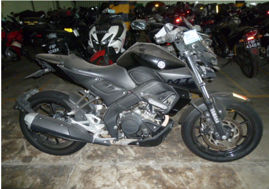
Photo 4 shows a general view of the right body of the Motorcycle at the time of our inspection. The Motorcycle was observed to have sustained damages all around. The body parts that were found to have been damaged include its head cowl, front mudguard, left cowl, right side mirror, front brake lever, gear shift pedal, right front footrest and rear sprocket nut, amongst others.
