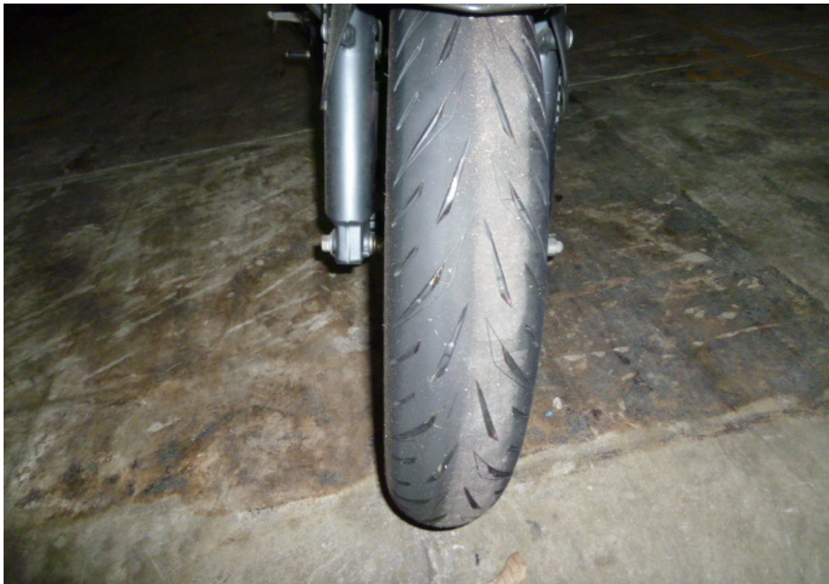
Photo 15 shows the front tyre of the Motorcycle at the time of our inspection. The front tyre was observed to be in serviceable condition with remaining tread depth of approximately 5mm. The pattern of the tread was also clearly visible. There was no tear, burst mark(s) and/or punctured hole(s) on the sidewalls as well as across the tread of the front tyre.
