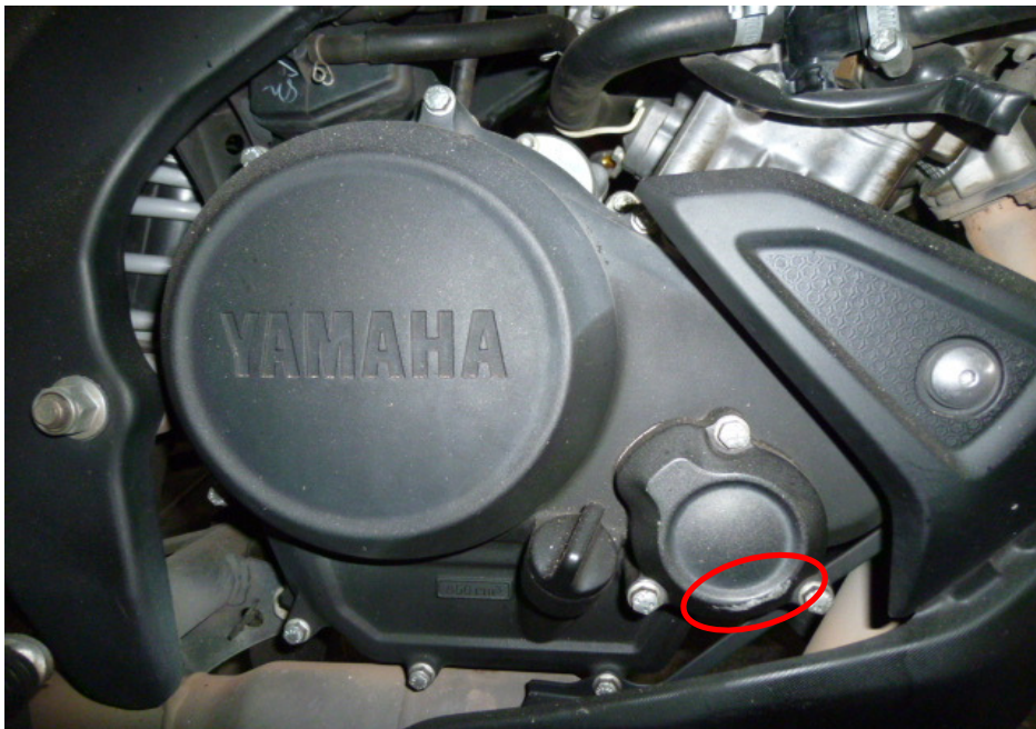
Photo 18 shows the right side of the engine of the Motorcycle at the time of our inspection. The various right engine components had sustained damage of grazing nature as a result of the accident (circled) however the engine components were still intact. There was also no fluid leak and/or fluid stain found around the right engine area of the Motorcycle.
