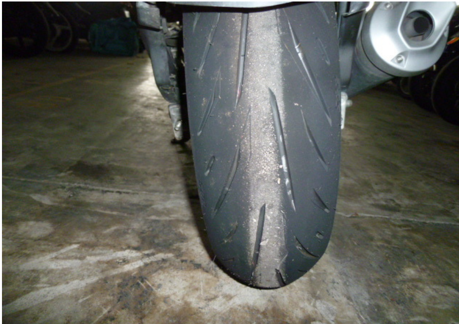
Photo 16 shows the condition of the Motorcycle's rear tyre. The rear tyre was observed to be in serviceable condition with remaining tread depth of approximately 8mm. The tyre was also observed to be sufficiently inflated for vehicular operation. We did not observe any tear, burst mark(s) and/or punctured hole(s) on the sidewalls as well as across the tread of the rear tyre.
