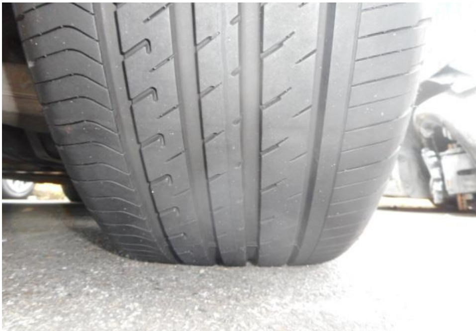
Photo 7 shows the condition of the rear right tyre of the Motor Car, which was observed to be in serviceable condition with remaining tread depth of approximately 7.1mm. The tyre, which was wrapped around standard alloy wheel rim, was also observed to be sufficiently inflated for vehicular operation.
