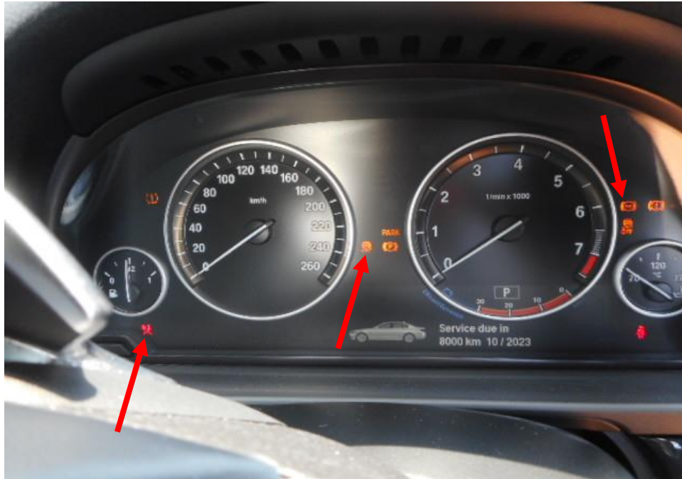
Photo 23 shows the warning light for Anti-Lock Brake System (ABS), Traction Control System (TCS), and Supplemental Restraint System (SRS) appearing on the instrument panel of the Motor Car during the self-test of its various electronic operating systems when its engine was cranked.
