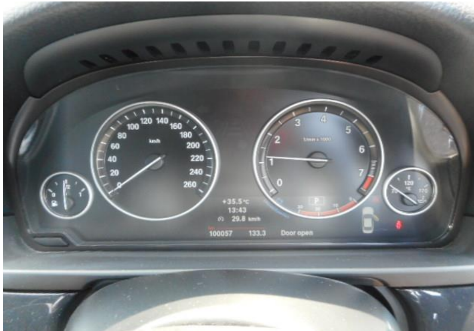
Photo 24 shows no warning lights illuminated on the instrument panel of the Motor Car after the engine was cranked. This would suggest that there was no abnormality to the various electronic operating systems of the Motor Car, like the ABS, TCS, and SRS.
