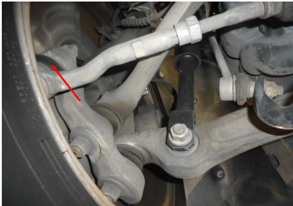
Photo 15 shows the various undercarriage components at the front right wheel of the Motor Car, in particular the steering tie rod end (arrowed). The various steering components were all found to be intact, suggesting that the steering system of the Motor Car was likely to be in serviceable condition at the material time of accident. There was also no sign of fluid stain(s) observed on the various undercarriage components.
