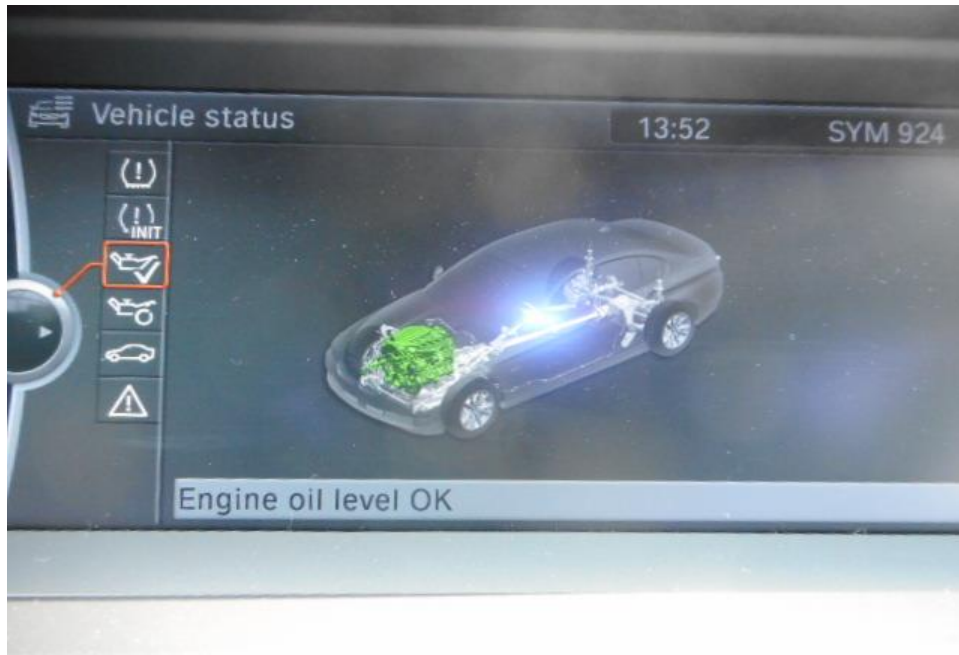
Photo 13 shows the engine oil level of the Motor Car at the time of my inspection. The engine oil was observed to be of sufficient level and without any visible contamination.
