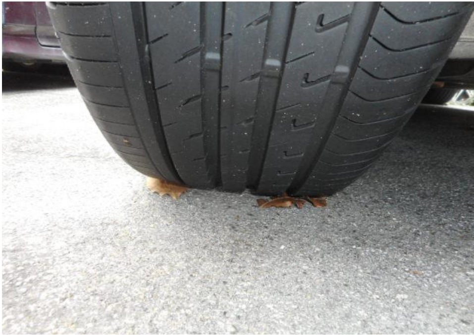
Photo 8 shows the condition of the rear left tyres of the Motor Car, which was observed to be in serviceable condition with remaining tread depth of approximately 6.9mm. The tyres, which were wrapped around standard alloy wheel rim, were also observed to be sufficiently inflated for vehicular operation. There was also no damage found on all 4 alloy wheel rims of the Motor Car.
