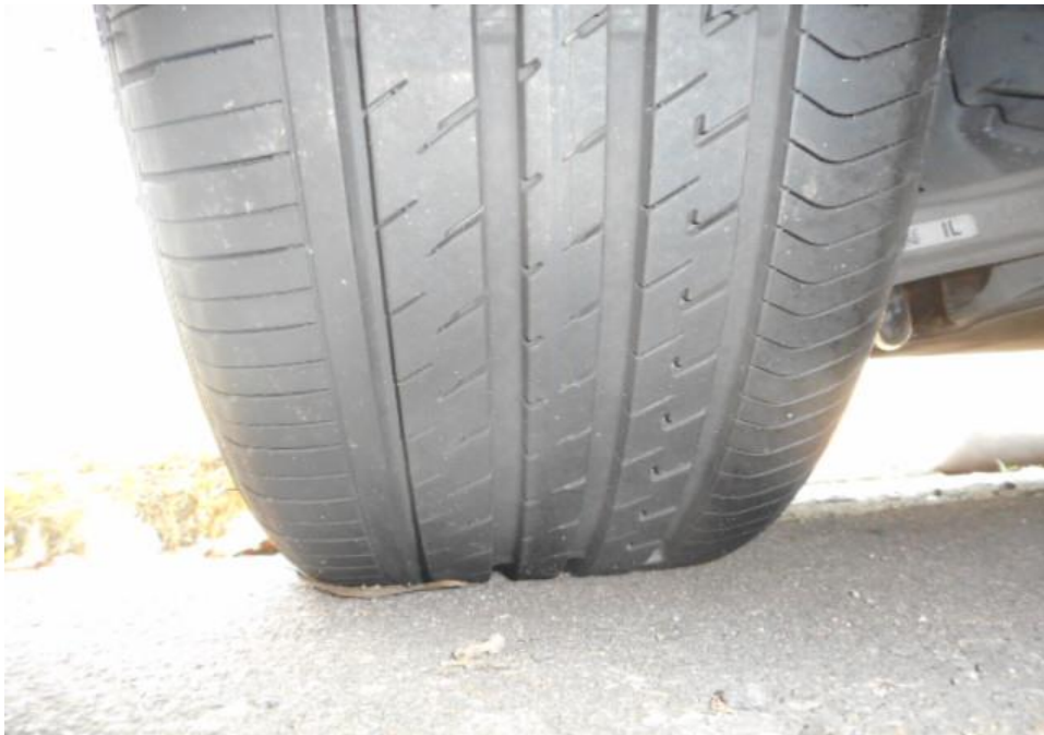
Photo 9 shows the condition of the rear right tyres of the Motor Car, which were observed to be in serviceable condition with remaining, tread depth of approximately 7.3mm. There was also no tear, cut or burst mark(s) on the outer and the inner sidewalls as well as across the tread of the 4 tyres that were fitted on the Motor Car.
