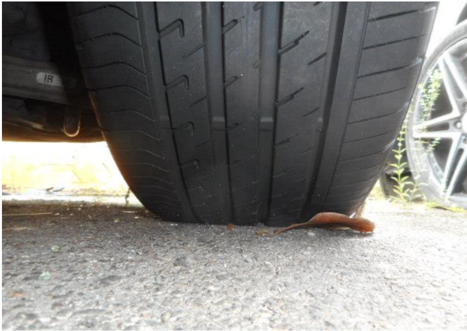
Photo 6 shows the condition of the front right tyre of the Motor Car, which was observed to be in serviceable condition with remaining tread depth of approximately 7.2mm. The tyre, which was wrapped around standard alloy wheel rim, was also observed to be sufficiently inflated for vehicular operation. There was no tear, cut or burst mark(s) on the outer and the inner sidewalls as well as across the tread of the 4 tyres that were fitted on the Motor Car.
