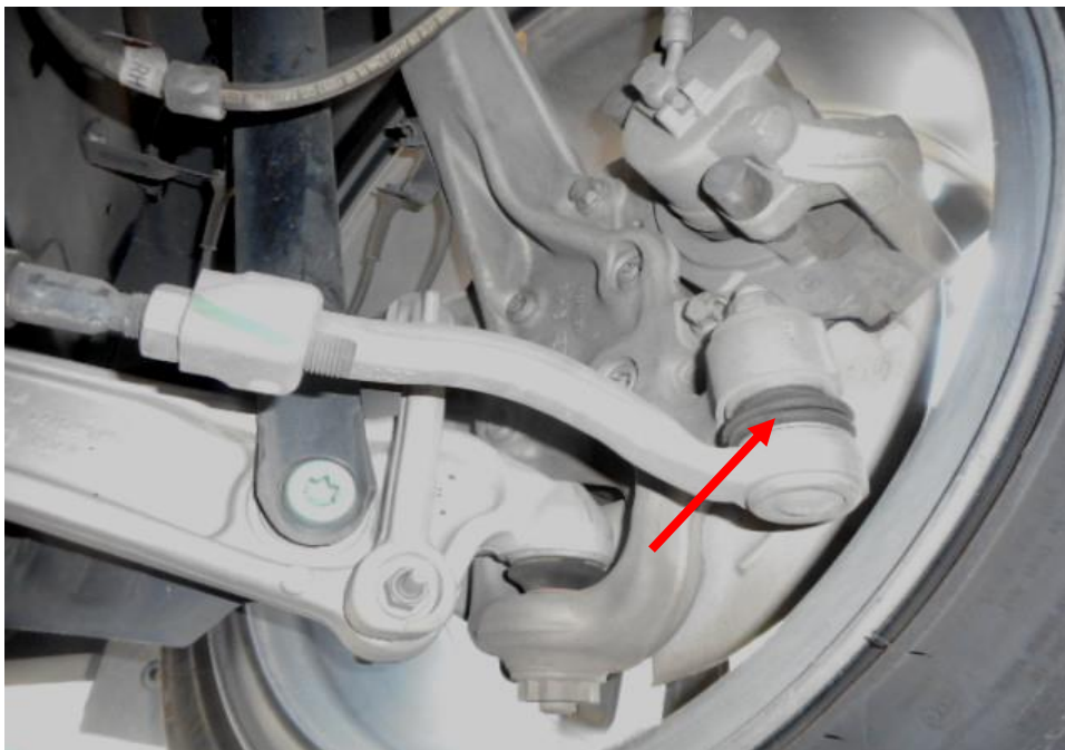
Photo 21 shows the various undercarriage components at the front right wheel of the Motor Car, in particular the steering tie rod (red arrow). The various steering components were all found to be intact, suggesting that the steering system of the Motor Car was likely to be in serviceable condition at the material time of accident. There was also no sign of fluid stain observed on the various undercarriage components at the front right wheel of the Motor Car.
