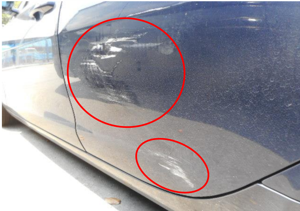
Photo 4 shows a close up view of the Motor Car's left body at the time of my inspection. The rear portion of the Motor Car was observed to have sustained damage. Its left rear door panel (circled) was the body part that were damaged as a result of the accident.
