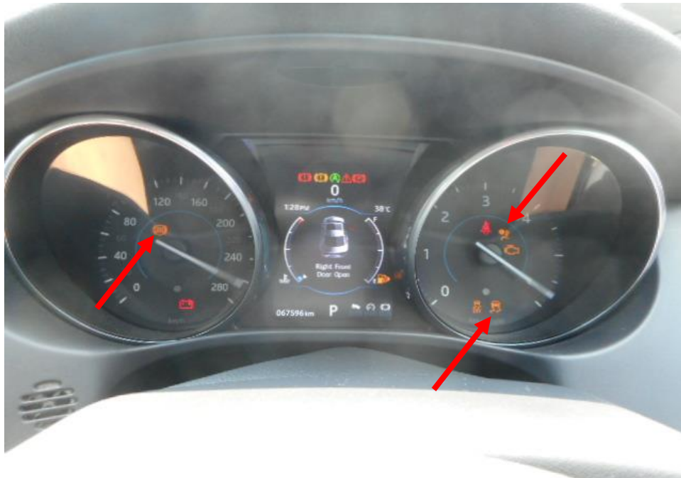
Photo 24 shows the warning light for Anti-Lock Brake System (ABS), Traction Control System (TCS), and Supplemental Restraint System (SRS) (arrowed) appearing on the instrument panel of the Motor Car during the self-test of its various electronic operating systems when its engine was cranked.
