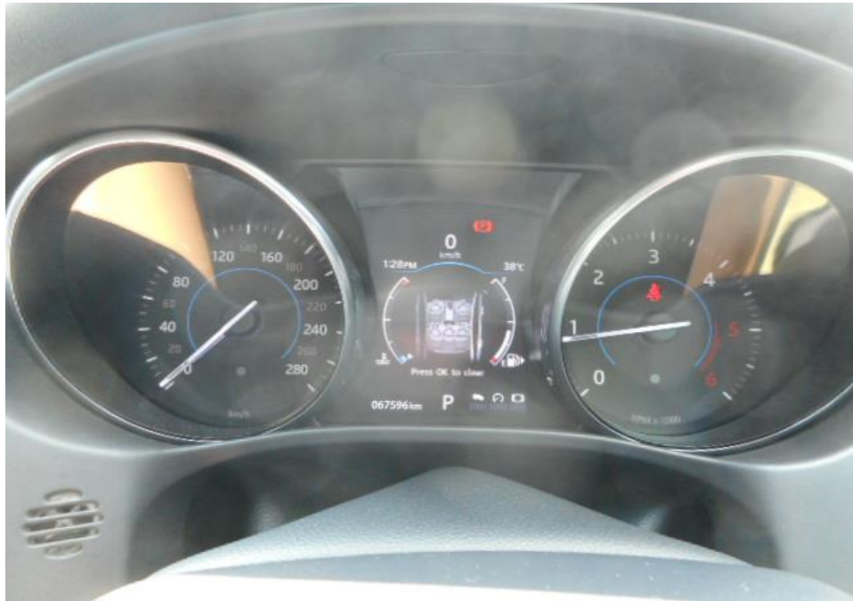
Photo 25 shows no warning lights illuminated on the instrument panel of the Motor Car after the engine was cranked. This would suggest that there was no abnormality to the electronic operating system of the Motor Car, like the ABS, TCS and SRS etc.
