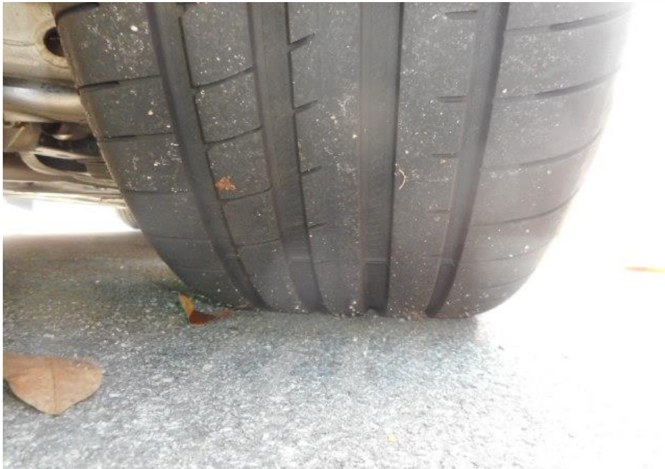
Photo 8 shows the condition of the rear right tyre of the Motor Car, which was observed to be in serviceable condition with remaining tread depth of approximately 6.6mm. The tyre was also observed to be sufficiently inflated for vehicular operation with no tear, cut or burst mark(s).
