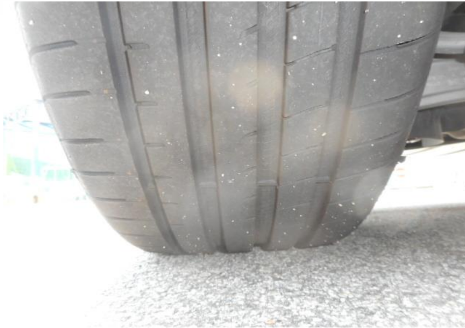
Photo 10 shows the condition of the front left tyre of the Motor Car, which was observed to be in serviceable condition with remaining tread depth of approximately 6.4mm. There was also no tear, cut or burst mark(s) on the outer and the inner sidewalls as well as across the tread of the Motor Car's 4 tyres.
