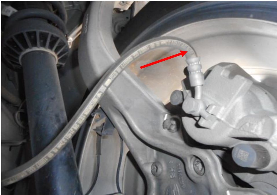
Photo 18 shows the brake hose/pipe (arrowed) at the front right wheel of the Motor Car. I did not observe any leakage of brake fluid at the time of my inspection of the Motor Car. Static tests of the Motor Car's braking system had indicated that there was no internal leakage of pressure/vacuum.
