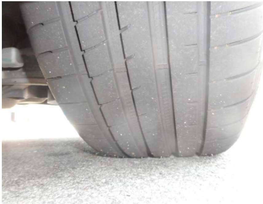
Photo 7 shows the condition of the front right tyre of the Motor Car, which was observed to be in serviceable condition with remaining tread depth of approximately 6.8mm. The tyre was sufficiently inflated for vehicular operation with no tear, cut or burst mark(s) on the outer and the inner sidewalls as well as across the tread. The 4 tyres of the Motor Car were wrapped around standard steel wheel rims without any damage.
