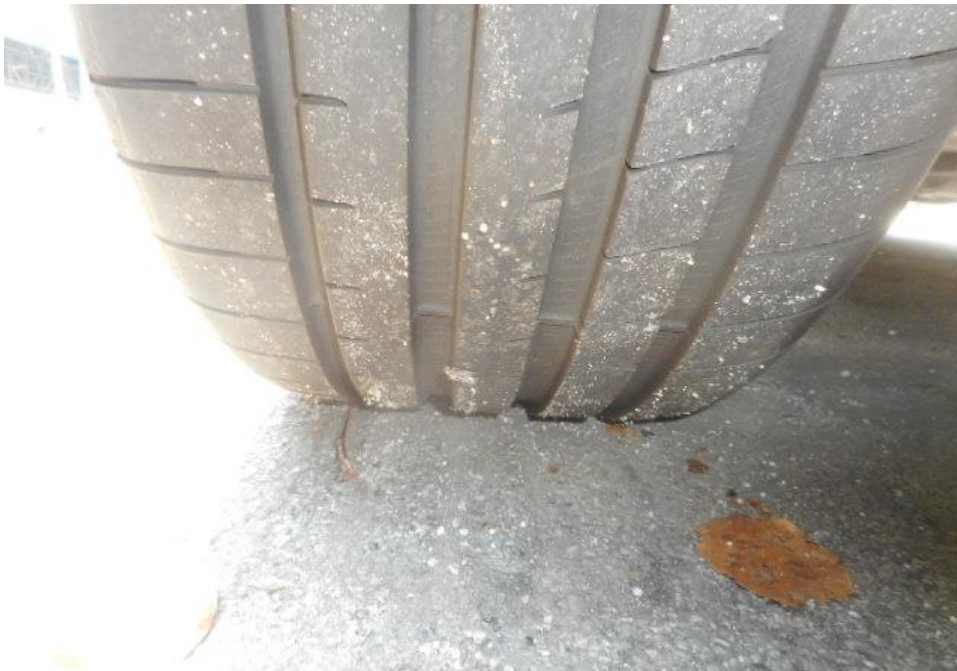
Photo 9 shows the condition of the rear left tyre of the Motor Car, which was observed to be in serviceable condition with remaining tread depth of approximately 6.9mm. The tyre, which was wrapped around steel wheel rim, was also observed to be sufficiently inflated for vehicular operation. The 4 tyres of the Motor Car were wrapped around standard steel wheel rims.
