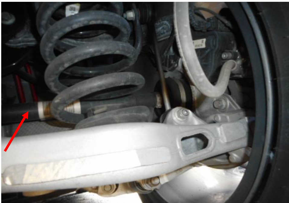
Photo 23 shows the various undercarriage components at the rear right wheel of the Motor Car, in particular the drive shaft (arrowed). The various components were all found to be intact, suggesting that the driveshaft of the Motor Car was likely to be in serviceable condition at the material time of accident. There was also no sign of fluid stain observed on the various undercarriage components at the rear right wheel of the Motor Car.
