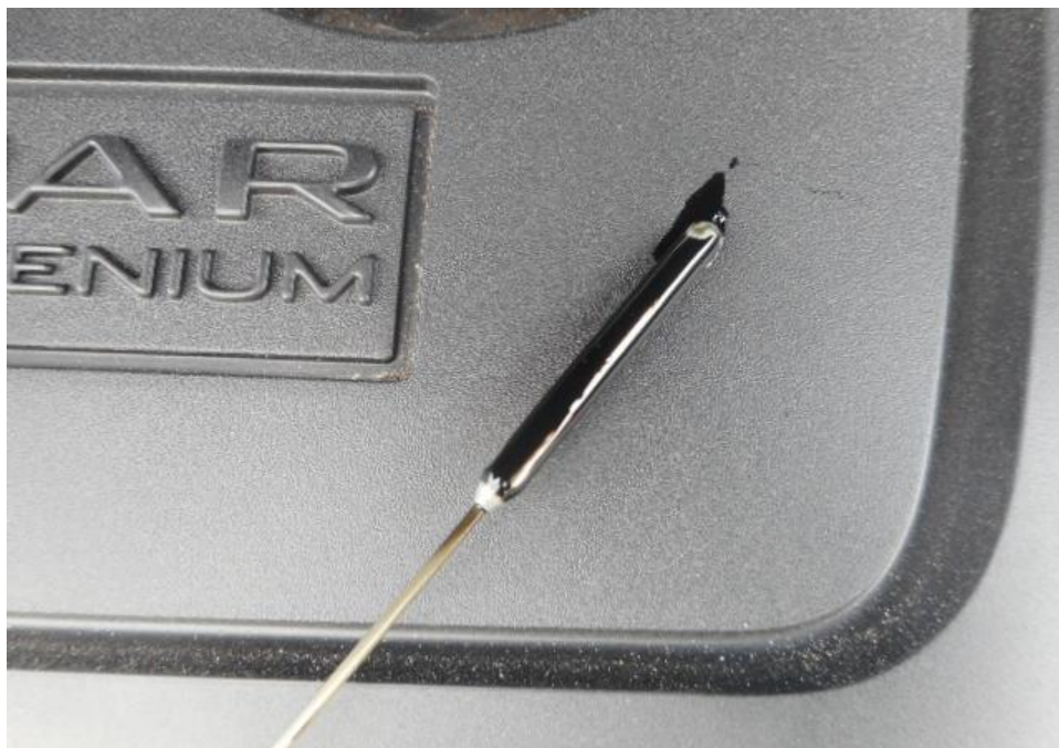
Photo 14 shows the engine oil dipstick of the Motor Car at the time of my inspection. The engine oil was observed to be of sufficient level and without any visible contamination.
