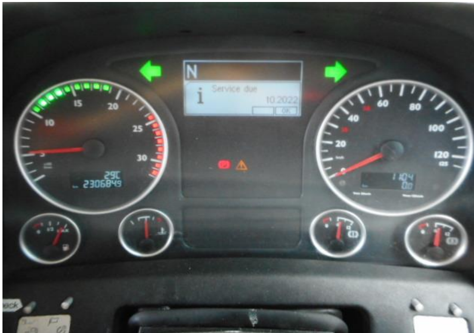
Photo 26 shows no warning lights illuminated on the instrument panel of the Motor Bus after the engine was cranked. This would suggest that there was no abnormality to the various electronic operating systems of the Motor Bus, like the TCS, ABS and etc.
