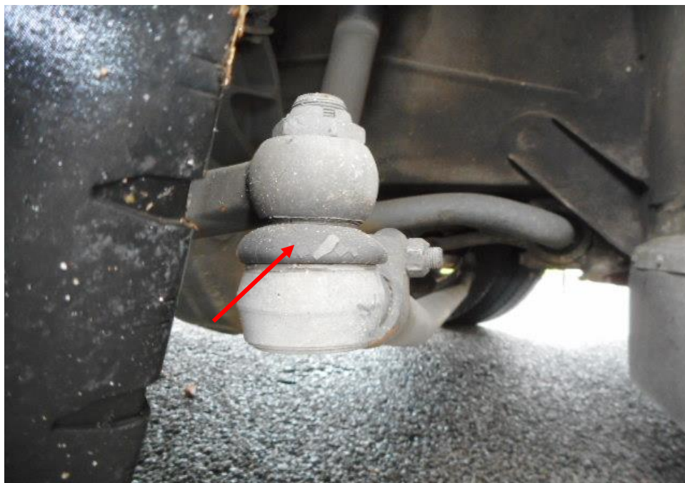
Photo 21 shows the various undercarriage components at the front left wheel of the Motor Bus, in particular the steering tie rod end (arrowed). The various undercarriage components of the Motor Bus were all found to be intact without any visible damage. There was also no sign of fluid stain(s) observed on the various undercarriage components.
