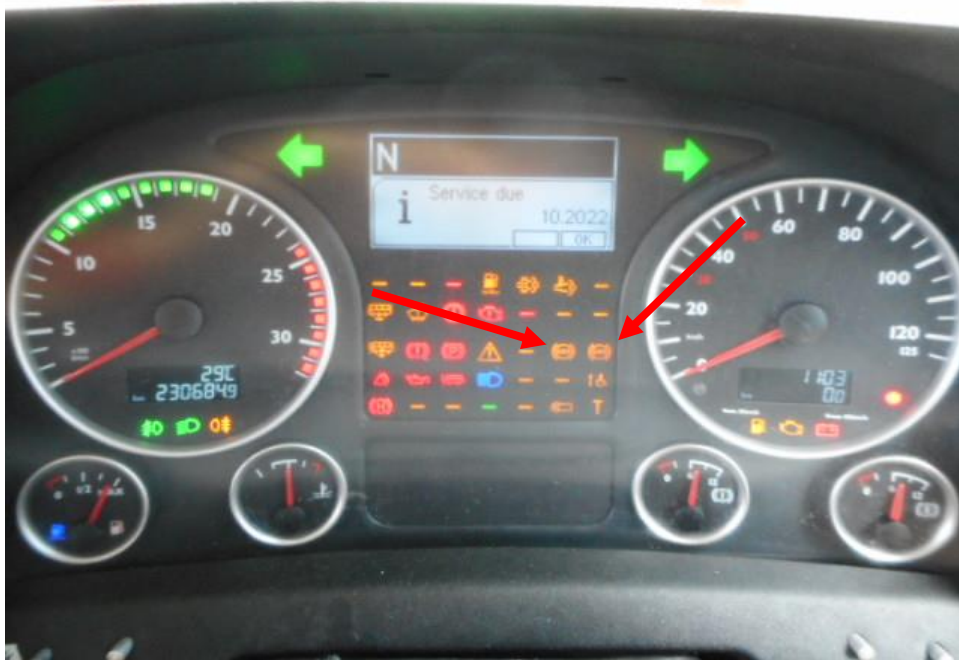
Photo 25 shows the warning light for Traction Control System (TCS) and Anti-Lock Braking System (ABS) appearing on the instrument panel of the Motor Bus during the self-test of its various electronic operating systems when its engine was cranked.
