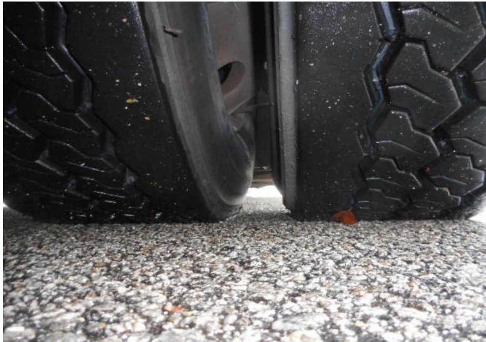
Photo 8 shows the condition of the rear right tyre of the Motor Bus, which was observed to be in serviceable condition with remaining tread depth of approximately 14mm. The tyre, which was wrapped around standard steel wheel rim, was also observed to be sufficiently inflated for vehicular operation.
