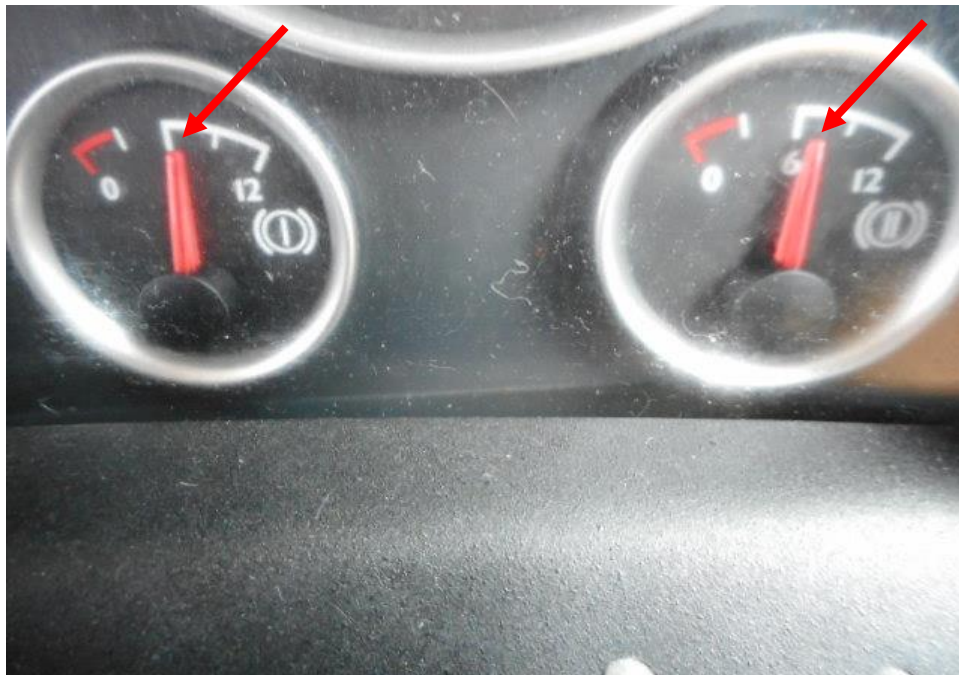
Photo 12 shows the air in the air brake cylinder of the Motor Bus at the time of my inspection. The air in the cylinder was observed to be of sufficient level & serviceable at the time of the accident.
