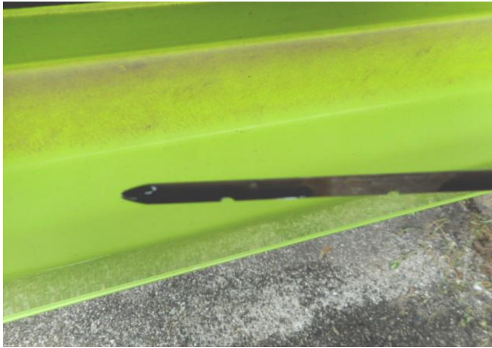
Photo 15 shows the engine oil dip stick system of the Motor Bus at the time of my inspection. The engine oil was observed to be sufficient for operation and without any visible contamination.
