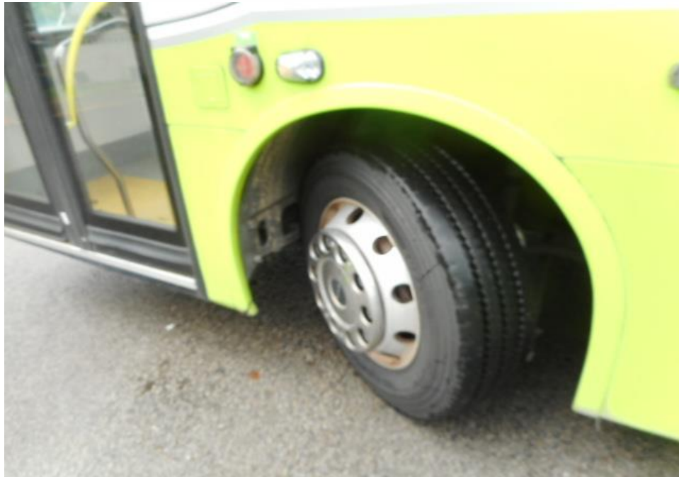
Photo 10 shows the condition of the front left tyres of the Motor Bus, which were observed to be in serviceable condition with remaining tread depth of approximately 14.4mm. There was also no tear, cut or burst mark(s) on the outer and the inner sidewalls as well as across the tread of the 8 tyres that were fitted on the Motor Bus.
