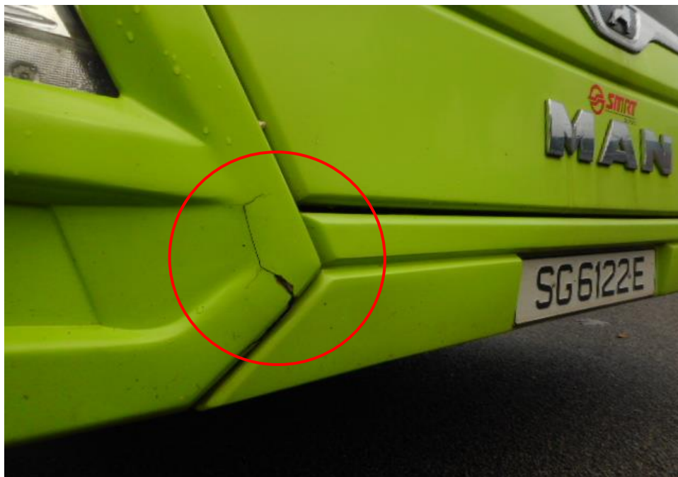
Photo 3 shows a close up view of the front body of the Motor Bus at the time of our inspection. The Motor Bus was observed to have sustained damages at its front bumper (circled) as a result of the accident.
