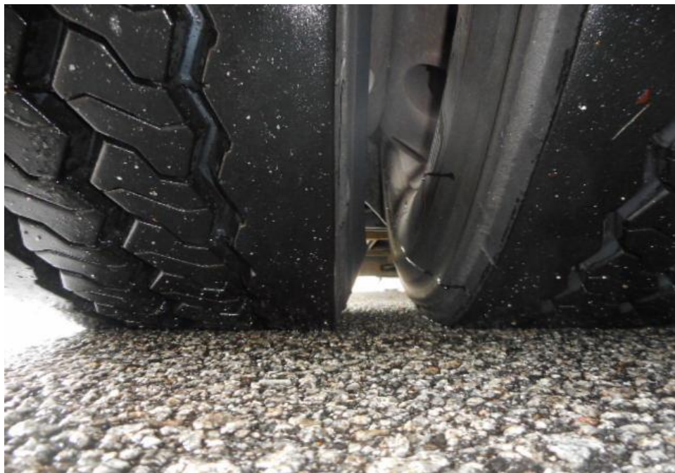
Photo 9 shows the condition of the rear left tyres of the Motor Bus, which was observed to be in serviceable condition with remaining tread depth of approximately 14.4mm. The tyres, which were wrapped around standard steel wheel rim, were also observed to be sufficiently inflated for vehicular operation. There was also no damage found on all 8 steel wheel rims of the Motor Bus.
