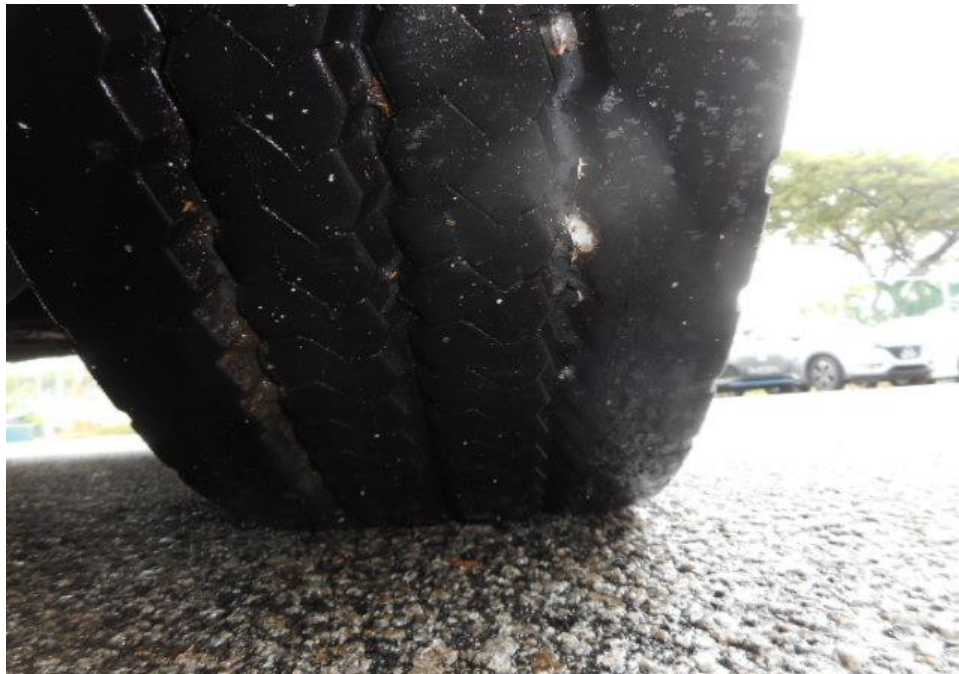
Photo 7 shows the condition of the front right tyre of the Motor Bus, which was observed to be in serviceable condition with remaining tread depth of approximately 14mm. The tyre, which was wrapped around standard steel wheel rim, was also observed to be sufficiently inflated for vehicular operation. There was no tear, cut or burst mark(s) on the outer and the inner sidewalls as well as across the tread of the 8 tyres that were fitted on the Motor Bus.
