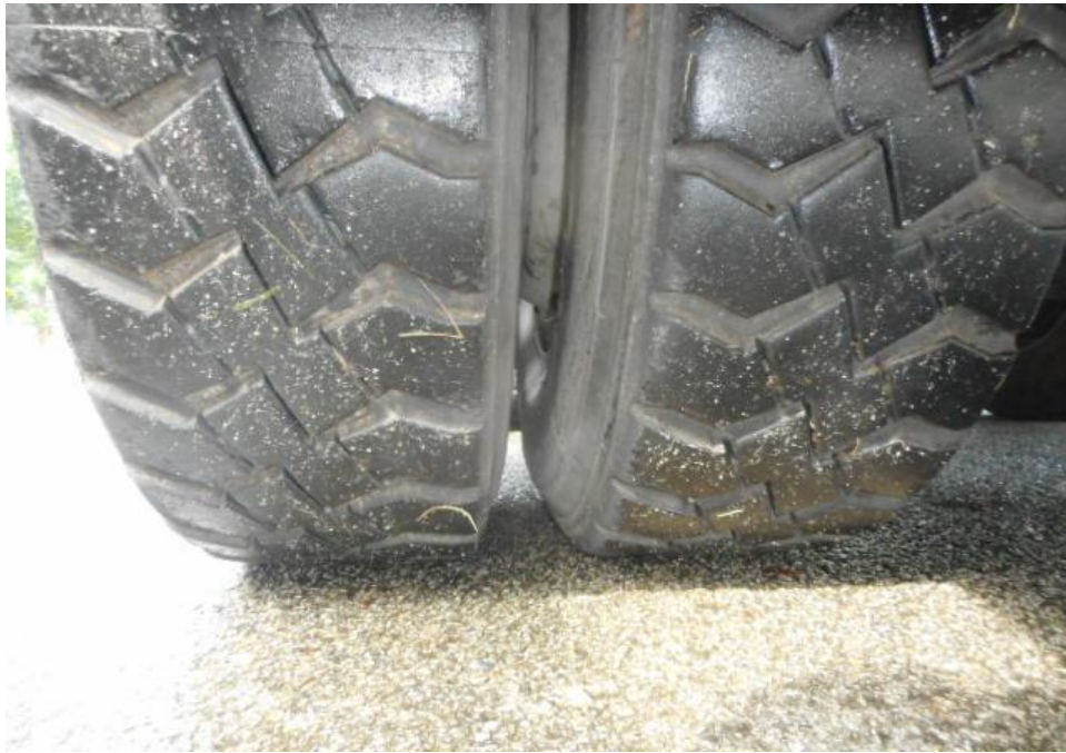
Photo 10 shows the condition of the front left tyres of the Garbage Truck, which were observed to be in serviceable condition with remaining tread depth of approximately 10.5mm. There was also no tear, cut or burst mark(s) on the outer and the inner sidewalls as well as across the tread of the 6 tyres that were fitted on the Garbage Truck.
