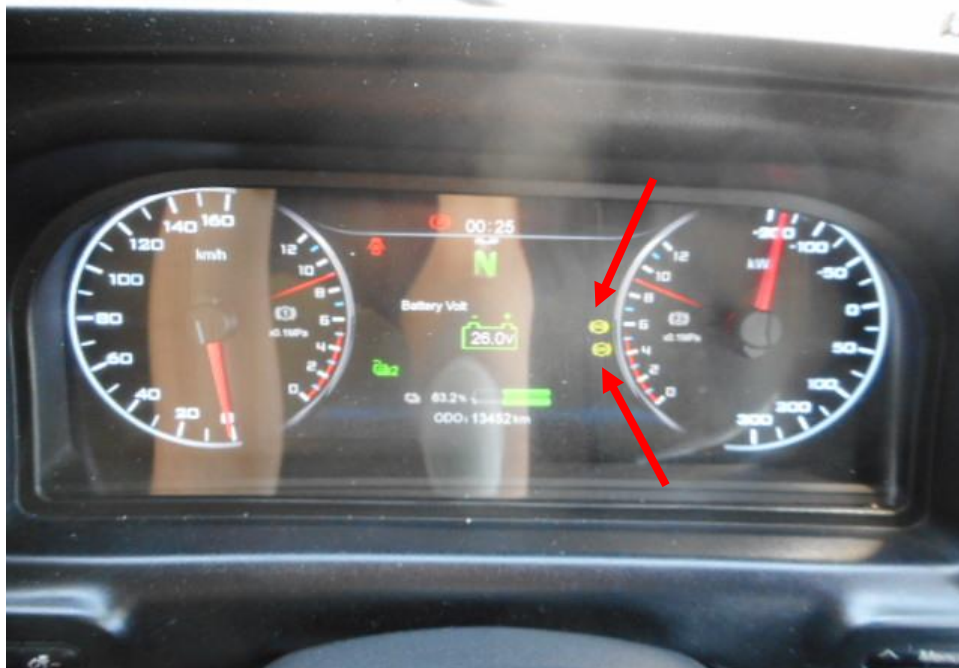
Photo 25 shows the warning light for Anti-Lock Brake System (ABS) and Anti-Slip Regulation (ASR) (arrowed) appearing on the instrument panel of the Garbage Truck during the self-test of its various electronic operating panel systems when its electric motor was cranked.
