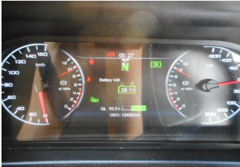
Photo 26 shows no warning lights illuminated on the instrument panel of the Garbage Truck after the electric motor was cranked. This would suggest that there was no abnormality to the electronic operating system of the Garbage Truck, like the ABS, ASR and etc.
