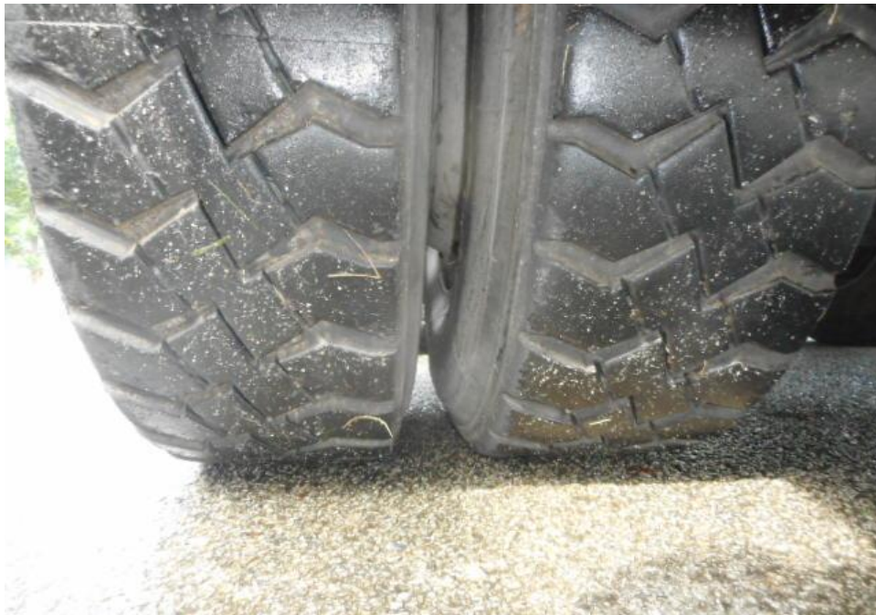
Photo 9 shows the condition of the rear left tyres of the Garbage Truck, which was observed to be in serviceable condition with remaining tread depth of approximately 12.8mm. The tyres, which were wrapped around standard steel wheel rim, were also observed to be sufficiently inflated for vehicular operation. There was also no damage found on all 6 steel wheel rims of the Garbage Truck.
