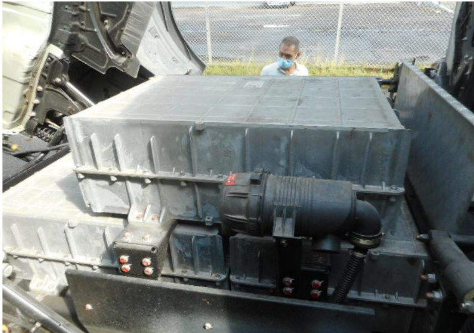
Photo 11 shows a general view of the Garbage Truck's electric motor compartment, which was accessed by lifting the front cabin of the Garbage Truck. The various parts and components inside the electric motor compartment were unaffected by the accident. There was also no sign(s) or indication(s) of fresh fluid leakage and/or fluid stain within the electric motor compartment
