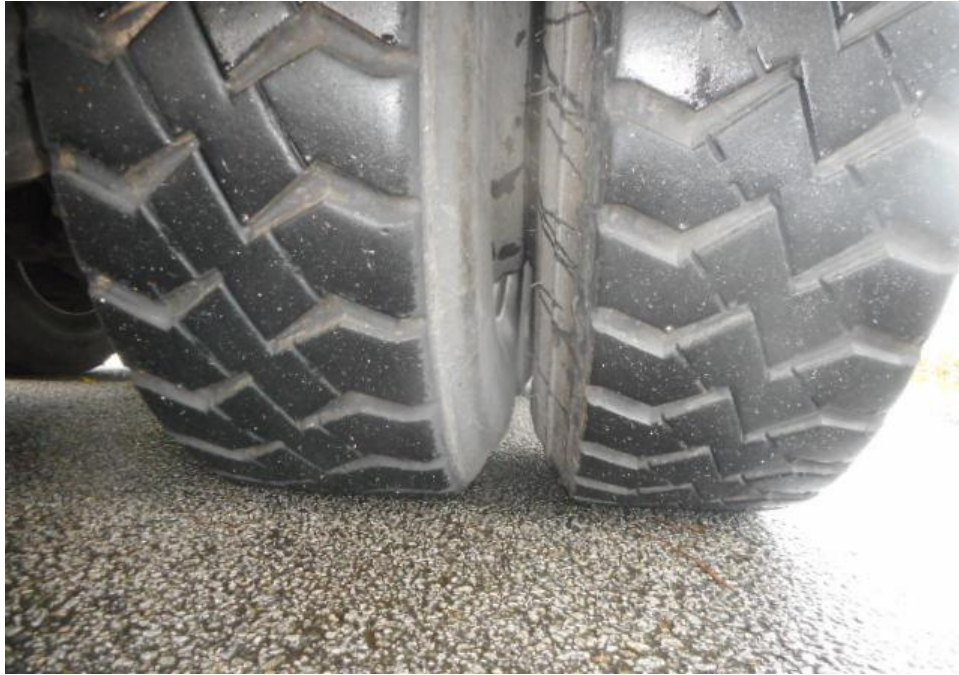
Photo 8 shows the condition of the rear right tyre of the Garbage Truck, which was observed to be in serviceable condition with remaining tread depth of approximately 9.4mm. The tyre, which was wrapped around standard steel wheel rim, was also observed to be sufficiently inflated for vehicular operation.
