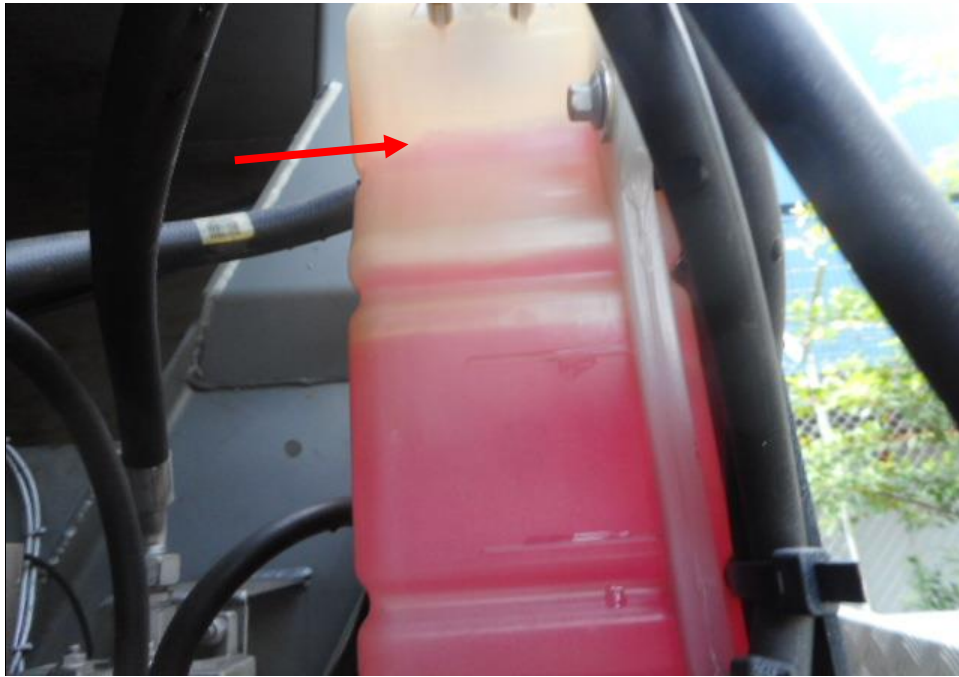
Photo 13 shows the electric motor coolant reservoir of the Garbage Truck at the time of my inspection. The electric motor coolant was observed to be of sufficient level (arrowed) and without any visible contamination.
