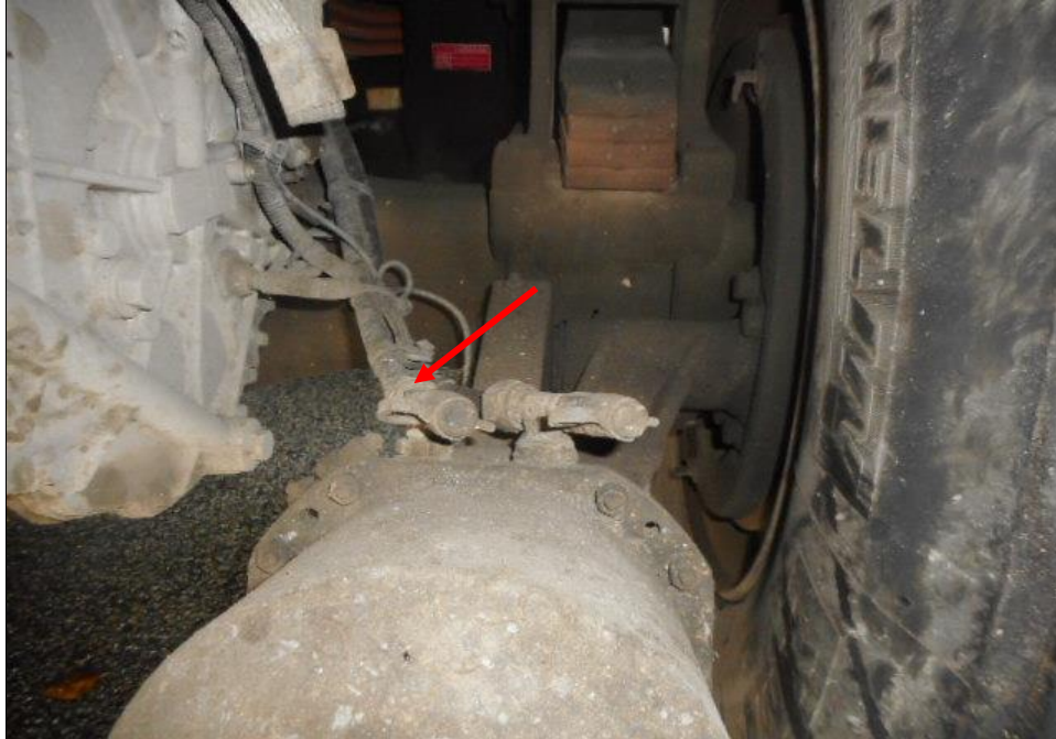
Photo 16 shows the brake pipe (arrowed) at the rear right wheel of the Garbage Truck. I did not observe any leakage of brake fluid at the time of my inspection of the Garbage Truck. My static tests of the Garbage Truck's braking system, along with my visual examination of the various mechanical components in the braking system, had indicated that there was no internal leakage of pressure/vacuum. Hence the braking system of the Garbage Truck was likely to be in serviceable condition at the material time of accident.
