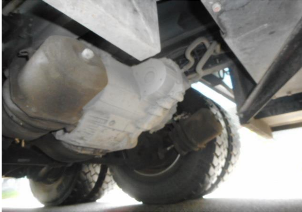
Photo 15 shows the undercarriage of the Garbage Truck, at the area where the electric motor housing located. I did not find any sign(s) or indication(s) of fluid leak, however old fluid stain(s) was observed on the underside of the Garbage Truck.
