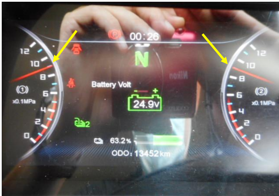
Photo 12 shows the air in the air brake cylinders of the Garbage Truck at the time of my inspection. The air in the cylinder was observed to be of sufficient level (arrowed) & serviceable at the time of the accident.
