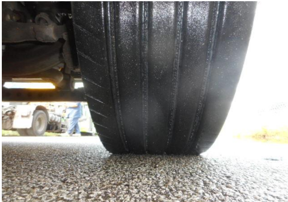
Photo 7 shows the condition of the front right tyre of the Garbage Truck, which was observed to be in serviceable condition with remaining tread depth of approximately 9.8mm. The tyre, which was wrapped around standard steel wheel rim, was also observed to be sufficiently inflated for vehicular operation. There was no tear, cut or burst mark(s) on the outer and the inner sidewalls as well as across the tread of the 6 tyres that were fitted on the Garbage Truck.
