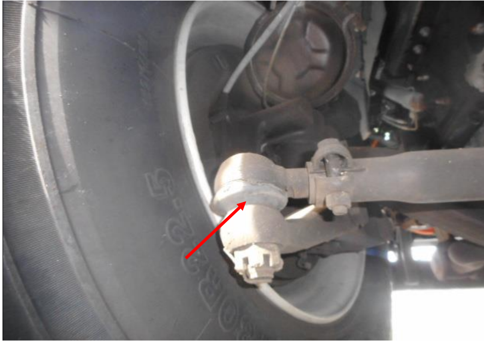
Photo 22 shows the various undercarriage components at the front left wheel of the Garbage Truck, in particular the steering tie rod end (arrowed). The various undercarriage components of the Garbage Truck were all found to be intact without any visible damage. There was also no sign of fluid stain(s) observed on the various undercarriage components.
