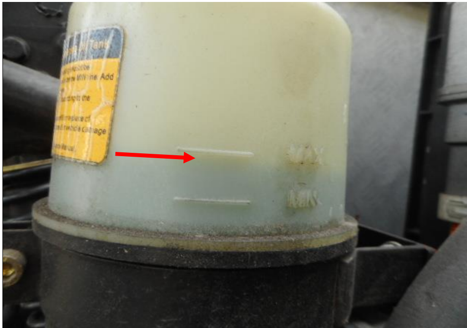
Photo 14 shows the power steering fluid reservoir of the Garbage Truck at the time of my inspection. The power steering fluid was observed to be of sufficient level (arrowed) and without any visible contamination.
