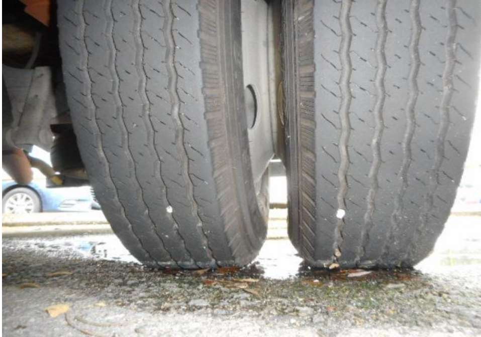
Photo 11 shows the condition of the rear left tyres of the Motor Lorry, which were observed to be in serviceable condition with remaining, tread depth of approximately 5.5mm.
