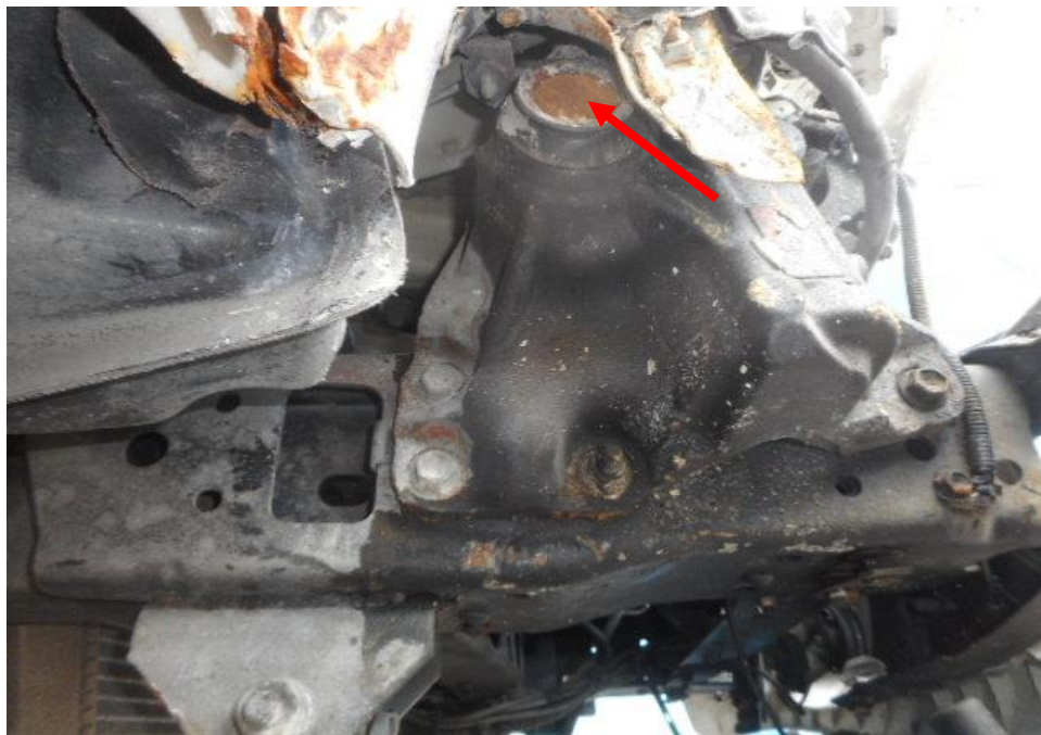
Photo 18 shows the steering box (arrowed) of the Motor Lorry's steering system. The steering box was observed to sustained damages a result of the accident.
