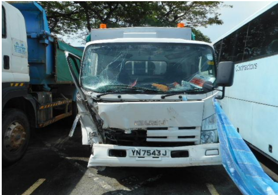
Photo 2 shows a general view of the front portion of the Motor Lorry at the time of our inspection. The Motor Lorry was observed sustained major damages to its front windscreen, front body panel and front bumper portion as well as its right door as a result of the accident.
