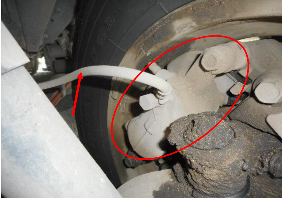
Photo 25 shows the brake hose/pipe (arrowed) at the front left wheel of the Motor Lorry. No leakage of brake fluid was observed. Visual examination of the various components of the braking system like the brake caliper (circled), brake booster, brake pedal etc had revealed all to be intact and without visible damage at the time of accident. There was also no sign of fluid stain(s) observed on the various undercarriage components.
