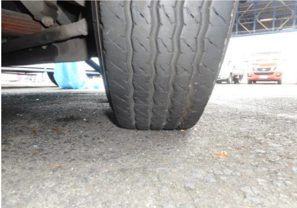
Photo 9 shows the condition of the front right tyre of the Motor Lorry, which were observed to be in serviceable condition with remaining, tread depth of approximately 7.8mm. The tyre, which was wrapped around standard steel wheel rim, it was observed to be sufficiently inflated for vehicular operation.
