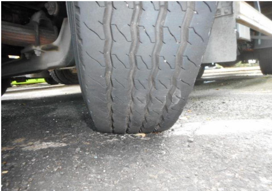
Photo 12 shows the condition of the front left tyre of the Motor Lorry, which were observed to be in serviceable condition with remaining, tread depth of approximately 9.3mm. There was also no tear, cut or burst mark(s) on the outer and the inner sidewalls as well as across the tread of the 6 tyres that were fitted on the Motor Lorry.
