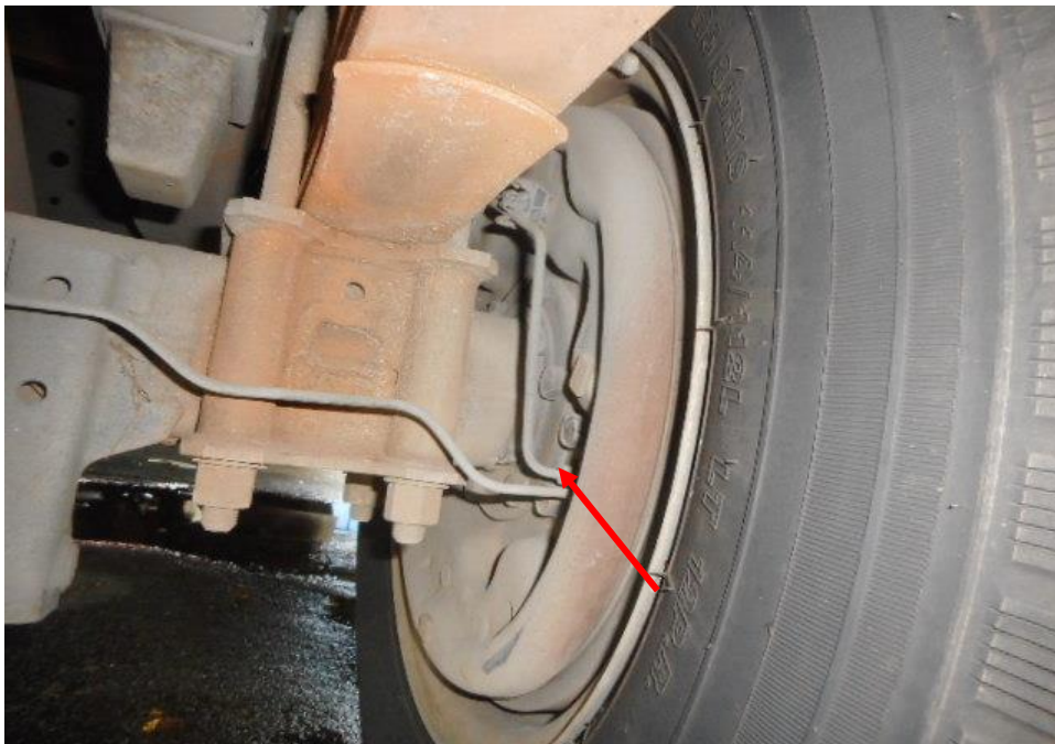
Photo 22 shows the brake pipe (arrowed) at the rear right wheel of the Motor Lorry. I did not observe any leakage of brake fluid at the time of my inspection of the Motor Lorry. My static tests of the Motor Lorry's braking system, along with my visual examination of the various mechanical components in the braking system, had indicated that there was no internal leakage of pressure/vacuum.
