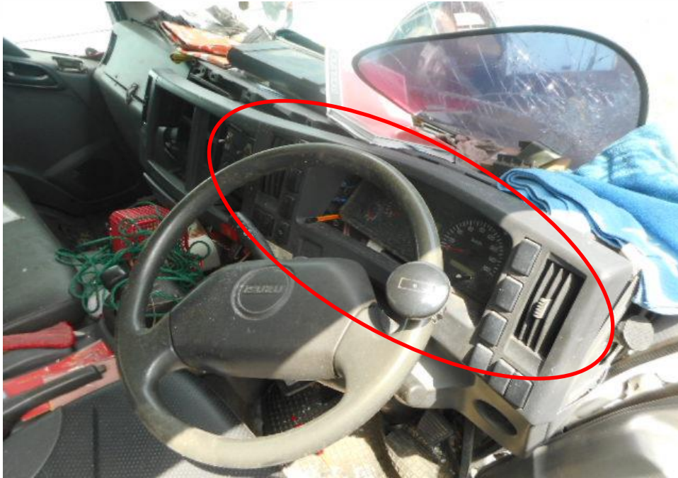
Photo 1 shows the close up view of the front portion of the Motor Lorry at the time of our inspection. The Motor Lorry was observed to have sustained major damages to its dashboard (circled) that was crushed due to the accident's impact.
