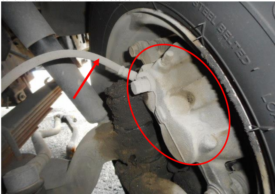
Photo 24 shows the brake hose/pipe (arrowed) at the front right wheel of the Motor Lorry. No leakage of brake fluid was observed. Visual examination of the various components of the braking system like the brake caliper (circled), brake booster, brake pedal etc had revealed all to be intact and without visible damage at the time of accident. There was also no sign of fluid stain(s) observed on the various undercarriage components.
