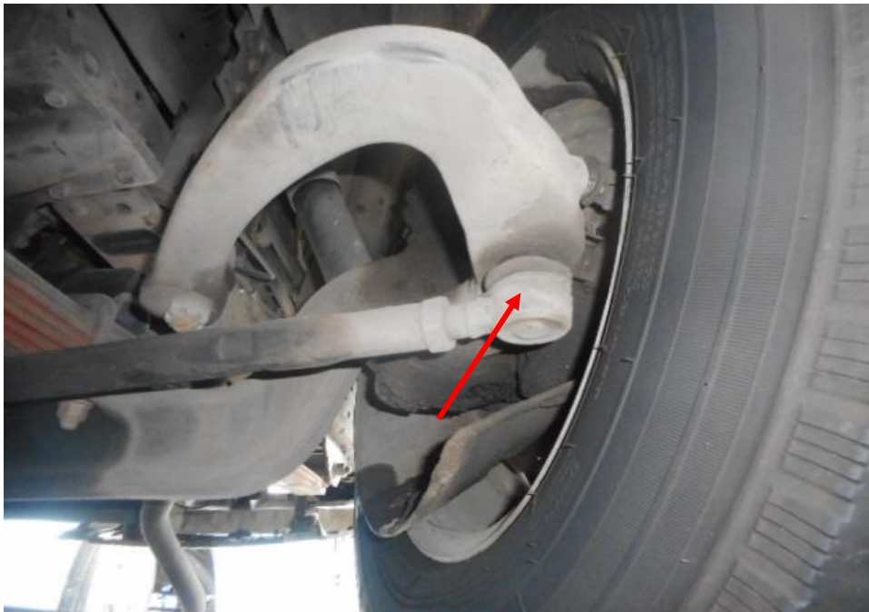
Photo 20 shows the various undercarriage components at the front right wheel of the Motor Lorry, in particular the steering tie rod end (arrowed). The various steering components were all found to be intact, suggesting that the steering system of the Motor Lorry was likely to be in serviceable condition at the material time of accident. There was also no sign of fluid stain(s) observed on the various undercarriage components.
