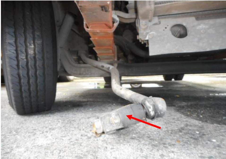
Photo 19 shows the steering box arm (arrowed) of the Motor Lorry's steering system. The steering box arm was observed to sustained damages a result of the accident.
