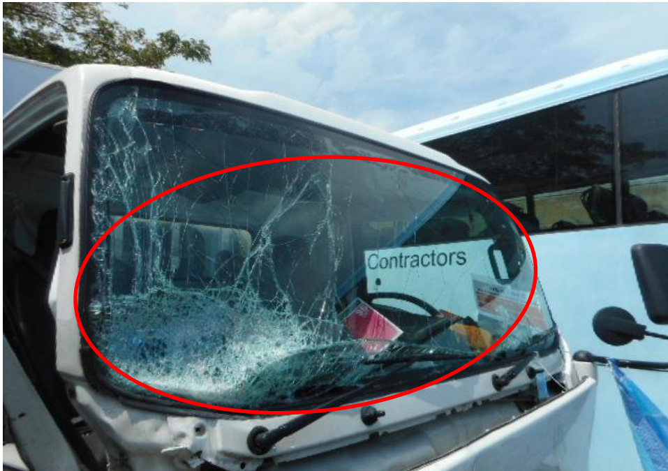
Photo 3 shows the close up view of the front portion of the Motor Lorry at the time of our inspection. The Motor Lorry was observed to have sustained major damages to its front windscreen (circled) as a result of the accident.
