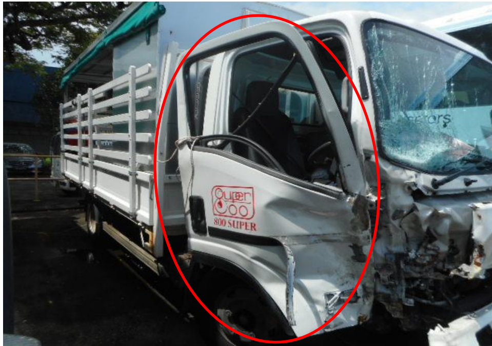
Photo 5 shows the close up view of the right door of the Motor Lorry at the time of our inspection. The Motor Lorry was observed to have sustained damages to its left door (circled) as a result of the accident.
