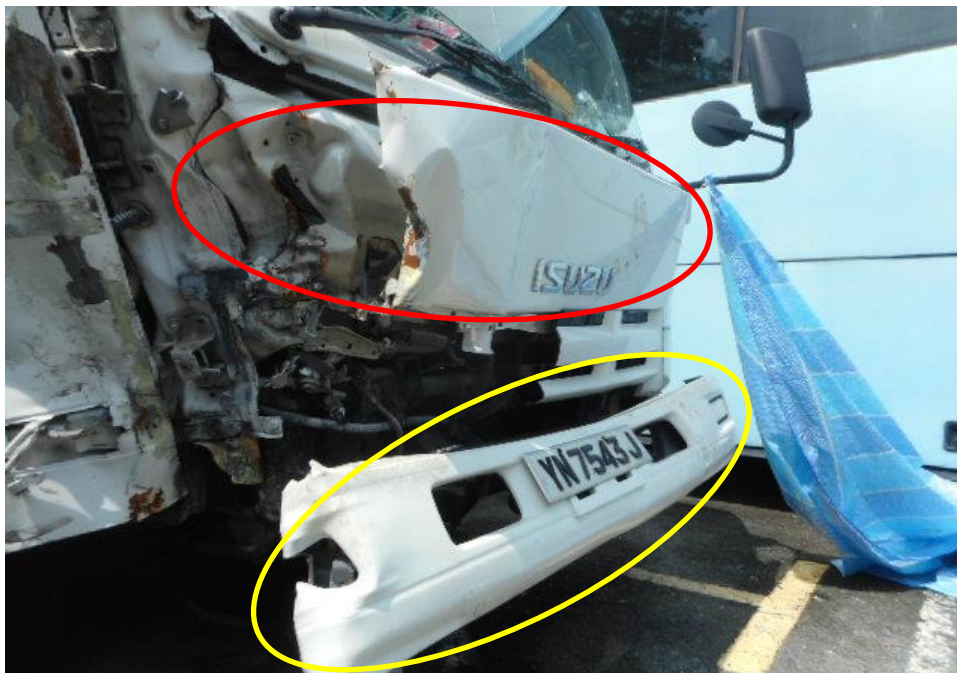
Photo 4 shows the close up view of the front portion of the Motor Lorry at the time of our inspection. The Motor Lorry was observed to have sustained major damages to its front body panel (red circle) and front bumper (yellow circle) that was damaged as a result of the accident's impact.
