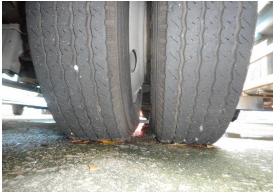
Photo 10 shows the condition of the rear right tyres of the Motor Lorry, which were observed to be in serviceable condition with remaining, tread depth of approximately 4.1mm. The tyre, which was wrapped around standard steel wheel rim, it was observed to be sufficiently inflated for vehicular operation.
