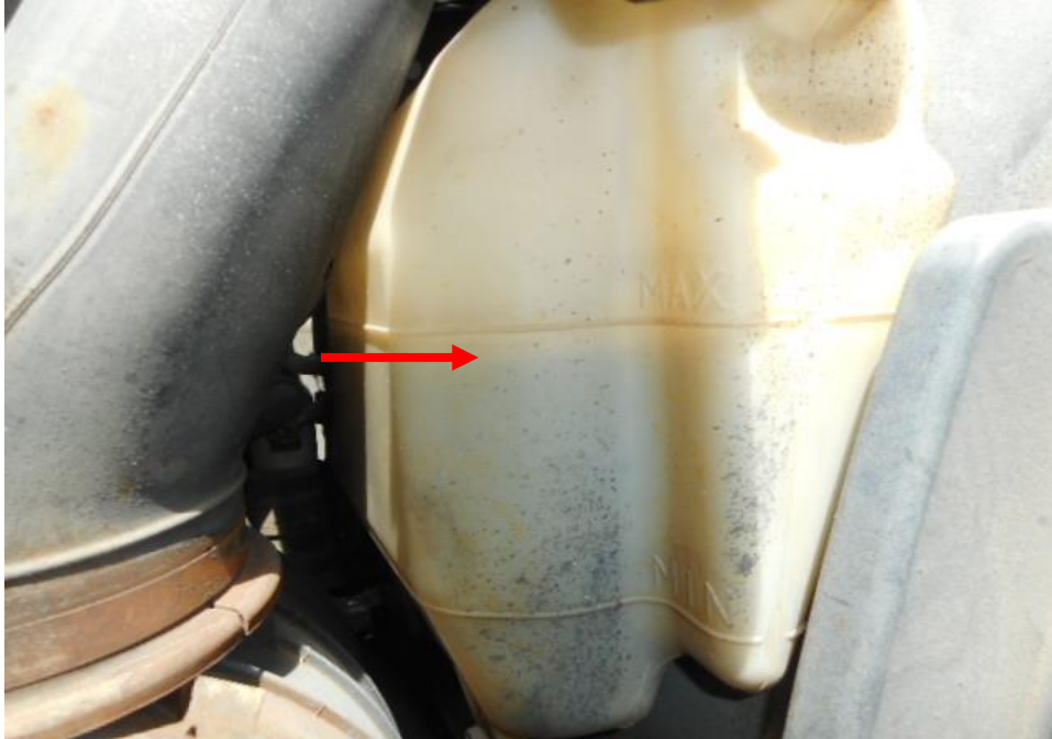
Photo 14 shows checks being carried out to the engine coolant of the Motor Lorry at the time of my inspection. The engine coolant was observed to be of sufficient level and without any visible contamination.
