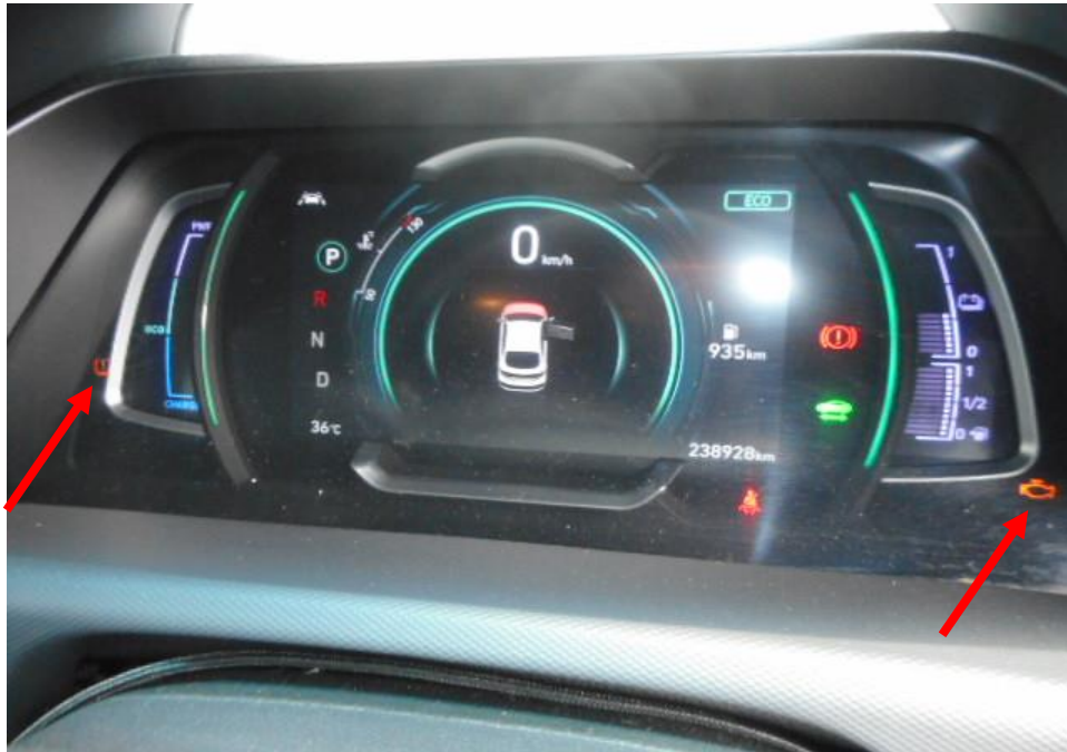
Photo 27 shows no warning lights illuminated on the instrument panel of the Motor Taxi after the engine was cranked. This would suggest that there was no abnormality to the electronic operating system of the Motor Taxi, like the ABS, EPS, SRS, and TC etc. However, only the engine and Tyre Pressure Monitoring System (TPMS) (arrowed) light remained illuminated as a result of the insufficient coolant in the engine as a result of the damaged coolant hose and the deflated front left and right tyres caused by the accident.
