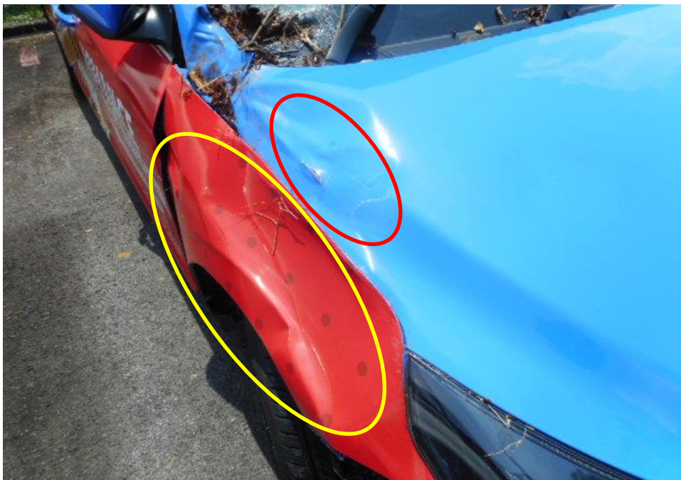
Photo 5 shows the close up view of the Motor Taxi's front body at the time of my inspection. The Motor Taxi was observed to have sustained damage at its front bumper (red circle) and front right fender (yellow circle) as a result of the accident.
