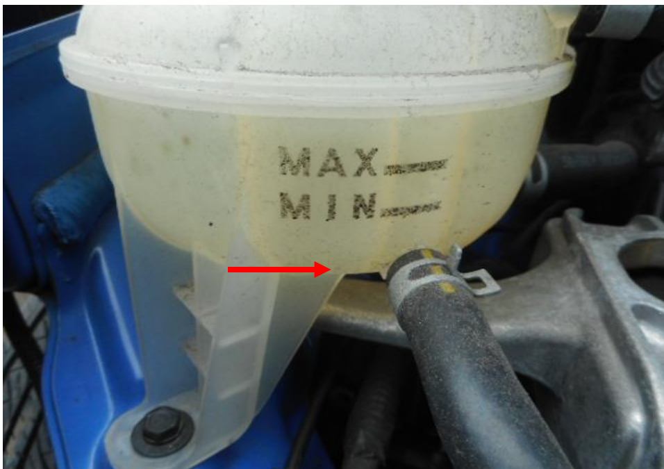
Photo 16 shows checks being carried out to the engine coolant of the Motor Taxi at the time of my inspection. The engine coolant was observed to be of insufficient level (arrowed) as the damage to the engine coolant hose has caused a leakage.
