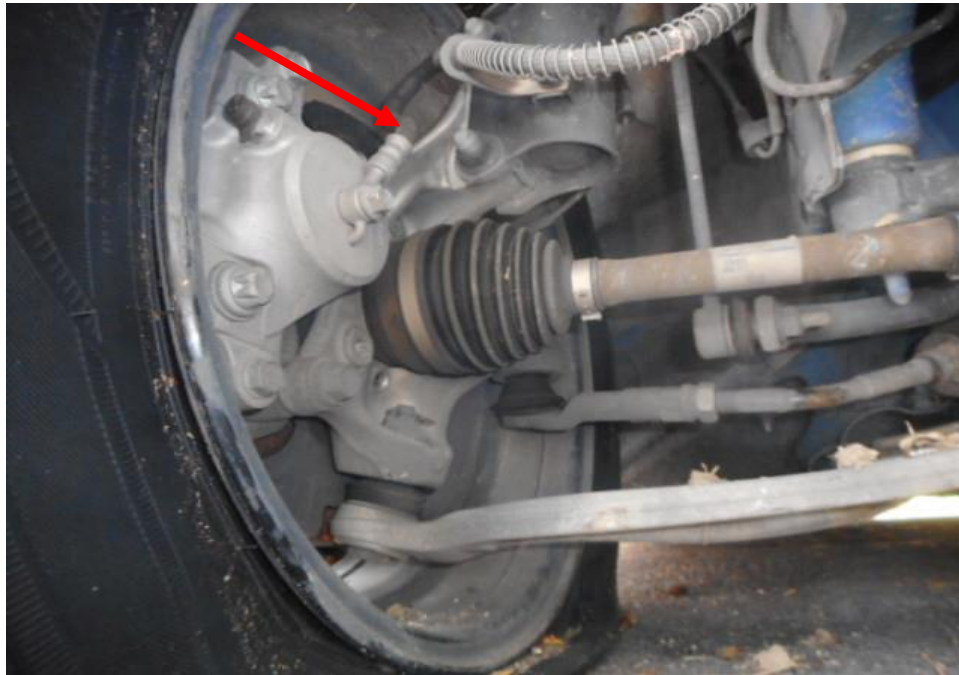
Photo 22 shows the brake hose/pipe (arrowed) at the front right wheel of the Motor Taxi. I did not observe any leakage of brake fluid at the time of my inspection of the Motor Taxi. Static tests of the Motor Taxi's braking system had indicated that there was no internal leakage of pressure/vacuum. The undercarriage components of the Motor Taxi were also all found to be intact and without any visible damage.
