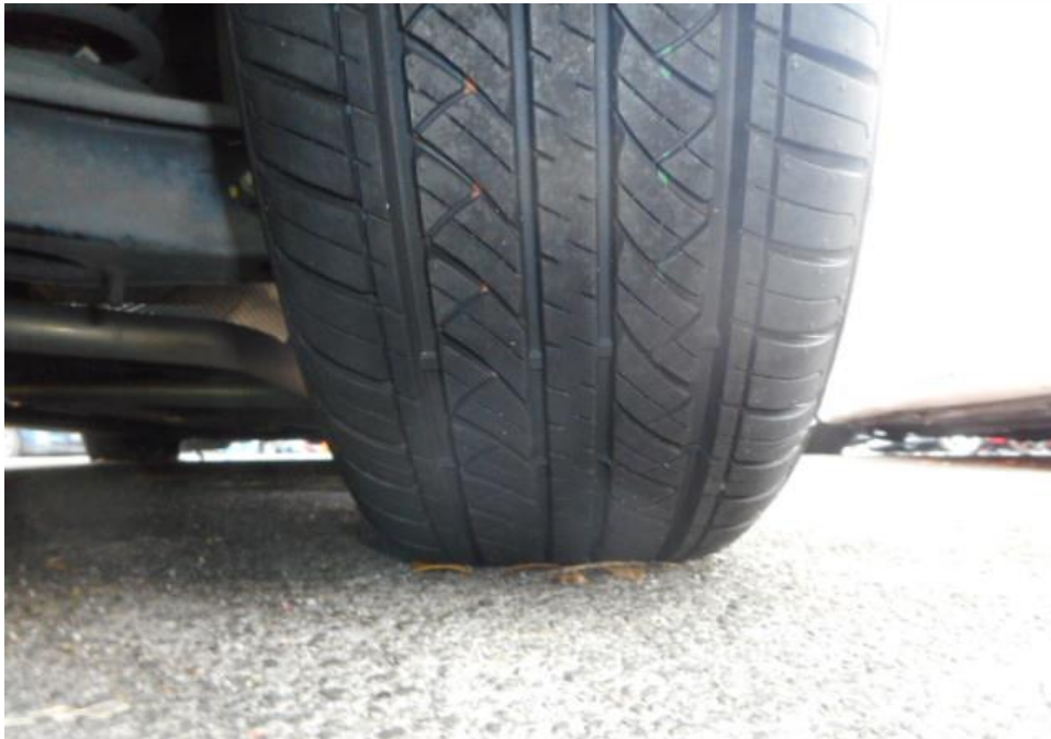
Photo 10 shows the condition of the rear right tyre of the Motor Taxi, which was observed to be in serviceable condition with remaining tread depth of approximately 8mm. The tyre was also observed to be sufficiently inflated for vehicular operation with no tear, cut or burst mark(s).
