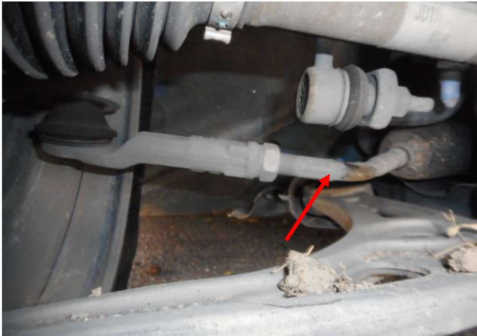
Photo 24 shows the various undercarriage components at the front right wheel of the Motor Taxi, in particular the steering tie rod (arrowed) was observed to be damaged as a result of the accident.
