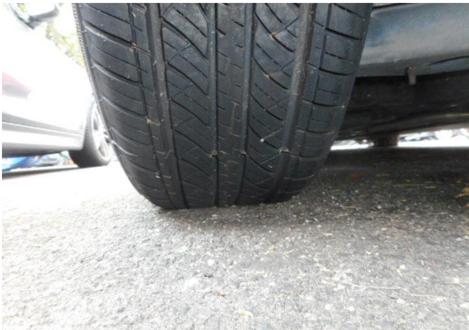
Photo 11 shows the condition of the rear left tyre of the Motor Taxi, which was observed to be in serviceable condition with remaining tread depth of approximately 7.8mm. The tyre, which was wrapped around steel wheel rim, was also observed to be sufficiently inflated for vehicular operation. The 4 tyres of the Motor Taxi were wrapped around standard steel wheel rims.
