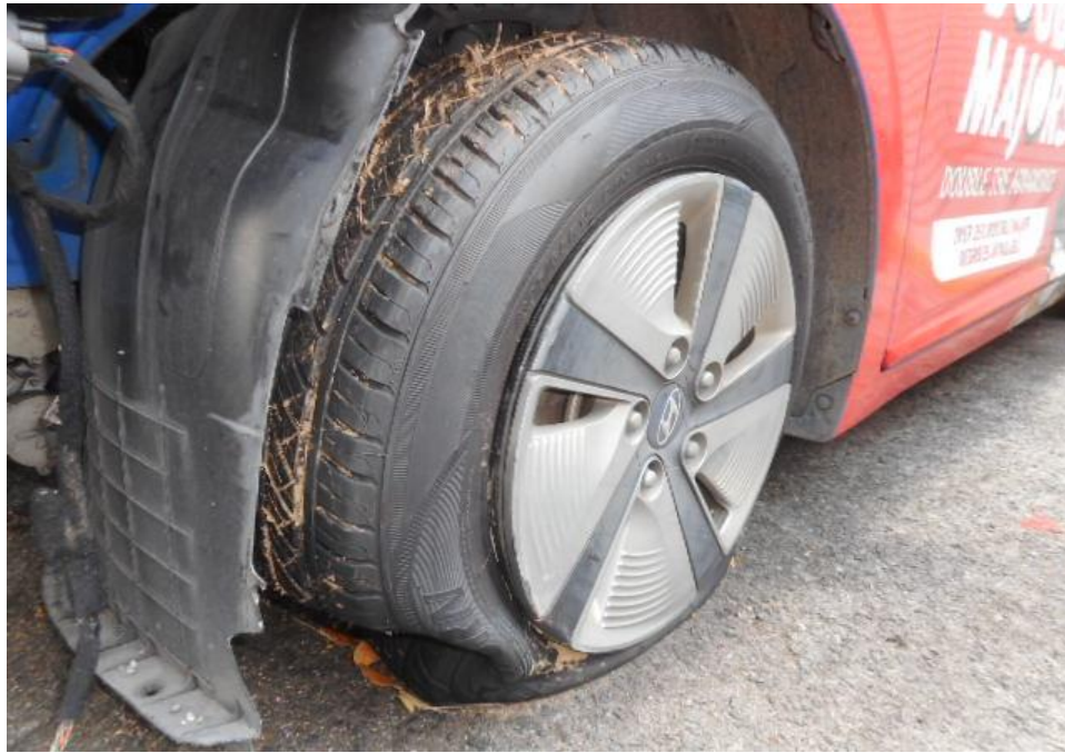
Photo 12 shows the condition of the front left tyre of the Motor Taxi, which was observed to be in unserviceable condition with remaining tread depth of approximately 5.7mm. The tyre was deflated and slip off the wheel rim as a result of the accident. There was no tear, cut or burst mark(s) on the outer and the inner sidewalls as well as across the tread.
