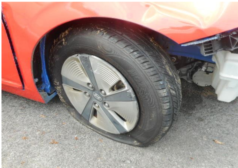
Photo 9 shows the condition of the front right tyre of the Motor Taxi, which was observed to be in unserviceable condition with remaining tread depth of approximately 5.5mm. The tyre was deflated and slip off the wheel rim as a result of the accident. There was no tear, cut or burst mark(s) on the outer and the inner sidewalls as well as across the tread.
