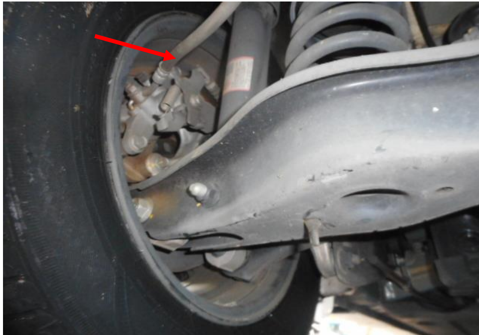
Photo 21 shows the brake hose/pipe (arrowed) at the rear left wheel of the Motor Taxi. I did not observe any leakage of brake fluid at the time of my inspection of the Motor Taxi. Static tests of the Motor Taxi's braking system had indicated that there was no internal leakage of pressure/vacuum. The undercarriage components of the Motor Taxi were also all found to be intact and without any visible damage.
