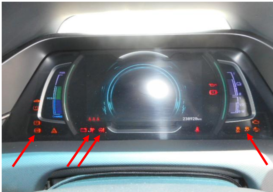
Photo 26 shows the warning light for Anti-Lock Brake System (ABS) and Power Steering System (EPS), Supplemental Restraint System (SRS) and Traction Control (TC) (arrowed) appearing on the instrument panel of the Motor Taxi during the self-test of its various electronic operating systems when its engine was cranked.
