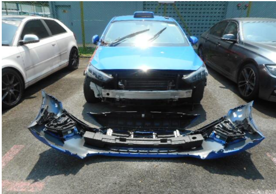
Photo 3 shows a general view of the Motor Taxi's front body at the time of my inspection. The front portion of the Motor Taxi was observed to have sustained damage. Its front windscreen, front bonnet, front bumper and front right fender was the body parts and various engine components were also damaged as a result of the accident.
