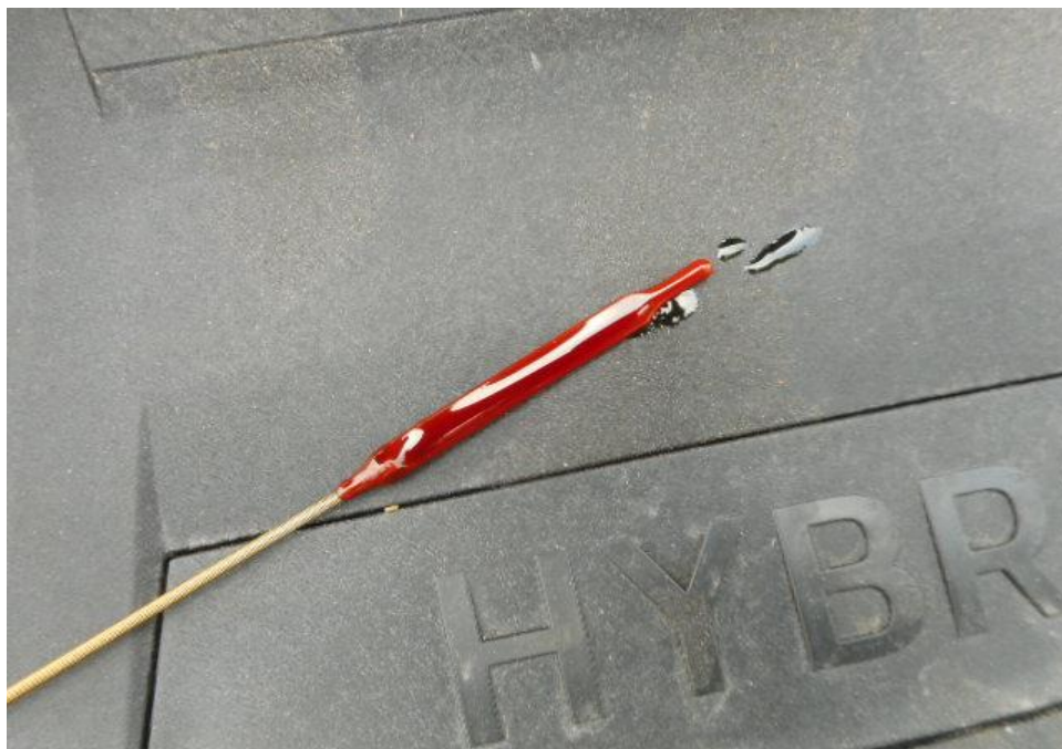
Photo 18 shows the engine oil dip stick of the Motor Taxi at the time of my inspection. The engine oil was observed to be of sufficient level and without any visible contamination.
