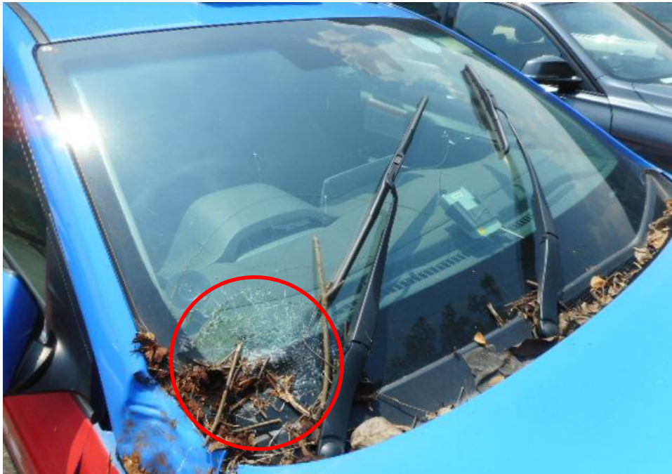
Photo 4 shows the close up view of the Motor Taxi's front body at the time of my inspection. The Motor Taxi was observed to have sustained damage at its front windscreen (circled) as a result of the accident.
