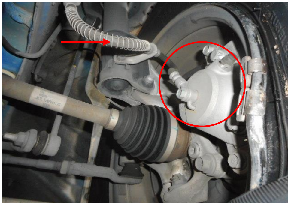
Photo 23 shows the brake hose/pipe (arrowed) at the front left wheel of the Motor Taxi. No leakage of brake fluid was observed. Visual examination of the various components of the braking system like the brake caliper (circled), brake booster, brake pedal etc had revealed all to be intact and without visible damage.
