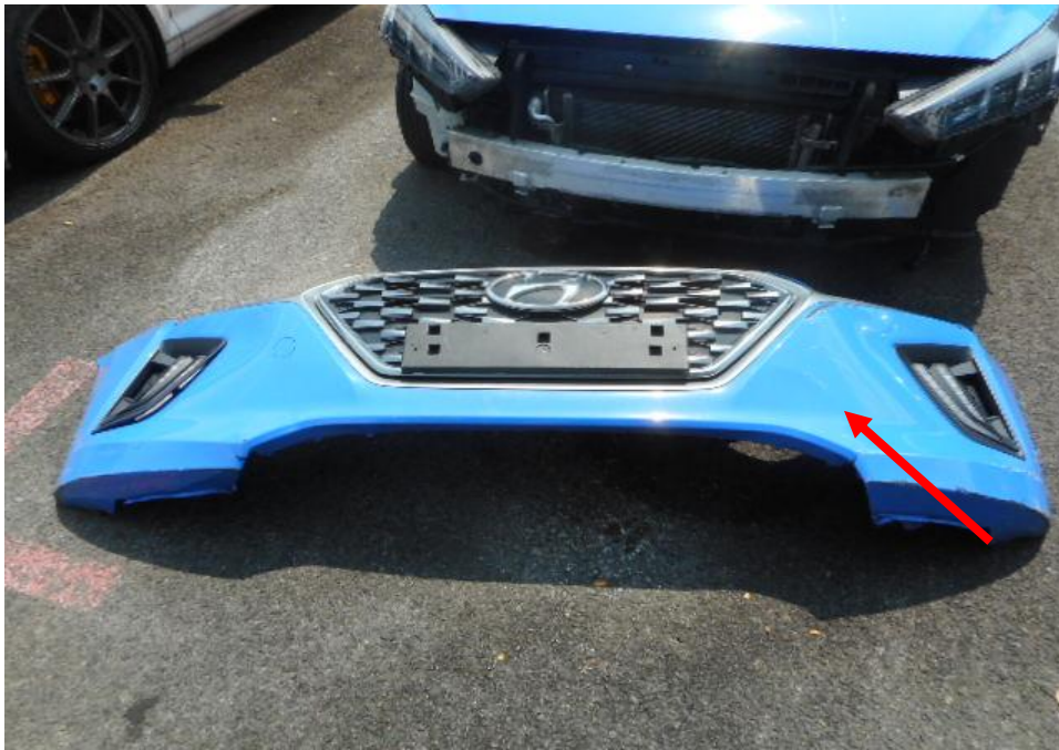
Photo 6 shows the close up view of the Motor Taxi's front body at the time of my inspection. The Motor Taxi was observed to have sustained damage at its front bumper (circled) and front left fender (arrowed) as a result of the accident.
