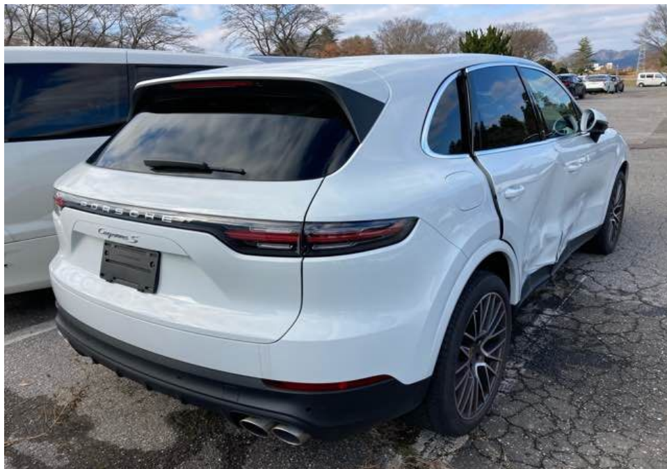
Photo 2 shows the rear right body of the Motor Car (photograph provided to me). The photographs provided to me had showed damage to the right side centre portion of the Motor Car. The front right door, rear right door and right side rocker panel garnish were amongst the body parts that were observed to have been damaged.
