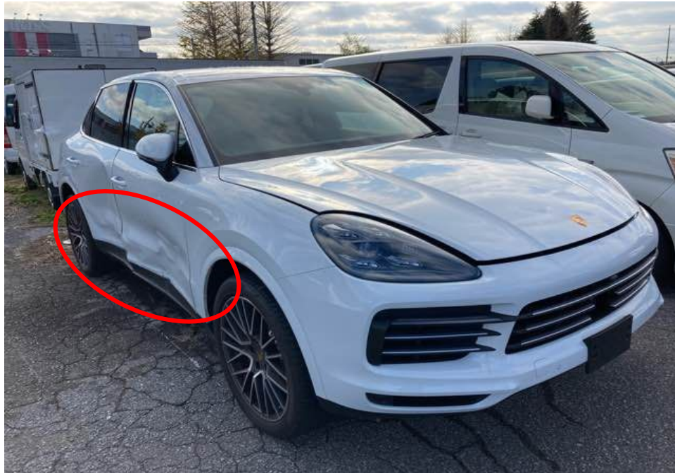
Photo 1 shows the front right body of the Motor Car (photograph provided to me). The photographs provided to me had showed damage to the right side centre portion (circled) of the Motor Car. The front right door, rear right door and right side rocker panel garnish were amongst the body parts that were observed to have been damaged.
