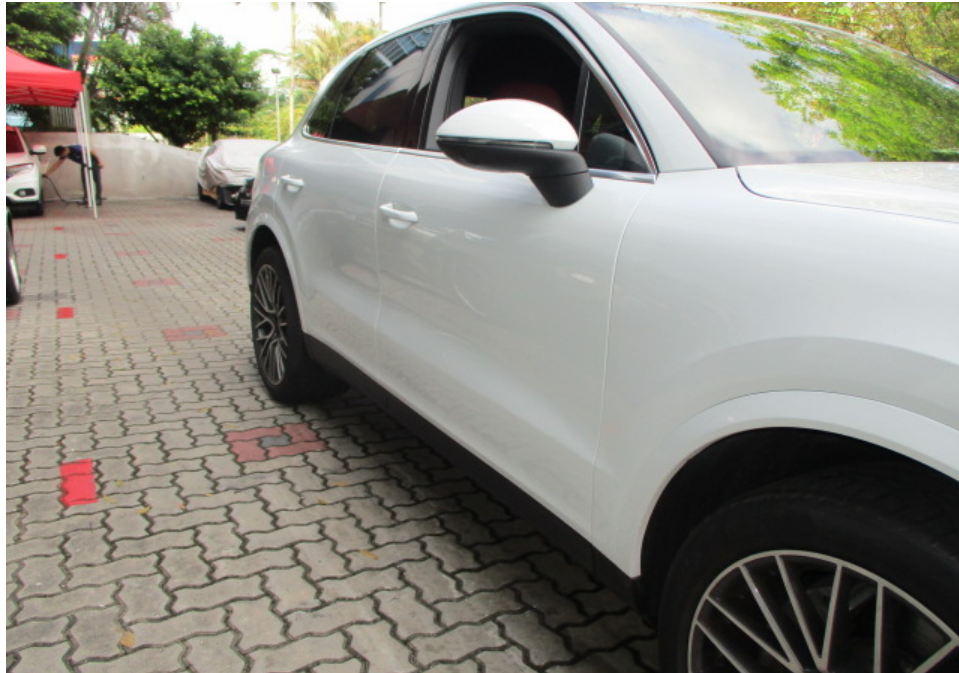
Photo 6 shows a closer view of the Motor Car's front right fender, front right door, right side wing mirror and right side rocker panel garnish. The body parts at the right side centre portion of the Motor Car were visually examined and it was observed that the repair/restoration works carried out to the damaged area of the Motor Car (refer to photograph 1 & 2 above) were reasonably adequate and in order.
