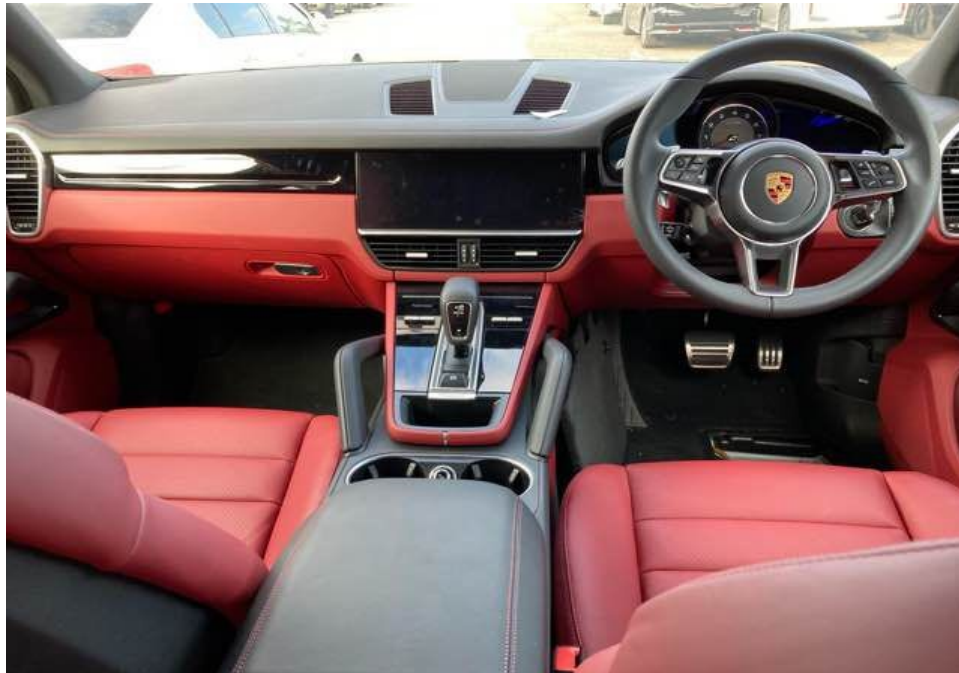
Photo 4 shows the interior compartment of the Motor Car (photograph provided to me). The various parts and components within the interior compartment were all intact and unaffected. The airbag(s) was not deployed as seen from the photographs that were provided to me.
