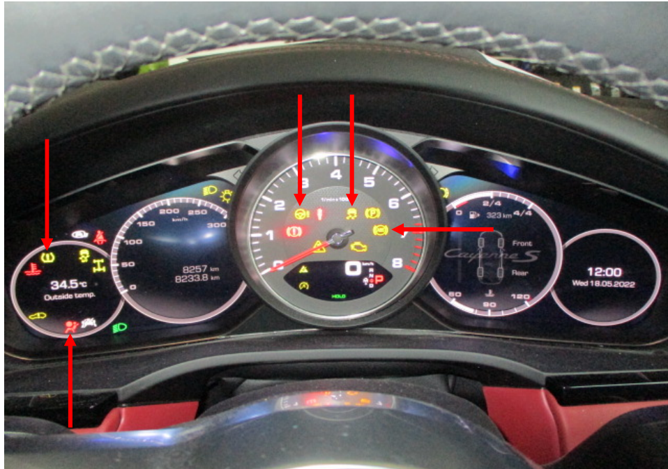
Photo 16 shows the warning lights for the various electronic safety features appearing on the instrument panel of the Motor Car during its self-test when the engine is cranked, in particular the ABS, SRS, EPS, TPM and TCS lights (arrowed).
