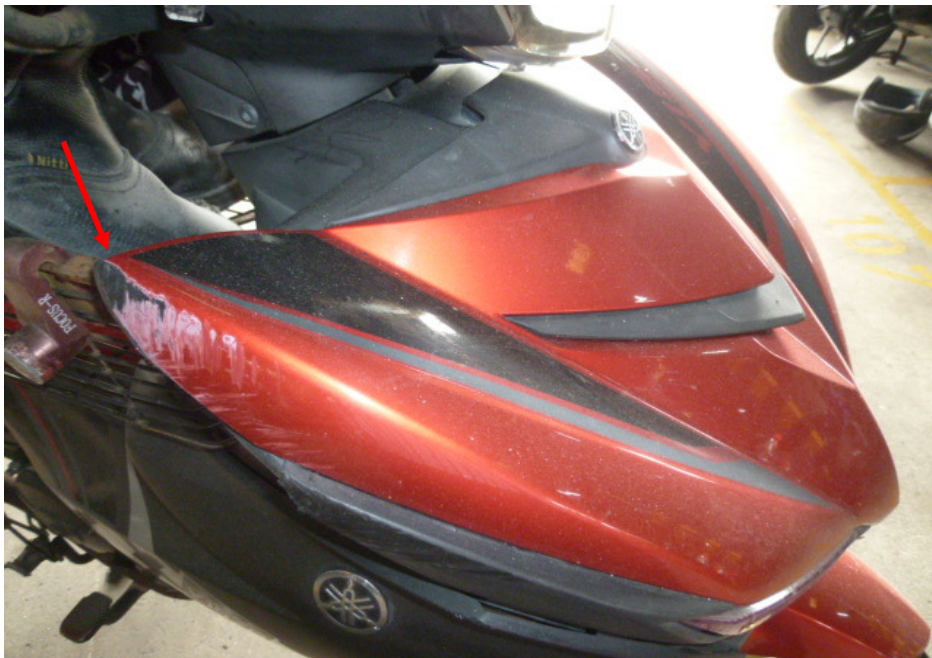
Photo 7 shows a closer view of the grazed front cowling (arrowed) of the Motorcycle as a result of the accident.
