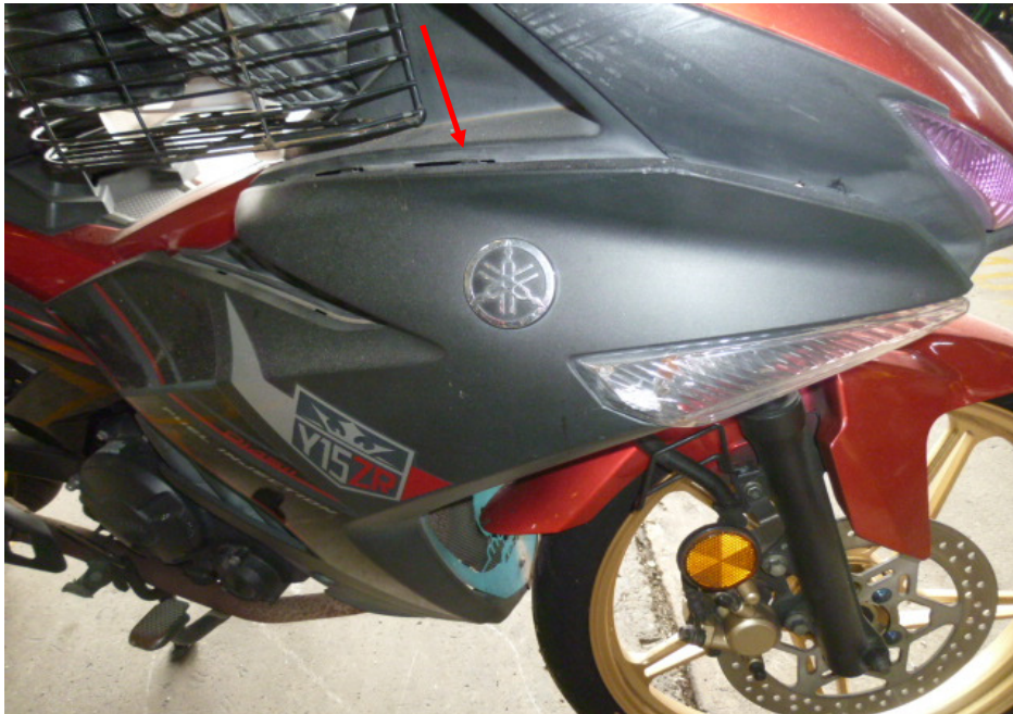
Photo 10 shows a closer view of the deformed right cowling of the Motorcycle as a result of the accident (arrowed).
