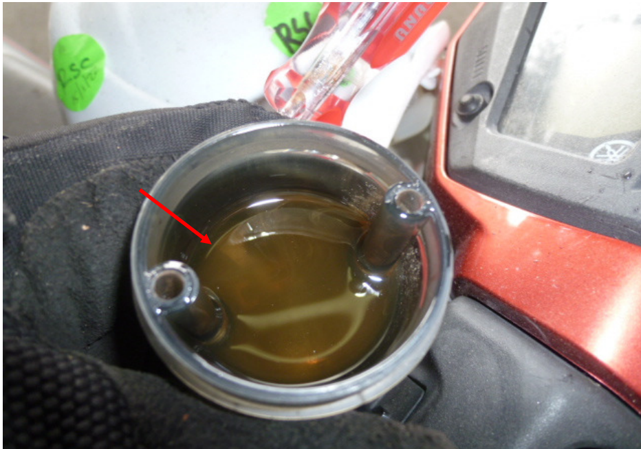
Photo 23 shows a close up view of the brake fluid reservoir for the front brake of the Motorcycle. The front brake fluid was observed to be of sufficient level for operational purposes. However it was found to be slightly contaminated (arrowed).
