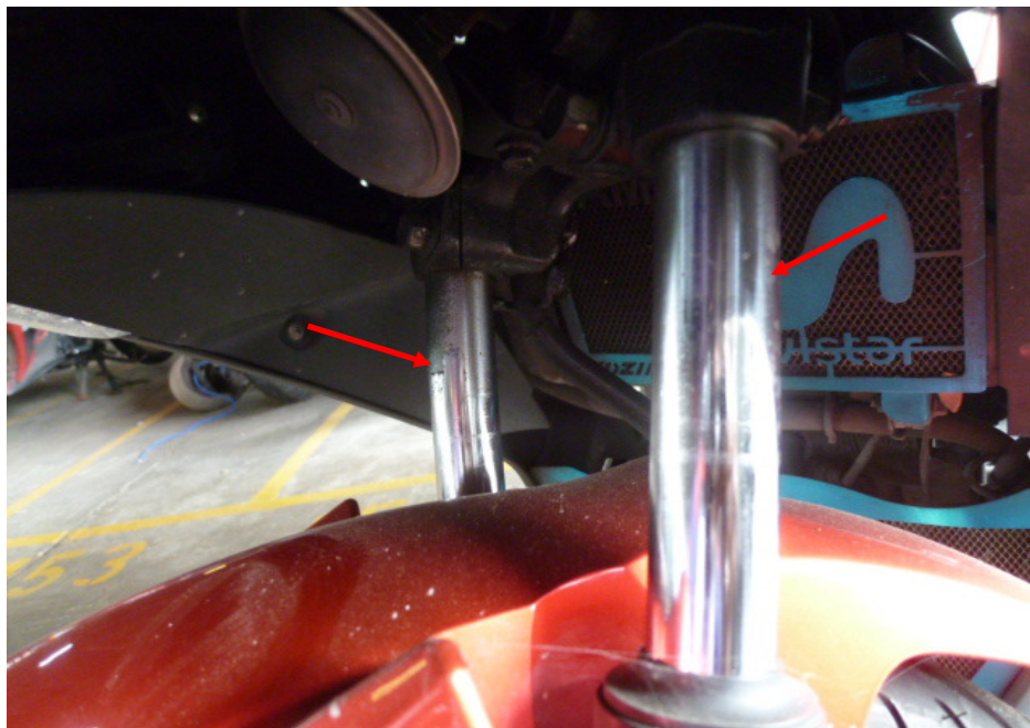
Photo 21 shows the front forks of the Motorcycle. The front forks were observed to be bent (arrowed) as a result of the accident. We were hence not able to conduct any tests on the steering system of the Motorcycle.
