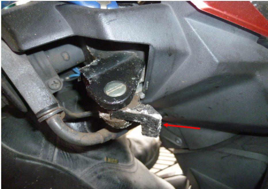
Photo 24 shows the front brake reservoir. We were unable to depress the front brake lever as part of it had broken off as a result of the accident (arrowed). Hence we were unable to determine if there was any leakage of pressure/vacuum in the front brake system.
