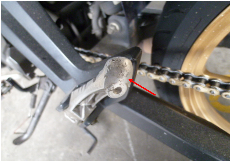
Photo 9 shows a closer view of the grazed left pillion footpeg of the Motorcycle as a result of the accident (arrowed).
