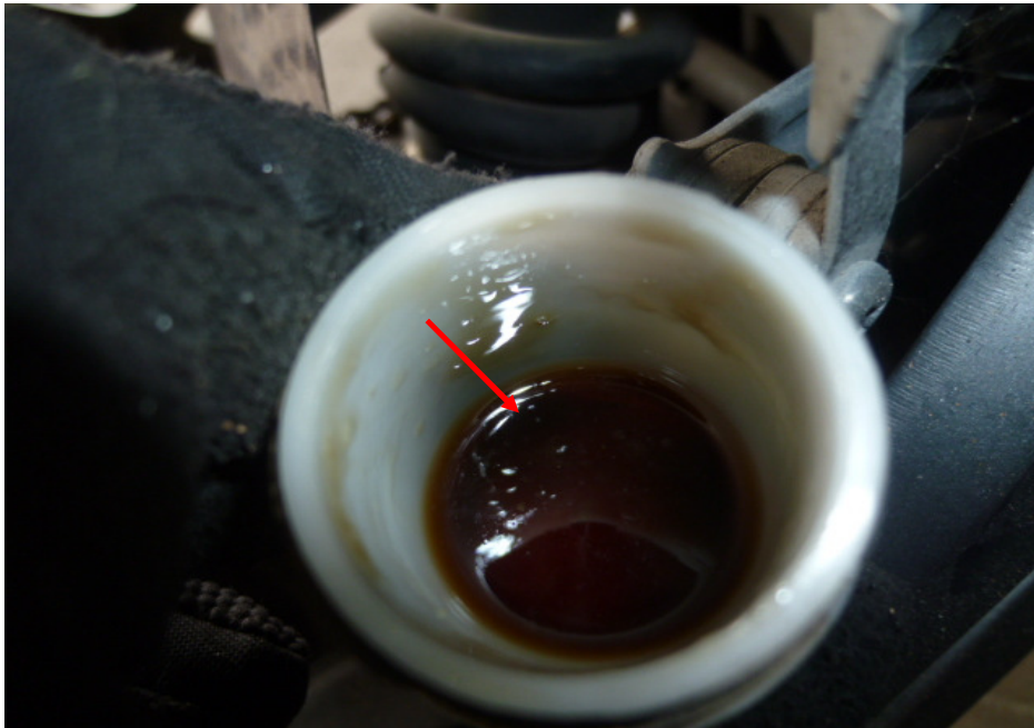
Photo 26 shows a close up view of the brake fluid reservoir for the rear brake of the Motorcycle. The rear brake fluid was observed to be of sufficient level for operational purposes. However it was found to be slightly contaminated (arrowed).
