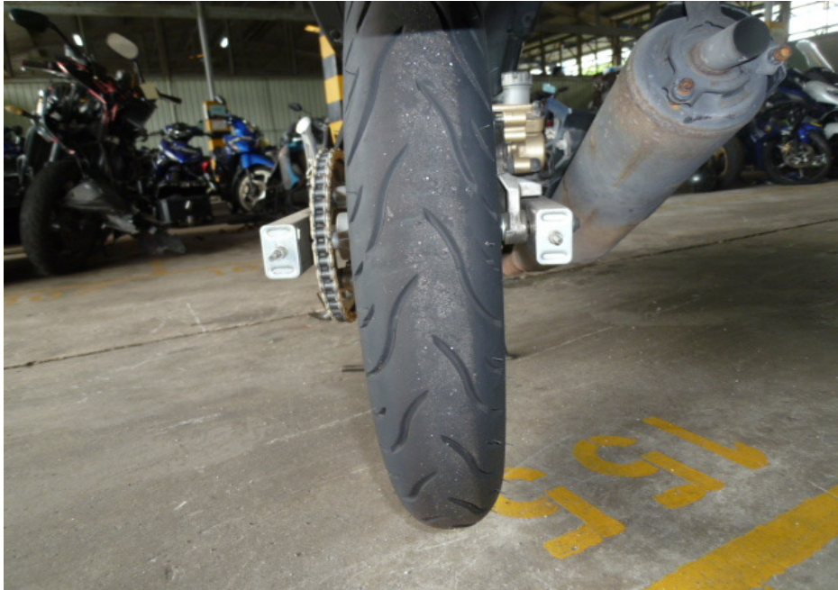
Photo 16 shows the condition of the Motorcycle's rear tyre. The rear tyre was observed to be in serviceable condition with remaining tread depth of approximately 5mm. The tyre was also observed to be sufficiently inflated for vehicular operation. We did not observe any tear, burst mark(s) and/or punctured hole(s) on the sidewalls as well as across the tread of the rear tyre.
