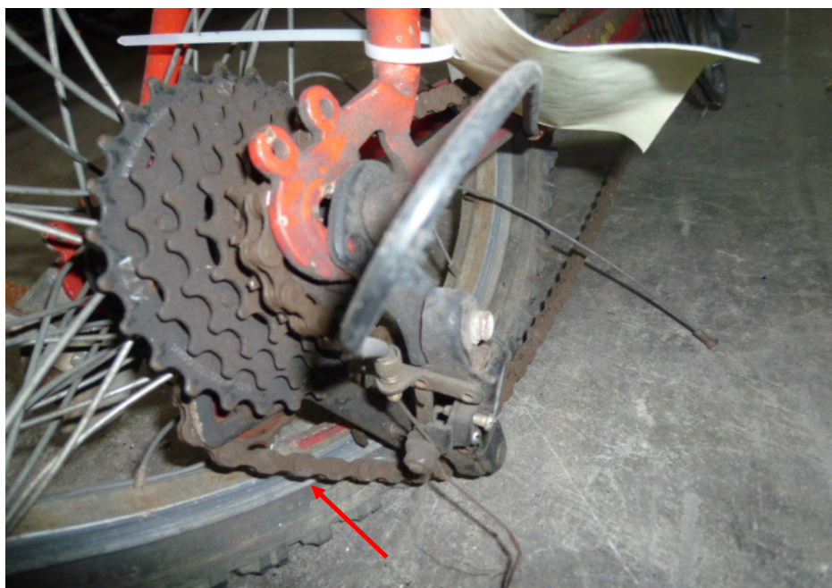
Photo 15 shows a close up view of the gear train of the Bicycle, which was observed to have sustained severe damages as a result of the accident (arrowed). No free play tension test can be conducted due to the extensive damages.
