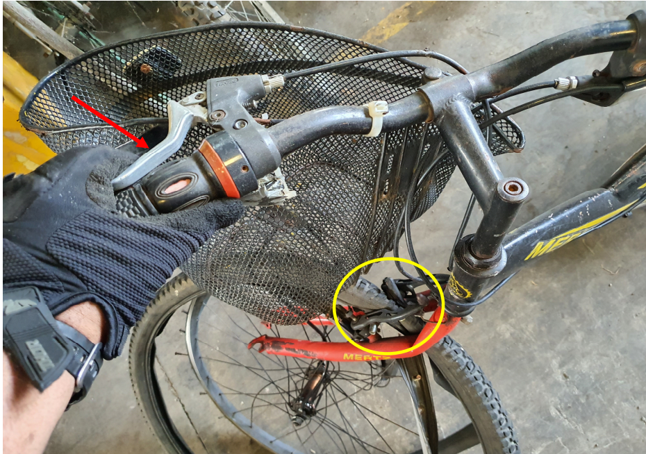
Photo 16 shows a static brake test conducted on the Bicycle's front brake. There was some resistance felt upon pressing the left hand brake lever (arrowed). It also shows that the front brake clamps responded to the gripping action (circled) after depressing the left hand brake lever.
