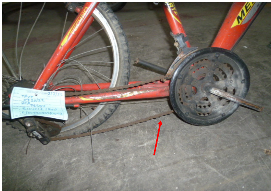
Photo 14 shows the general view of the gear train of the Bicycle which was found to be severely damaged as a result of the accident. The chain was also observed to be dislodged from the gear train most likely as a result of the accident (arrowed).
