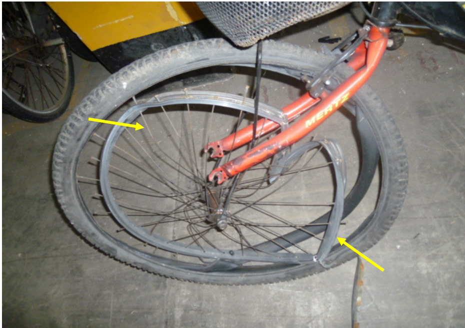
Photo 11 shows the bent spokes and bent front wheel rim of the Bicycle at the time of our inspection (arrowed).
