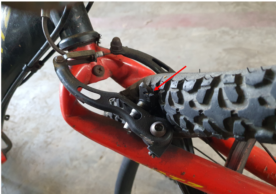
Photo 17 shows a close up view of the front brake clamps responding to the gripping action. The rubber brake blocks pressed against the front wheel rim upon depressing the left hand brake lever. However due to the misalignment of
