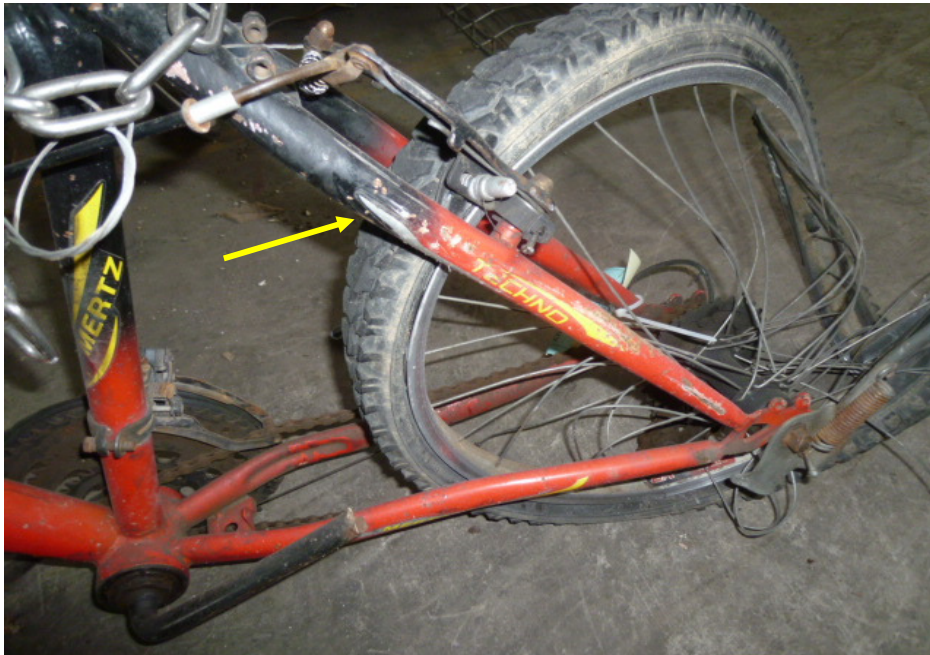
Photo 9 shows the grazed rear sub frame of the Bicycle as a result of the accident (arrowed).
