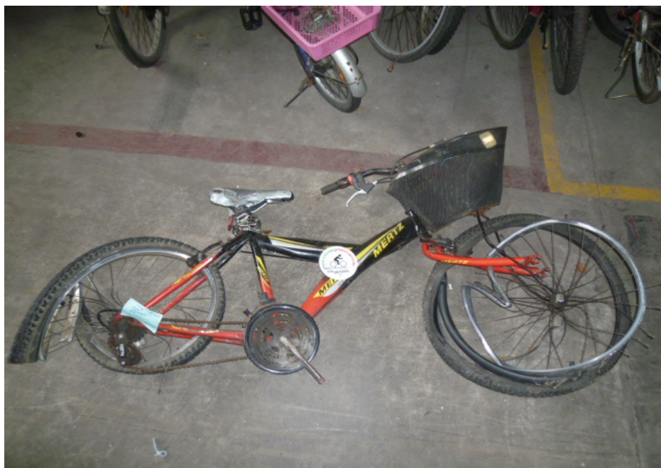
Photo 2 shows the right body of the Bicycle at time of our inspection. The Bicycle had sustained damages all around. The body parts that were found to have been damaged include its front basket, rear sub frame, pedals, braking components, gear train and rack, amongst others as a result of the accident.
