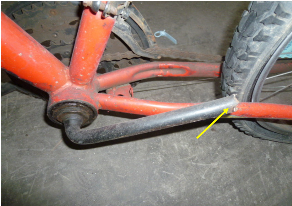
Photo 7 shows the broken left pedal of the Bicycle as a result of the accident (arrowed).
