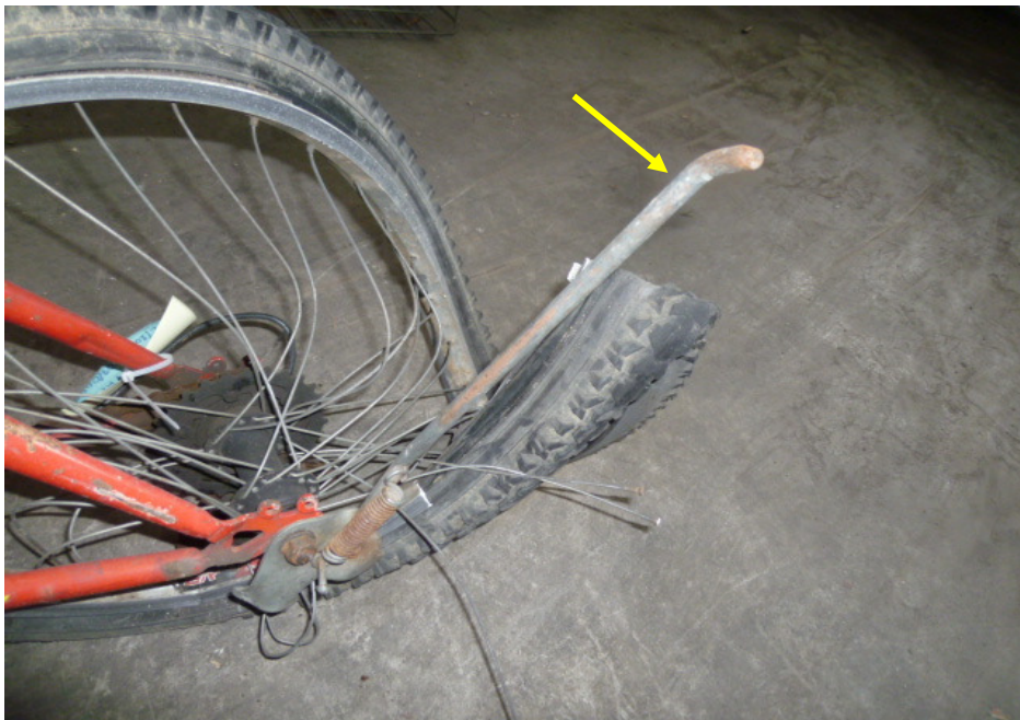
Photo 6 shows a close-up view of the bent side stand of the Bicycle due to the accident (arrowed).
