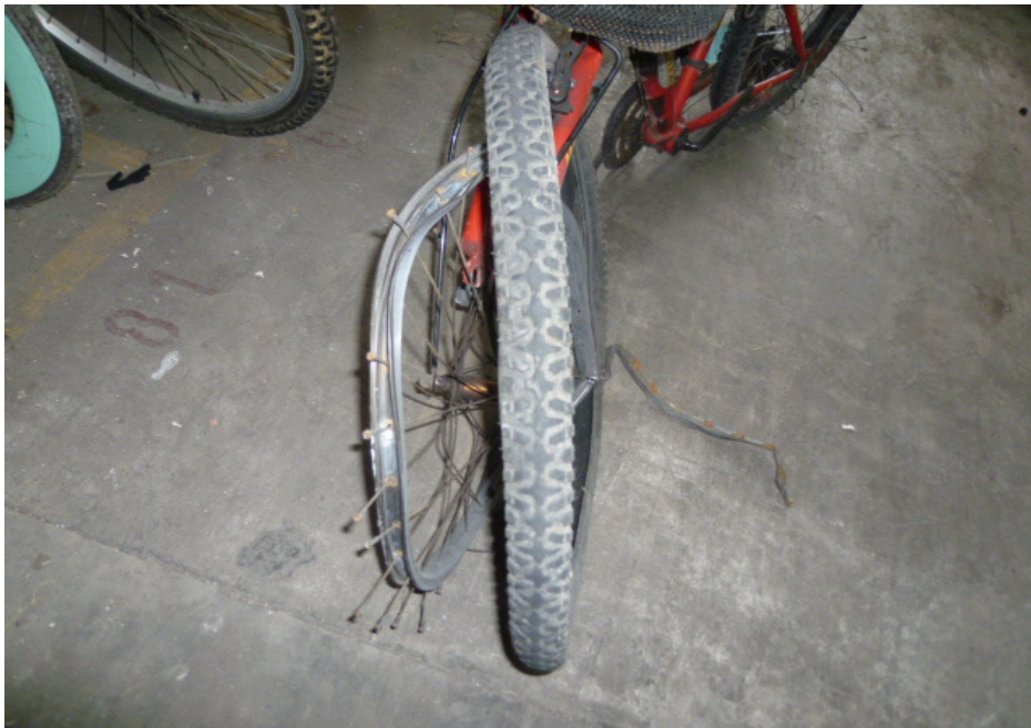
Photo 10 shows the deflated front tyre of the Bicycle most likely as a result of the accident. The pattern of the tread was clearly visible. There was no tear, burst mark(s) and/or punctured hole(s) on the sidewalls as well as across the tread of the front tyre.
