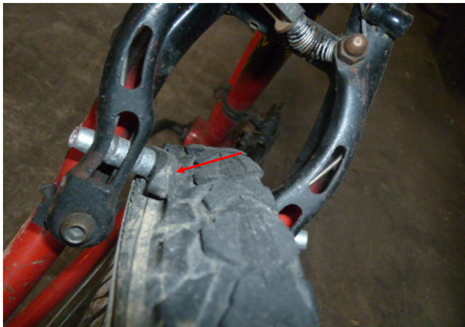
Photo 19 shows a close up view of the rear brake clamps responding to the gripping action. The rubber brake blocks pressed against the rear wheel rim upon depressing the right hand brake lever. However due to the misalignment of the
