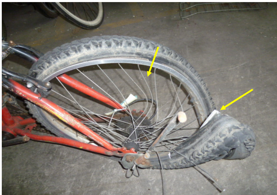
Photo 13 shows the bent spokes and bent rear wheel rim of the Bicycle at the time of our inspection (arrowed).
