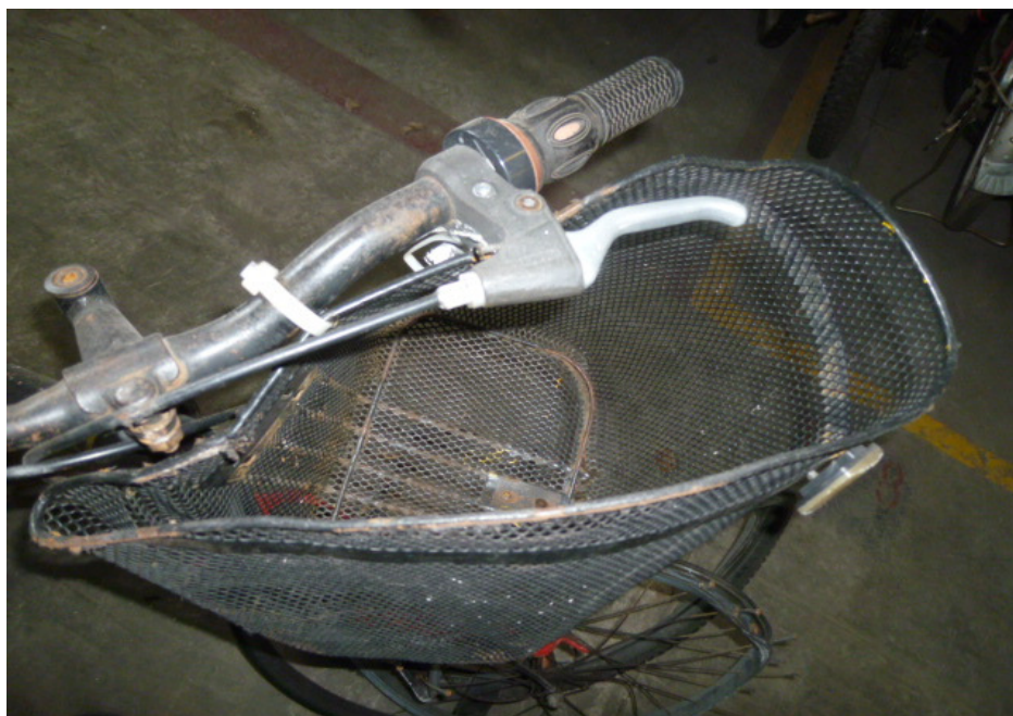
Photo 4 shows the damaged front basket of the Bicycle at the time of our inspection.
