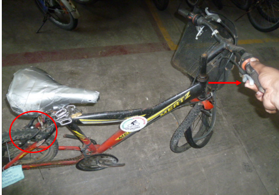
Photo 18 shows a static brake test conducted on the Bicycle's rear brake. There was some resistance felt upon pressing the right hand brake lever (arrowed). It also shows that the rear brake clamps responded to the gripping action (circled) after depressing the right hand brake lever.
