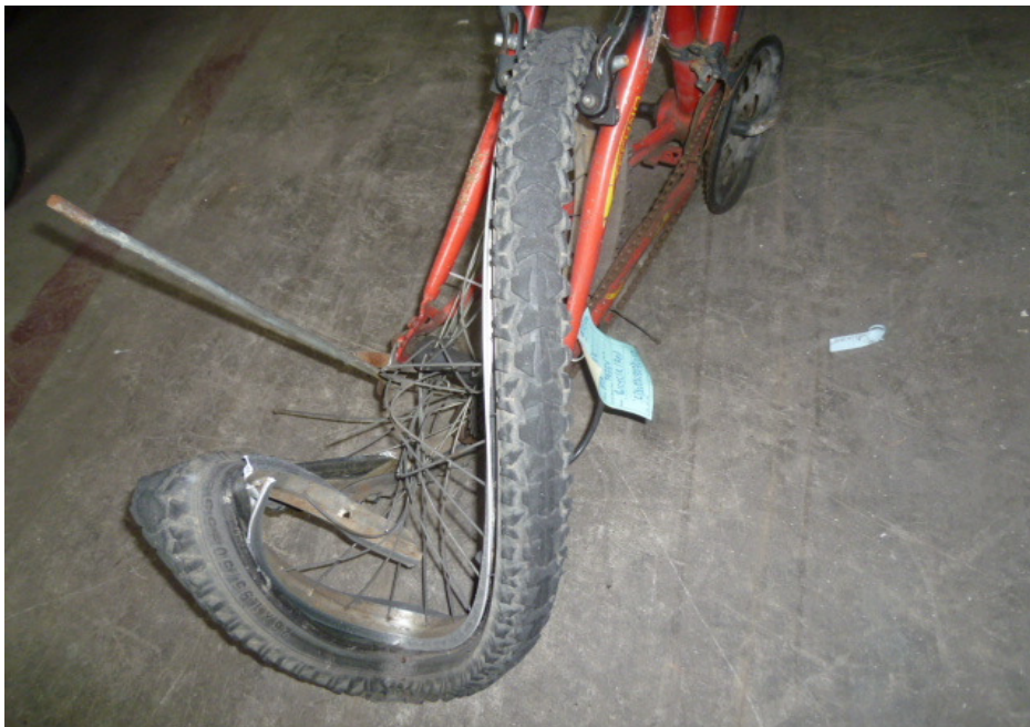
Photo 12 shows the deflated rear tyre of the Bicycle most likely as a result of the accident. The pattern of the tread was clearly visible. There was no tear, burst mark(s) and/or punctured hole(s) on the sidewalls as well as across the tread of the rear tyre.
