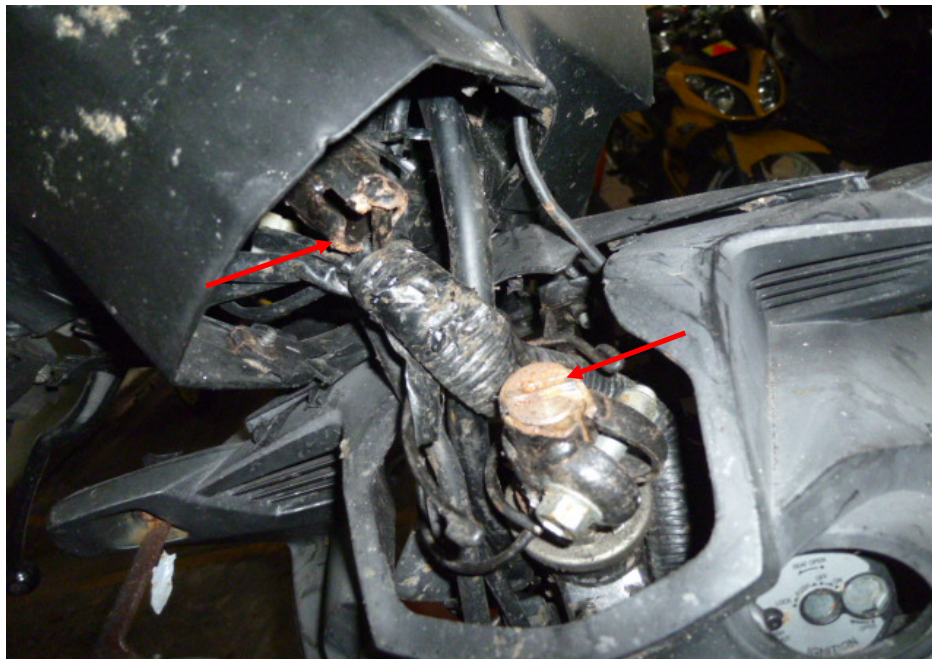
Photo 25 shows the steering stem of the Motorcycle. The steering stem was observed to be broken as a result of the accident (arrowed). We were hence not able to conduct any tests on the steering system of the Motorcycle.
