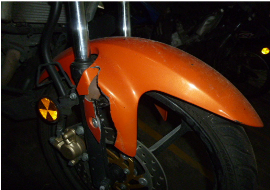
Photo 6 shows a closer view of the cracked front mudguard which was amongst the body parts of the Motorcycle that had sustained damage as a result of the accident.
