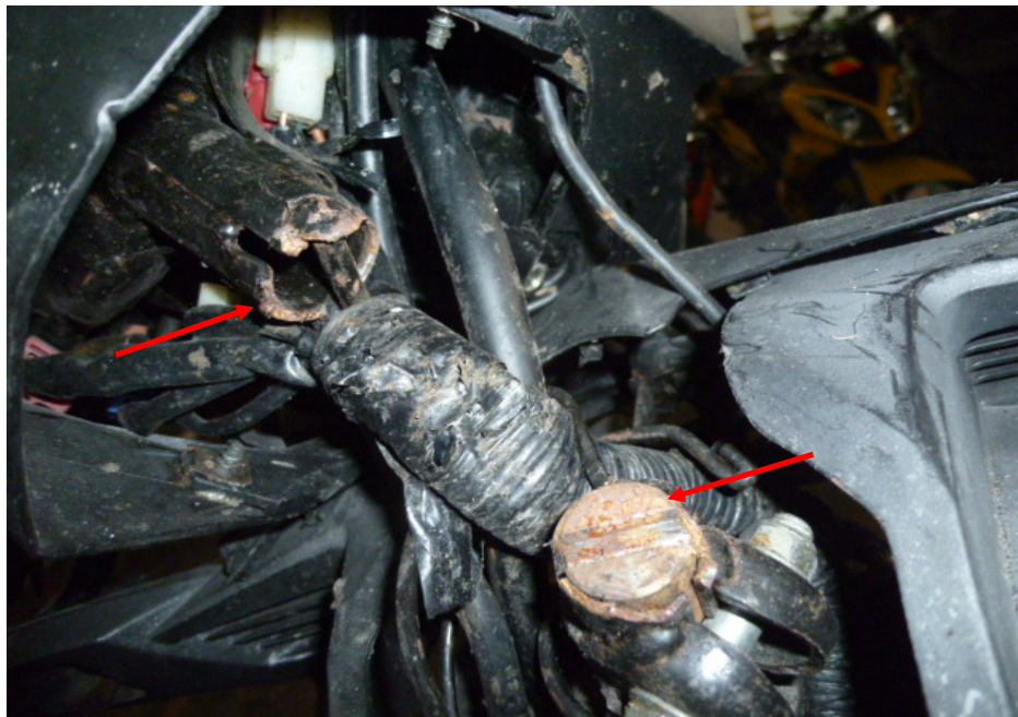
Photo 26 shows a close up view of the steering stem of the Motorcycle. The steering stem was observed to be broken as a result of the accident (arrowed). We were hence not able to conduct any tests on the steering system of the Motorcycle.
