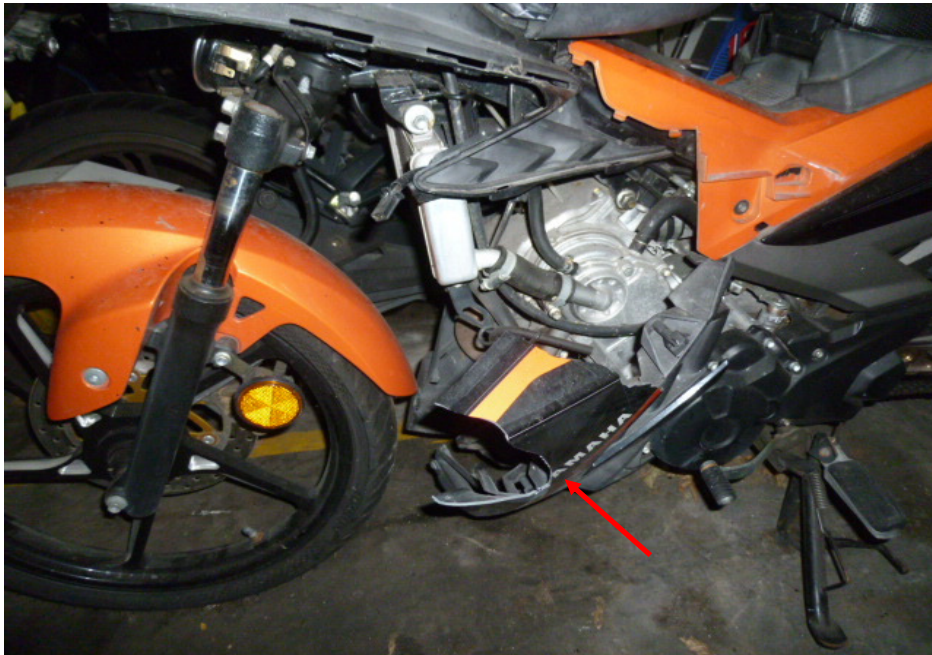
Photo 13 shows a closer view of the cracked left cowling of the Motorcycle as a result of the accident (arrowed).
