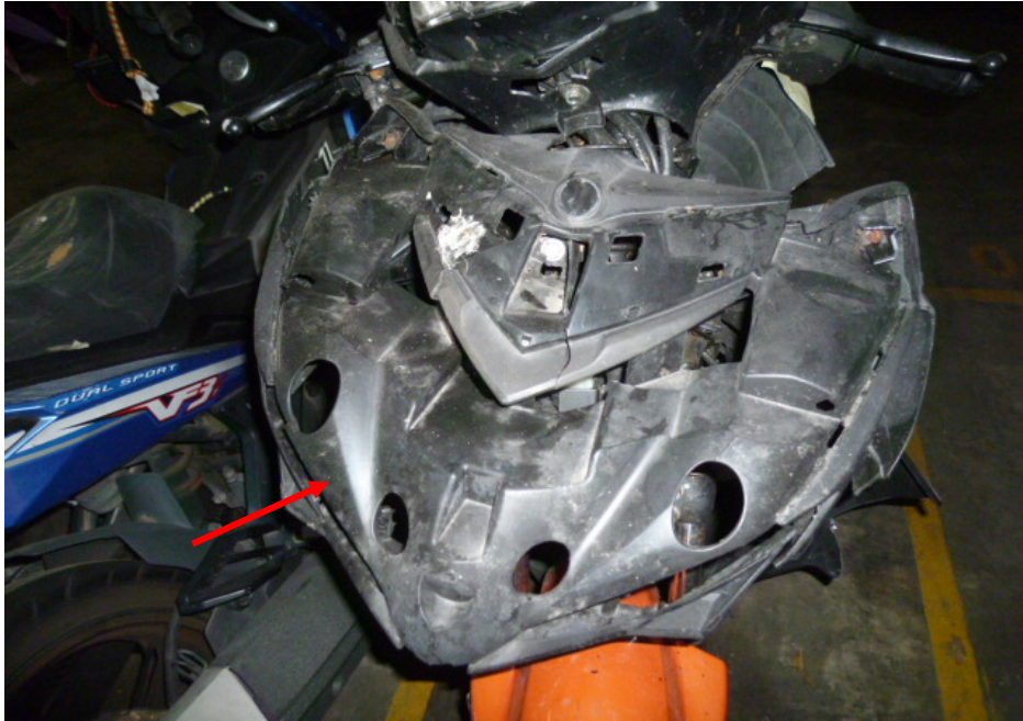
Photo 9 shows a closer view of the missing front cowling of the Motorcycle as a result of the accident (arrowed).
