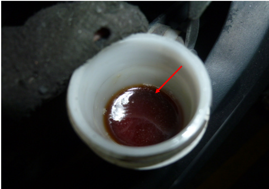
Photo 32 shows the brake fluid reservoir for the rear brake of the Motorcycle. The brake fluid was observed to be of sufficient level for operating purposes. However it was found to be slightly contaminated (arrowed).
