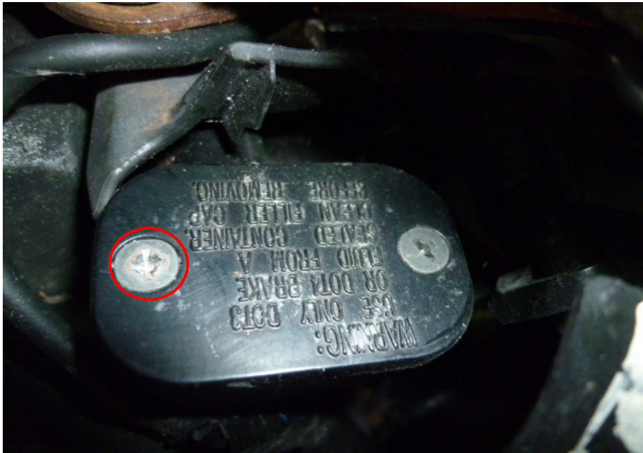
Photo 28 shows the brake fluid reservoir cover for the front brake of the Motorcycle. We were unable to examine whether the front brake fluid was without contamination due to the worn out screw (circled).
