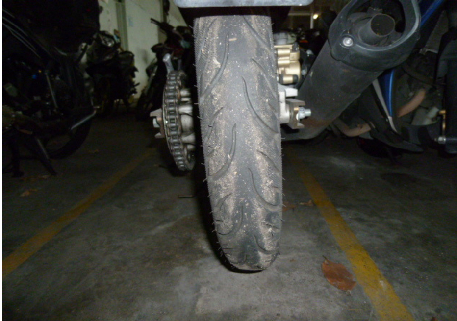
Photo 19 shows the condition of the Motorcycle's rear tyre. The rear tyre was observed to be in serviceable condition with remaining tread depth of approximately 4mm. There was no tear, burst mark(s) and/or punctured hole(s) on the sidewalls as well as across the tread of the rear tyre. However the rear tyre was observed to be deflated.
