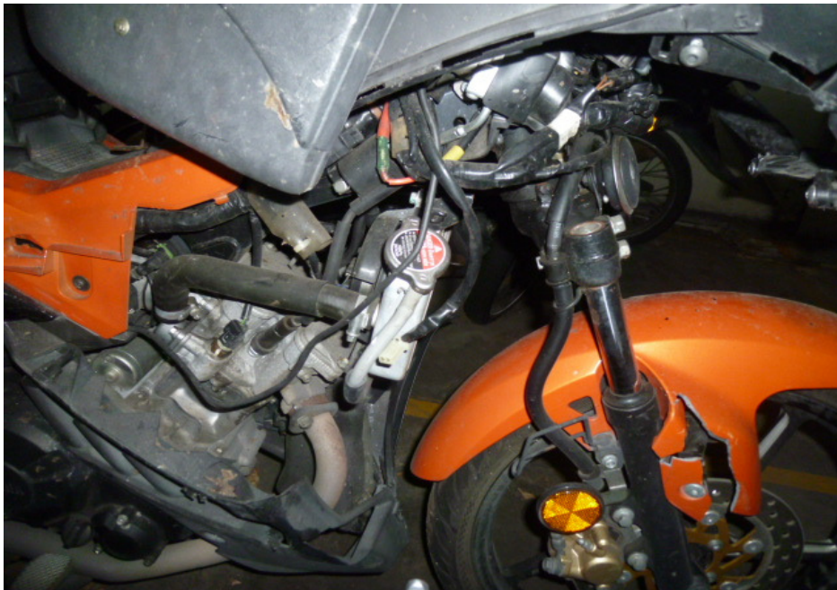
Photo 8 shows a closer view of the missing right cowling of the Motorcycle as a result of the accident.
