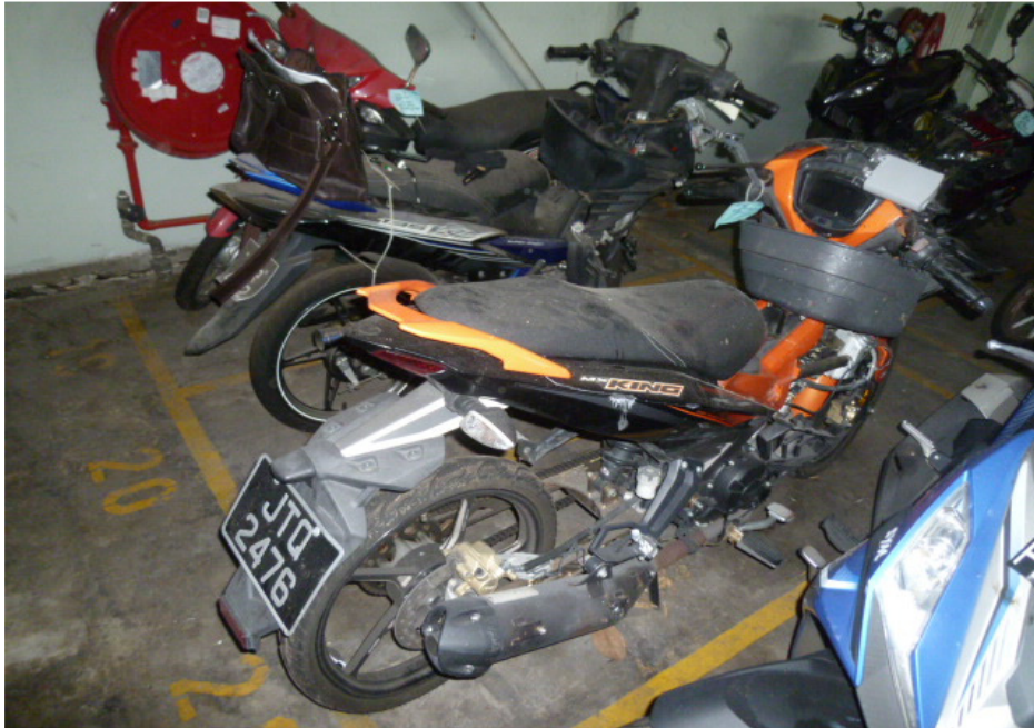
Photo 5 shows a general view of the right rear body of the Motorcycle at the time of our inspection. The Motorcycle was observed to have sustained damages all around. The body parts that were found to have been damaged include its steering stem, headlight assembly, front cowling, front mudguard, side cowlings, side mirrors, front brake lever and right rear side cover, amongst others.
