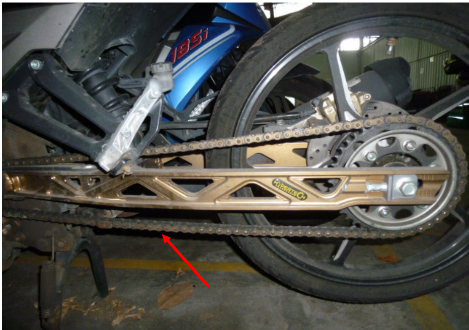
Photo 23 shows the general view of the gear train (arrowed) of the Motorcycle, which was observed to be intact with no misalignment. It was also adequately lubricated for operating purposes.
