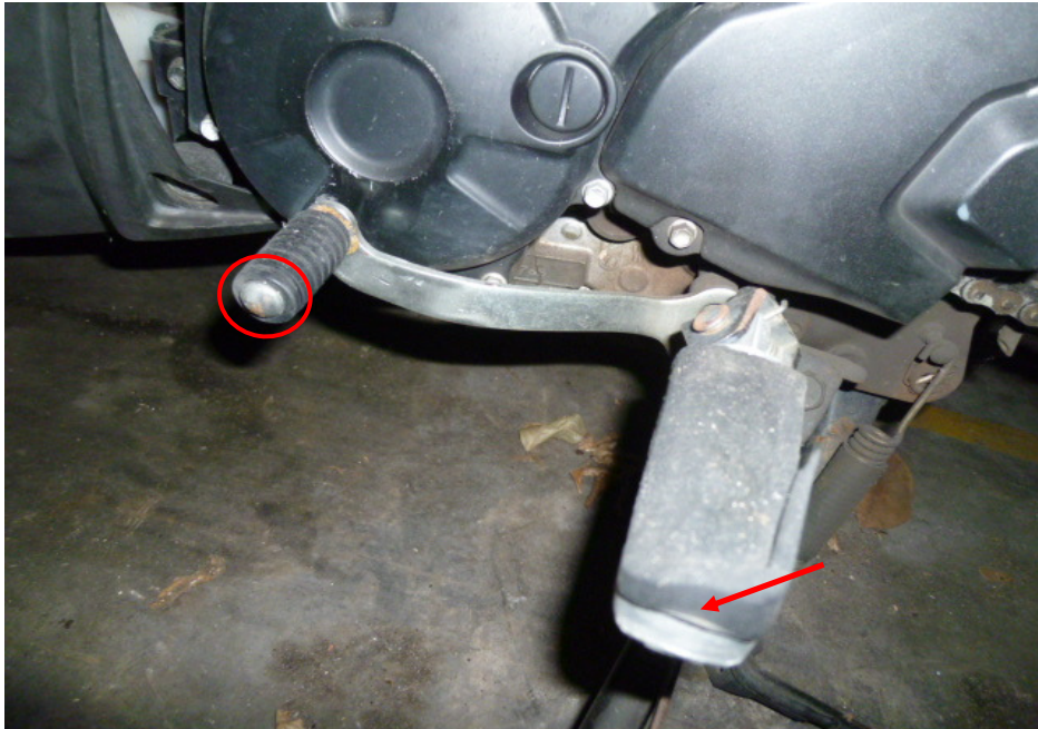
Photo 15 shows the gear shift pedal (circled) and left front footrest (arrowed) of the Motorcycle that had sustained damage as a result of the accident.
