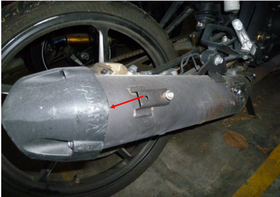
Photo 17 shows the grazed exhaust muffler heat shield of the Motorcycle as a result of the accident (arrowed).
