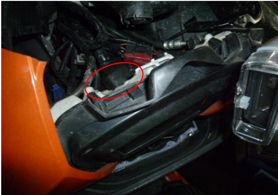
Photo 1 shows the damaged speedometer gauge of the Motorcycle as a result of the accident (circled). Hence the mileage of the Motorcycle could not be recorded at the time of our inspection.
