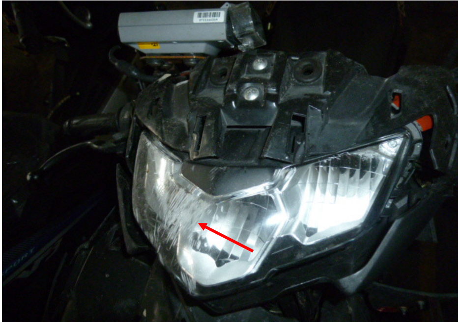
Photo 7 shows the grazed headlight assembly (arrowed), which was amongst the body parts of the Motorcycle that had sustained damage as a result of the accident.
