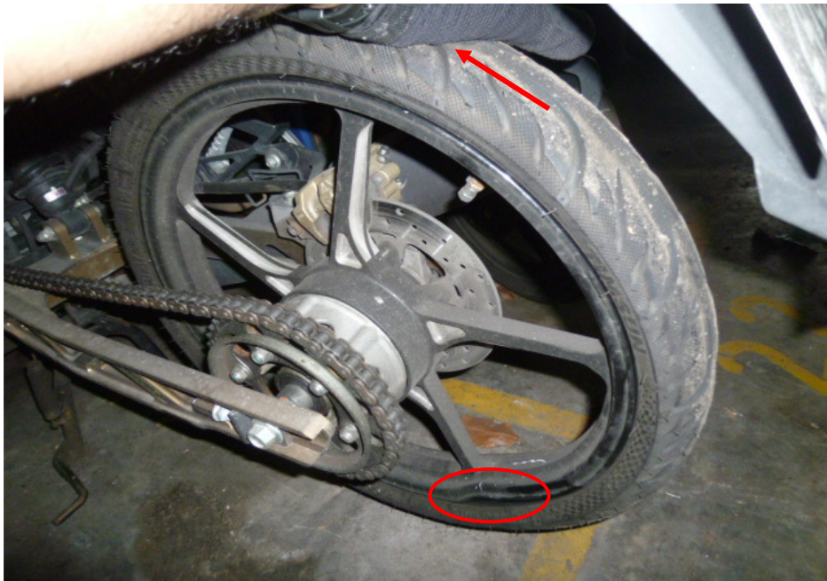
Photo 20 shows the bent rear wheel rim (circled) and deflated rear tyre (arrowed) of the Motorcycle at the time of our inspection.
