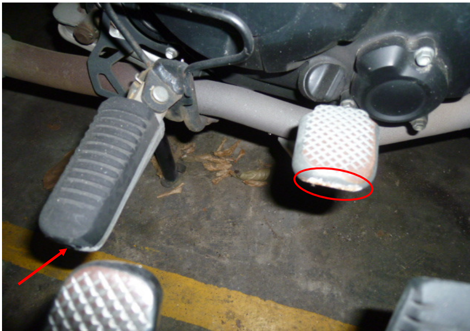
Photo 16 shows the rear brake pedal (circled) and right front footrest (arrowed) of the Motorcycle that had sustained damage as a result of the accident.
