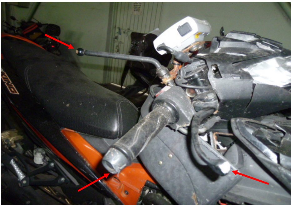
Photo 10 shows the right handlebar end, front brake lever and right side mirror (arrowed), which were amongst the body parts of the Motorcycle that had sustained damage as a result of the accident.
