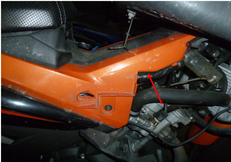
Photo 12 shows a closer view of the cracked right centre cover (arrowed) which was amongst the body parts of the Motorcycle that had sustained damage as a result of the accident.
