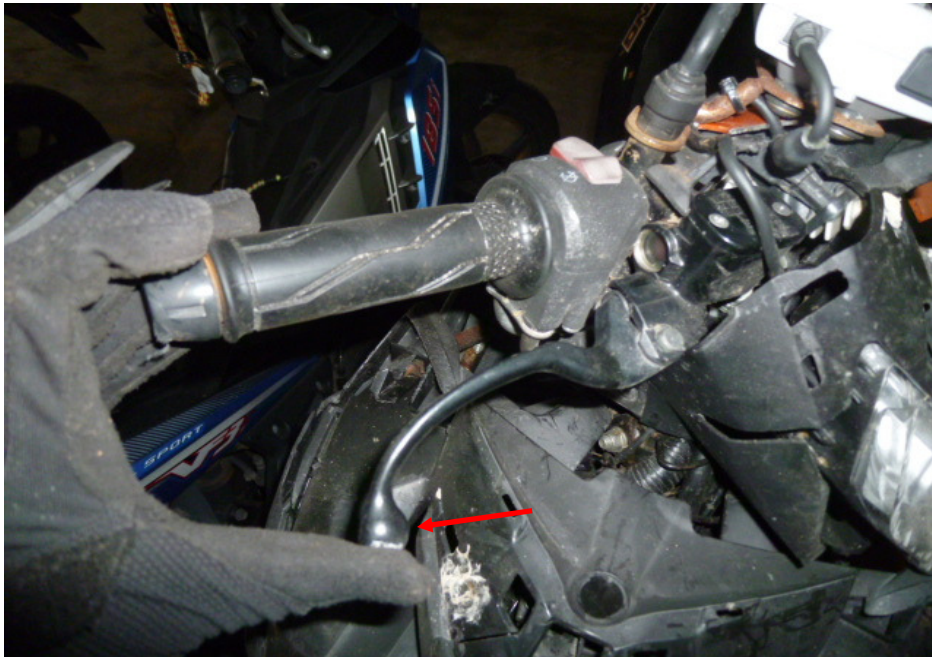
Photo 30 shows the front brake lever being depressed. There was some resistance felt (spongy like feel) upon pressing the front brake lever (arrowed). This would indicate that there is no leakage of pressure/vacuum in the front brake system.
