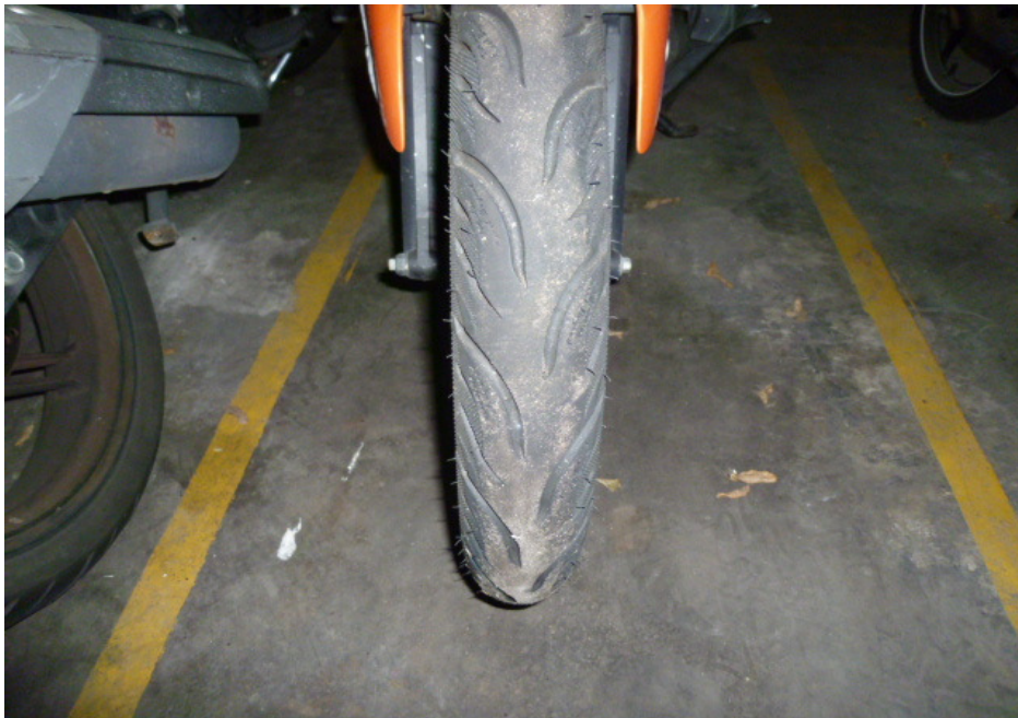
Photo 18 shows the condition of the Motorcycle's front tyre. The front tyre was observed to be in serviceable condition with remaining tread depth of approximately 5mm. The tyre was also observed to be sufficiently inflated for vehicular operation. We did not observe any tear, burst mark(s) and/or punctured hole(s) on the sidewalls as well as across the tread of the front tyre.
