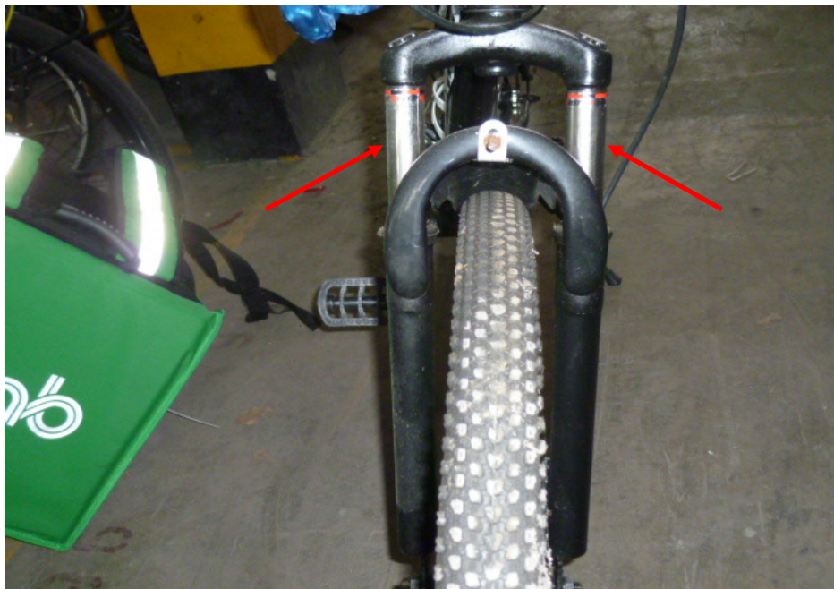
Photo 17 shows the front fork assembly (arrowed) of the Bicycle. The front forks and fork bracket of the Bicycle were both found to be intact and undamaged. Turning the Bicycle's handle bar towards the left and right did not produce any abnormal free play. The steering system of the Bicycle was in serviceable condition at the time of our inspection.
