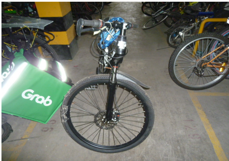
Photo 19 shows the front wheel of the Bicycle turned towards its full right. Turning the Bicycle's handle bar towards the right did not produce any abnormal free play and/or resistance. This would indicate that the steering system of the Bicycle was in serviceable condition at the time of our inspection.
