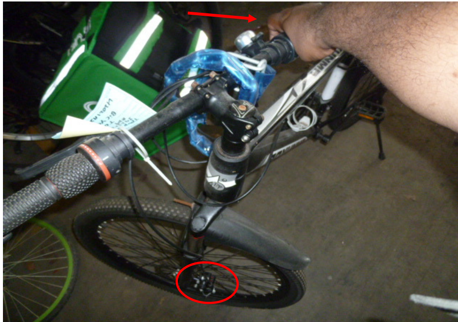
Photo 20 shows a static brake test conducted on the Bicycle's front brake. There was some resistance felt upon pressing the right hand brake lever (arrowed). It also shows that the front brake pads responded to the gripping action (circled) after depressing the right hand brake lever.
