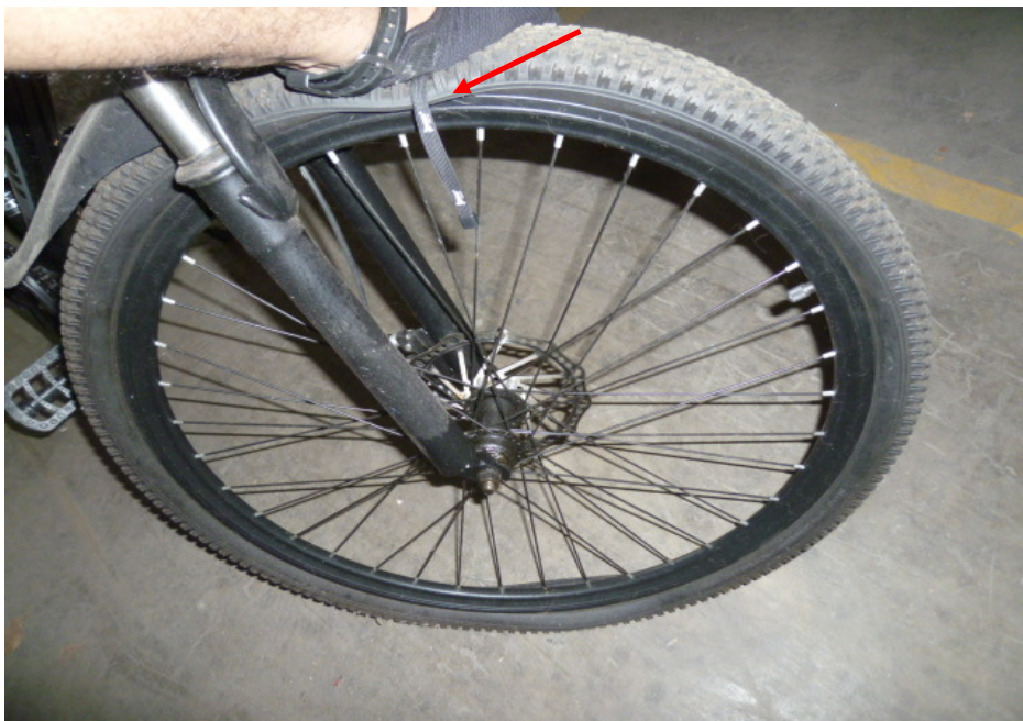
Photo 12 shows the deflated front tyre of the Bicycle (arrowed).
