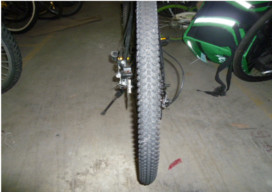
Photo 13 shows the rear tyre of the Bicycle. The pattern of the tread was clearly visible. There was no tear, burst mark(s) and/or punctured hole(s) on the sidewalls as well as across the tread of the rear tyre. However the rear tyre was observed to be deflated.
