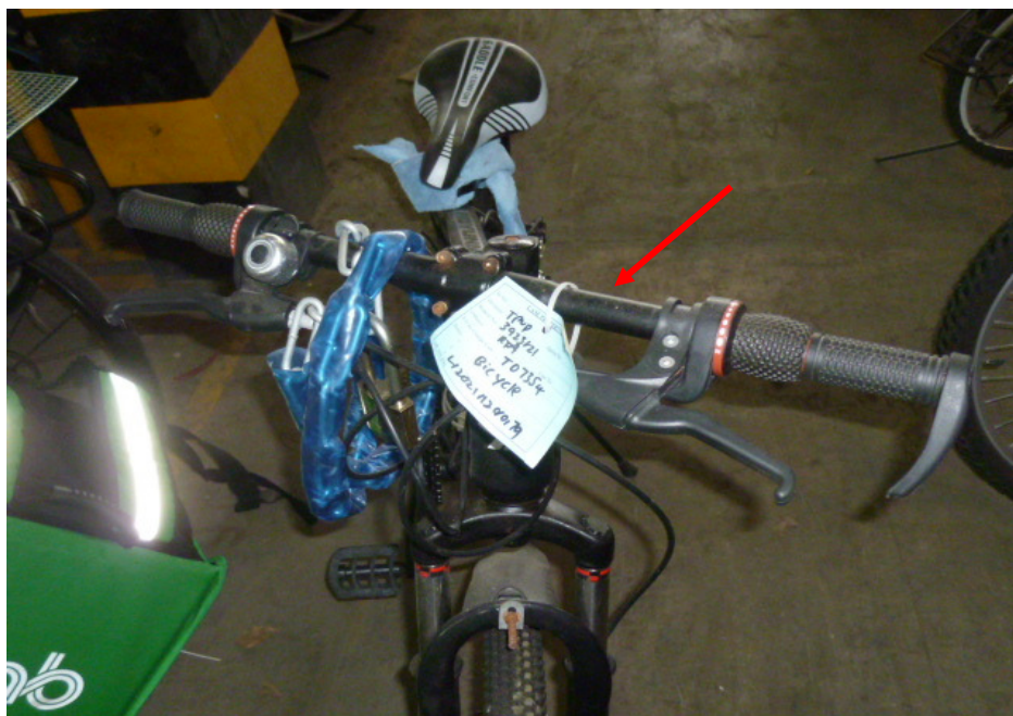
Photo 10 shows a close-up view of the deformed handlebar of the Bicycle as a result of the accident (arrowed).
