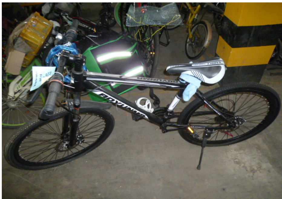
Photo 4 shows the left body of the Bicycle at the time of our inspection. The Bicycle had sustained damages all around. The front mudguard, handlebar, left hand brake lever guard, right hand brake lever, right handlebar end and left pedal, amongst others as a result of the accident.
