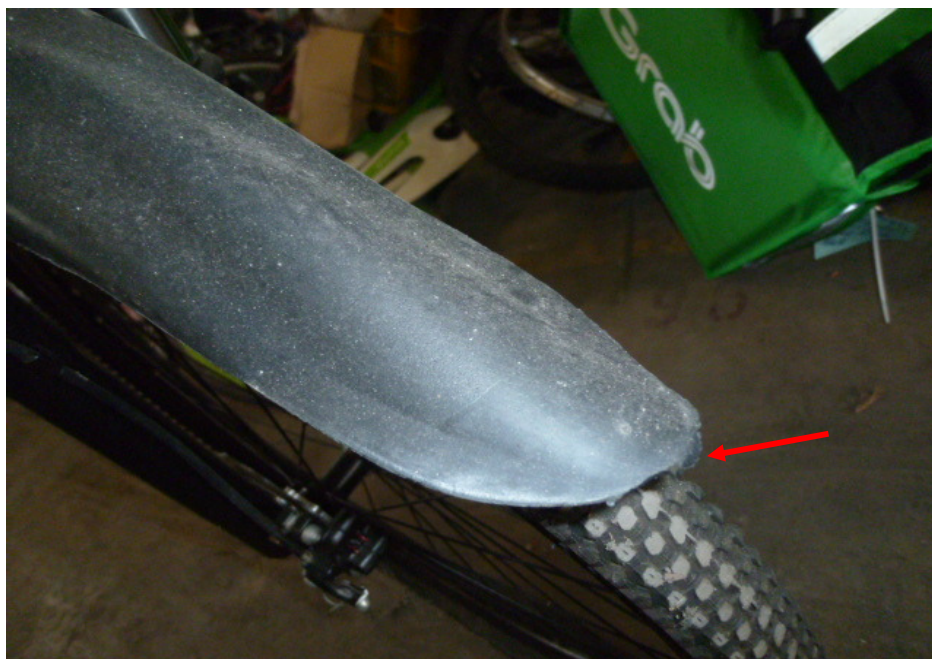
Photo 7 shows the damages of grazing nature on the front mudguard (arrowed) of the Bicycle at the time of our inspection.
