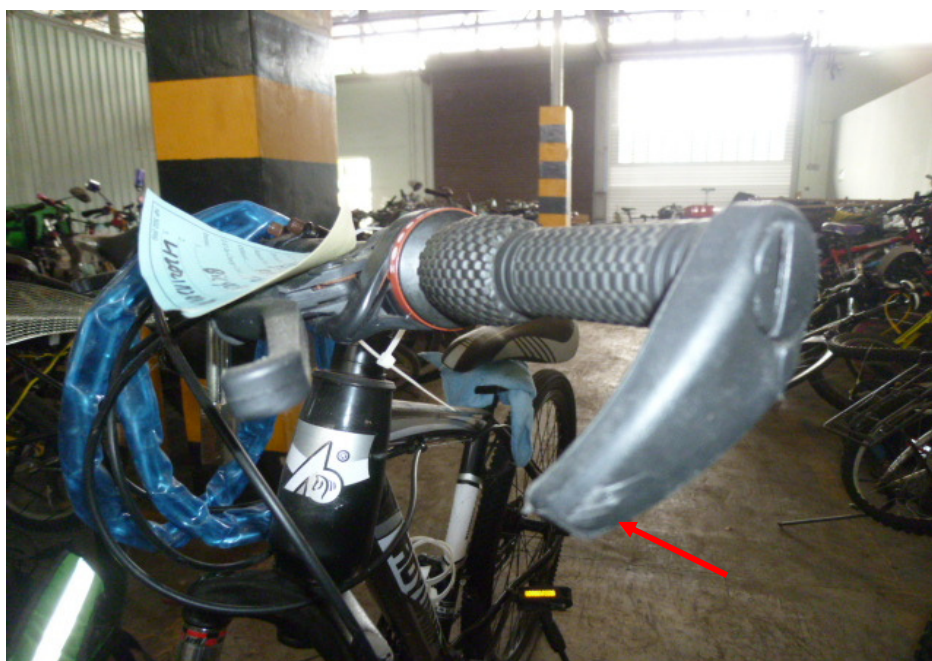
Photo 6 shows the damaged left hand brake lever guard (arrowed) of the Bicycle at the time of our inspection.
