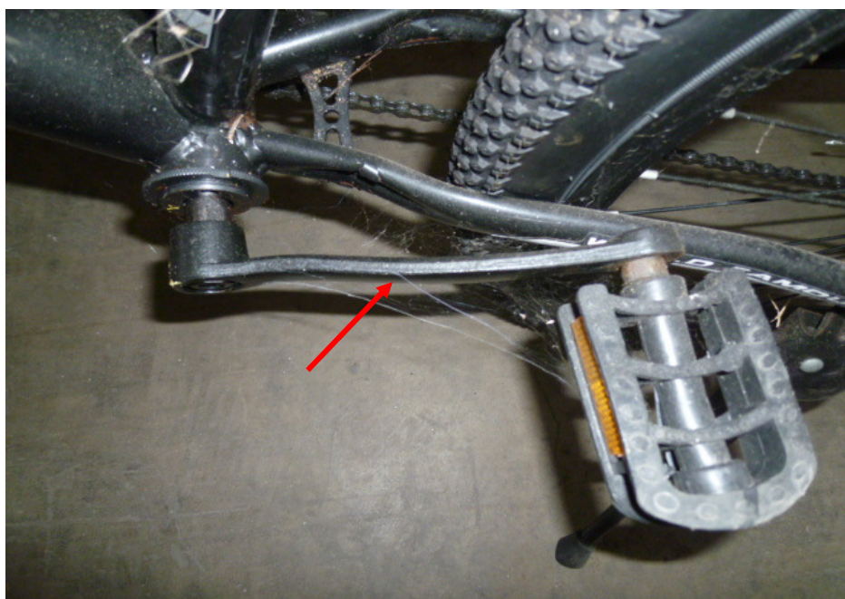
Photo 8 shows the deformed left pedal of the Bicycle at the time of our inspection (arrowed).
