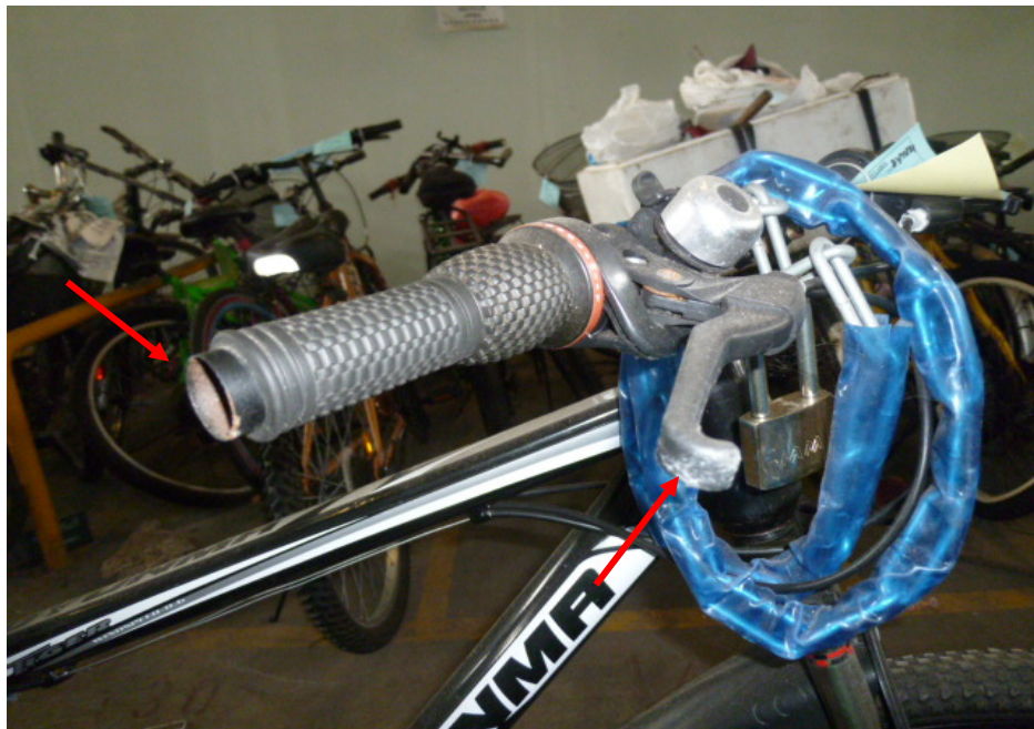
Photo 9 shows the damages of grazing nature on the right hand brake lever and right handlebar end of the Bicycle at the time of our inspection (arrowed).
