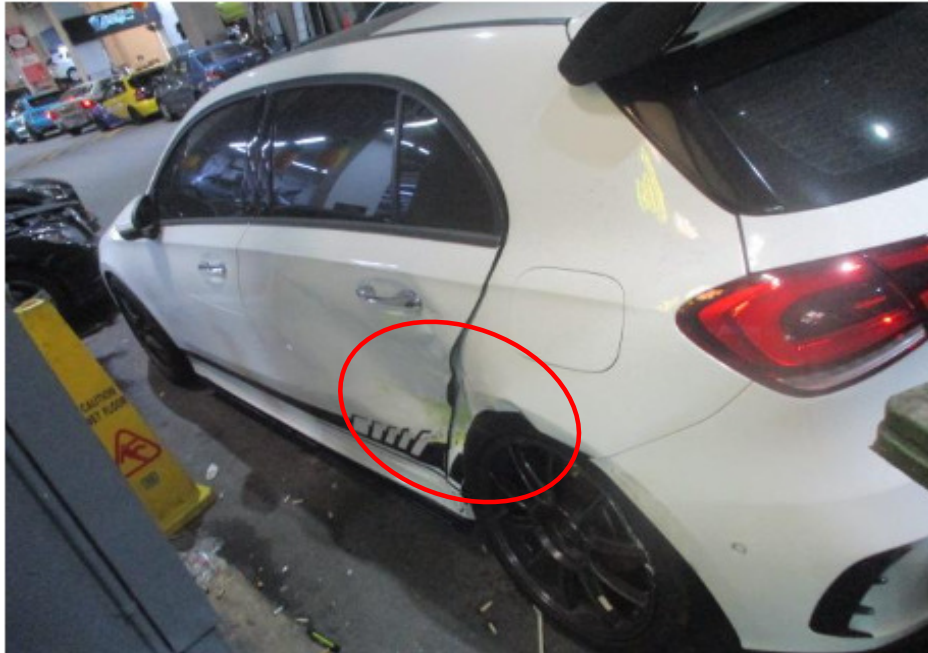
Photo 8 shows a view of the left rear portion of the Insured Vehicle during the physical inspection at Teamwork. The Insured Vehicle had sustained damages to its left rear portion as a result of the accident (circled).
