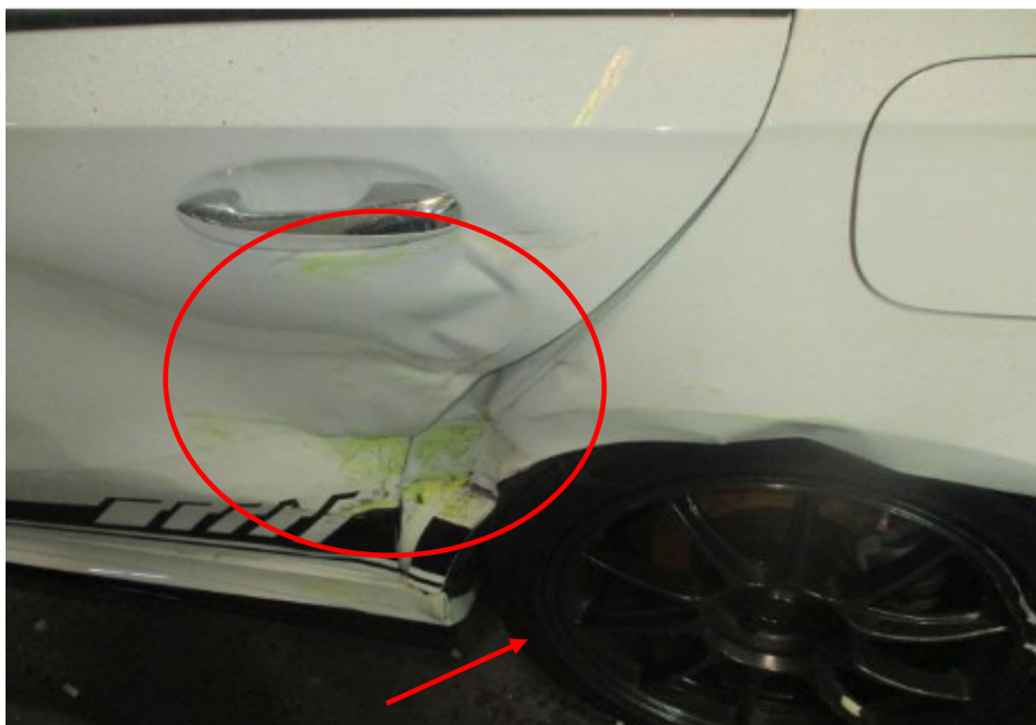
Photo 9 shows a closer view of the dents, yellow paint transfer marks and graze marks on the left rear portion of the Insured Vehicle (circled). There was also a misalignment of the left rear wheel rim (arrowed).
