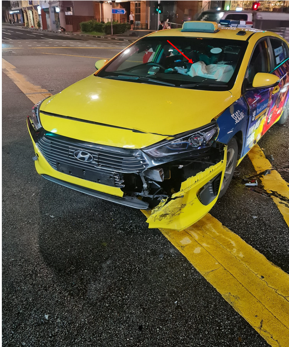
Photo 5 shows a frontal view of the Taxi post- accident. It seems to correlate with Mr Ong's statement in which he mentioned the front passenger airbag of the Taxi had been deployed upon collision (arrowed).
