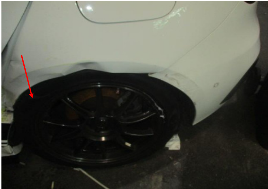
Photo 10 shows the misalignment of the left wheel rim of the Insured Vehicle (arrowed) which would appear to correspond to the left rear portion of the Insured Vehicle being hit by the frontal portion of the Taxi.
