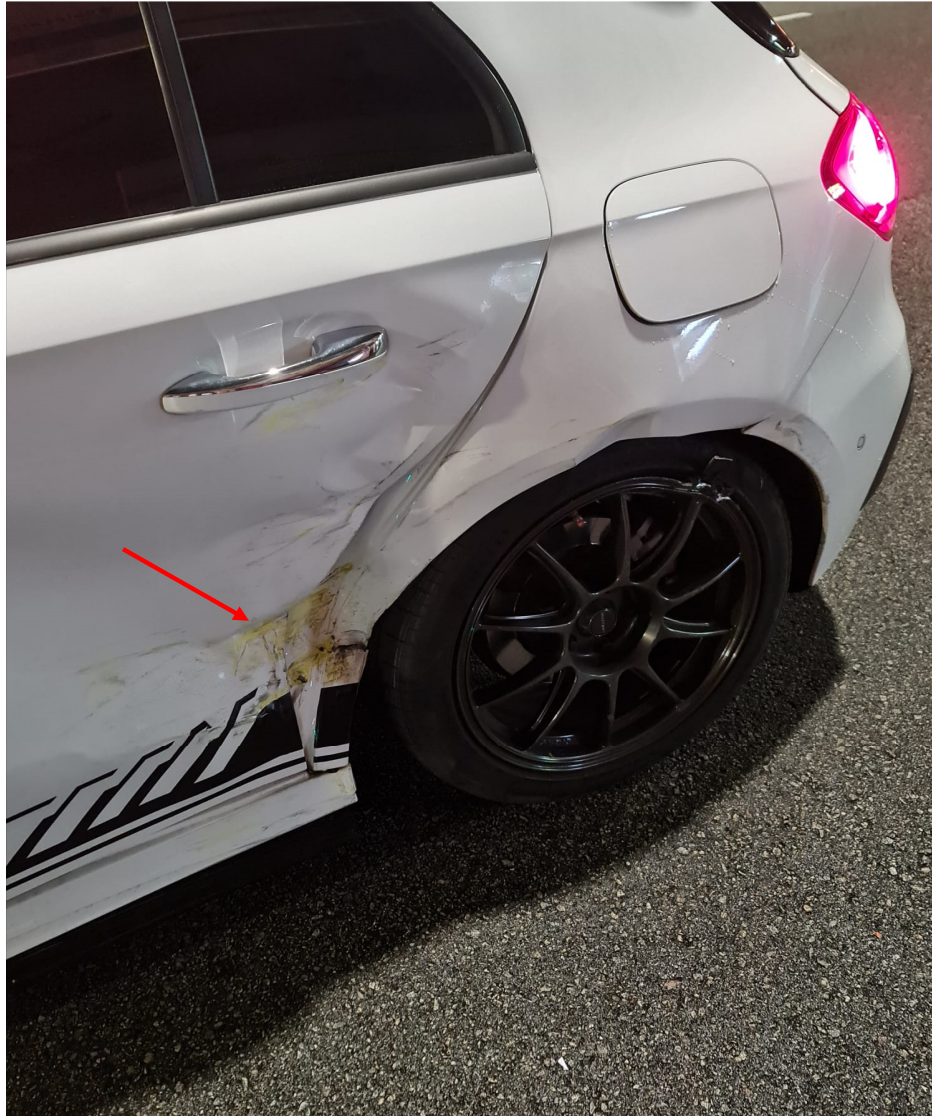
Photo 3 shows a closer view of the damages sustained to the Insured Vehicle as a result of the accident. It seems to correlate with Mr Ong's statement in which the frontal portion of the Taxi had collided into the left rear portion of the Insured Vehicle (arrowed).
