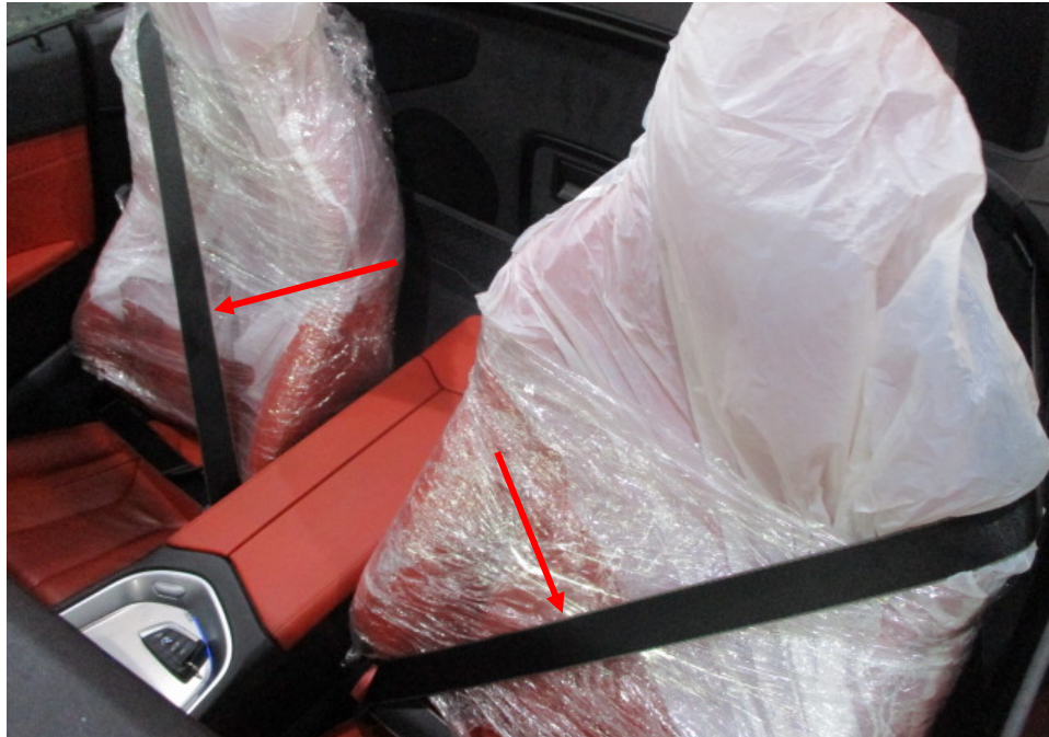
Photo 15 shows the seats of the Motor Car. All the seats of the Motor Car were secured via seat rails to the floorboard. They were also fitted with a retractable seat belt reel and a pre-tensioner. The seat belts (arrowed) were tested and were able to be fastened into the respective pre-tensions that were fitted on the side of each individual seat.
