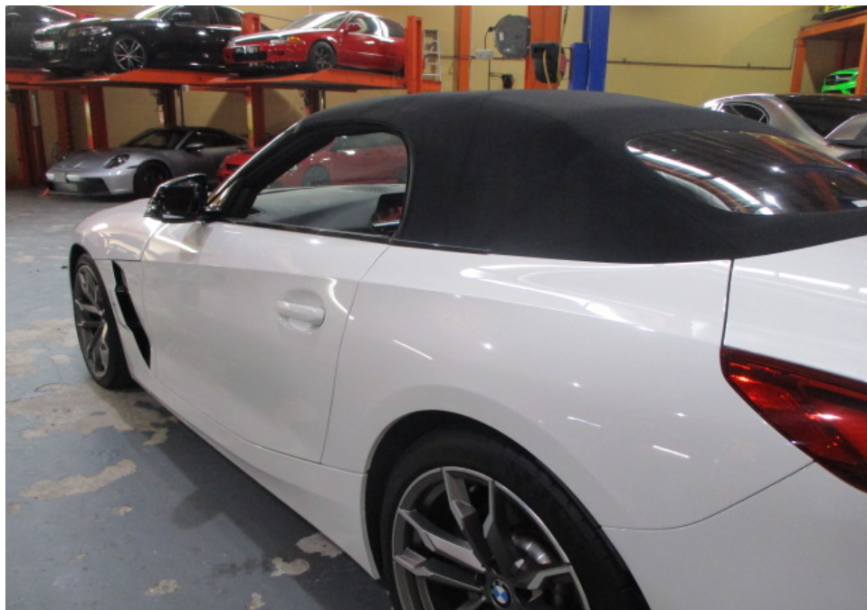
Photo 10 shows a closer view of the Motor Car's left rear body panel, front left door and front left door handle at the time of my inspection. The body parts at the left rear portion of the Motor Car were visually examined and it was observed that the repair/restoration works carried out to the damaged area of the Motor Car (refer to photograph 3 above) were reasonably adequate and in order.
