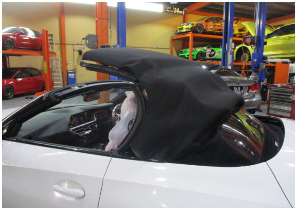
Photo 16 shows the Motor Car's soft top roof being tested. It was observed that as a safety feature, the soft top roof could only open and close when the Motor Car was in a stationary position. When opened, the soft top roof is completely folded into the rear compartment with no parts protruding out of the Motor Car's body. The soft top roof was also found adequately secured to the "A" pillar after closing.
