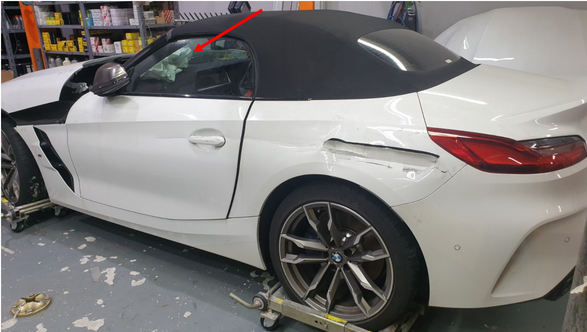
Photo 3 shows the left rear body of the Motor Car (photograph provided to me). Apart for the front right portion, I had also observed damage to the left rear portion of the Motor Car. Body parts damaged include the left rear body panel, front left door and front left door handle. The front left passenger airbag (arrowed) was also deployed.
