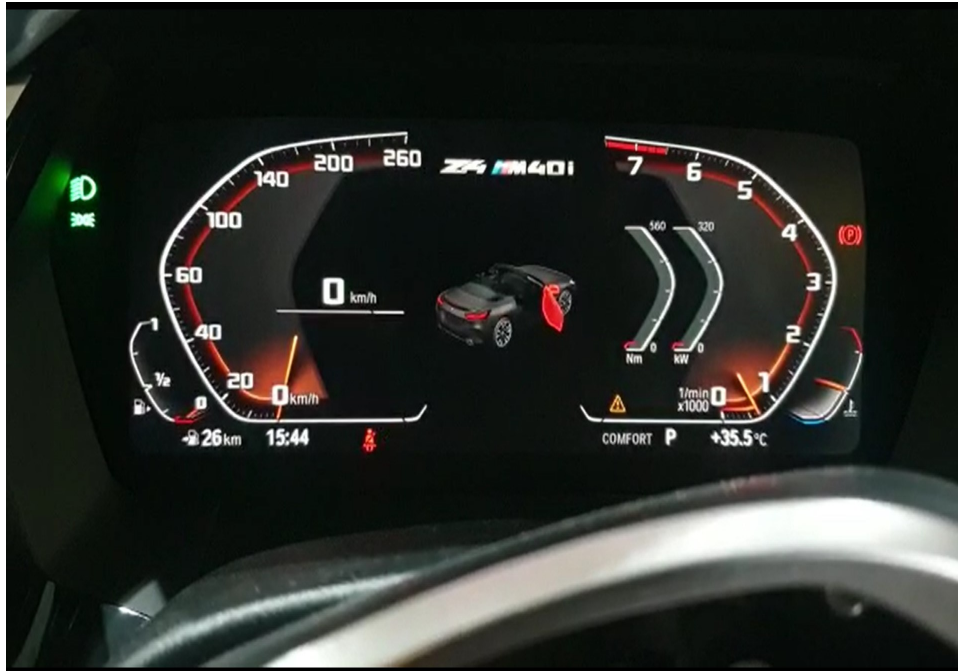
Photo 19 shows the respective warning lights no longer illuminated, indicating that there is no fault detected to the ABS, SRS, IAS, TPM and DSC systems of the Motor Car during the self-test. These electronic systems were hence in working condition at the time of my inspection.
