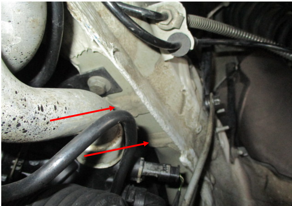
Photo 33 shows the chassis/structural body at the underside front left of the Motor Car. I did not find any weld marks other than original spot weld marks on the chassis/structural body of the Motor Car. The original factory sealant (arrowed) at the joints along the chassis/structural body was untouched, indicating no work was done on the chassis/structural body of the Motor Car and that the chassis/structural body was originally fitted.
