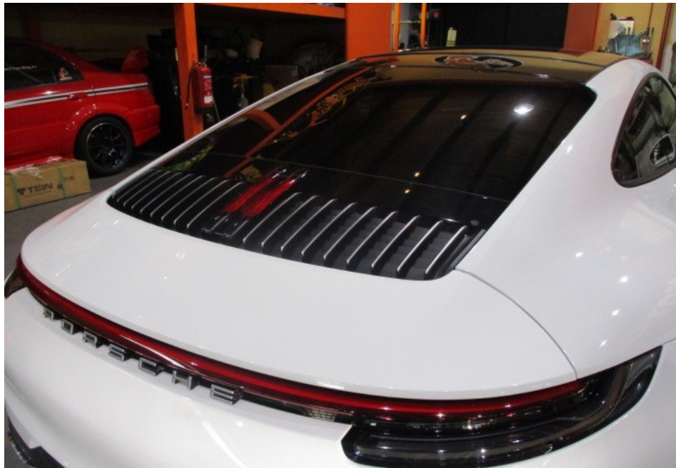
Photo 17 shows a closer view of the Motor Car's rear top cover and rear centre lamp. The body parts at the rear portion of the Motor Car were visually examined and it was observed that the repair/restoration works carried out to the damaged area of the Motor Car (refer to photograph 3 & 4 above) were reasonably adequate and in order.
