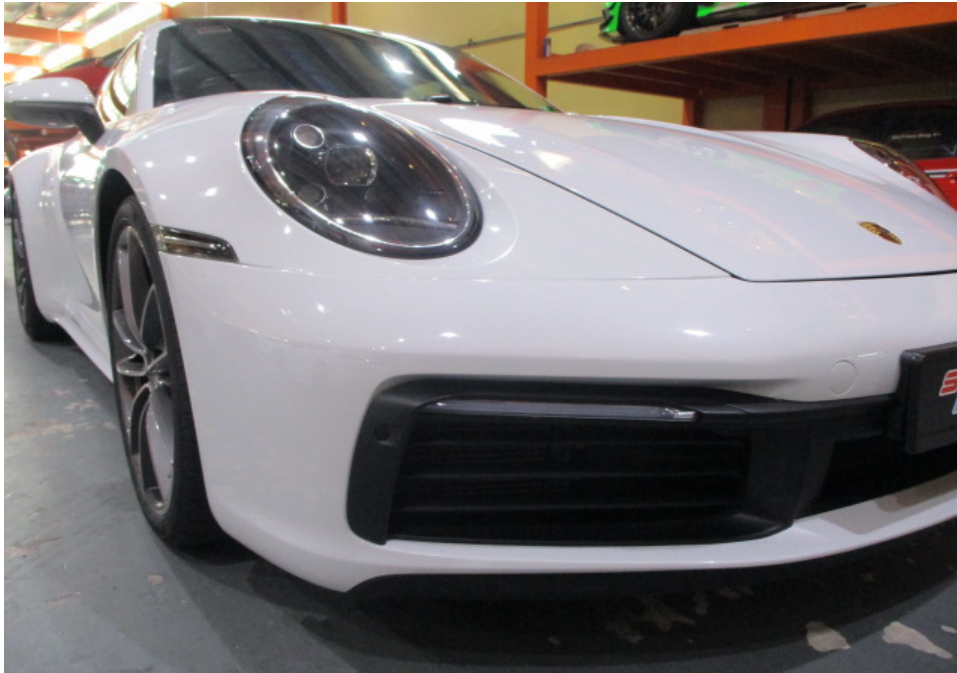
Photo 10 shows a closer view of the Motor Car's front bumper, front bumper right lower grille, front right day light, front right headlamp and front right signal lamp. The body parts at the frontal portion of the Motor Car were visually examined and it was observed that the repair/restoration works carried out to the damaged area of the Motor Car (refer to photograph 1 & 2 above) were reasonably adequate and in order.
