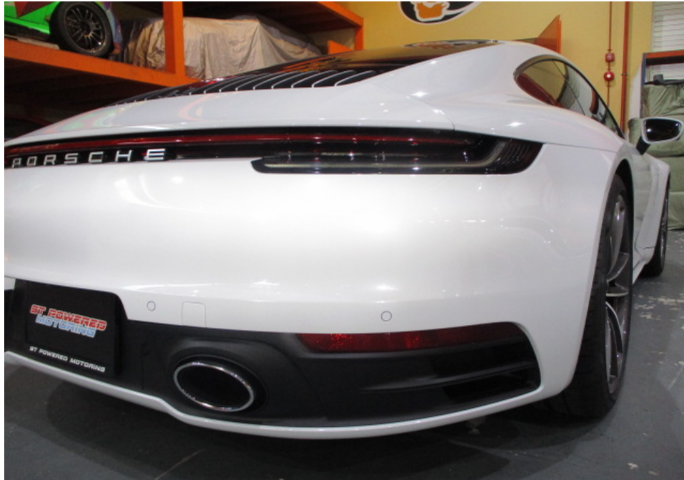
Photo 16 shows a closer view of the Motor Car's rear bumper, rear bumper lower cover, rear bumper right reflector, rear bumper sensors and rear right taillamp. The body parts at the rear portion of the Motor Car were visually examined and it was observed that the repair/restoration works carried out to the damaged area of the Motor Car (refer to photograph 3 & 4 above) were reasonably adequate and in order.
