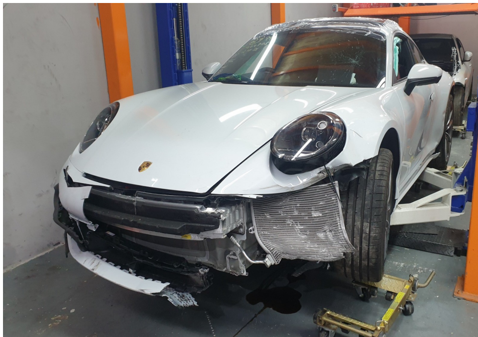
Photo 1 shows the front left body of the Motor Car (photograph provided to me). The photographs provided to me had showed damage to the frontal portion of the Motor Car. The front bumper, front bumper sponge, front bumper reinforcement, front left headlamp, front left aircon condenser and front windscreen were amongst the body parts that were observed to have been damaged. The left curtain airbag and front left passenger airbag were also observed to be deployed.
