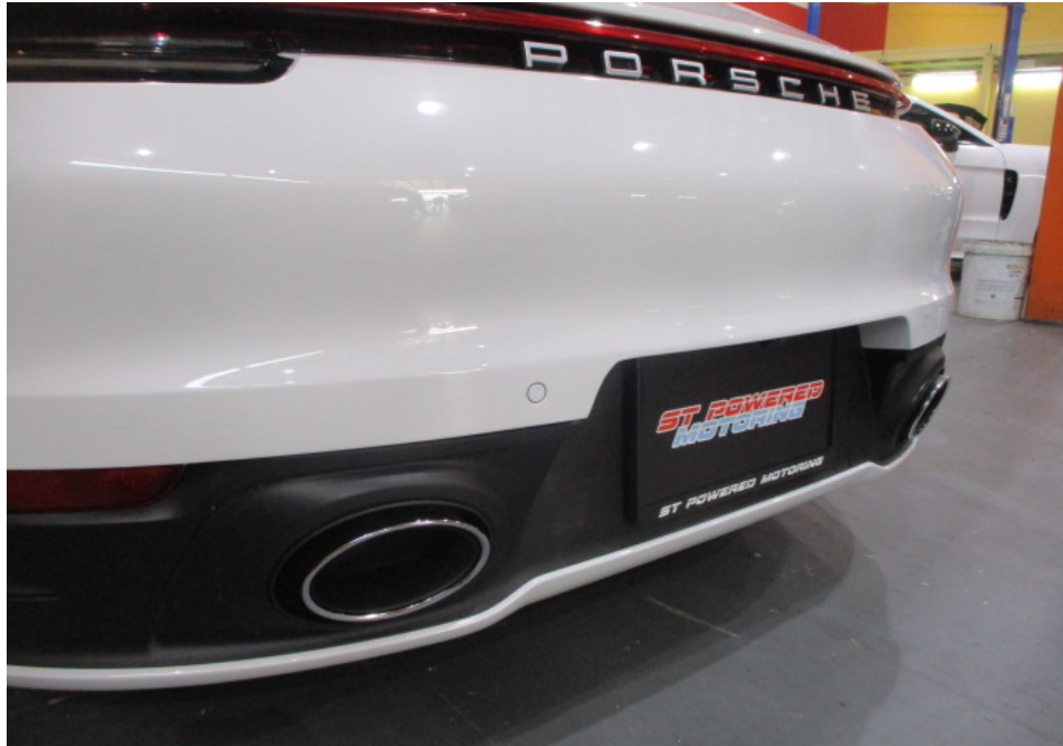
Photo 14 shows a closer view of the Motor Car's rear bumper, rear bumper lower cover and rear bumper sensors. The body parts at the rear portion of the Motor Car were visually examined and it was observed that the repair/restoration works carried out to the damaged area of the Motor Car (refer to photograph 3 & 4 above) were reasonably adequate and in order.
