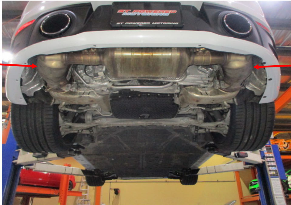
Photo 28 shows the Motor Car's exhaust system. My examination of the Motor Car's exhaust system revealed no sign(s) or indication(s) of any cut or weld marks along its exhaust pipes, on its catalytic converters (arrowed) and on its rear muffler.
