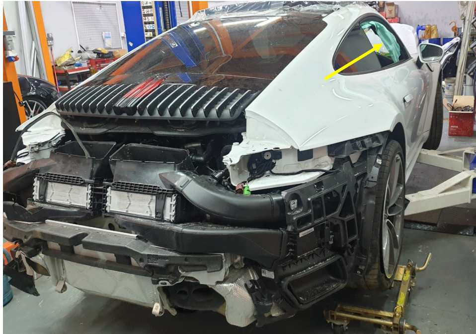
Photo 3 shows the rear right body of the Motor Car (photograph provided to me). Apart for the frontal portion, I had also observed several body parts at the Motor Car's rear portion to be missing/dislodged/damaged. These body parts include the rear bumper and all its related parts and attachments, rear taillamps, rear top cover and rear centre lamp amongst others. The right curtain airbag (arrowed) was deployed.
