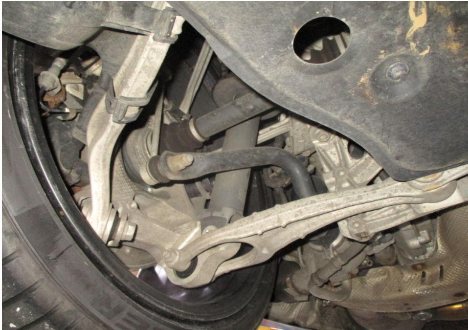
Photo 24 shows a general view of the control arms and linkages at the rear right wheel of the Motor Car. I did not observe any fluid leak and/or fluid stain on the underside of the Motor Car. All of the Motor Car's undercarriage components were observed to be intact and secured in an appropriate manner.
