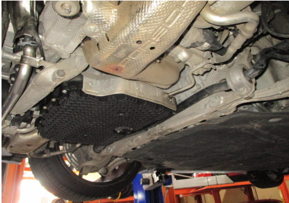
Photo 30 shows another view of the Motor Car's engine compartment. The engine compartment was at the rear underside of the Motor Car. The various parts and components inside the engine compartment were all observed to be intact and properly fitted. There was also no sign(s) or indication(s) of fluid leak and/or fluid stain found inside the engine compartment.
