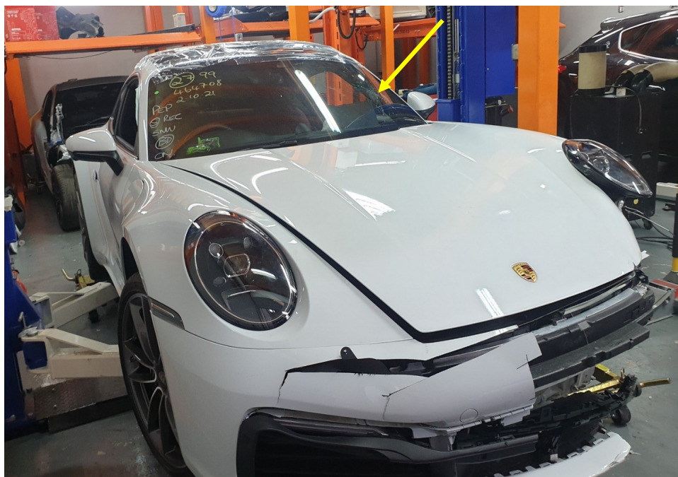
Photo 2 shows the front right body of the Motor Car (photograph provided to me). The photographs provided to me had showed damage to the frontal portion of the Motor Car. The front bumper, front bumper centre lower grille, front bumper sensors, front bonnet and front windscreen (arrowed) were amongst the body parts that were observed to have been damaged.
