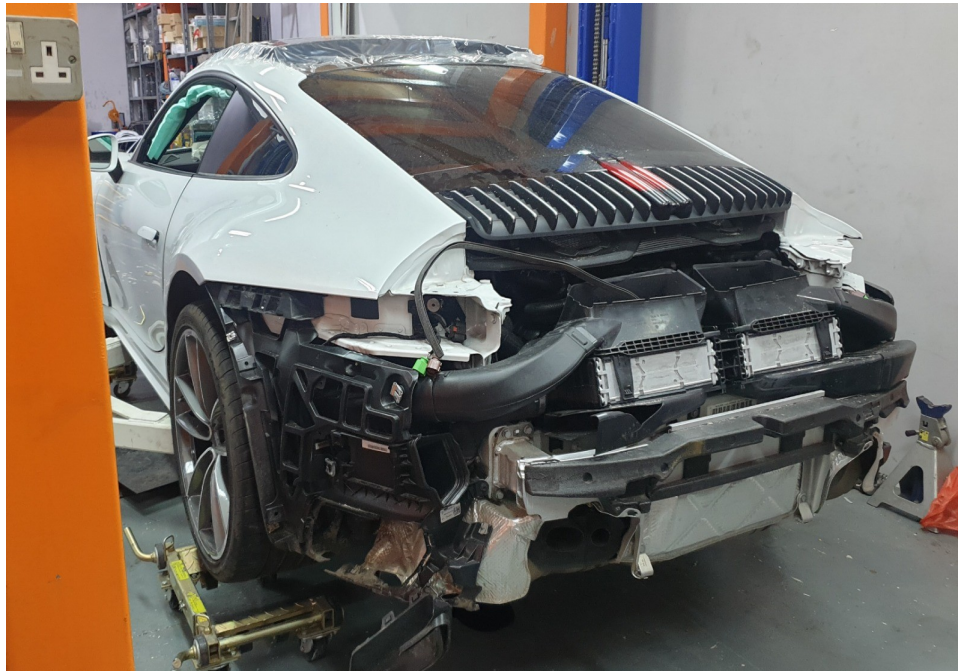
Photo 4 shows the rear left body of the Motor Car (photograph provided to me). Apart for the frontal portion, I had also observed several body parts at the Motor Car's rear portion to be missing/dislodged/damaged. These body parts include the rear bumper and all its related parts and attachments, rear taillamps, rear top cover and rear centre lamp amongst others.
