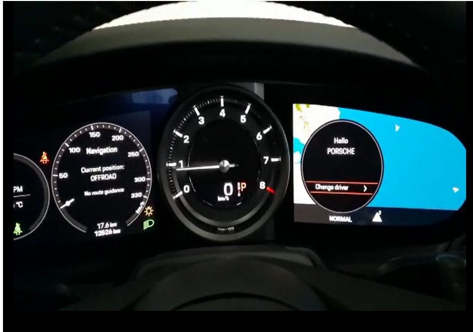
Photo 22 shows the respective warning lights no longer illuminated, indicating that there is no fault detected to the ABS, SRS, EPS, TPM and TCS systems of the Motor Car during the self-test. These electronic systems were hence in working condition at the time of my inspection.
