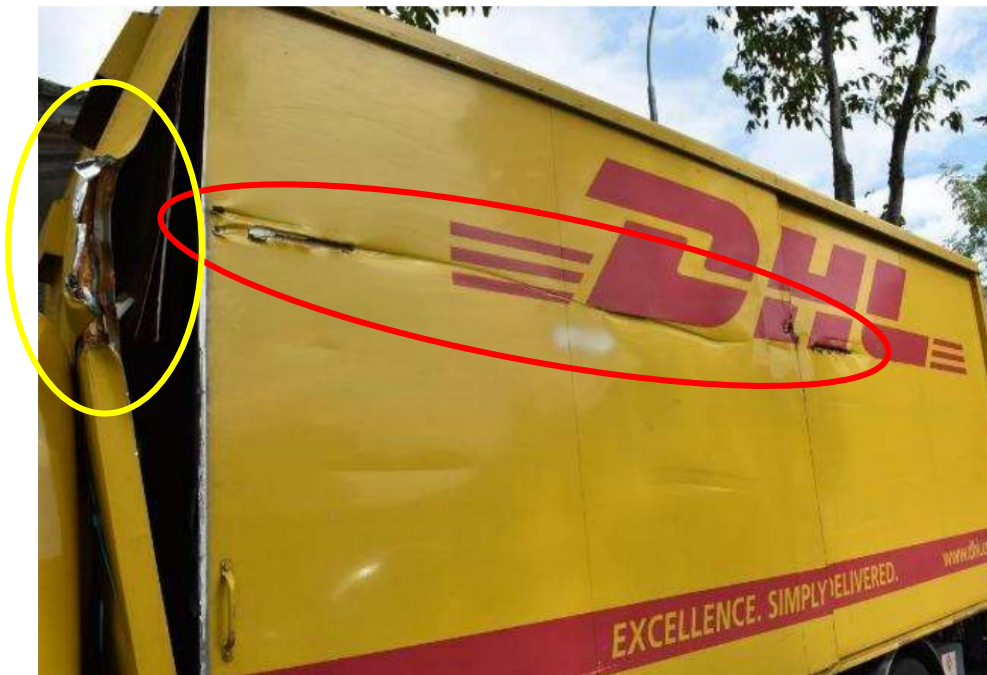
Photo 2 shows a closer view of the damaged cargo box, at the left centre portion of the Insured Vehicle. The cut to the cargo box was horizontally across the left sliding door and left rear panel (red circle), at a significant height above ground level. The frame (yellow circle) at the left side of the front facing panel of the cargo box was also observed to be bent towards the front of the Insured Vehicle.
