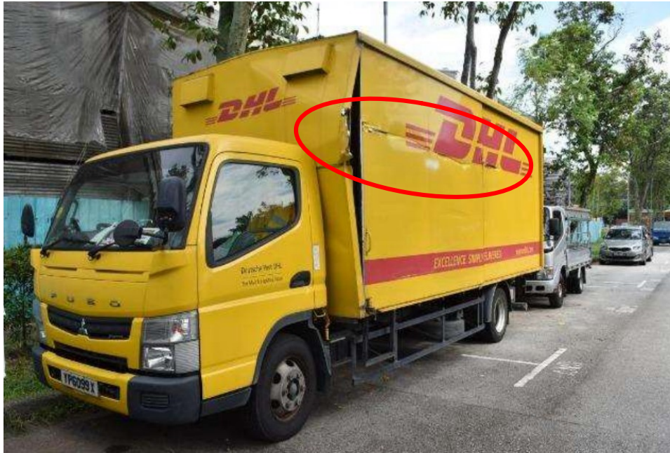
Photo 1 shows the Insured Vehicle before the start of repair. The photographs contained in the Vehicle Damage Inspection Report of the Insured Vehicle had showed damage that was confined to the left centre portion (circled) of the Insured Vehicle. The left sliding door and left rear panel of the Insured Vehicle's cargo box was observed to be horizontally cut. The frame at the left side of the front facing panel of the cargo box was also observed to be bent.
