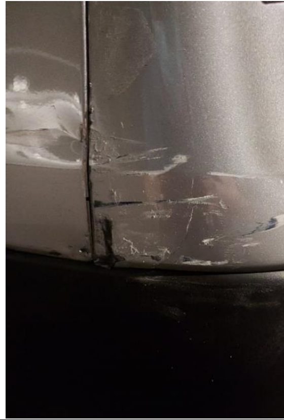
Scratches and cracked on the left rear bumper (GBH6930K) after the incident
