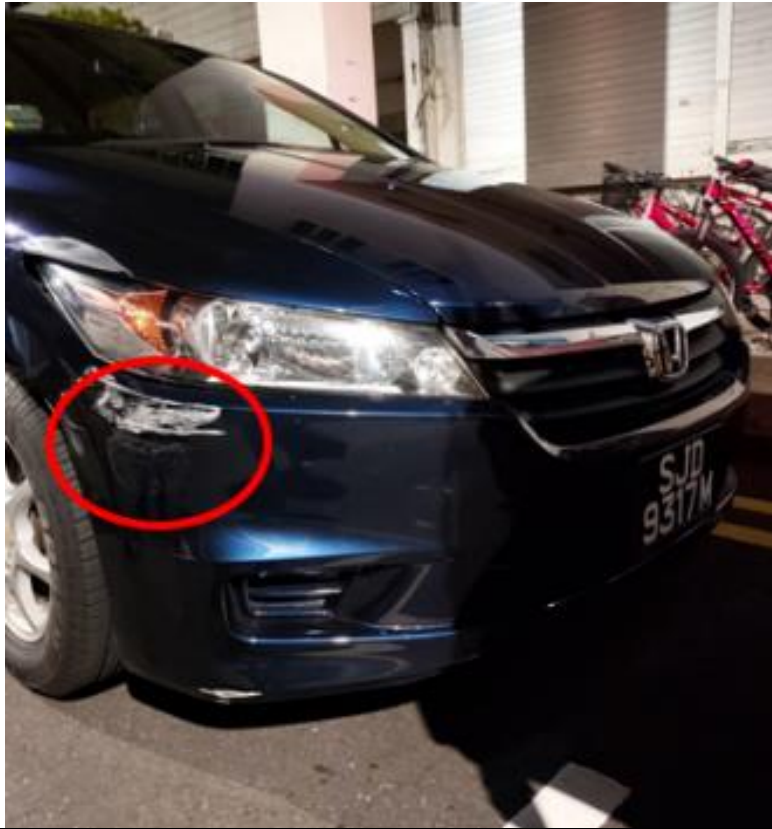
Scratches on the right front bumper of Vehicle (SJD9317M) after the incident
