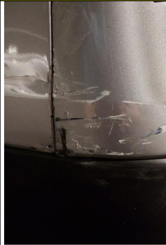
Scratches and cracked on the left rear bumper of ICA van (GBH6930K) after the incident
