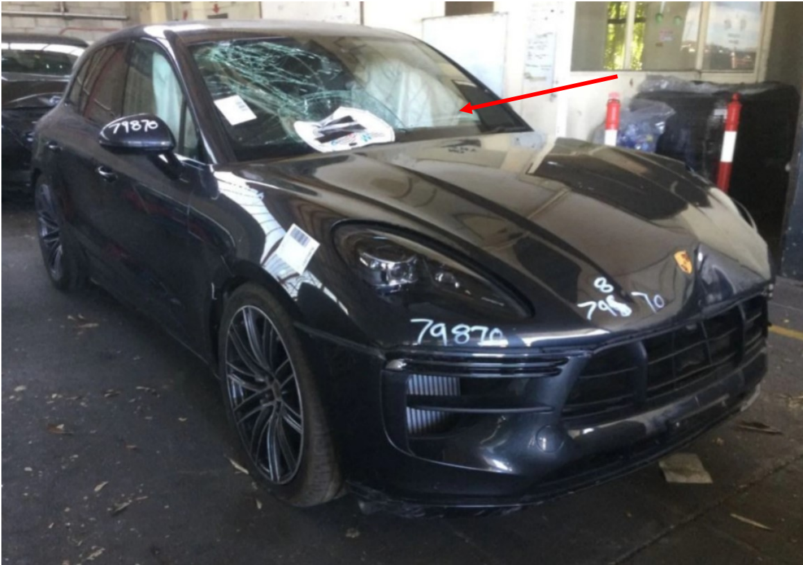
Photo 3 shows the front right body of the Motor Car (photograph provided to me). The photographs provided to me had showed damage to the front portion of the Motor Car. The front bumper, radiator grille, front bonnet and front windscreen were amongst the body parts that were observed to have been damaged. The left curtain airbag (arrowed) was deployed.
