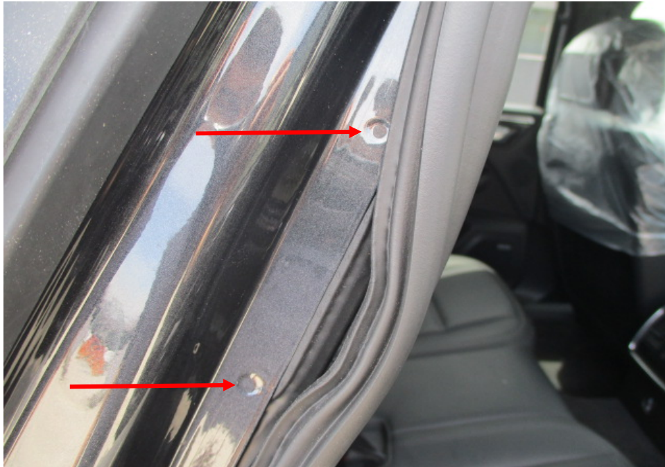
Photo 33 shows the right side "C" pillar of the Motor Car. I did not find any weld marks other than original spot weld marks (arrowed) on the right side "C" pillar of the Motor Car which, indicates that there was no re-welding works carried out. In general, I had found all the non-detachable body panels of the Motor Car to be originally fitted at the time of my inspection.
