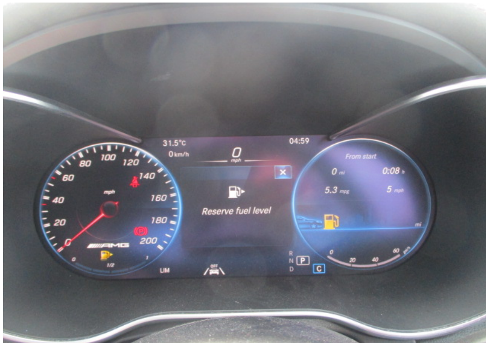
Photo 17 shows the respective warning lights no longer illuminated, indicating that there is no fault detected to the ABS, SRS, EPS, TPM and TCS systems of the Motor Car during the self-test. These electronic systems were hence in working condition at the time of my inspection.
