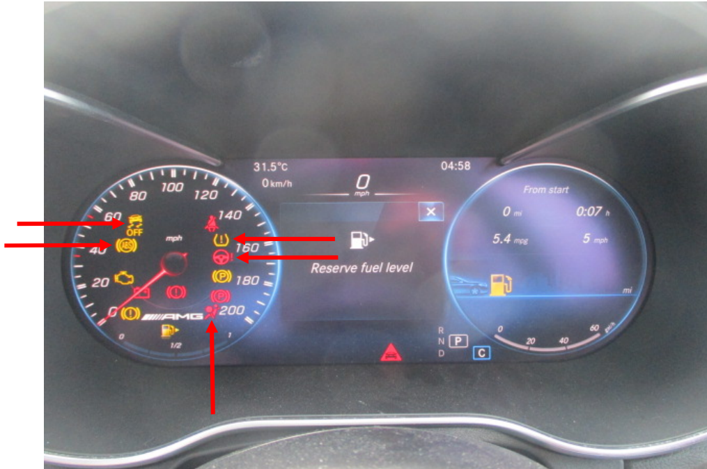
Photo 16 shows the warning lights for the various electronic safety features appearing on the instrument panel of the Motor Car during its self-test when the engine is cranked, in particular the ABS, SRS, EPS, TPM and TCS lights (arrowed).
