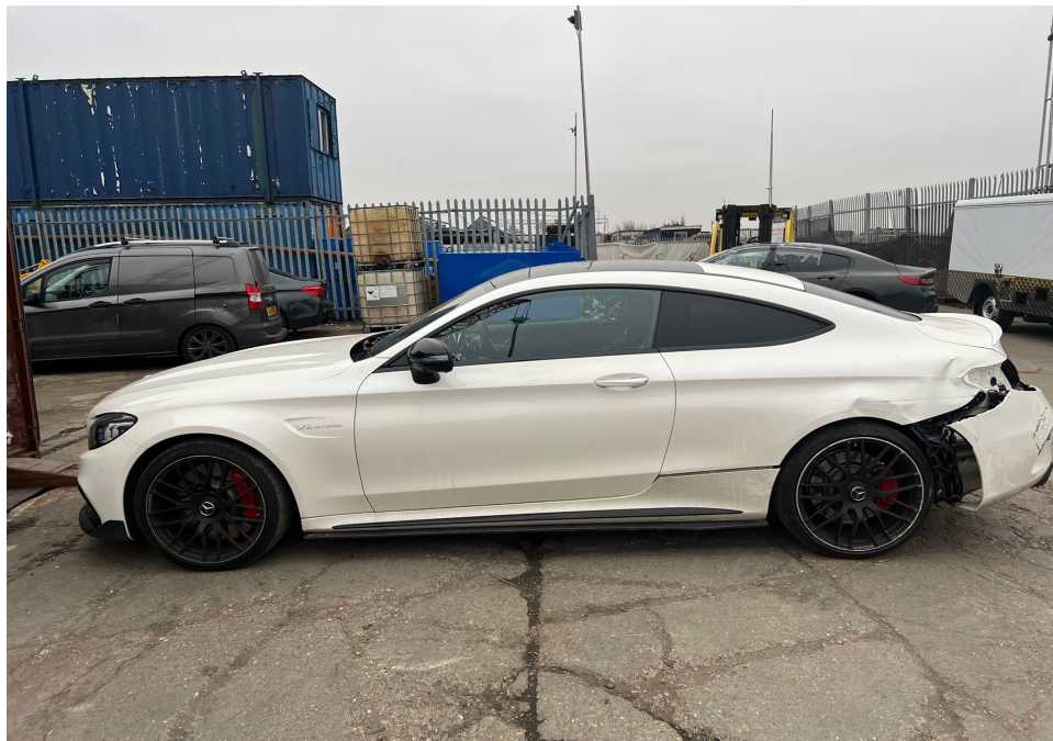
Photo 2 shows the left side body of the Motor Car (photograph provided to me). The Motor Car was observed to have sustained damage at its rear left portion. The rear bumper, rear left taillamp, rear left fender and rear left wheel rim were amongst the body parts that were observed to have been damaged. The airbag(s) was not deployed as seen from the photographs that were provided to me.
