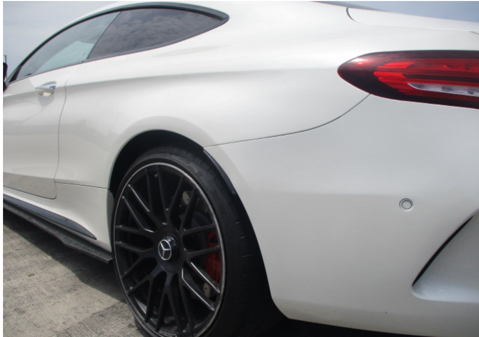
Photo 8 shows a closer view of the Motor Car's rear bumper, rear bumper left sensor, rear left taillamp, rear left fender and rear left wheel rim at the time of my inspection. The body parts at the rear left portion of the Motor Car were visually examined and it was observed that the repair/restoration works carried out to the damaged area of the Motor Car (refer to photograph 1 & 2 above) were reasonably adequate and in order.
