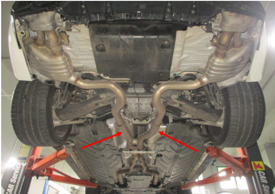
Photo 23 shows the rear section of the Motor Car's exhaust system. My examination of the Motor Car's exhaust system revealed no sign(s) or indication(s) of any cut or weld marks along its exhaust pipes (arrowed), on its rear mufflers and on its catalytic converters.
