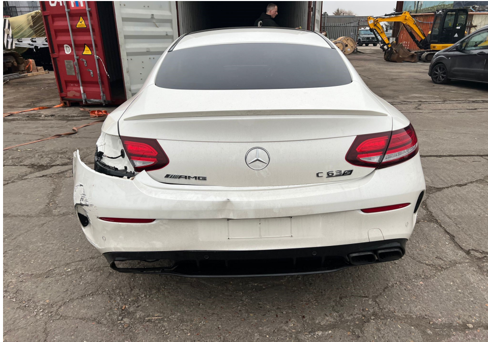
Photo 1 shows the rear body of the Motor Car (photograph provided to me). The Motor Car was observed to have sustained damage at its rear left portion. The rear bumper, rear bumper lower cover and rear left taillamp were amongst the body parts that were observed to have been damaged.
