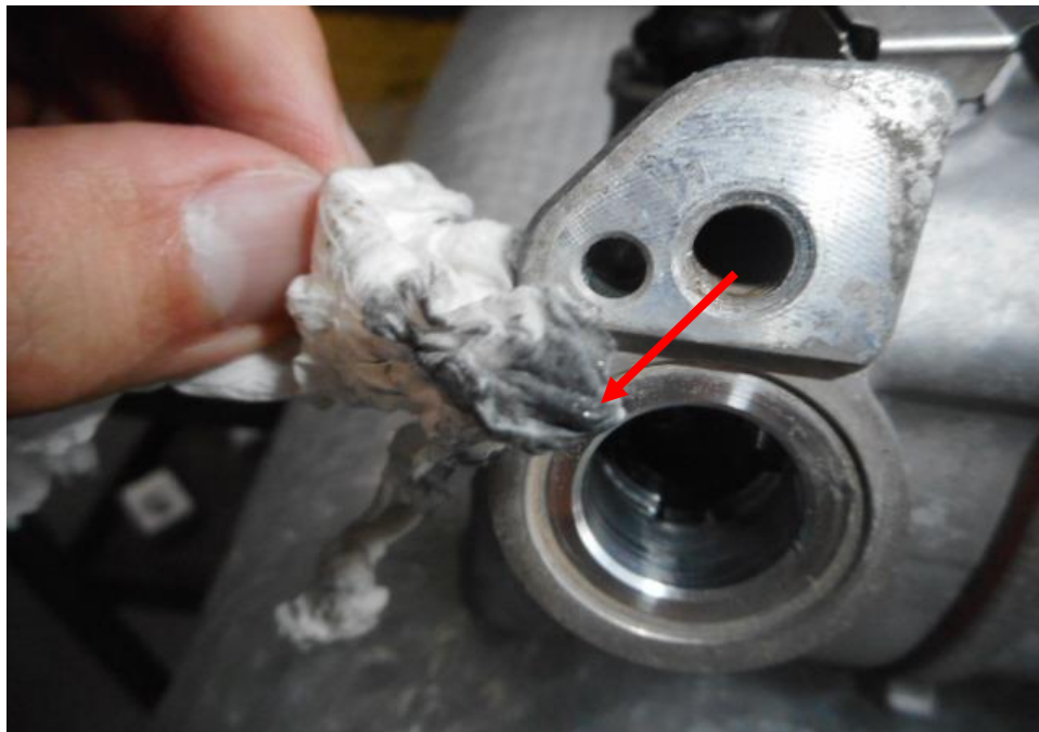
Photo 9 shows the close up view of the aircon compressor of the Insured Vehicle at the time of our inspection. The internals of the aircon compressor was observed to be filled up with black liquid and metal fillings (arrowed) which was caused by the damaged aircon compressor bearing at the time of inspection.
