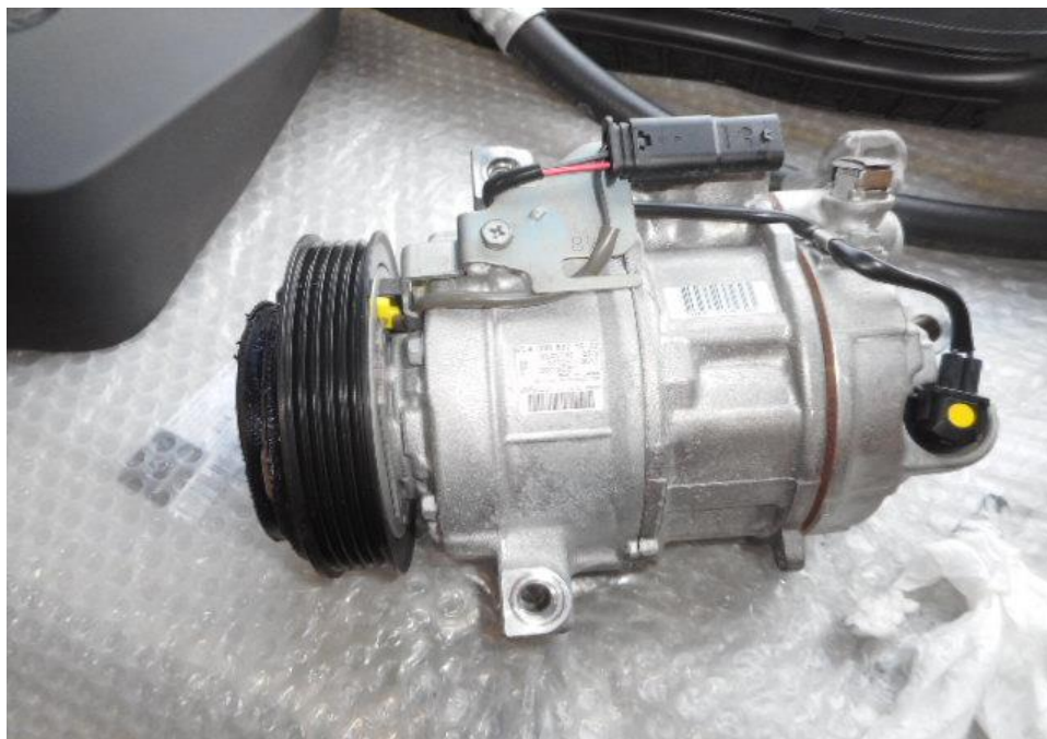
Photo 6 shows the aircon compressor unit of the Insured Vehicle at the time of our inspection. The aircon compressor unit is observed to be taken out of the Insured Vehicle and inspected.
