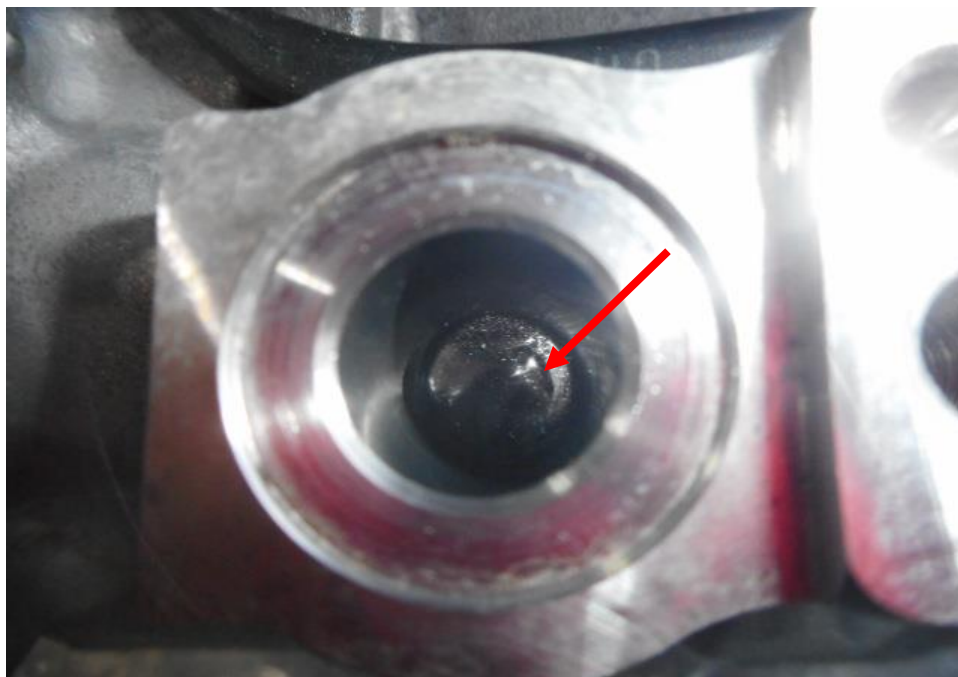
Photo 8 shows the close up view of the aircon compressor of the Insured Vehicle at the time of our inspection. The internals of the aircon compressor was observed to be filled up with black liquid and metal fillings (arrowed) which was caused by the damaged aircon compressor bearing at the time of inspection.
