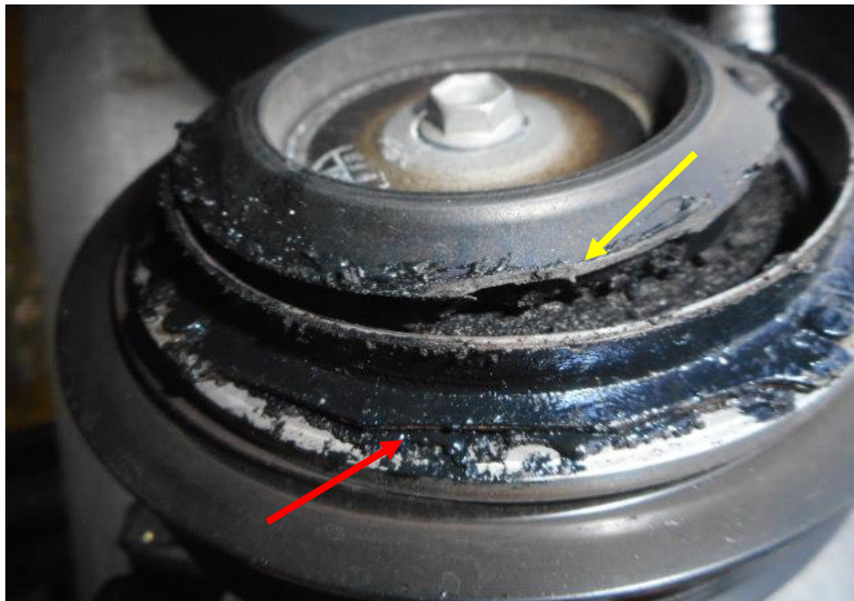
Photo 7 shows the aircon compressor unit portion of the Insured Vehicle at the time of our inspection. The bearing (yellow arrow) of the aircon compressor unit is observed to be damaged and the grease (red arrow) inside it has leaked out.
