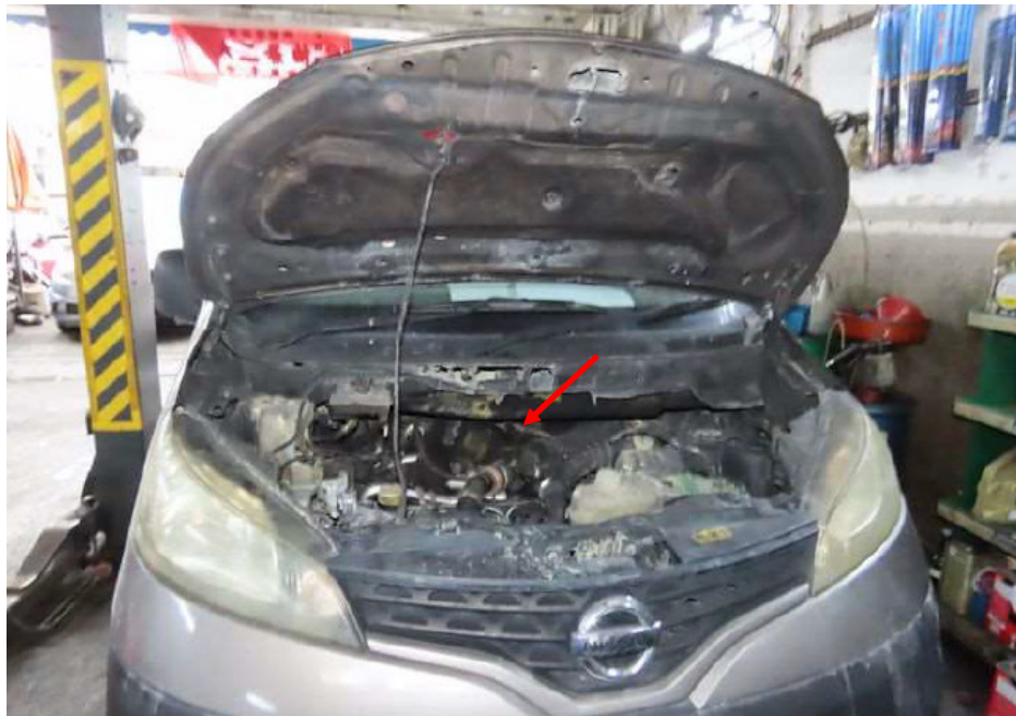
Photo 22 shows the engine compartment of the Insured Vehicle at HSL post-incident. In general, the information that could be gathered from this photograph had corresponded to the events that were related to us by Mr Yee, which is the fire to the Insured Vehicle had started from the engine compartment (arrowed).
