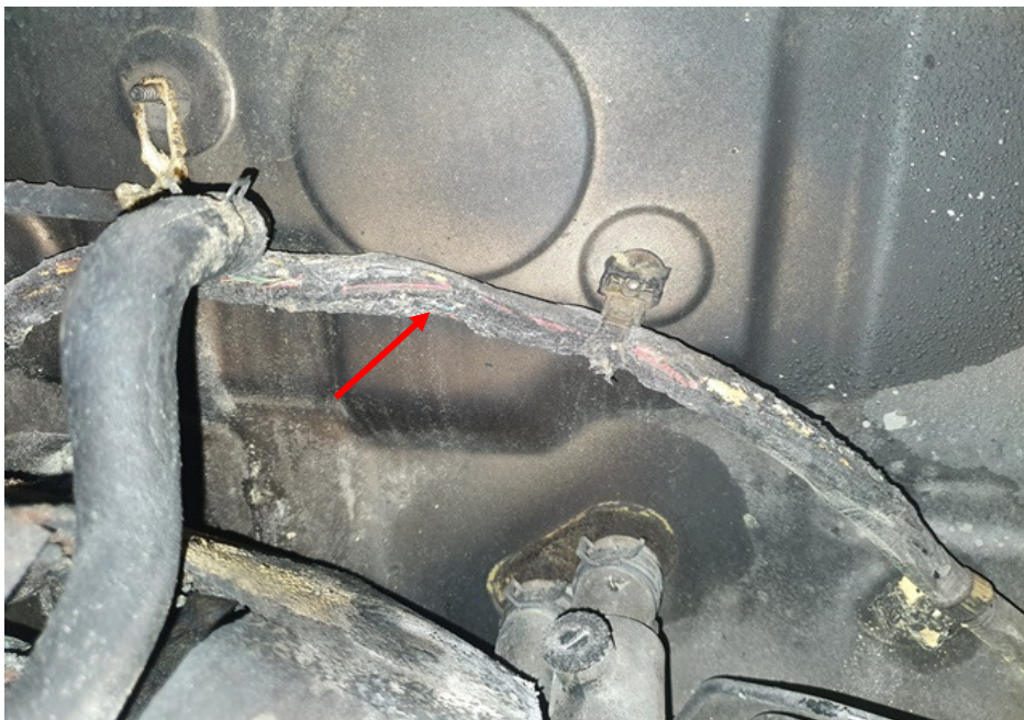
Photo 12 shows a closer view of the wirings around the centre rear portion of the engine compartment which is near to the vicinity where the fire to the Insured Vehicle had likely started. We observed greenish residue on the wirings (arrowed) at the centre rear portion of the engine compartment.
