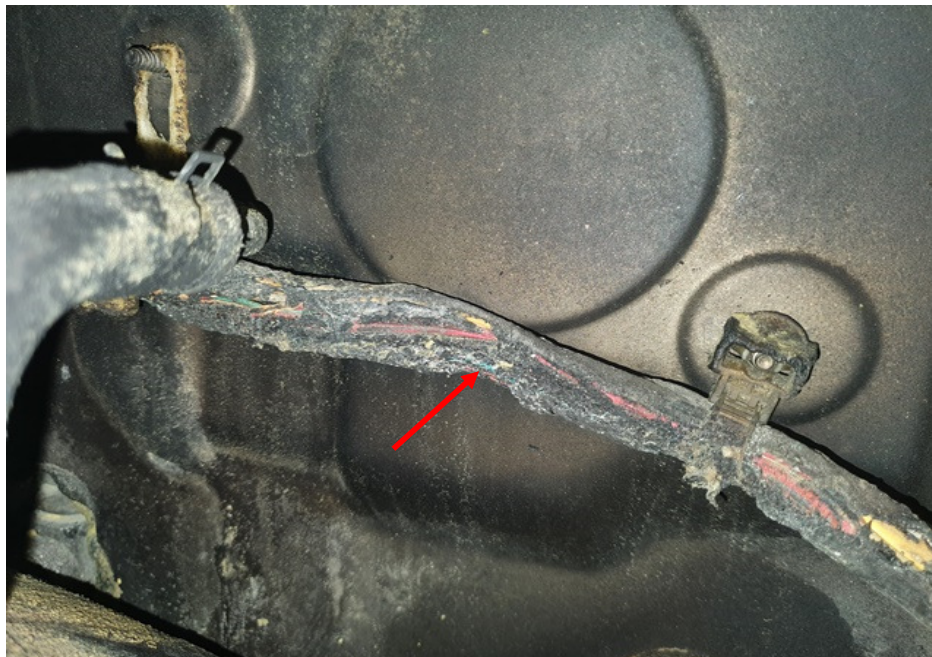
Photo 13 shows a close up view of the wirings around the centre rear portion of the engine compartment which is near to the vicinity where the fire to the Insured Vehicle had likely started. We observed greenish residue on the wirings (arrowed) at the centre rear portion of the engine compartment.
