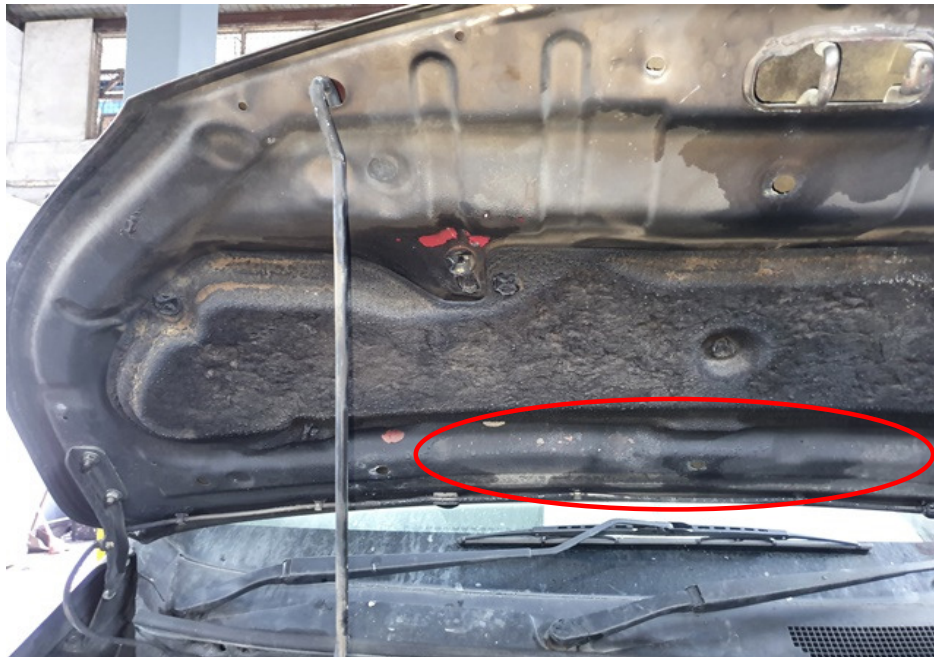
Photo 8 shows the rust that had developed on the underside of the front bonnet, around the rear centre portion (circled). The development of rust is an indication that this area was subjected to prolonged exposure to high heat intensity, which had caused the steel/metal material of the front bonnet to be exposed to natural environmental condition. Hence the fire to the Insured Vehicle can be determined to have originated towards the centre rear portion of the engine compartment.
