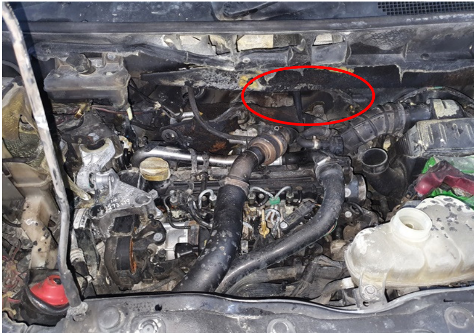
Photo 9 shows the burnt stretches of original factory fitted wirings near the firewall, which is in the immediate vicinity where the fire to the Insured Vehicle had likely started. Faint traces of greenish residue were found on some of the wirings (circled). The presence of such greenish residue suggests occurrence of an electrical short circuit.
