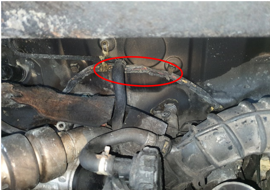
Photo 11 shows a close up view of the burnt stretches of original factory fitted wirings near the firewall, which is in the immediate vicinity where the fire to the Insured Vehicle had likely started. Faint traces of greenish residue were found on some of the wirings (circled).
