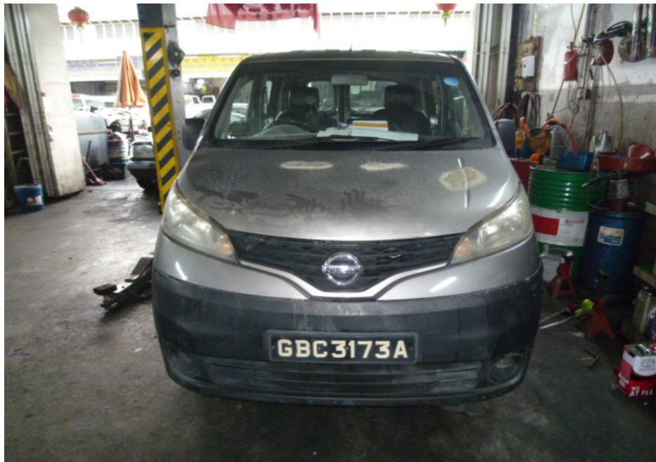
Photo 1 shows the general view of the front portion of the Insured Vehicle at the time of our inspection. The fire damage to the Insured Vehicle was confined to its frontal portion. Its front bonnet and front windscreen were amongst the body parts that were found to have been affected as a result of the fire.
