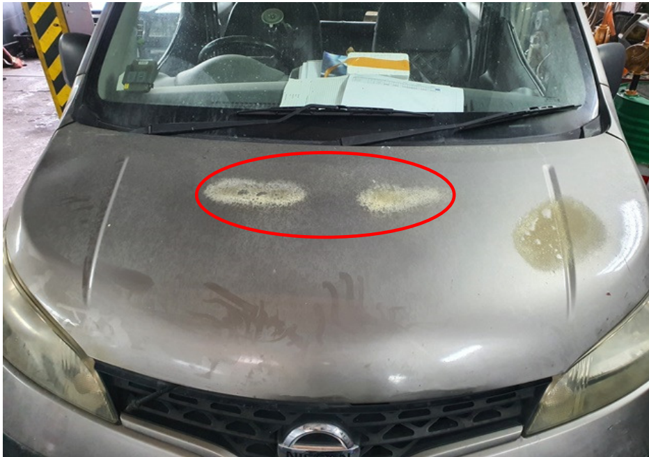
Photo 7 shows the burn pattern and whitish burn marks (circled) that were found on the rear centre portion of the front bonnet of the Insured Vehicle. Such whitish burn marks are a result of exposure to prolonged heat intensity, which may indicate where the fire had started. Rust would also begin to develop on these areas soon after the fire.
