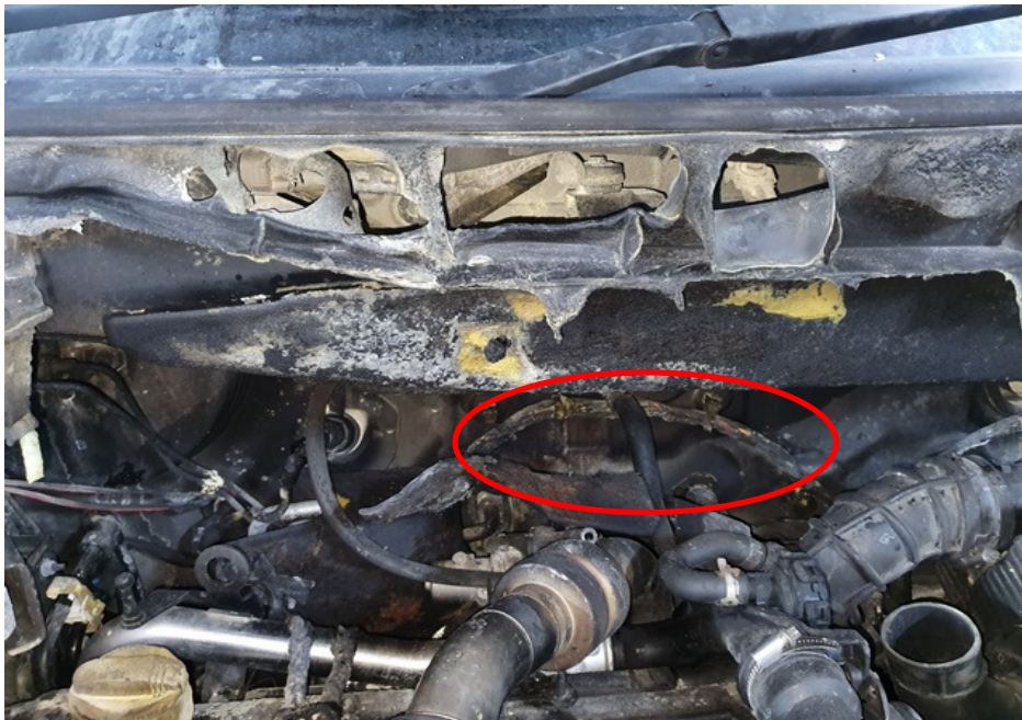
Photo 10 shows a closer view of the burnt stretches of original factory fitted wirings near the firewall, which is in the immediate vicinity where the fire to the Insured Vehicle had likely started (circled).
