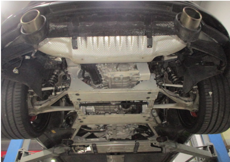
Photo 27 shows the Motor Car's exhaust system after dismantling of the rear undercovers. In general, my examination of the Motor Car's exhaust system revealed no sign(s) or indication(s) of any cut or weld marks along its exhaust pipes, on its catalytic converters and on its rear muffler.
