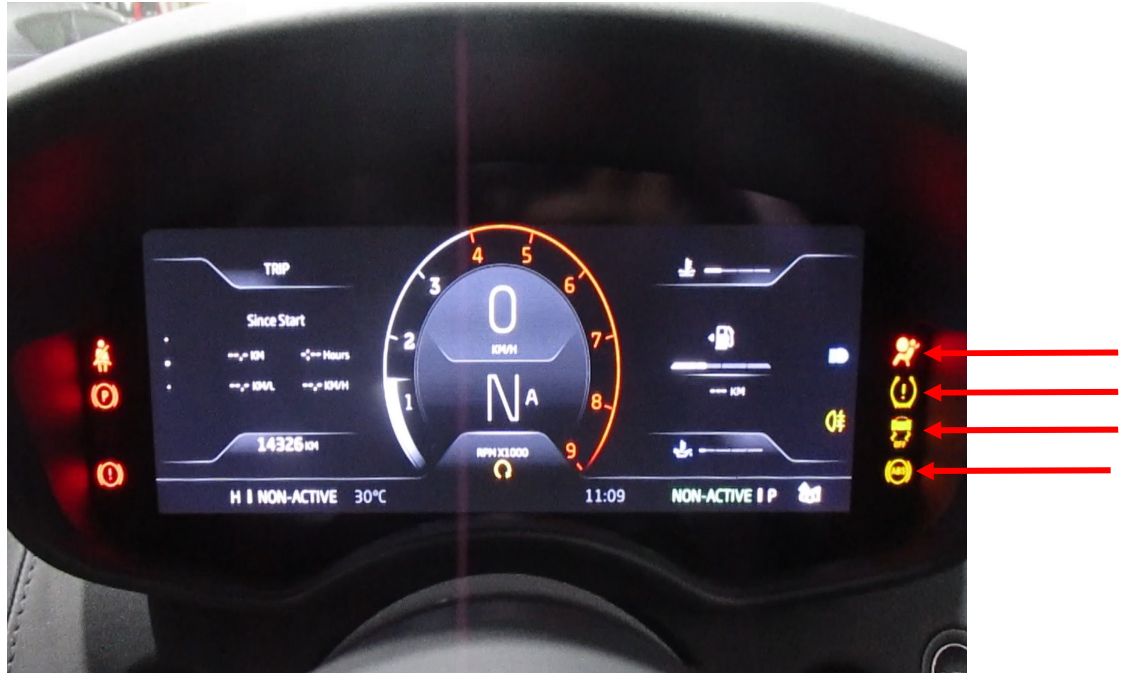
Photo 20 shows the warning lights for the various electronic safety features appearing on the instrument panel of the Motor Car during its self-test when the engine is cranked, in particular the ABS, SRS, TPM and TCS lights (arrowed).
