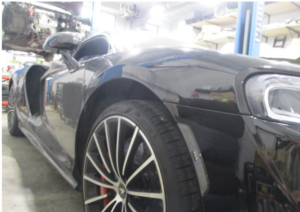
Photo 9 shows a closer view of the Motor Car's front bumper, front bumper right reflector, front right fender and front right wheel rim at the time of my inspection. The body parts at the front right portion of the Motor Car were visually examined and it was observed that the repair/restoration works carried out to the damaged area of the Motor Car (refer to photograph 1 & 2 above) were reasonably adequate and in order.
