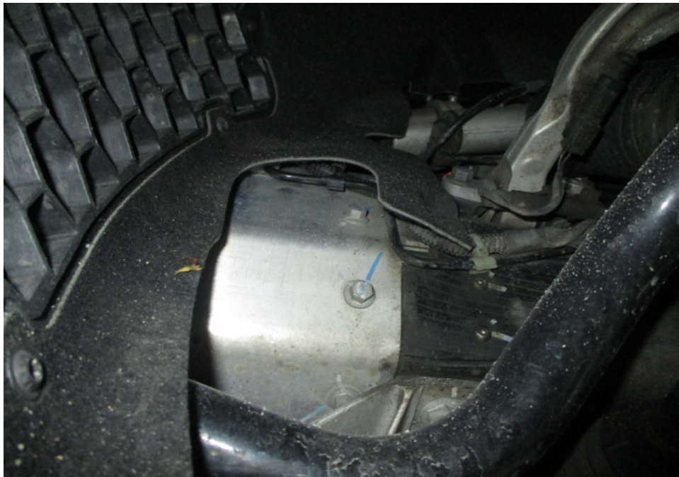
Photo 31 shows the aluminium chassis/structural body at the underside front left of the Motor Car. The original factory sealant at the joints along the chassis/structural body was observed to be untouched. In general, I had found no work was carried out on the chassis/structural body of the Motor Car. The aluminium chassis/structural body of the Motor Car was originally fitted.
