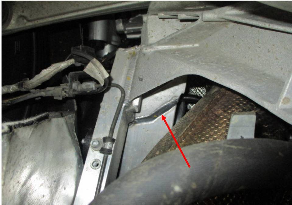
Photo 30 shows the aluminium chassis/structural body at the underside rear left of the Motor Car. I did not find any weld marks other than original spot weld marks on the chassis/structural body of the Motor Car. The original factory sealant (arrowed) at the joints along the chassis/structural body was untouched, indicating no work was done on the chassis/structural body of the Motor Car and that the chassis/structural body was originally fitted.
