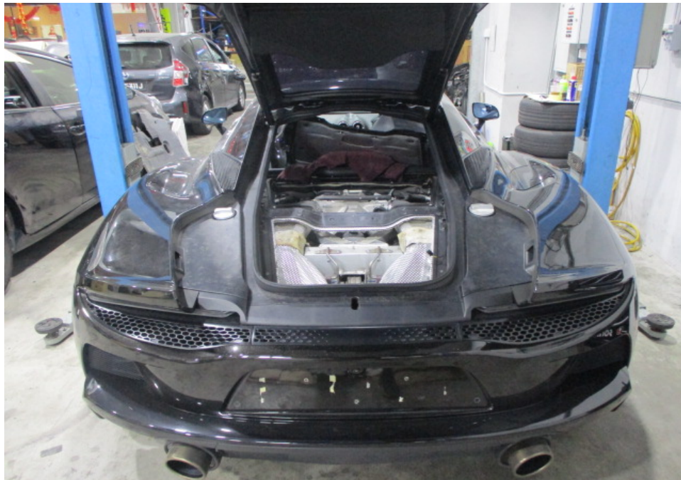
Photo 15 shows a general of the Motor Car's engine compartment at the time of my inspection. I had found the various parts and components inside the engine compartment to be intact and properly fitted. There was also no sign(s) or indication(s) of fluid leak and/or fluid stain found inside the engine compartment. Refer to photograph 16, 17 & 28 below.
