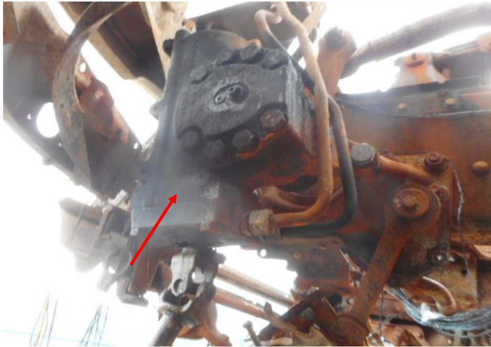
Photo 13 shows the steering box component (arrowed) at the front of the Prime Mover, it was observed to be burnt as a result of the fire.
