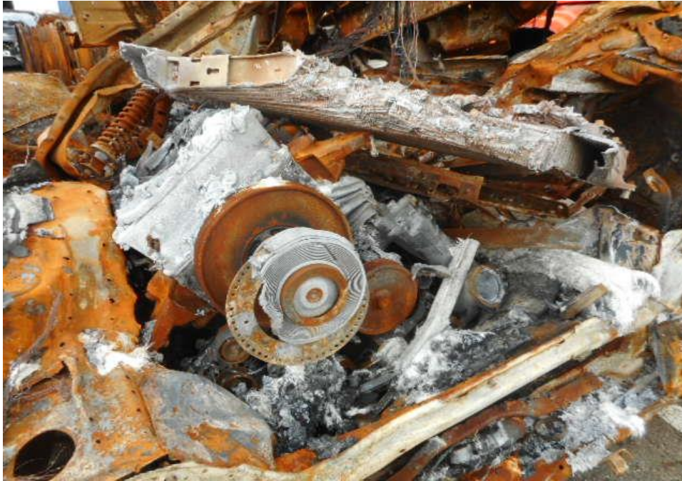
Photo 12 shows the engine compartment (arrowed) of the Prime Mover, all the engine components had been burnt as a result of the fire.
