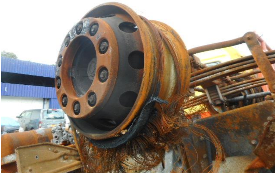
Photo 11 shows the condition of the front left tyre of the Prime Mover, which were observed to be in unserviceable condition as it was badly burnt as a result of the fire.
