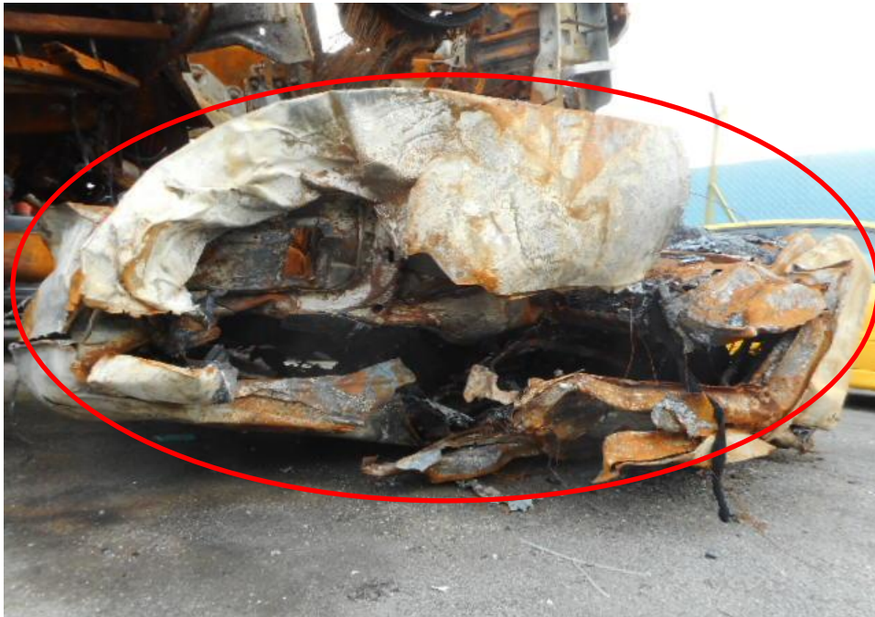
Photo 3 shows a close up view of the Prime Mover's front body at the time of my inspection. The front cabin (circled) of the Prime Mover was observed to be damaged as a result of the accident and fire.
