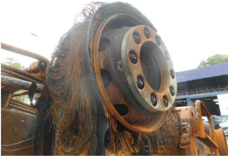
Photo 8 shows the condition of the front right tyre of the Prime Mover, which were observed to be in unserviceable condition as it was badly burnt as a result of the fire.
