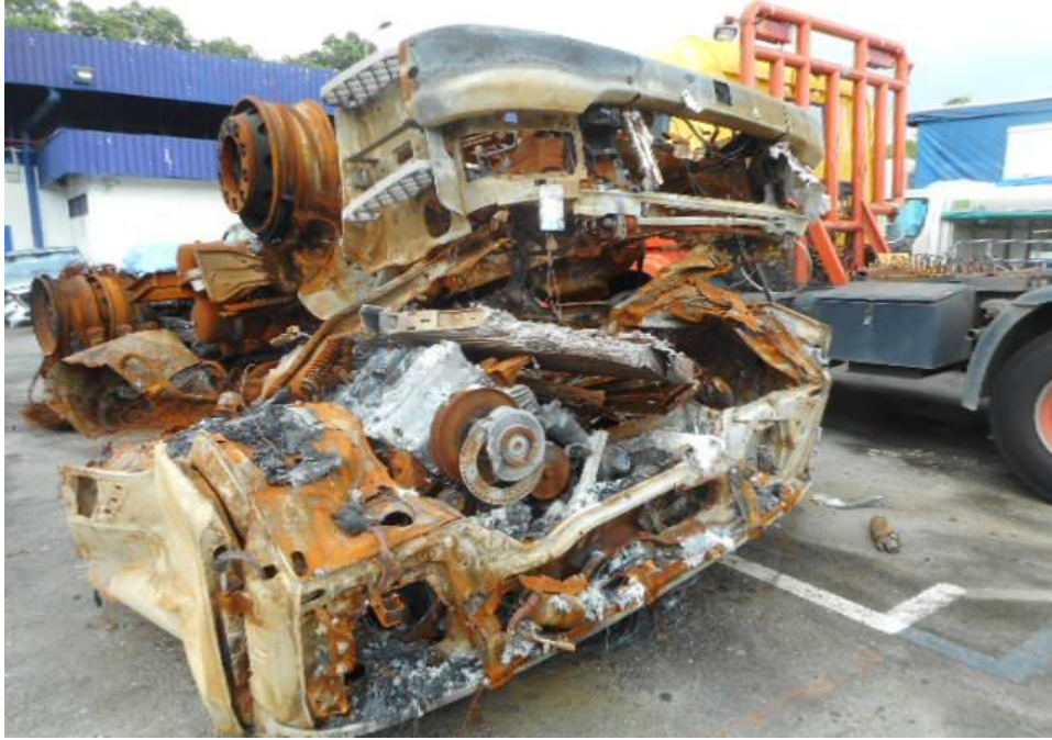
Photo 2 shows a general view of the Prime Mover's front body at the time of my inspection. The front cabin of the Prime Mover was observed to be damaged as a result of the accident and fire.
