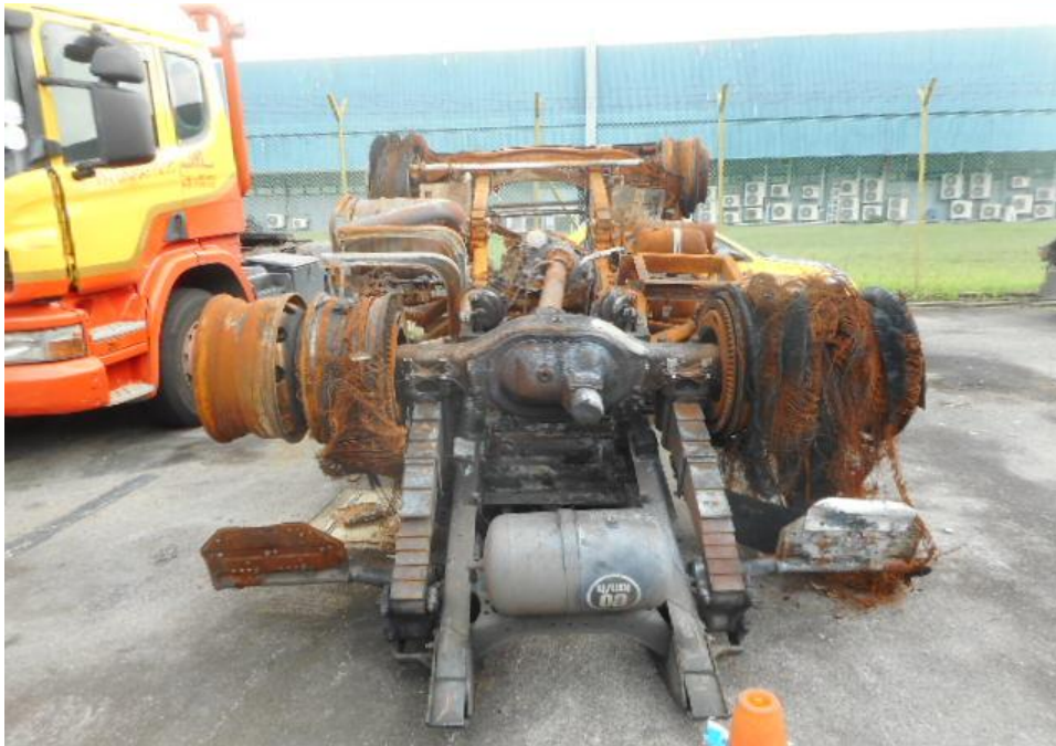
Photo 6 shows a general view of the Prime Mover's rear body at the time of my inspection. The rear portion of the Prime Mover was observed to be damaged as a result of the accident and fire.
