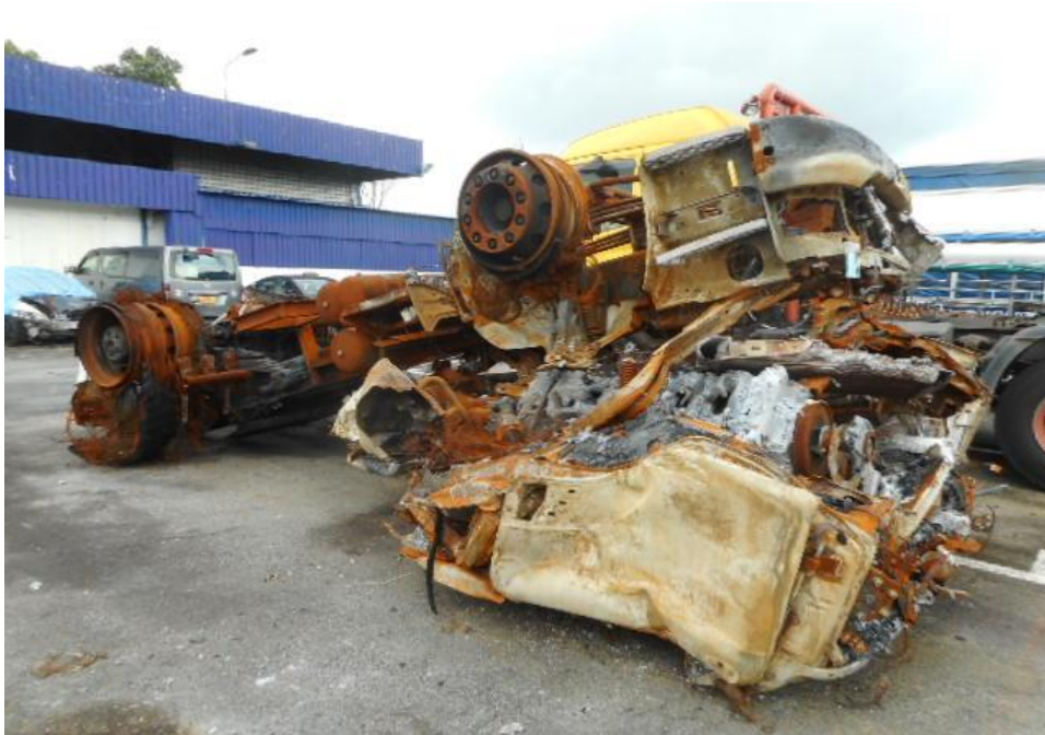
Photo 5 shows a general view of the Prime Mover's left body at the time of my inspection. The left portion of the Prime Mover was observed to be damaged as a result of the accident and fire.
