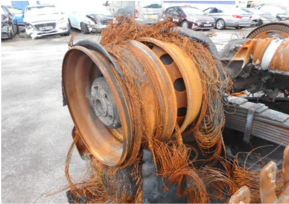
Photo 10 shows the condition of the rear left tyre of the Prime Mover, which were observed to be in unserviceable condition as it was badly burnt as a result of the fire.
