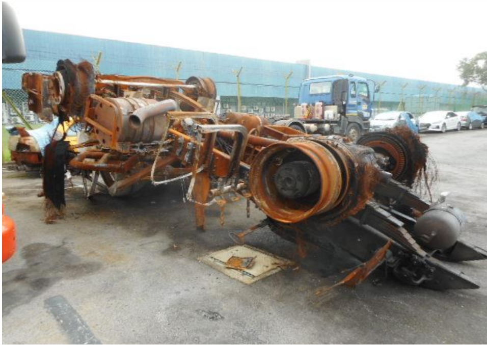
Photo 4 shows a general view of the Prime Mover's right body at the time of my inspection. The right portion of the Prime Mover was observed to be damaged as a result of the accident and fire.
