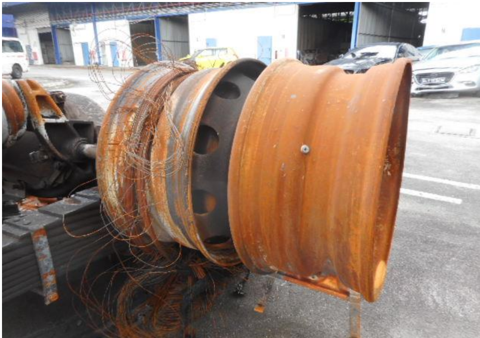
Photo 9 shows the condition of the rear right tyres of the Prime Mover, which were observed to be in unserviceable condition as it was badly burnt as a result of the fire.
