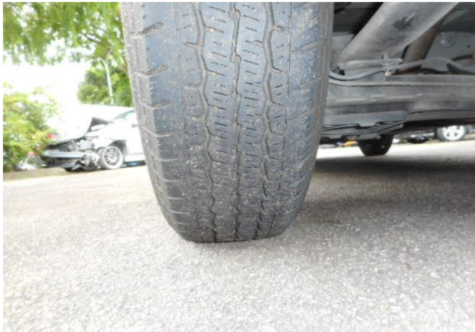
Photo 9 shows the condition of the rear left tyres of the Motor Van, which was observed to be in serviceable condition with remaining tread depth of approximately 4.4mm. The tyres, which were wrapped around standard steel wheel rim, were also observed to be sufficiently inflated for vehicular operation. There was also no damage found on all 4 steel wheel rims of the Motor Van.
