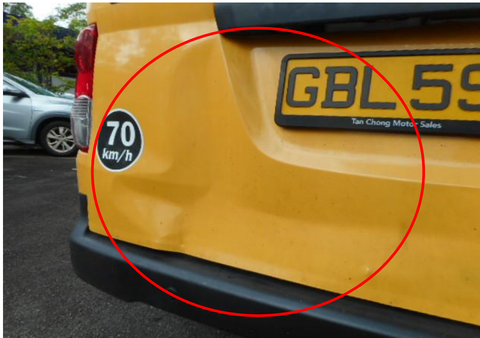
Photo 3 shows a close up view of the Motor Van's rear portion at the time of my inspection. It appeared to have sustained damage at its rear portion. Its rear body panel (circled) was damage at the time of my inspection as a result of the accident.
