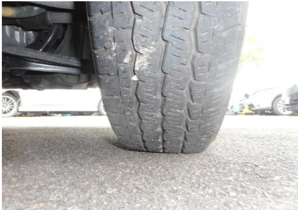
Photo 7 shows the condition of the front right tyre of the Motor Van, which was observed to be in serviceable condition with remaining tread depth of approximately 6.1mm. The tyre, which was wrapped around standard steel wheel rim, was also observed to be sufficiently inflated for vehicular operation. There was no tear, cut or burst mark(s) on the outer and the inner sidewalls as well as across the tread of the 4 tyres that were fitted on the Motor Van.
