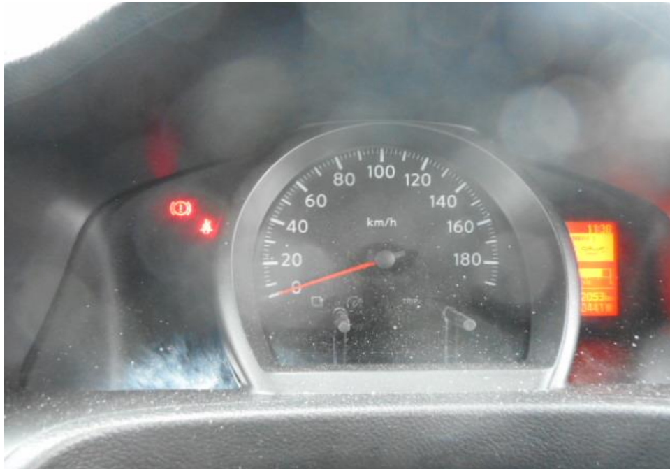
Photo 24 shows no warning lights illuminated on the instrument panel of the Motor Van after the engine was cranked. This would suggest that there was no abnormality to the electronic operating system of the Motor Van, like the ABS, EPS, SRS and etc.
