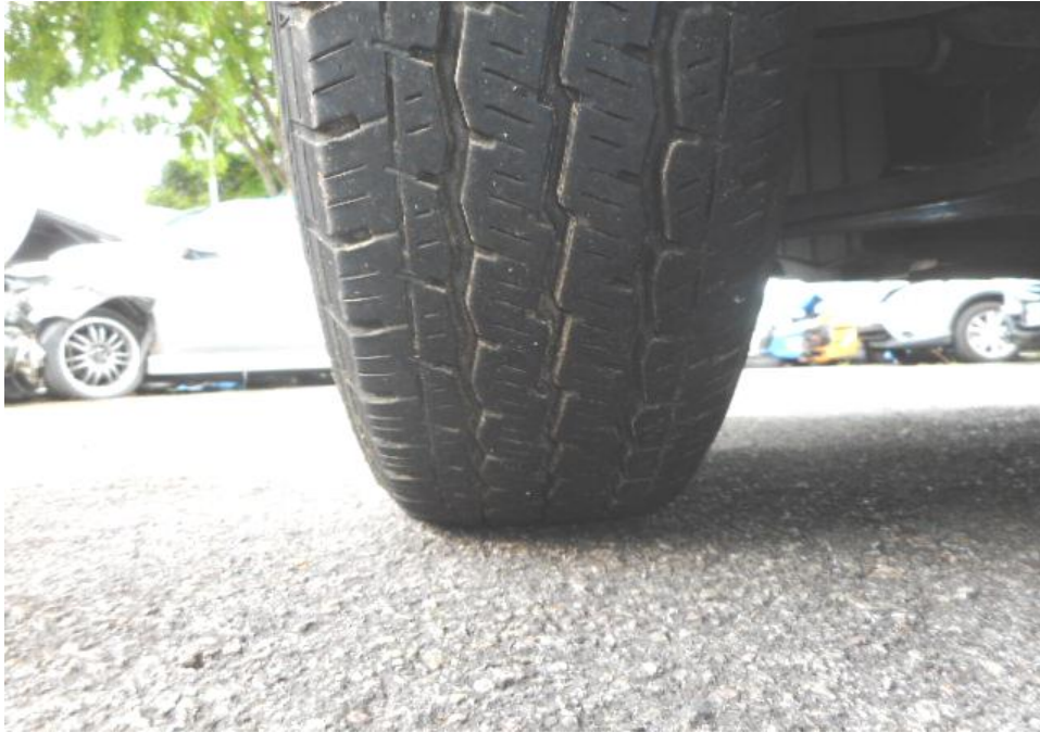
Photo 10 shows the condition of the rear right tyres of the Motor Van, which were observed to be in serviceable condition with remaining, tread depth of approximately 5.9mm. There was also no tear, cut or burst mark(s) on the outer and the inner sidewalls as well as across the tread of the 4 tyres that were fitted on the Motor Van.
