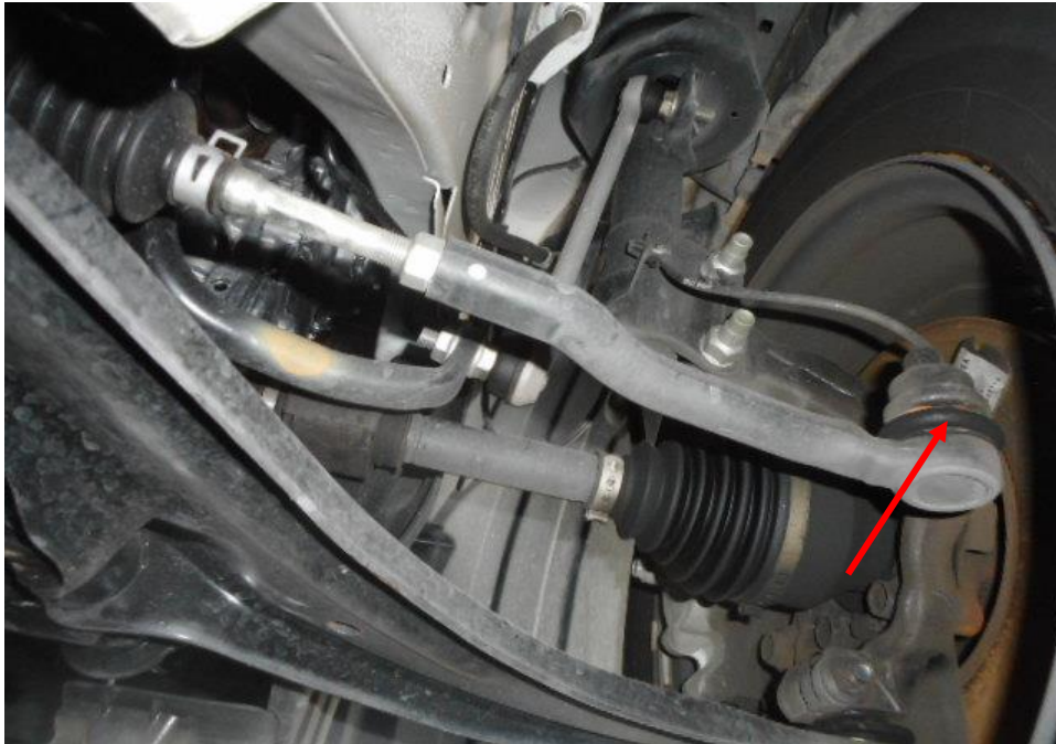
Photo 16 shows the various undercarriage components at the front right wheel of the Motor Van, in particular the steering tie rod end (arrowed). The various steering components were all found to be intact, suggesting that the steering system of the Motor Van was likely to be in serviceable condition at the material time of accident. There was also no sign of fluid stain(s) observed on the various undercarriage components.
