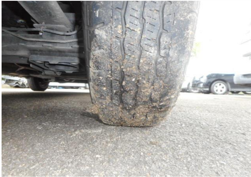
Photo 8 shows the condition of the rear right tyre of the Motor Van, which was observed to be in serviceable condition with remaining tread depth of approximately 4.9mm. The tyre, which was wrapped around standard steel wheel rim, it was observed to be sufficiently inflated for vehicular operation.
