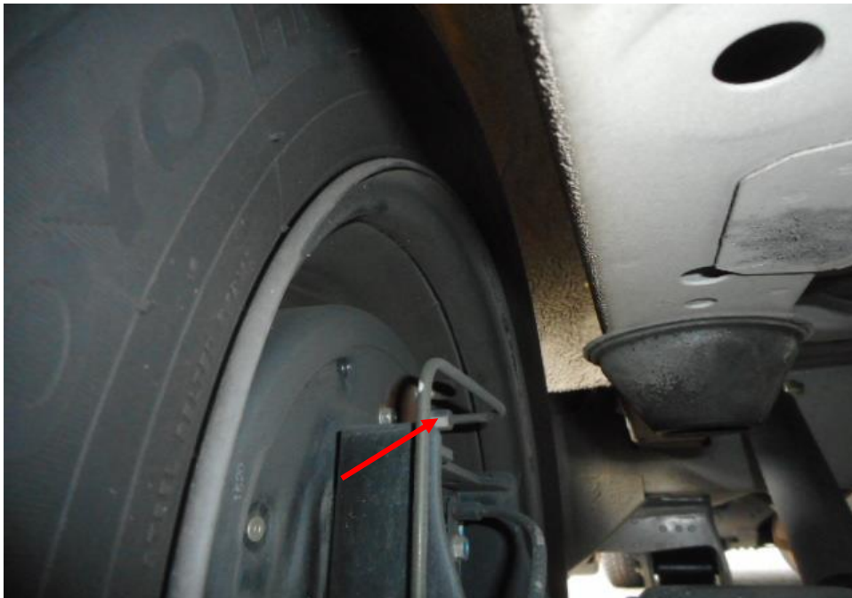
Photo 19 shows the brake pipe (arrowed) at the rear left wheel of the Motor Van. I did not observe any leakage of brake fluid at the time of my inspection of the Motor Van. My static tests of the Motor Van's braking system, along with my visual examination of the various mechanical components in the braking system had indicated that there was no internal leakage of pressure/vacuum. Hence the braking system of the Motor Van was likely to be in serviceable condition at the material time of accident.
