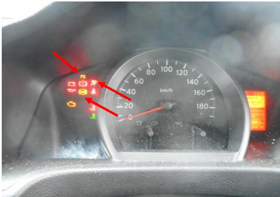
Photo 23 shows the warning light for Anti-Lock Brake System (ABS), Electrical Power Steering System (EPS) and Supplemental Restraint System (SRS) (arrowed) appearing on the instrument panel of the Motor Van during the self-test of its various electronic operating systems when its engine was cranked.
