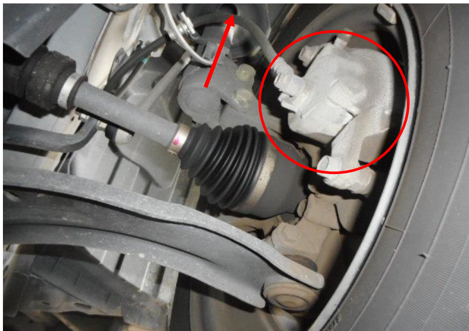
Photo 21 shows the brake hose/pipe (arrowed) at the front left wheel of the Motor Van. No leakage of brake fluid was observed. Visual examination of the various components of the braking system like the brake caliper (circled), brake booster, brake pedal etc had revealed all to be intact and without visible damage at the time of accident. There was also no sign of fluid stain(s) observed on the various undercarriage components.
