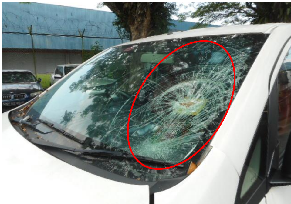
Photo 3 shows a close up view of the Motor Van's frontal portion at the time of my inspection. It appeared to have sustained damage at its frontal portion. Its front windscreen (circled) was damage at the time of my inspection as a result of the accident.
