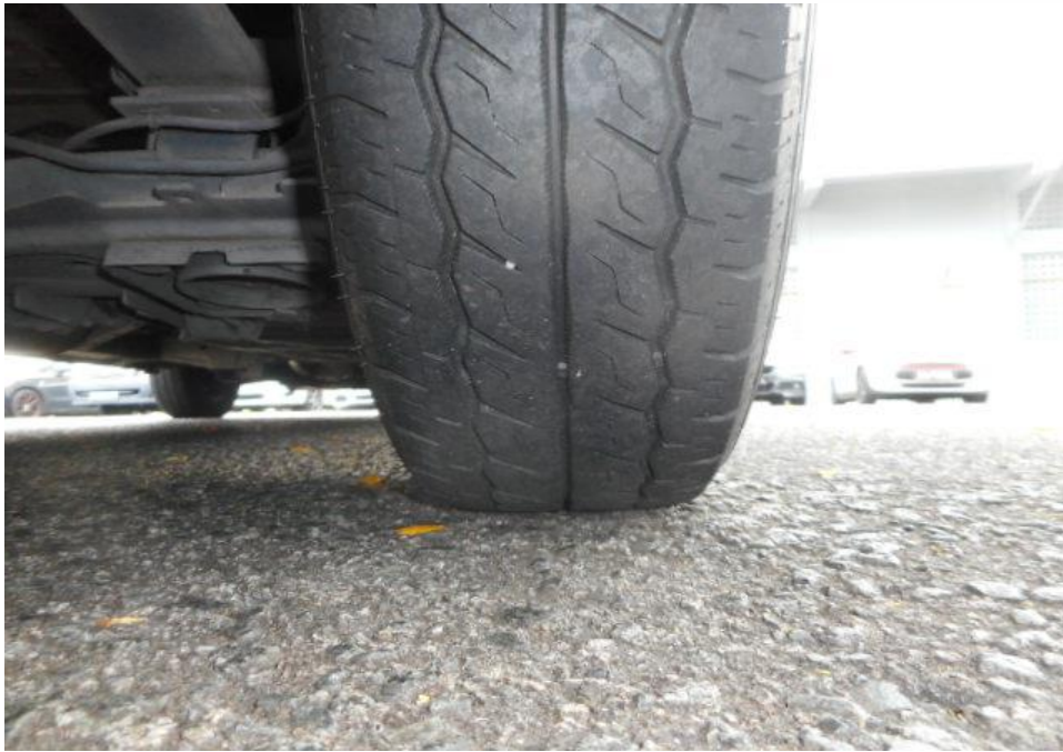
Photo 10 shows the condition of the rear right tyre of the Motor Van, which was observed to be in serviceable condition with remaining tread depth of approximately 5.2mm. The tyre, which was wrapped around standard steel wheel rim, it was observed to be sufficiently inflated for vehicular operation.
