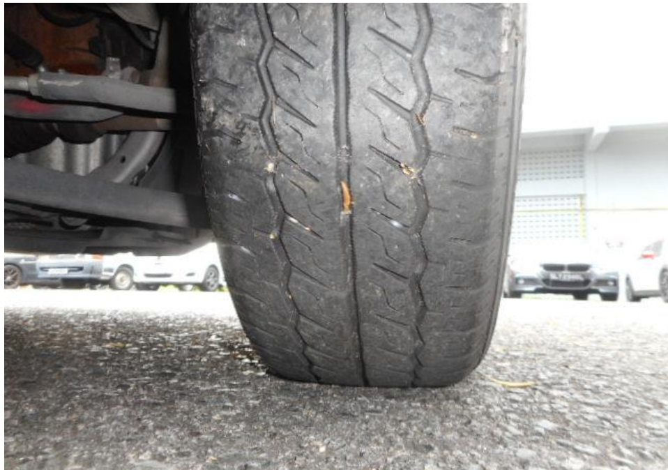
Photo 9 shows the condition of the front right tyre of the Motor Van, which was observed to be in serviceable condition with remaining tread depth of approximately 5.2mm. The tyre, which was wrapped around standard steel wheel rim, was also observed to be sufficiently inflated for vehicular operation. There was no tear, cut or burst mark(s) on the outer and the inner sidewalls as well as across the tread of the 4 tyres that were fitted on the Motor Van.
