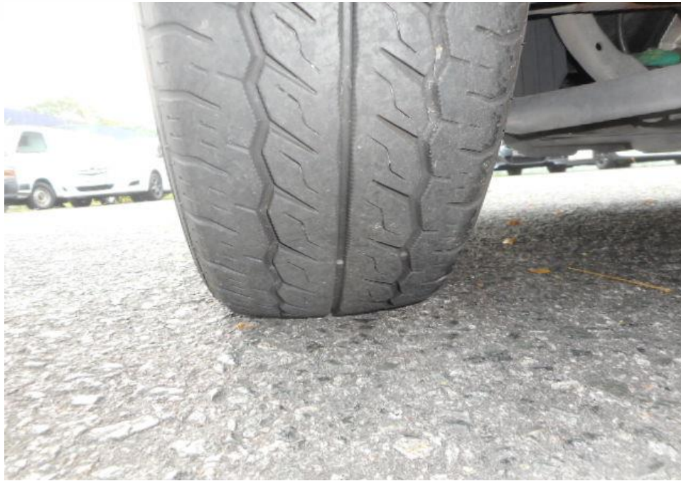
Photo 12 shows the condition of the rear right tyres of the Motor Van, which were observed to be in serviceable condition with remaining, tread depth of approximately 5.2mm. There was also no tear, cut or burst mark(s) on the outer and the inner sidewalls as well as across the tread of the 4 tyres that were fitted on the Motor Van.
