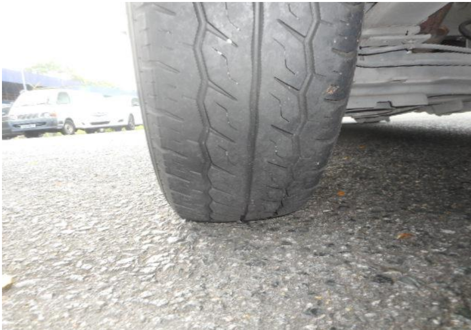
Photo 11 shows the condition of the rear left tyres of the Motor Van, which was observed to be in serviceable condition with remaining tread depth of approximately 5mm. The tyres, which were wrapped around standard steel wheel rim, were also observed to be sufficiently inflated for vehicular operation. There was also no damage found on all 4 steel wheel rims of the Motor Van.
