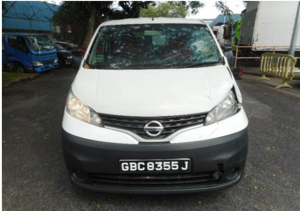
Photo 2 shows a general view of the Motor Van's frontal portion at the time of my inspection. It appeared to have sustained damage at its frontal portion. Its front windscreen, front bonnet, front left headlamp and front bumper were damage at the time of my inspection.
