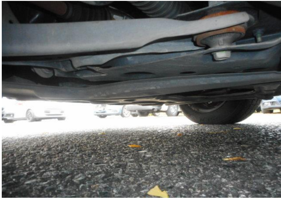
Photo 17 shows the undercarriage of the Motor Van, at the area where the engine housing and transmission housing are located. . I did not find any sign(s) or indication(s) of fluid leak and/or fluid stain(s) on the underside of the Motor Van.
