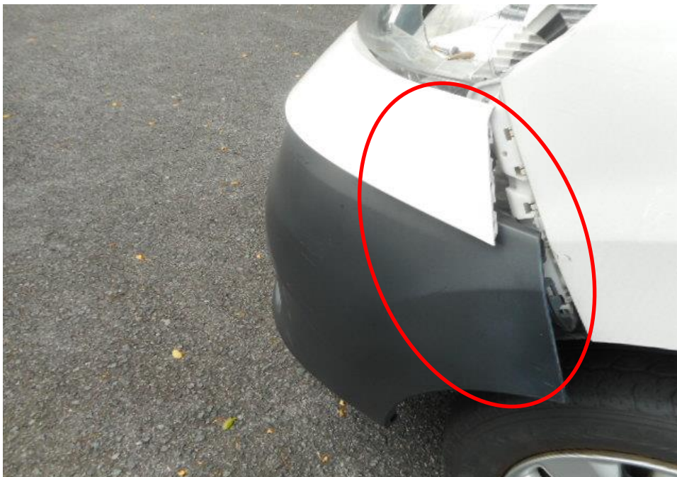
Photo 5 shows a close up view of the Motor Van's frontal portion at the time of my inspection. It appeared to have sustained damage at its frontal portion. Its front bumper (circled) was damage at the time of my inspection as a result of the accident.
