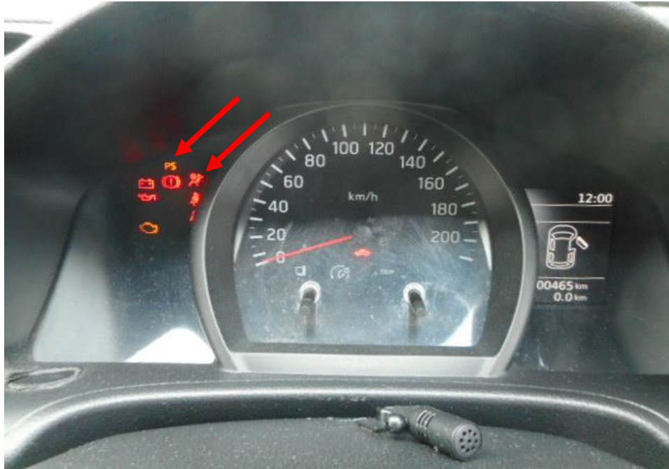
Photo 25 shows the warning light for Electric Power Steering System (EPS) and Supplemental Restraint System (SRS) (arrowed) appearing on the instrument panel of the Motor Van during the self-test of its various electronic operating systems when its engine was cranked.
