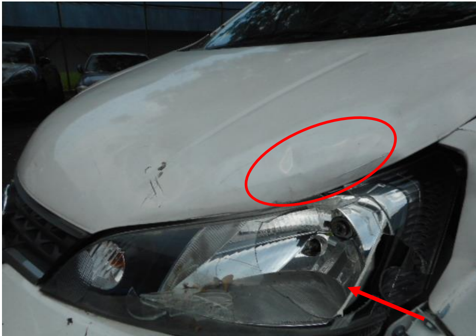
Photo 4 shows a close up view of the Motor Van's frontal portion at the time of my inspection. It appeared to have sustained damage at its frontal portion. Its front bonnet (circled) and front left headlamp (arrowed) was damage at the time of my inspection as a result of the accident.
