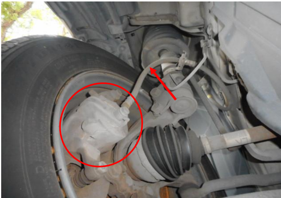
Photo 23 shows the brake hose/pipe (arrowed) at the front left wheel of the Motor Van. No leakage of brake fluid was observed. Visual examination of the various components of the braking system like the brake caliper (circled), brake booster, brake pedal etc had revealed all to be intact and without visible damage at the time of accident. There was also no sign of fluid stain(s) observed on the various undercarriage components.
