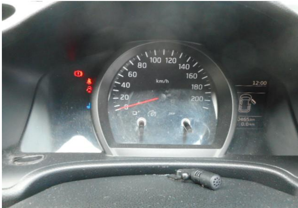
Photo 26 shows no warning lights illuminated on the instrument panel of the Motor Van after the engine was cranked. This would suggest that there was no abnormality to the electronic operating system of the Motor Van, like the EPS, SRS and etc.
