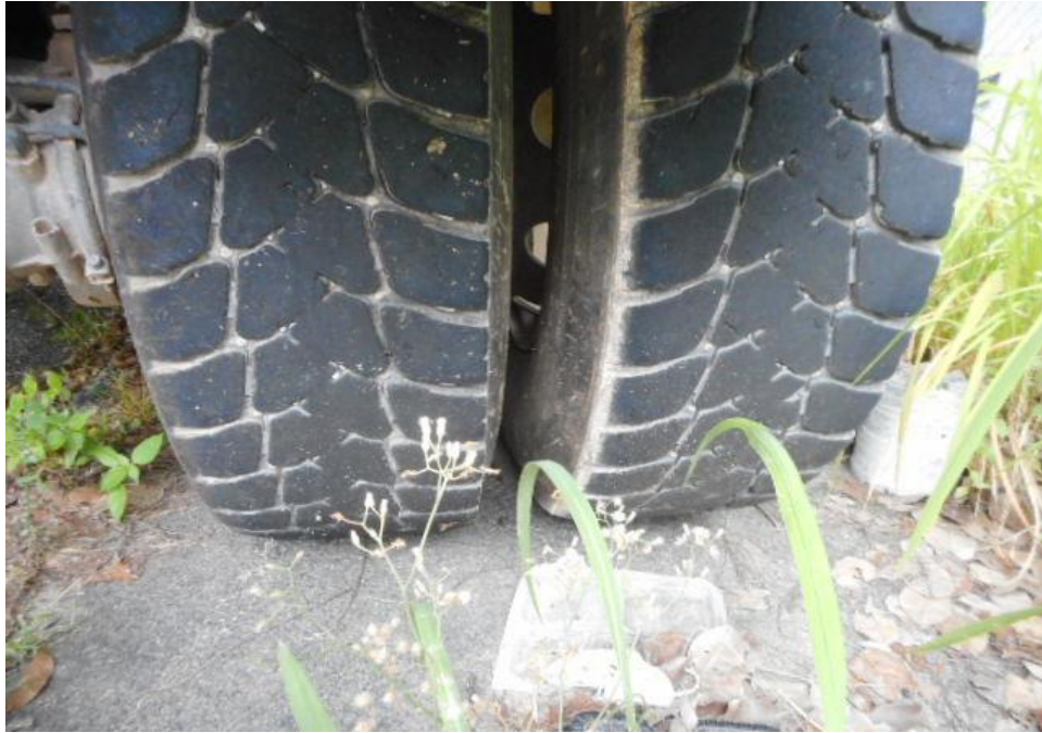
Photo 10 shows the condition of the rear right tyre of the Tipper Truck, which was observed to be in serviceable condition with remaining tread depth of approximately 6.1mm. The tyre, which was wrapped around standard steel wheel rim, was also observed to be sufficiently inflated for vehicular operation.
