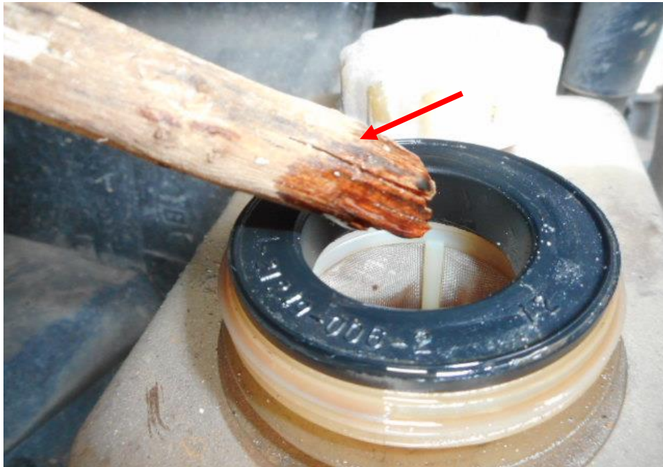
Photo 15 shows checks being carried out to the power steering fluid of the Tipper Truck at the time of my inspection. The power steering fluid was observed to be of sufficient level (arrowed) and without any visible contamination.
