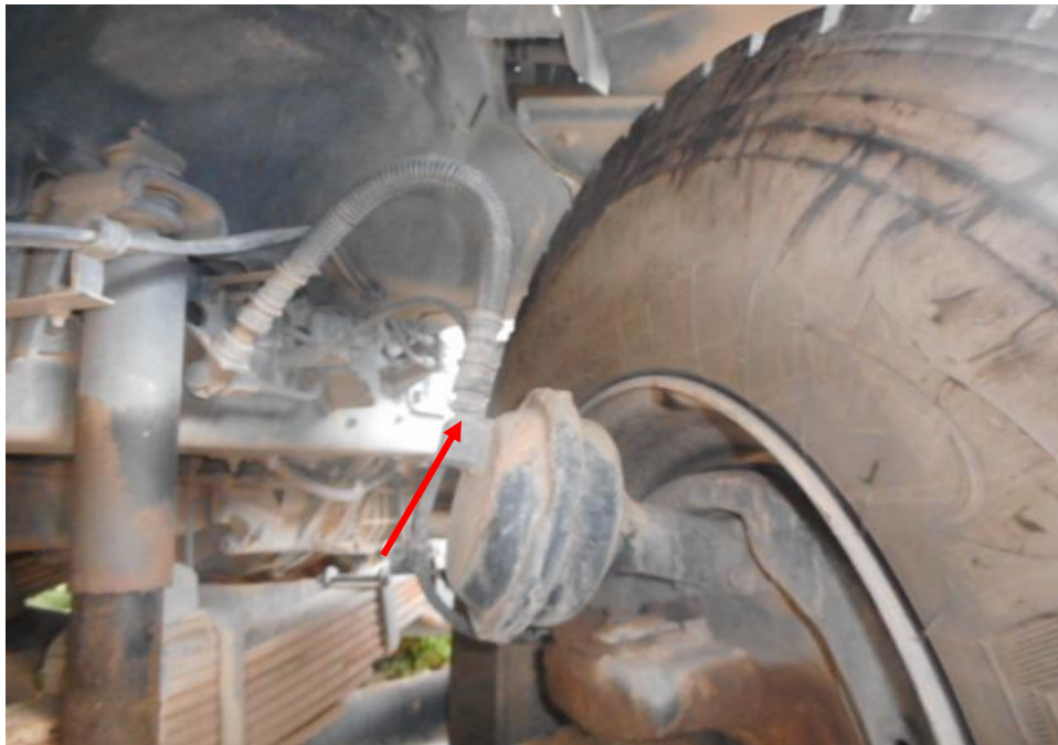
Photo 20 shows the brake pipe (arrowed) at the front left wheel of the Tipper Truck. I did not observe any leakage of brake fluid at the time of my inspection of the Tipper Truck and the various mechanical components was observed to be intact.
