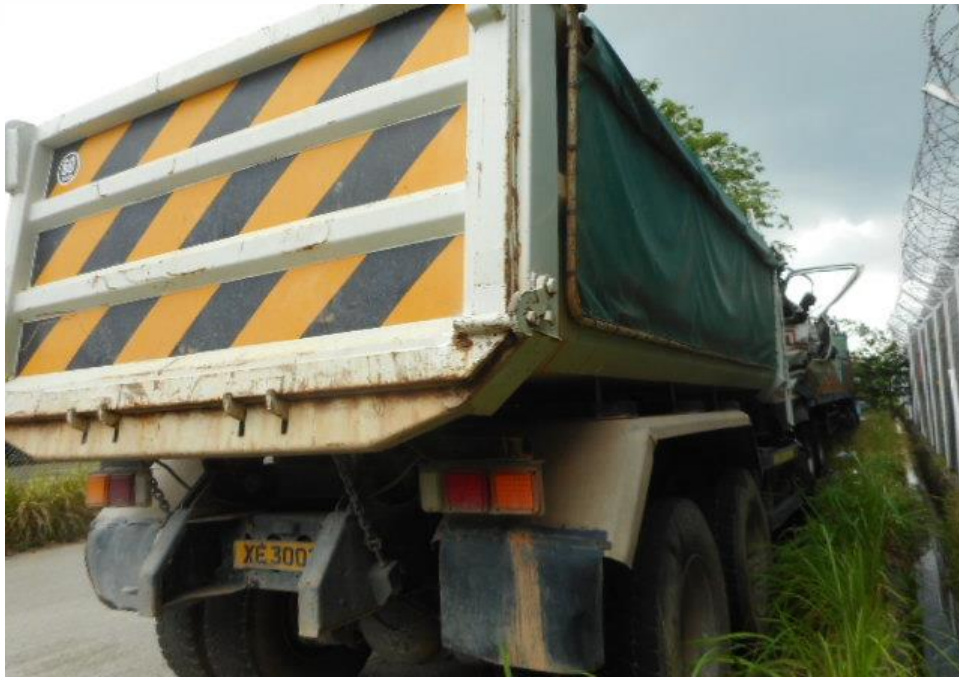
Photo 6 shows a general view of the right body of the Tipper Truck at the time of my inspection, it was observed to have been unaffected by the accident.
