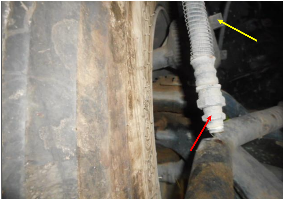
Photo 19 shows the brake pipe (red arrow) and the air brake unit (yellow arrow) of the front right wheel of the Tipper Truck, it was observed to be damaged and broken off as a result of the accident.
