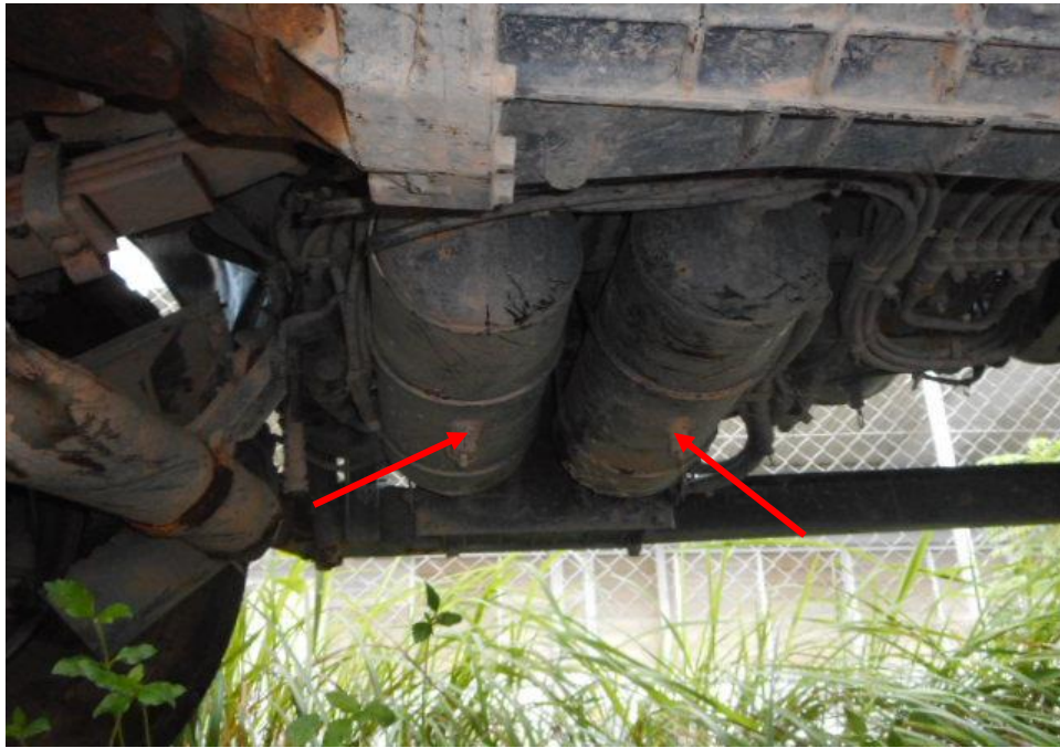
Photo 23 shows the air brake cylinders (arrowed) at the undercarriage of the Tipper Truck. I did not observe any leakage of brake fluid at the time of my inspection of the Tipper Truck and the various mechanical components was observed to be intact.
