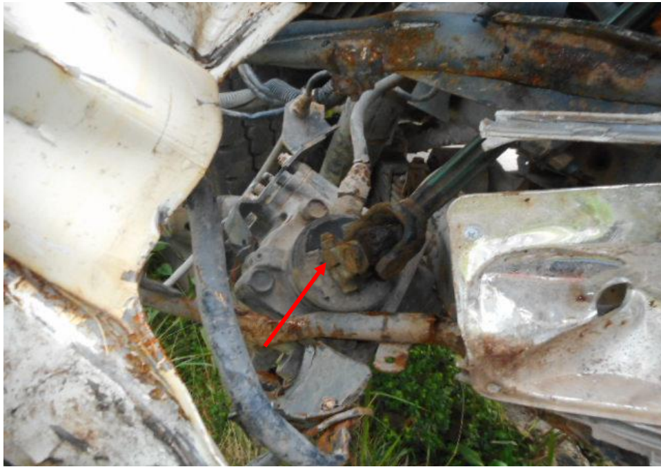
Photo 18 shows the steering box component (arrowed) at the undercarriage of the Tipper Truck was found to be damaged as a result of the accident.
