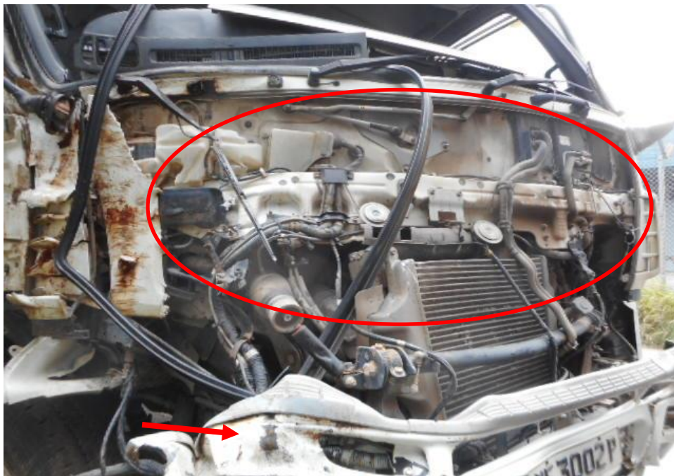
Photo 3 shows the close up view of the Tipper Truck front body at the time of my inspection. The Tipper Truck was observed to have sustained damage at its front body panel (circled) and front bumper (arrowed) was also damaged as a result of the accident.
