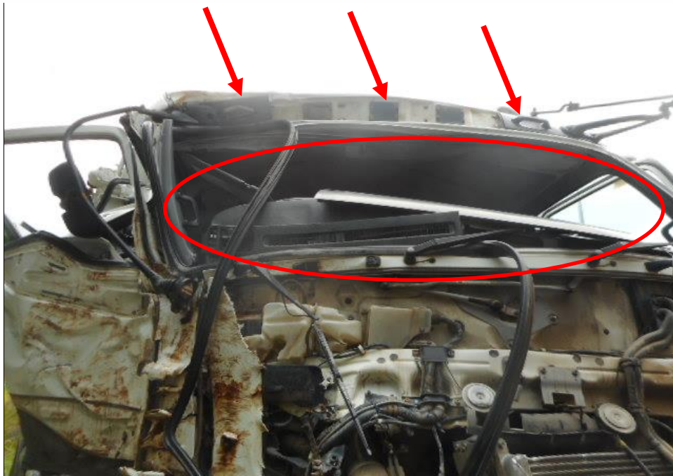
Photo 2 shows the close up view of the Tipper Truck front body at the time of my inspection. The Tipper Truck was observed to have sustained damage at its front cabin (arrowed) and front windscreen (circled), as a result of the accident.
