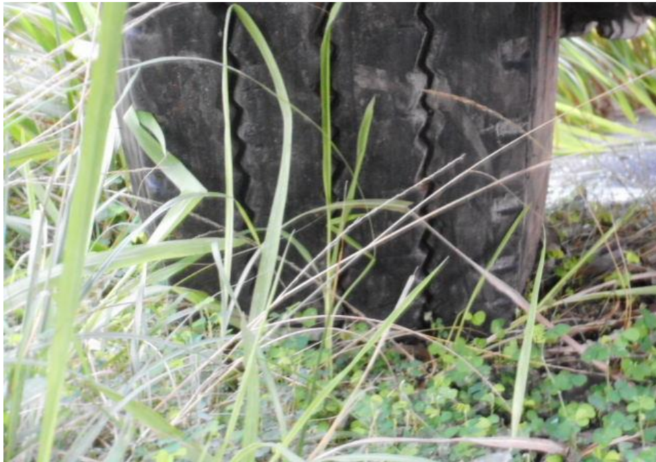
Photo 9 shows the condition of the front right tyre of the Tipper Truck, which was observed to be in serviceable condition with remaining tread depth of approximately 8.7 mm. The tyre, which was wrapped around standard steel wheel rim, was also observed to be sufficiently inflated for vehicular operation. There was no tear, cut or burst mark(s) on the outer and the inner sidewalls as well as across the tread of the 10 tyres that were fitted on the Tipper Truck.
