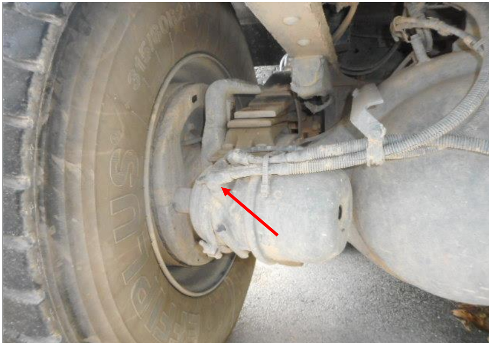
Photo 22 shows the brake pipe (arrowed) at the rear left wheel of the Tipper Truck. I did not observe any leakage of brake fluid at the time of my inspection of the Tipper Truck and the various mechanical components was observed to be intact.
