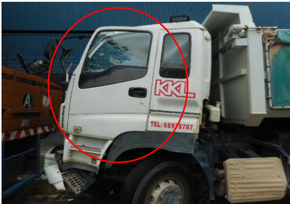
Photo 5 shows the close up view of the Tipper Truck front body at the time of my inspection. The Tipper Truck was observed to have sustained damage at its front left door (circled) as a result of the accident.
