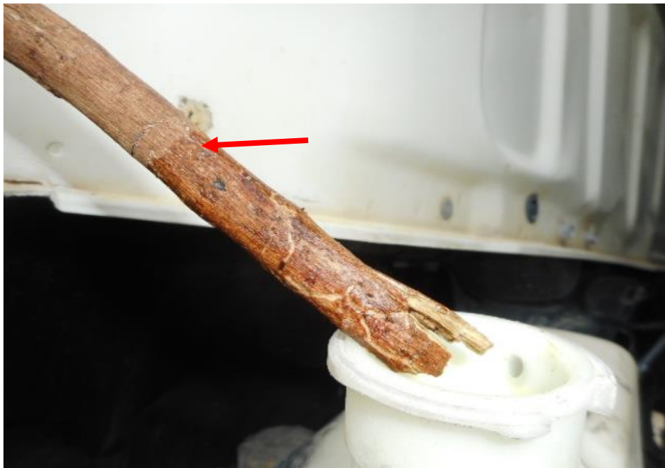
Photo 14 shows checks being carried out to the engine coolant of the Tipper Truck at the time of my inspection. The engine coolant was observed to be of sufficient level (arrowed) and without any visible contamination.
