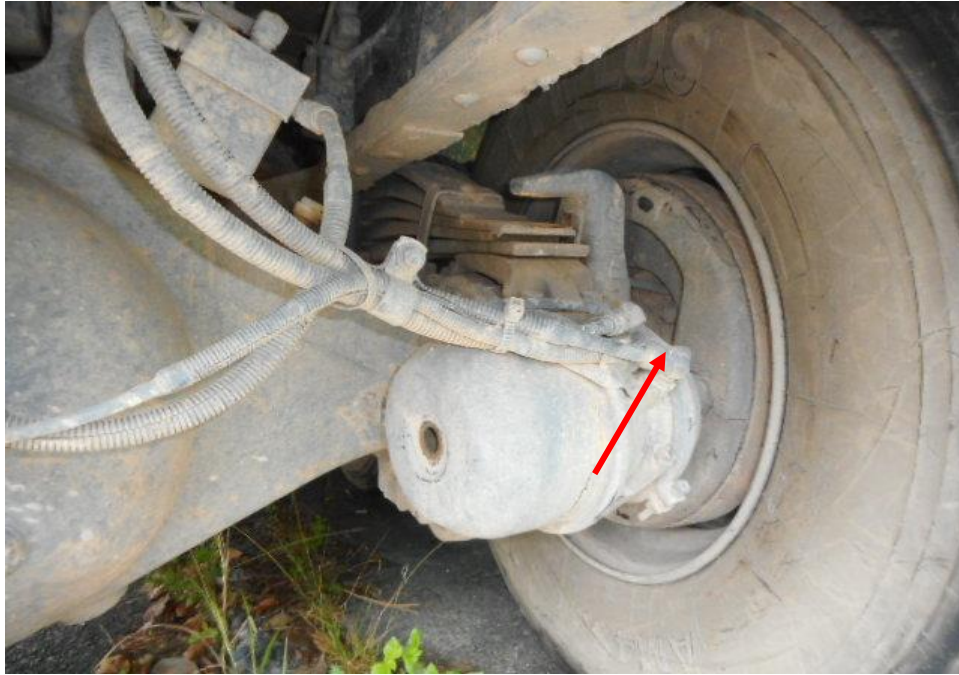
Photo 21 shows the brake pipe (arrowed) at the rear right wheel of the Tipper Truck. I did not observe any leakage of brake fluid at the time of my inspection of the Tipper Truck and the various mechanical components was observed to be intact.
