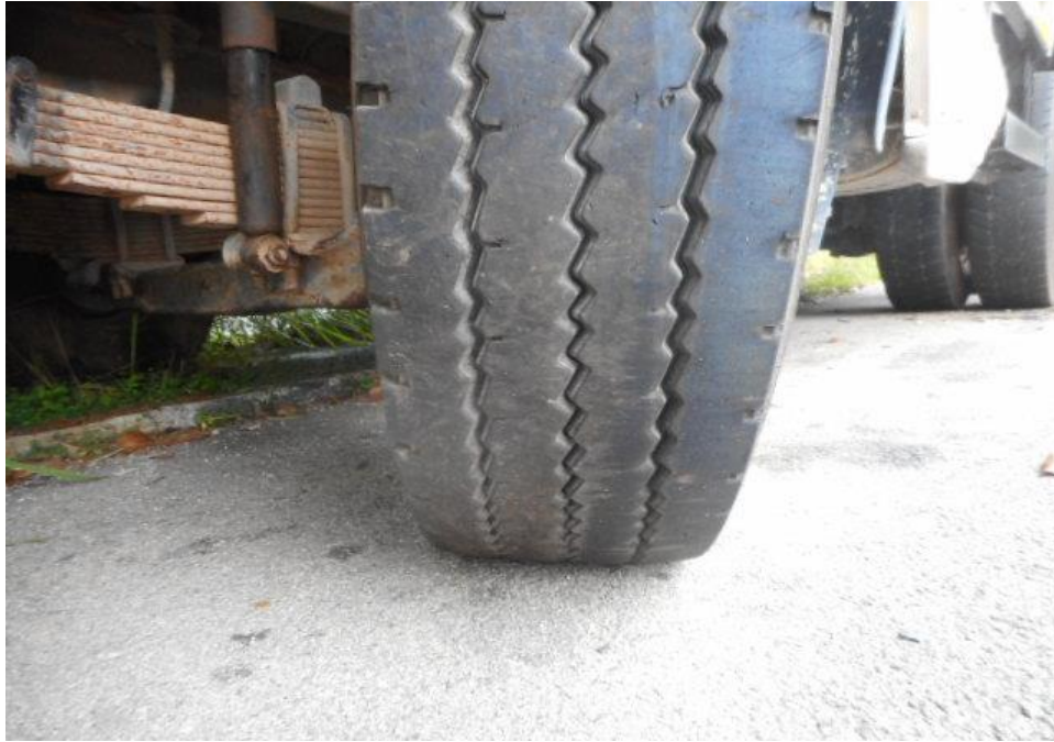
Photo 12 shows the condition of the front left tyres of the Tipper Truck, which were observed to be in serviceable condition with remaining tread depth of approximately 11.7mm. There was also no tear, cut or burst mark(s) on the outer and the inner sidewalls as well as across the tread of the 10 tyres that were fitted on the Tipper Truck.
