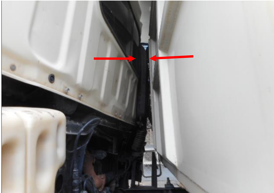
Photo 13 shows the close up view of the Tipper Truck front underside at the time of my inspection. The Tipper Truck was observed to have sustained damage at its engine, its oil hoses (red arrow) and radiator (yellow arrow) was also damaged as a result of the accident.
