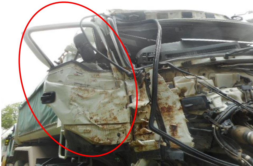
Photo 4 shows the close up view of the Tipper Truck front body at the time of my inspection. The Tipper Truck was observed to have sustained damage at its front right door (circled) as a result of the accident.
