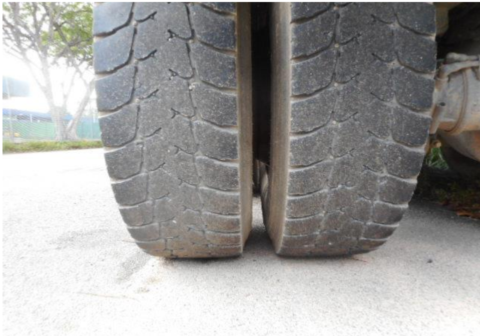
Photo 11 shows the condition of the rear left tyres of the Tipper Truck, which was observed to be in serviceable condition with remaining tread depth of approximately 5.8mm. The tyres, which were wrapped around standard steel wheel rim, were also observed to be sufficiently inflated for vehicular operation. There was also no damage found on all 10 steel wheel rims of the Tipper Truck.
