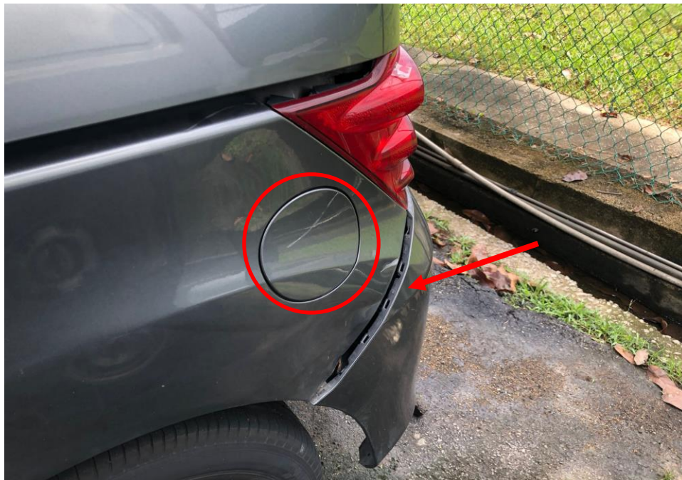
Photo 3 shows a close up view of the Motor Car's rear body at the time of my inspection. The rear portion of the Motor Car was observed to have sustained damage. Its rear body panel (circled), and rear bumper (arrowed) was the body parts that were damaged as a result of the accident.
