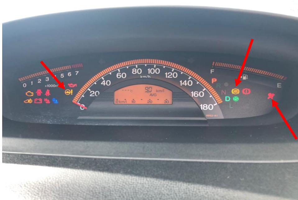
Photo 23 shows the warning light for Anti-Lock Brake System (ABS), Traction Control System (TCS) and Supplemental Restraint System (SRS) (arrowed) appearing on the instrument panel of the Motor Car during the self-test of its various electronic operating systems when its engine was cranked.
