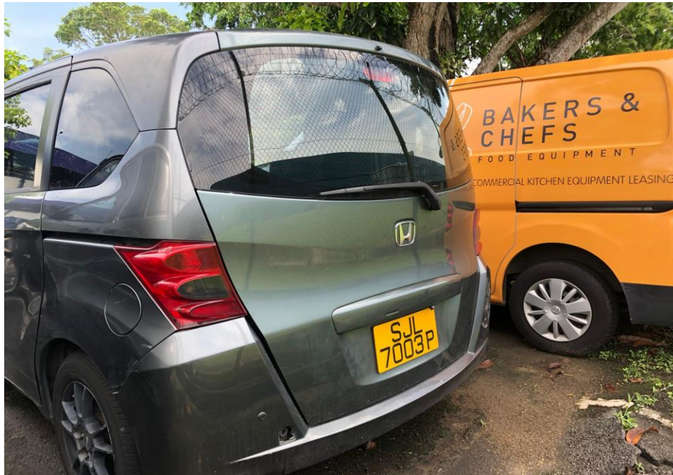
Photo 2 shows a general view of the Motor Car's rear body at the time of my inspection. The rear portion. Its rear body panel and rear bumper was the body parts that were damaged as a result of the accident.
