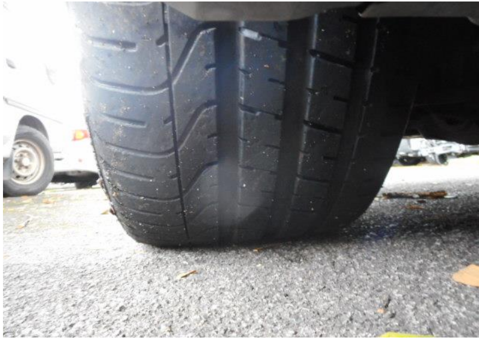
Photo 10 shows the condition of the front left tyre of the Motor Car, which was observed to be in serviceable condition with remaining tread depth of approximately 5.7mm. There was also no tear, cut or burst mark(s) on the outer and the inner sidewalls as well as across the tread of the Motor Car's 4 tyres.
