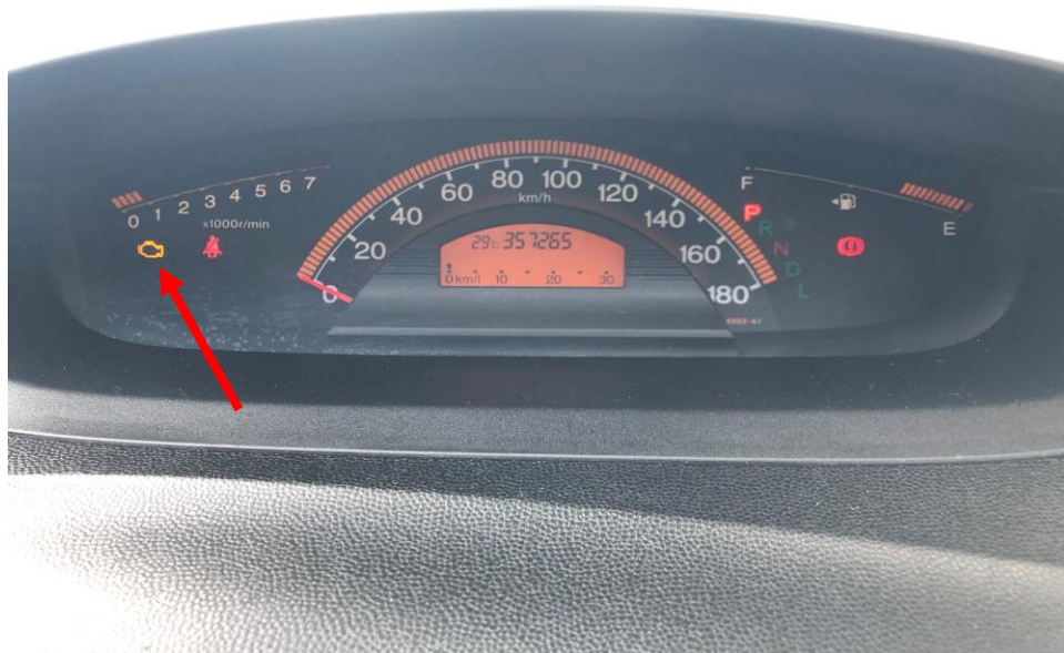
Photo 24 shows no warning lights illuminated on the instrument panel of the Motor Car after the engine was cranked. Only the engine light (arrowed) remained illuminated on, this is due to a pre-existing fault in the system and did not affect the Motor Car in its operational test. However, this would suggest that there was no abnormality to the other electronic operating system of the Motor Car, like the ABS, TCS and SRS etc.
