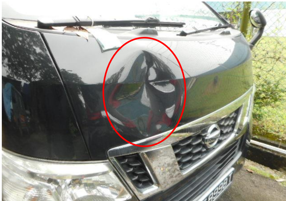
Photo 3 shows a close up view of the Motor Van's frontal portion at the time of my inspection. It appeared to have sustained damage at its frontal portion. Its front body panel (circled) was damage at the time of my inspection as a result of the accident.
