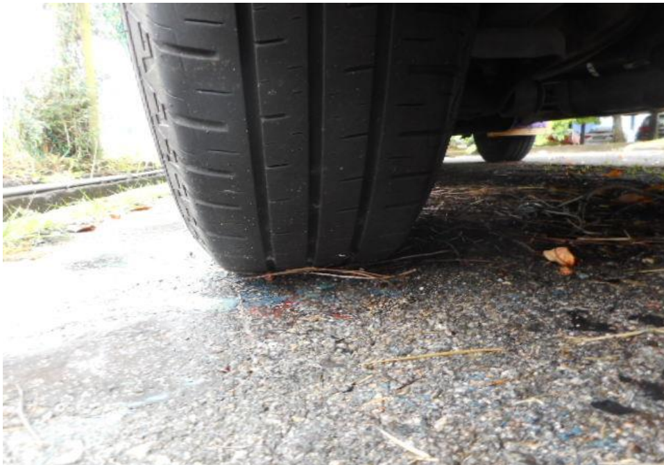
Photo 9 shows the condition of the rear left tyres of the Motor Van, which was observed to be in serviceable condition with remaining tread depth of approximately 3.7mm. The tyres, which were wrapped around standard steel wheel rim, were also observed to be sufficiently inflated for vehicular operation. There was also no damage found on all 4 steel wheel rims of the Motor Van.
