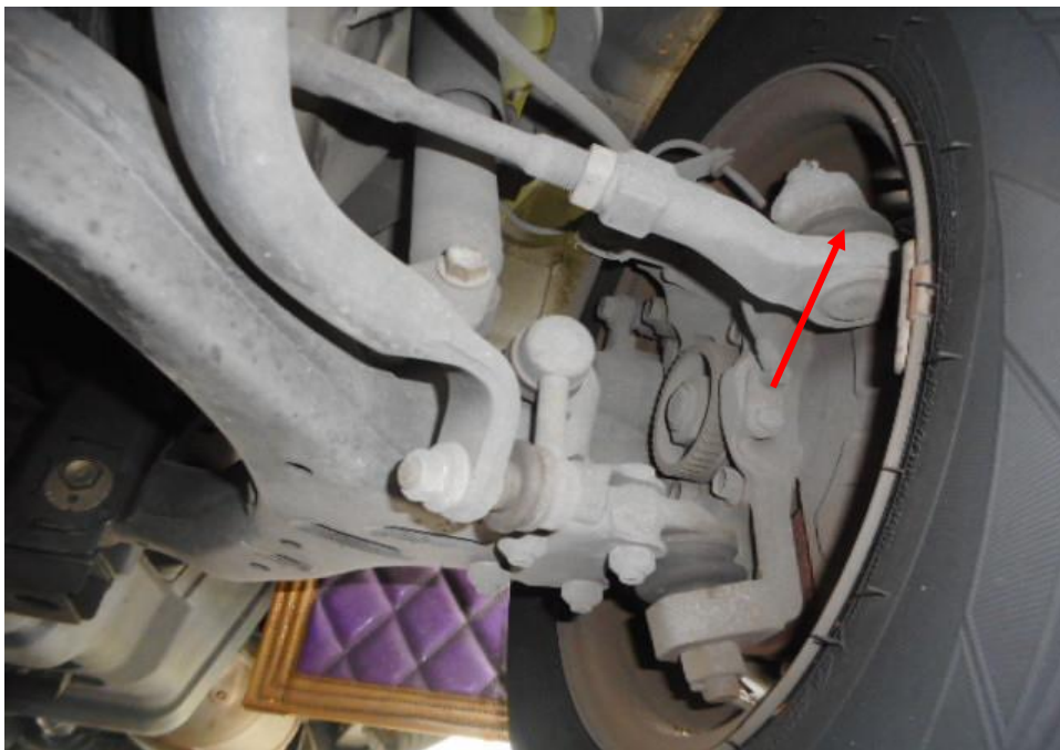
Photo 17 shows the various undercarriage components at the front left wheel of the Motor Van, in particular the steering tie rod end (arrowed). The various undercarriage components of the Motor Van were all found to be intact without any visible damage. There was also no sign of fluid stain(s) observed on the various undercarriage components.
