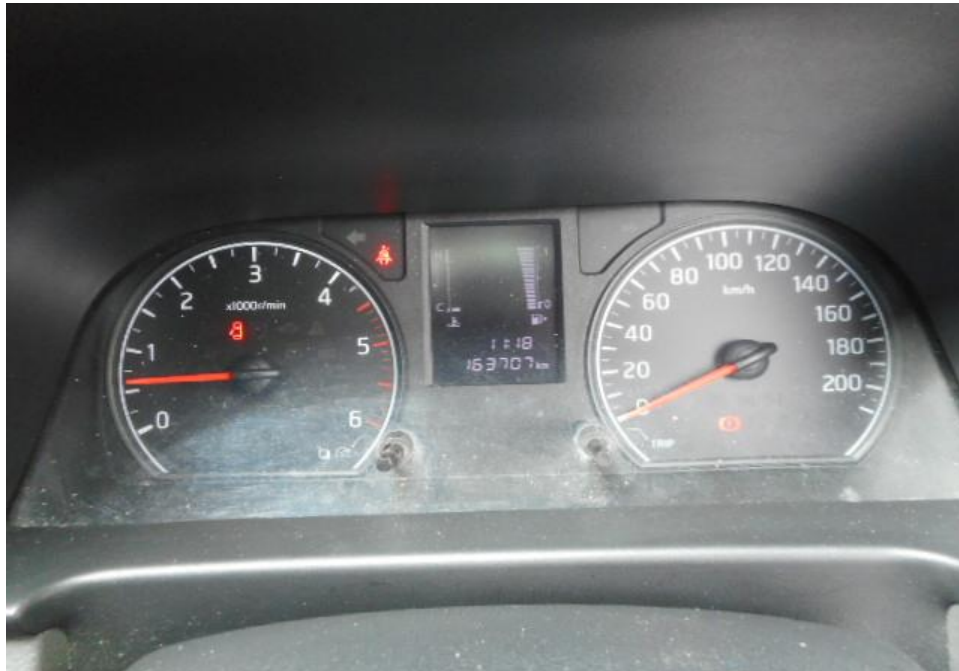
Photo 24 shows no warning lights illuminated on the instrument panel of the Motor Van after the engine was cranked. This would suggest that there was no abnormality to the electronic operating system of the Motor Van, like the ABS, SRS and etc.
