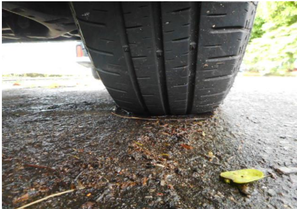
Photo 7 shows the condition of the front right tyre of the Motor Van, which was observed to be in serviceable condition with remaining tread depth of approximately 5.2mm. The tyre, which was wrapped around standard steel wheel rim, was also observed to be sufficiently inflated for vehicular operation. There was no tear, cut or burst mark(s) on the outer and the inner sidewalls as well as across the tread of the 4 tyres that were fitted on the Motor Van.
