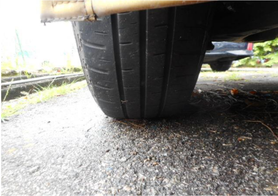
Photo 10 shows the condition of the rear right tyres of the Motor Van, which were observed to be in serviceable condition with remaining, tread depth of approximately 4.4mm. There was also no tear, cut or burst mark(s) on the outer and the inner sidewalls as well as across the tread of the 4 tyres that were fitted on the Motor Van.
