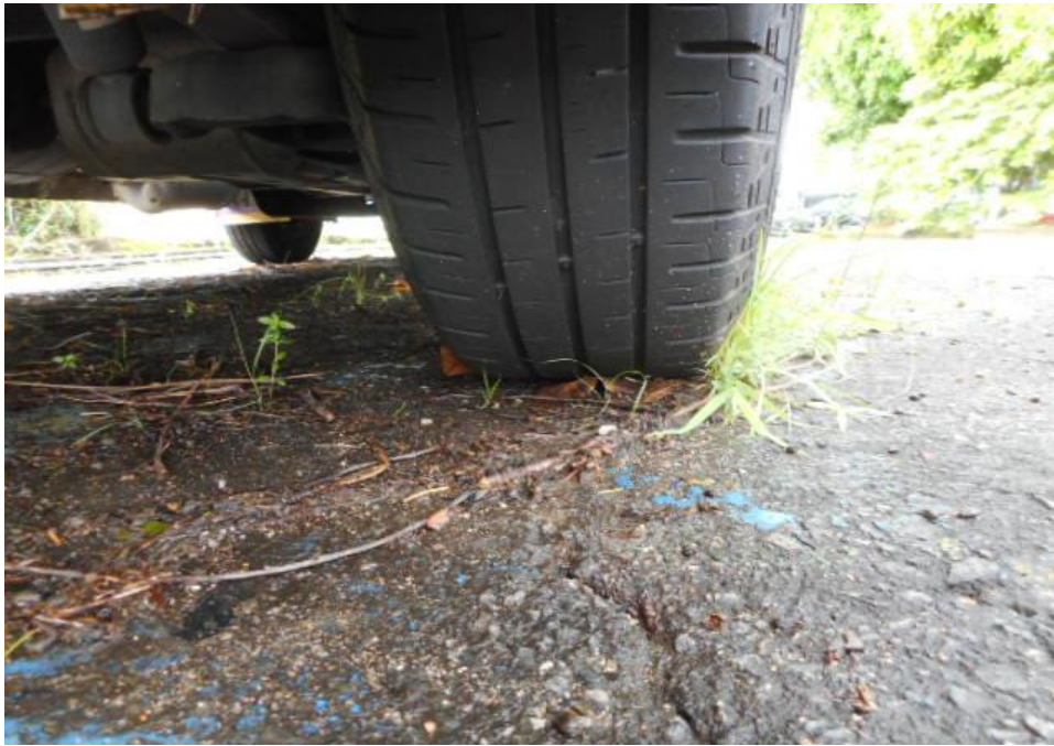
Photo 8 shows the condition of the rear right tyre of the Motor Van, which was observed to be in serviceable condition with remaining tread depth of approximately 3.8mm. The tyre, which was wrapped around standard steel wheel rim, it was observed to be sufficiently inflated for vehicular operation.
