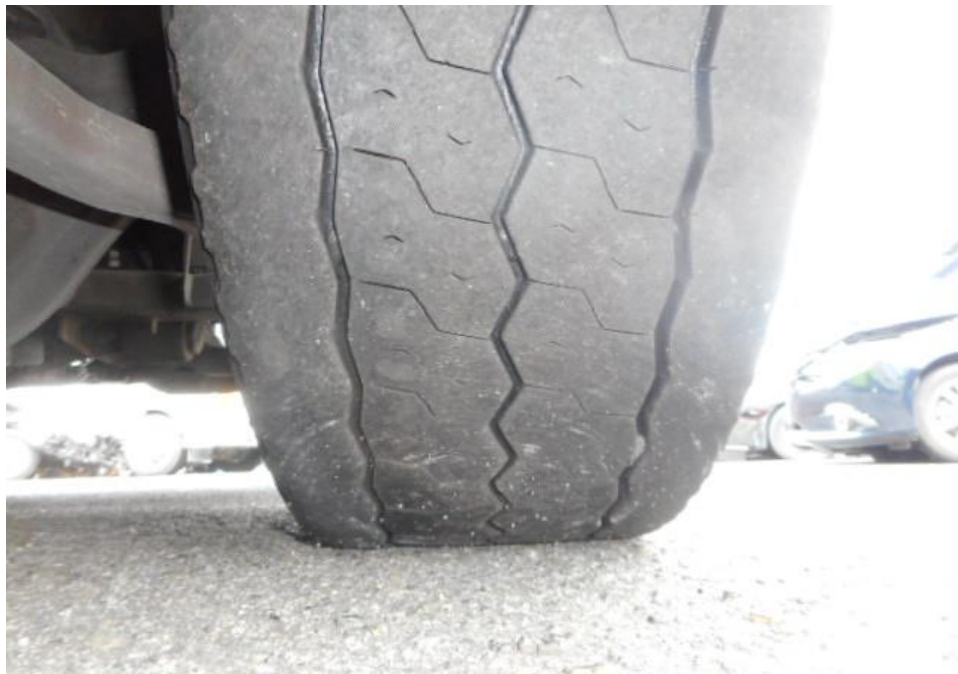
Photo 7 shows the condition of the front right tyre of the Motor Bus, which was observed to be in serviceable condition with remaining tread depth of approximately 8.9mm. The tyre, which was wrapped around standard steel wheel rim, was also observed to be sufficiently inflated for vehicular operation. There was no tear, cut or burst mark(s) on the outer and the inner sidewalls as well as across the tread of the 8 tyres that were fitted on the Motor Bus.
