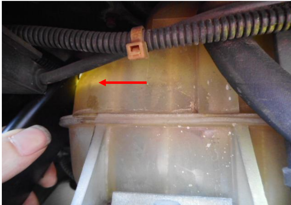
Photo 13 shows the engine coolant reservoir of the Motor Bus at the time of my inspection. The engine coolant was observed to be of sufficient level (arrowed) and without any visible contamination.
