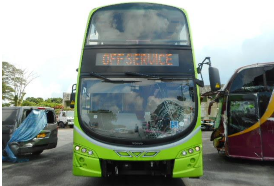
Photo 3 shows a general view of the front body of the Motor Bus at the time of my inspection. The Motor Bus was observed to have sustained damages at its front windscreen was observed to be damaged at time of our inspection.
