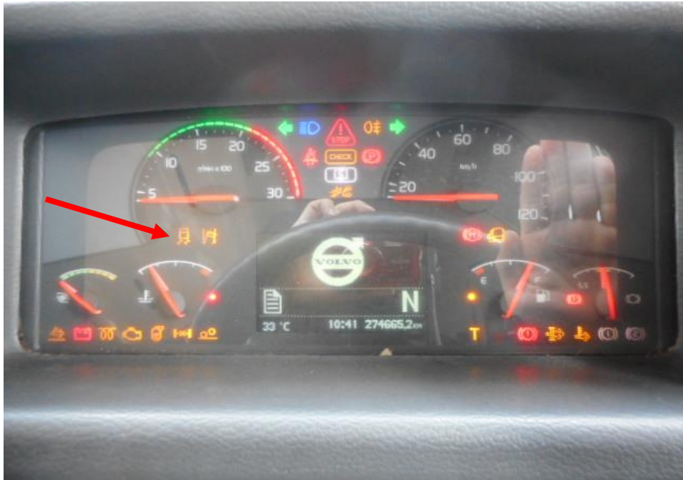
Photo 25 shows the warning light for Traction Control System (TCS) appearing on the instrument panel of the Motor Bus during the self-test of its various electronic operating systems when its engine was cranked.
