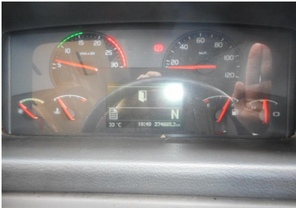
Photo 26 shows no warning lights illuminated on the instrument panel of the Motor Bus after the engine was cranked. This would suggest that there was no abnormality to the various electronic operating systems of the Motor Bus, like the TCS and etc.
