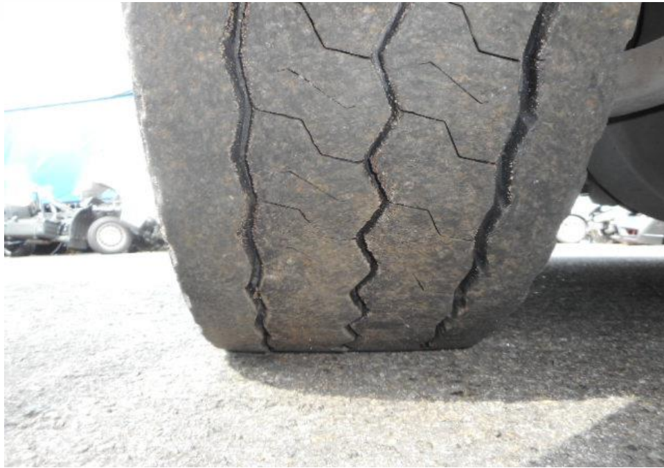
Photo 10 shows the condition of the front left tyres of the Motor Bus, which were observed to be in serviceable condition with remaining tread depth of approximately 13.4mm. There was also no tear, cut or burst mark(s) on the outer and the inner sidewalls as well as across the tread of the 8 tyres that were fitted on the Motor Bus.
