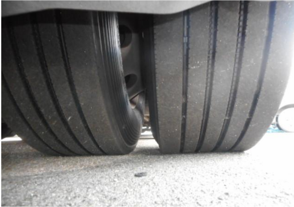
Photo 8 shows the condition of the rear right tyre of the Motor Bus, which was observed to be in serviceable condition with remaining tread depth of approximately 8.9mm. The tyre, which was wrapped around standard steel wheel rim, was also observed to be sufficiently inflated for vehicular operation.
