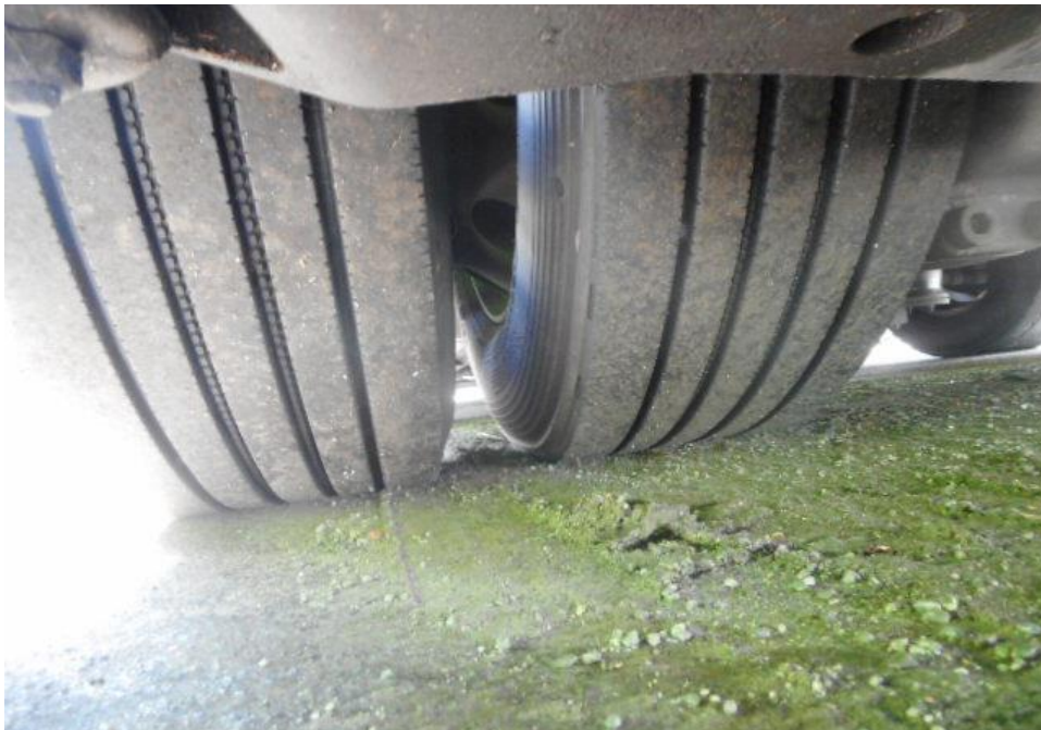
Photo 9 shows the condition of the rear left tyres of the Motor Bus, which was observed to be in serviceable condition with remaining tread depth of approximately 13.8mm. The tyres, which were wrapped around standard steel wheel rim, were also observed to be sufficiently inflated for vehicular operation. There was also no damage found on all 8 steel wheel rims of the Motor Bus.
