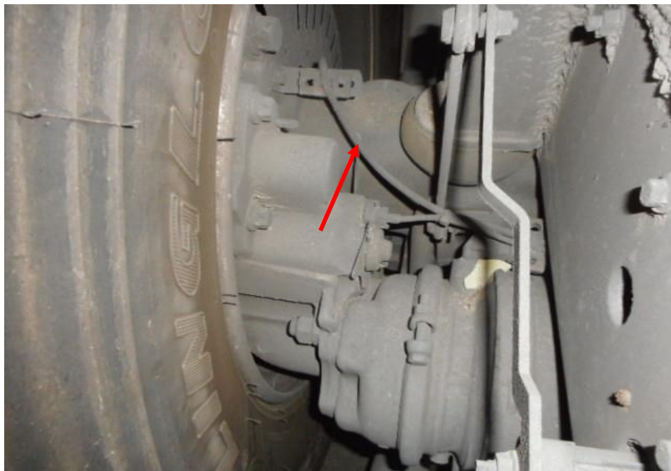
Photo 27 shows the brake pipe (arrowed) at the rear left wheel of the Motor Bus. I did not observe any leakage of brake fluid at the time of my inspection of the Motor Bus and the various mechanical components was observed to be intact.
