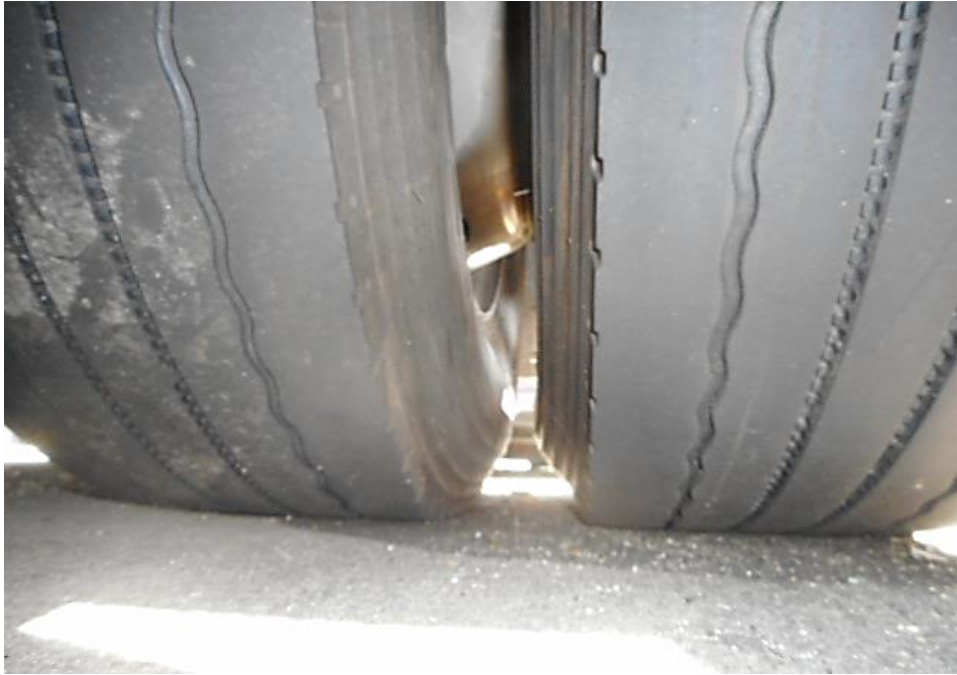
Photo 13 shows the condition of the rear right tyre of the Motor Bus, which was observed to be in serviceable condition with remaining tread depth of approximately 7.8mm. The tyre was also observed to be sufficiently inflated for vehicular operation.
