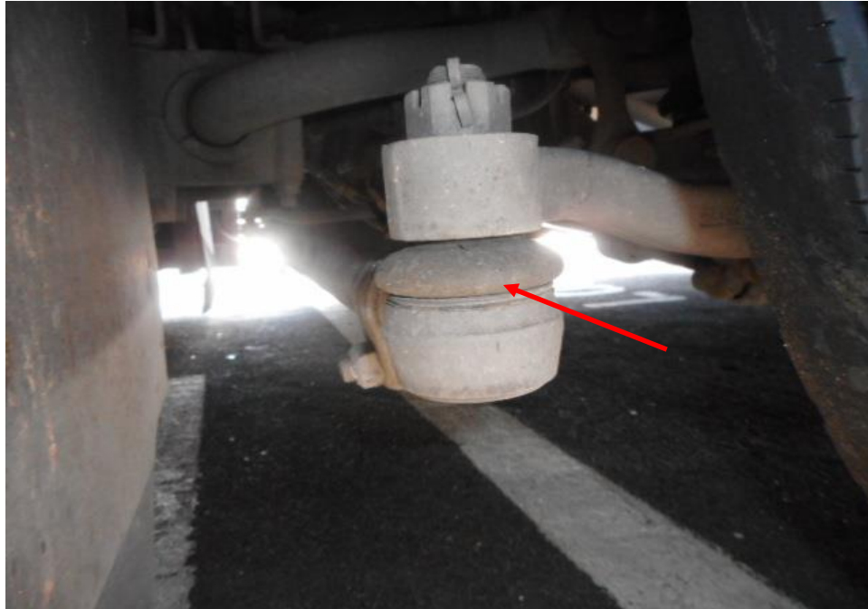
Photo 22 shows the front right wheel components of the front steering system of the Motor Bus. The various undercarriage components of the Motor Bus were all observed to be intact and without any visible damage. This had included the steering rack and steering ball joints (arrowed) of the Motor Bus, which were observed to be securely attached to the front right wheel.
