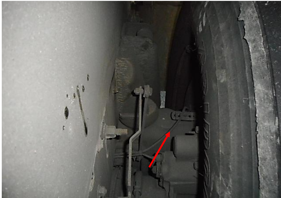
Photo 26 shows the brake pipe (arrowed) at the rear right wheel of the Motor Bus. I did not observe any leakage of brake fluid at the time of my inspection of the Motor Bus and the various mechanical components was observed to be intact.
