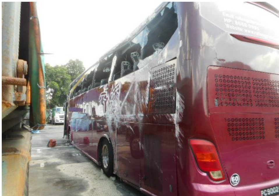
Photo 10 shows a general view of the left side of the Motor Bus at the time of our inspection. The Motor Bus was observed to have sustained damages at its left body panels and windcreens as a result of the accident.
