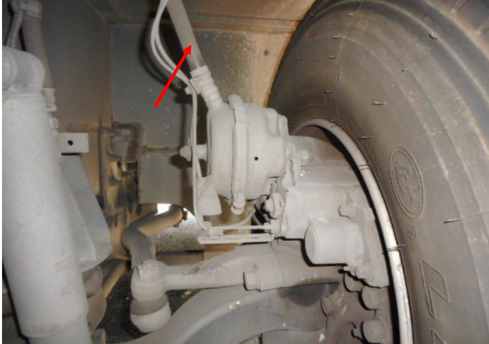
Photo 24 shows the brake pipe (arrowed) at the front right wheel of the Motor Bus. I did not observe any leakage of brake fluid/air at the time of my inspection of the Motor Bus and the various mechanical components was observed to be intact.
