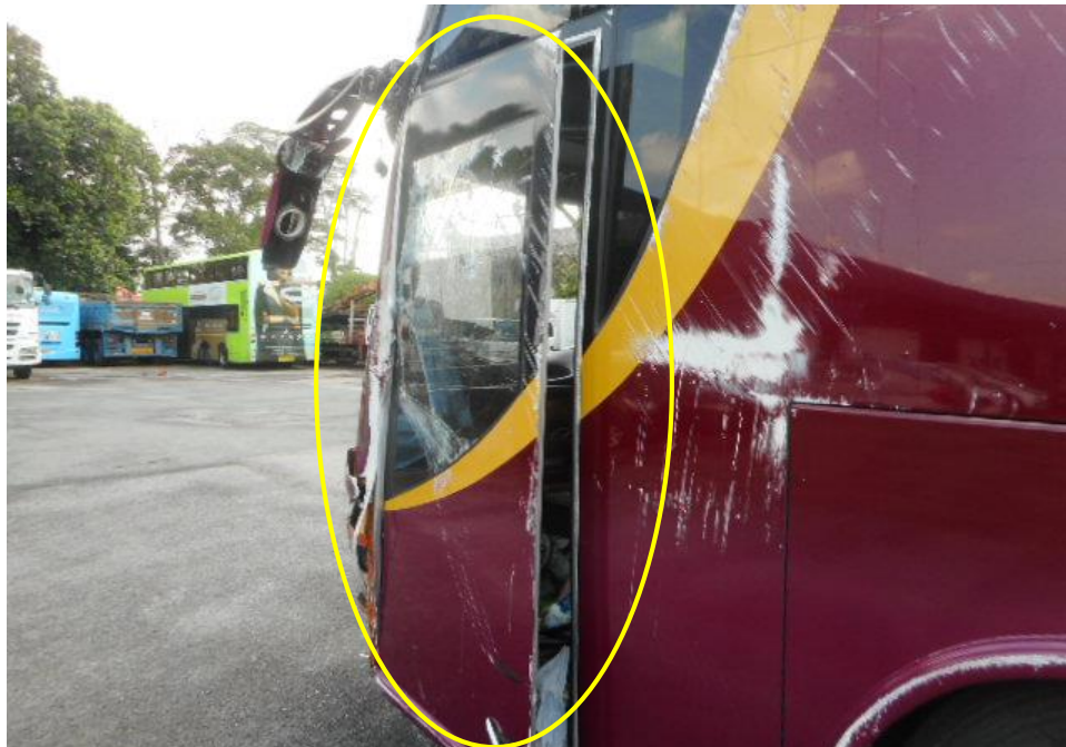
Photo 6 shows a close up view of the front body of the Motor Bus at the time of our inspection. The Motor Bus was observed to have sustained damages at its front door (circled) as a result of the accident.
