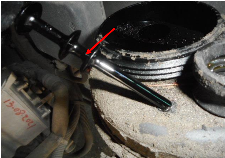
Photo 19 shows the power steering fluid reservoir of the Motor Bus at the time of my inspection. The power steering fluid was observed to be of sufficient level (arrowed) and without any visible contamination.
