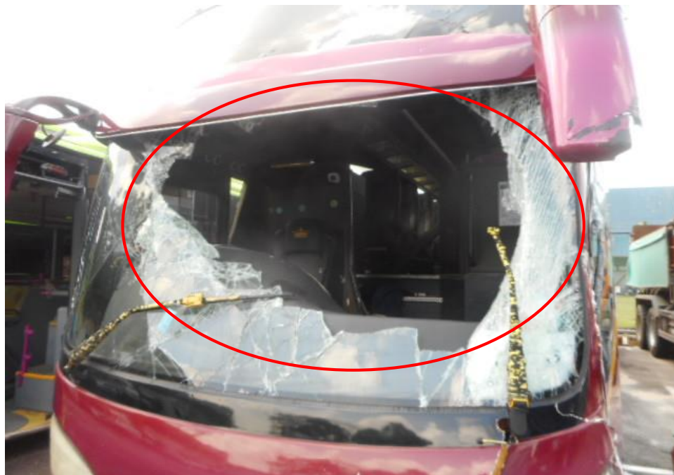
Photo 4 shows a close up view of the front body of the Motor Bus at the time of our inspection. The Motor Bus was observed to have sustained damages at its front windscreen (circled) as a result of the accident.
