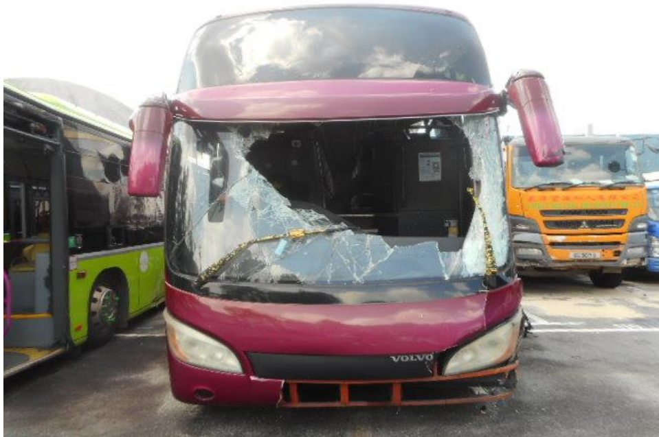
Photo 3 shows a general view of the front body of the Motor Bus at the time of our inspection. The Motor Bus was observed to have sustained damages at its front windscreen, front bumper, front door, right & left body panels as well as its windscreens was observed to be damaged at time of our inspection.
