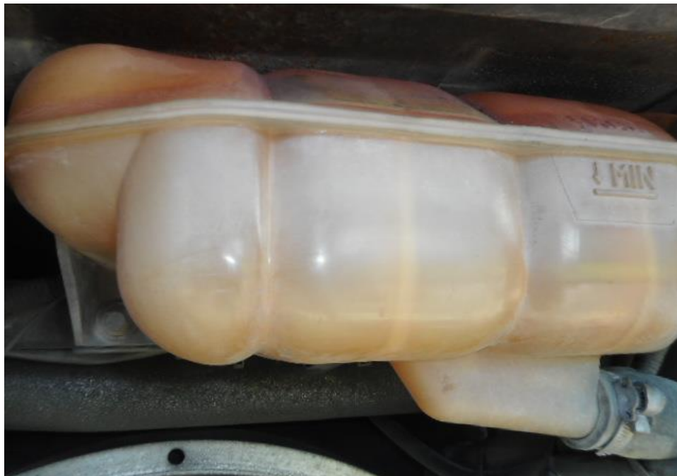
Photo 17 shows checks being carried out to the engine coolant of the Motor Bus at the time of my inspection. The engine coolant was observed to be of insufficient level.
