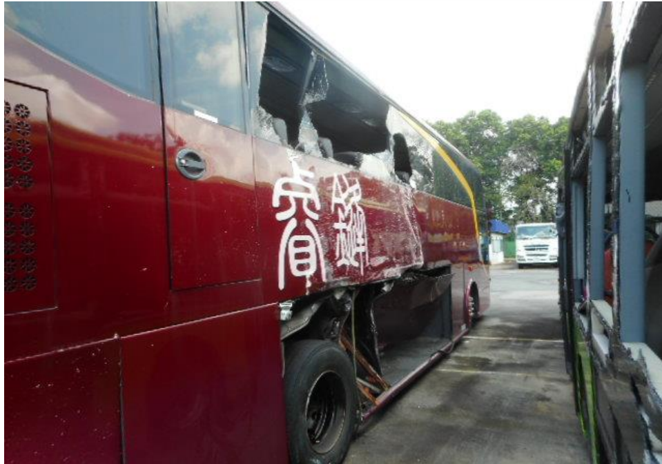
Photo 7 shows a general view of the right side of the Motor Bus at the time of our inspection. The Motor Bus was observed to have sustained damages at its right body panels and windscreens as a result of the accident.
