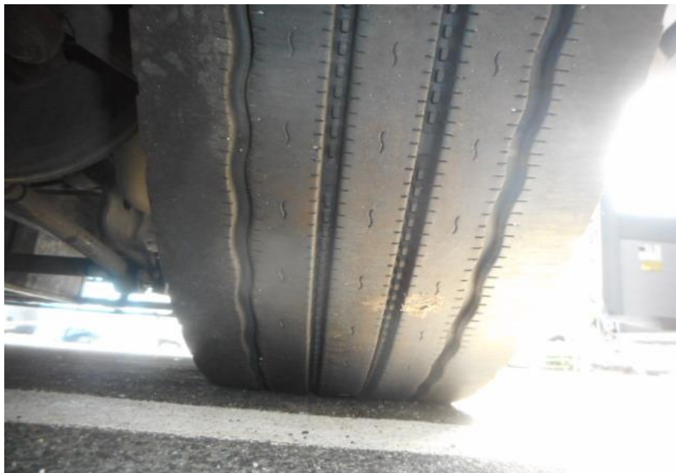
Photo 12 shows the condition of the front right tyre of the Motor Bus, which was observed to be in serviceable condition with remaining tread depth of approximately 11.1mm. The tyre was also observed to be sufficiently inflated for vehicular operation.
