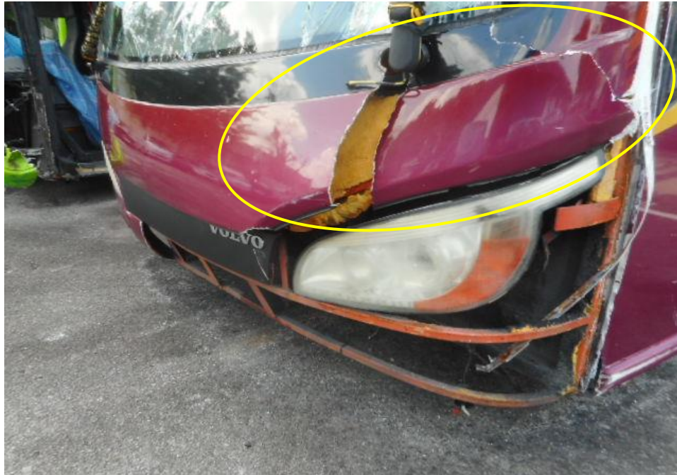
Photo 5 shows a close up view of the front body of the Motor Bus at the time of our inspection. The Motor Bus was observed to have sustained damages at its front bumper (circled) as a result of the accident.
