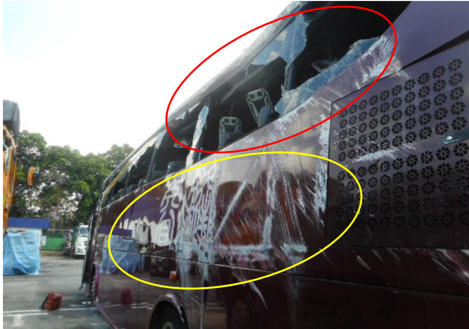
Photo 11 shows a close up view of the left side of the Motor Bus at the time of our inspection. The Motor Bus was observed to have sustained damages at its left body panels (yellow circle) and windscreens (red circle) as a result of the accident.
