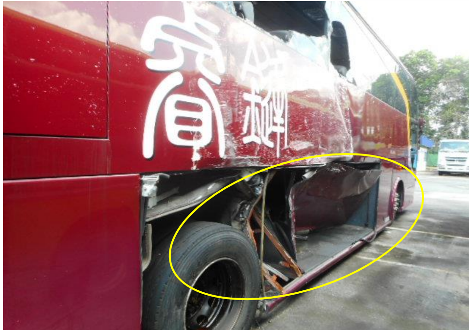
Photo 9 shows a close up view of the right side of the Motor Bus at the time of our inspection. The Motor Bus was observed to have sustained damages at its right body panels (yellow circle) as a result of the accident.
