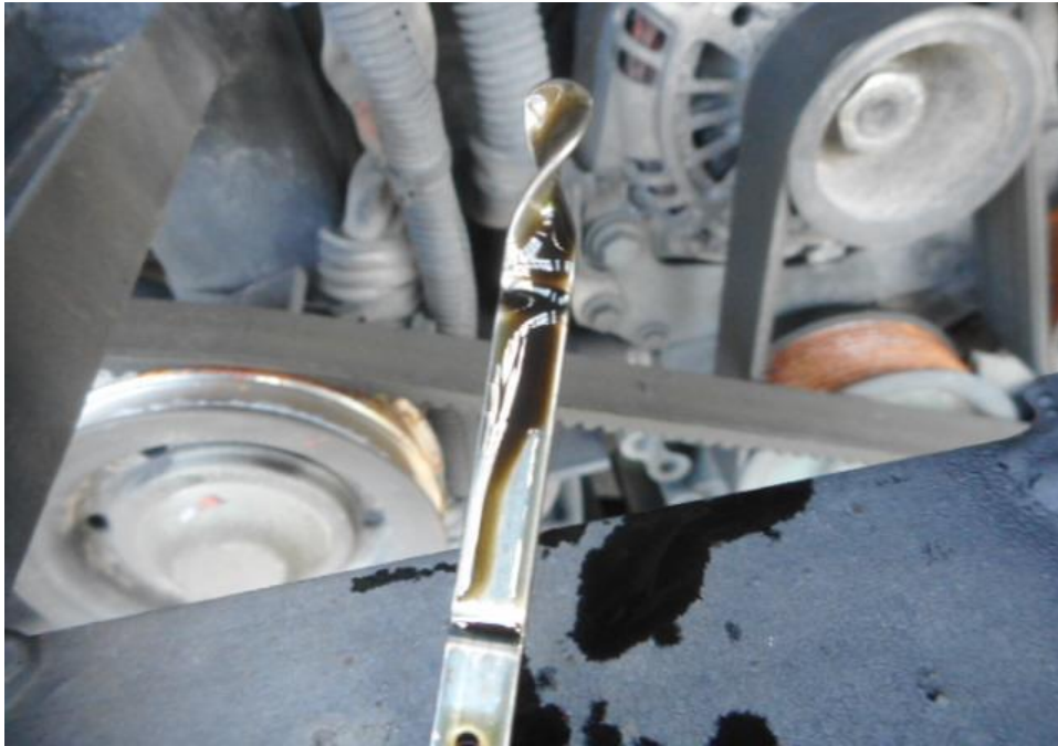
Photo 18 shows the engine oil dipstick of the Motor Bus at the time of my inspection. The engine oil was observed to be of sufficient level and without any visible contamination.
