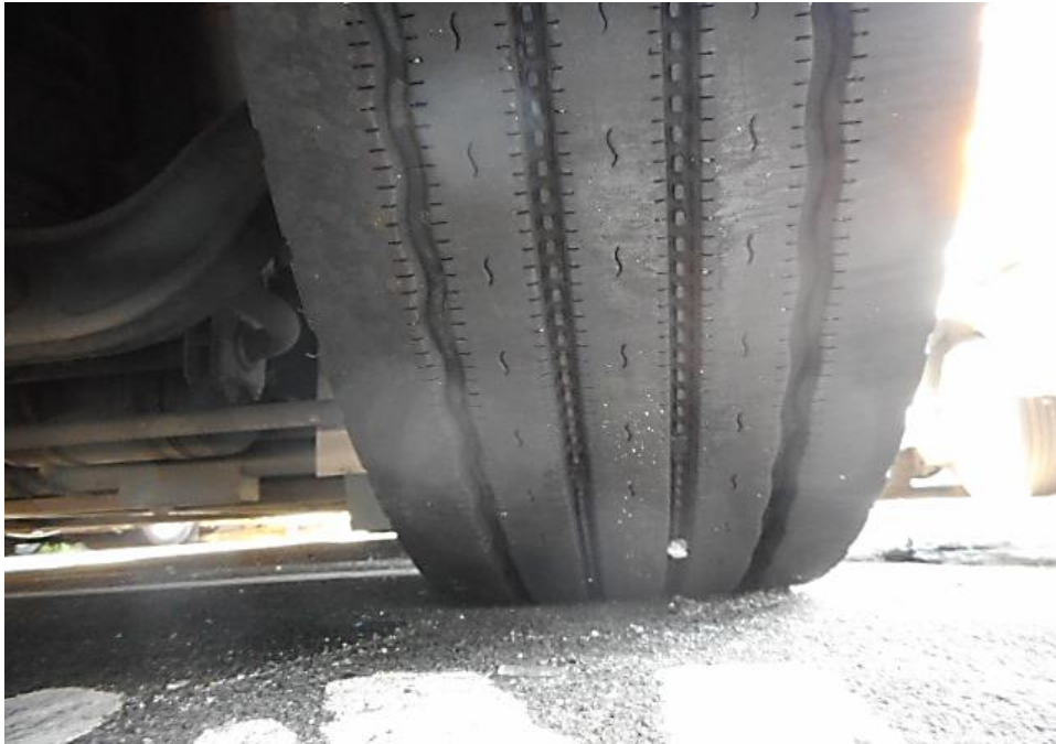
Photo 15 shows the condition of the front left tyre of the Motor Bus, which was observed to be in serviceable condition with remaining tread depth of approximately 13.5mm. The tyre was also observed to be sufficiently inflated for vehicular operation.
