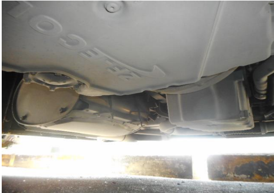
Photo 20 shows the undercarriage of the Motor Bus, at the area where the engine housing and transmission housing are located. I did not find any sign(s) or indication(s) of fluid leak and/or fluid stain(s) on the underside of the Motor Bus.
