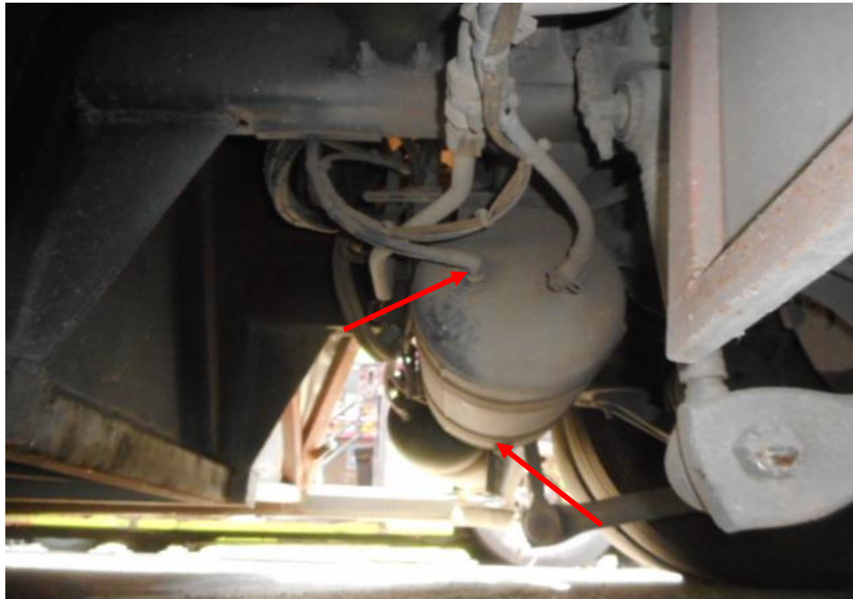
Photo 28 shows the air brake cylinders (arrowed) at the undercarriage of the Motor Bus. I did not observe any leakage of brake fluid at the time of my inspection of the Motor Bus and the various mechanical components was observed to be intact.
