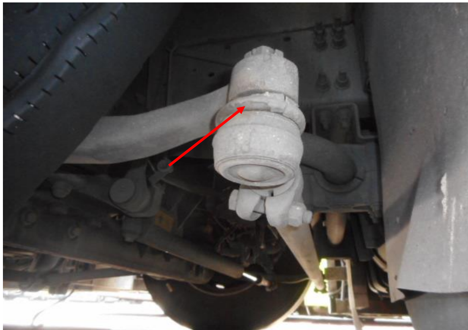
Photo 23 shows the front left wheel components of the front steering system of the Motor Bus. The various undercarriage components of the Motor Bus were all observed to be intact and without any visible damage. This had included the steering rack and steering ball joints (arrowed) of the Motor Bus, which were observed to be securely attached to the front left wheel.
