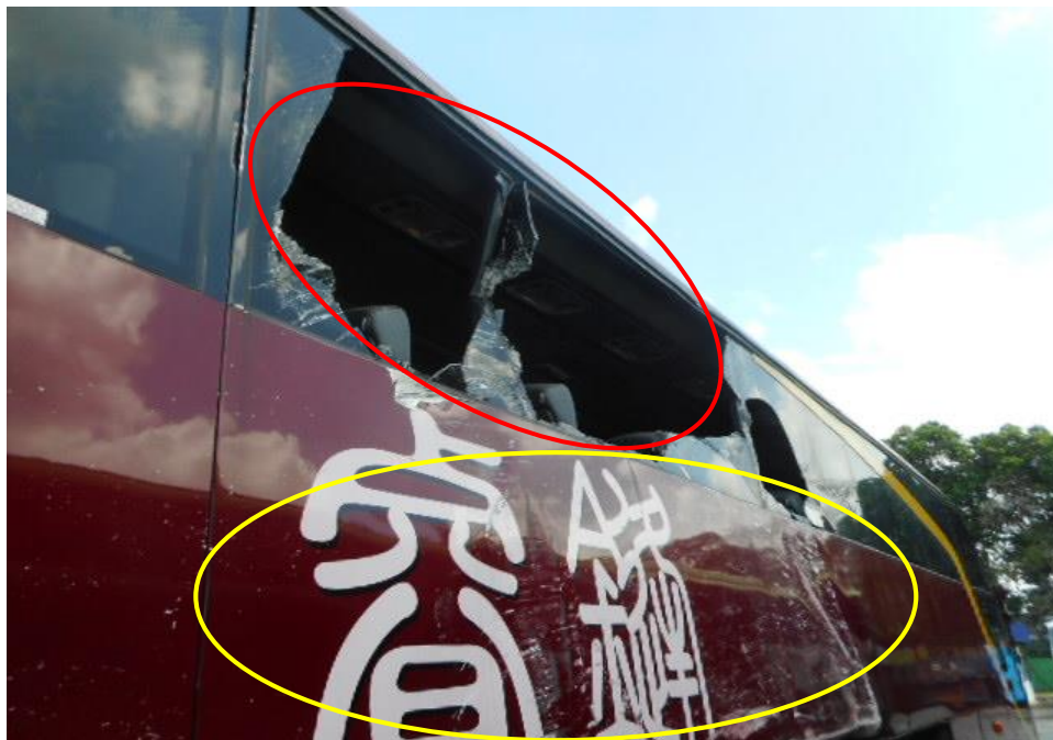
Photo 8 shows a close up view of the right side of the Motor Bus at the time of our inspection. The Motor Bus was observed to have sustained damages at its right body panels (yellow circle) and windscreens (red circle) as a result of the accident.
