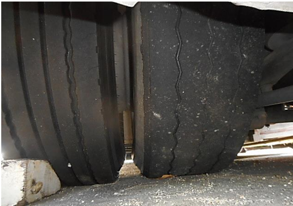
Photo 14 shows the condition of the rear right tyres of the Motor Bus, which were observed to be in serviceable condition with remaining tread depth of approximately 10.5mm. The tyres, which were wrapped around standard alloy wheel rims, were also observed to be sufficiently inflated for vehicular operation.
