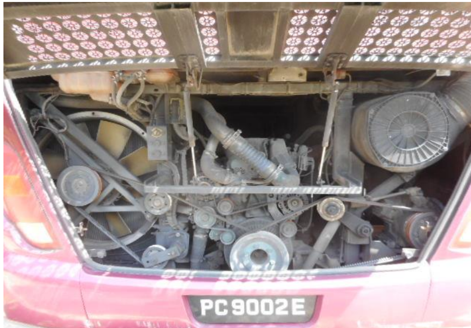
Photo 16 shows a general view of the Motor Bus engine compartment. The various parts and components inside the engine compartment were unaffected by the accident. There was also no sign(s) or indication(s) of fluid leakage and/or fluid stain within the engine compartment.
