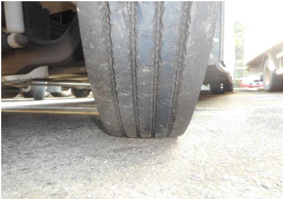
Photo 13 shows the condition of the front left tyres of the Motor Bus, which were observed to be in serviceable condition with remaining tread depth of approximately 10.2mm. There was also no tear, cut or burst mark(s) on the outer and the inner sidewalls as well as across the tread of the 6 tyres that were fitted on the Motor Bus.
