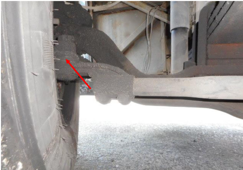
Photo 23 shows the various undercarriage components at the front left wheel of the Motor Bus, in particular the steering tie rod end (arrowed). The various steering components were all found to be intact. There was also no sign of fluid stain(s) observed on the various undercarriage components.
