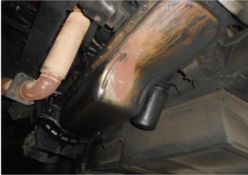
Photo 17 shows the undercarriage of the Motor Bus, at the area where the engine housing and transmission housing are located. I did not find any sign(s) or indication(s) of fluid leak and/or fluid stain(s) on the underside of the Motor Bus.
