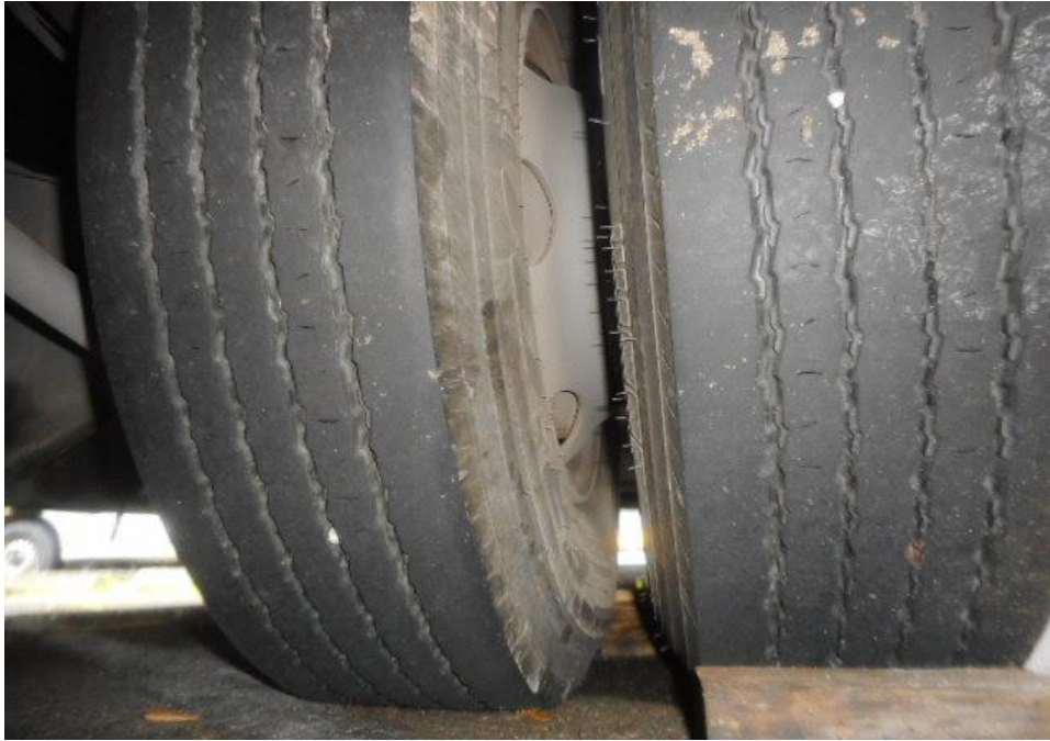
Photo 12 shows the condition of the rear left tyres of the Motor Bus, which was observed to be in serviceable condition with remaining tread depth of approximately 9mm. The tyres, which were wrapped around standard steel wheel rim, were also observed to be sufficiently inflated for vehicular operation. There was also no damage found on all 6 steel wheel rims of the Motor Bus.
