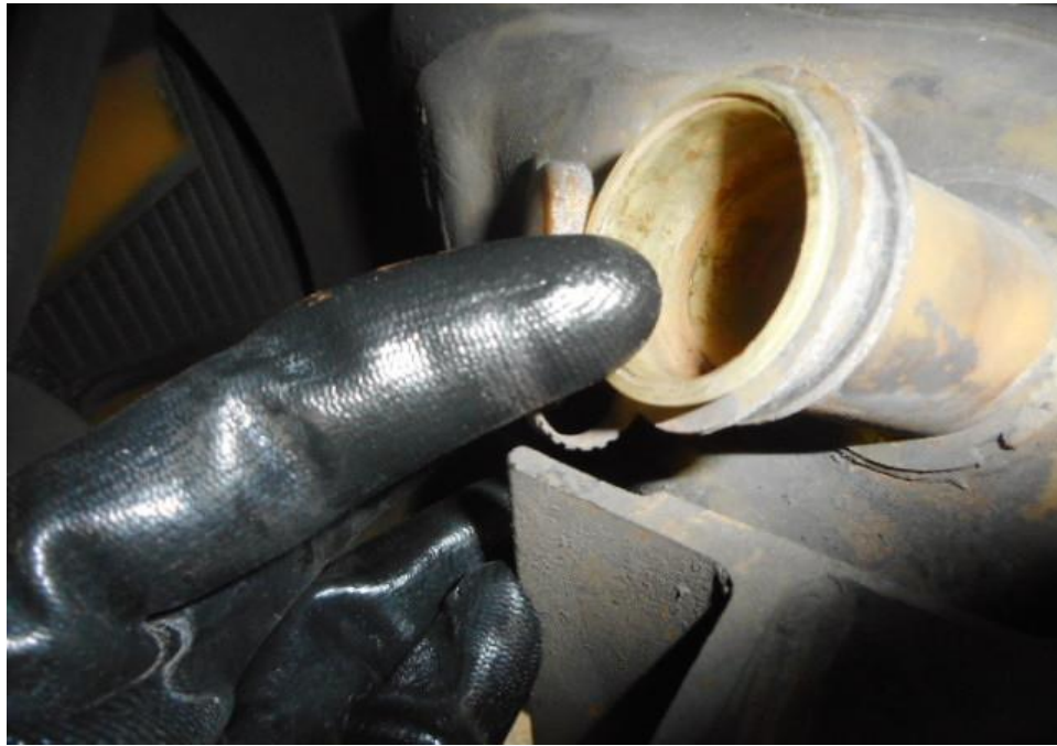
Photo 15 shows the engine coolant reservoir of the Motor Bus at the time of my inspection. The engine coolant was observed to be of insufficient level likely due to a leakage as a result of the accident.
