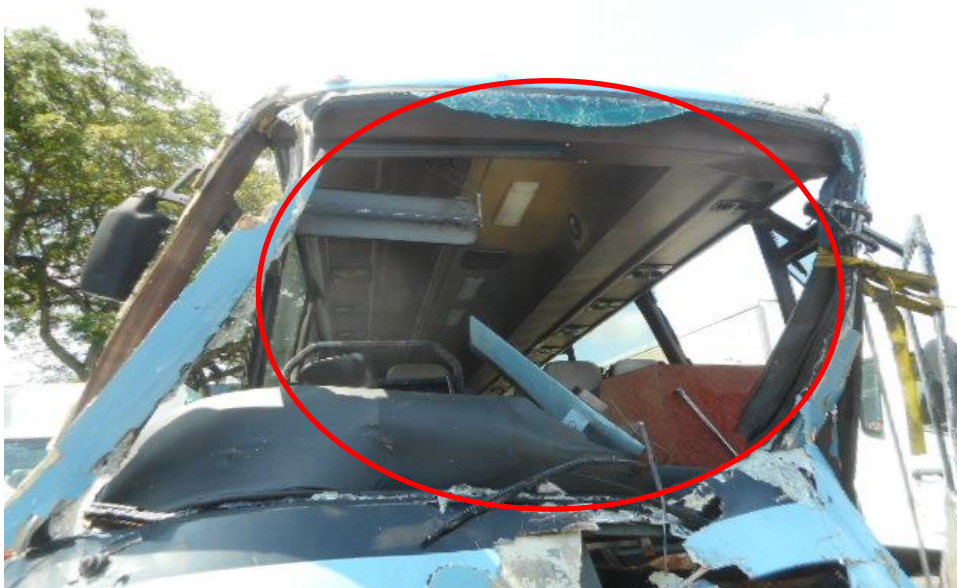
Photo 5 shows a close up view of the front body of the Motor Bus at the time of my inspection. The Motor Bus was observed to sustained damage at its front portion. Its front windscreen (circled) were damage at the time of my inspection as a result of the accident.
