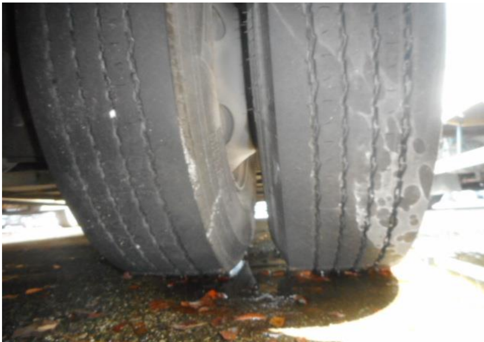
Photo 11 shows the condition of the rear right tyre of the Motor Bus, which was observed to be in serviceable condition with remaining tread depth of approximately 8.9mm. The tyre, which was wrapped around standard steel wheel rim, was also observed to be sufficiently inflated for vehicular operation.
