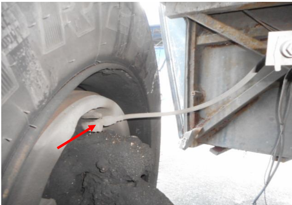
Photo 21 shows the brake pipe (arrowed) at the front left wheel of the Motor Bus. I did not observe any leakage of brake fluid at the time of my inspection of the Motor Bus. My visual examination of the various mechanical components of the braking system where generally intact and unaffected by the accident.
