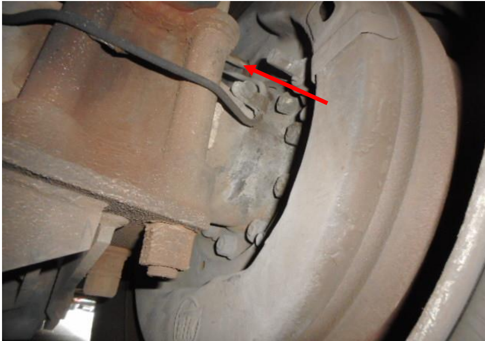
Photo 18 shows the brake pipe (arrowed) at the rear right wheel of the Motor Bus. I did not observe any leakage of brake fluid at the time of my inspection of the Motor Bus. My visual examination of the various mechanical components of the braking system where generally intact and unaffected by the accident.
