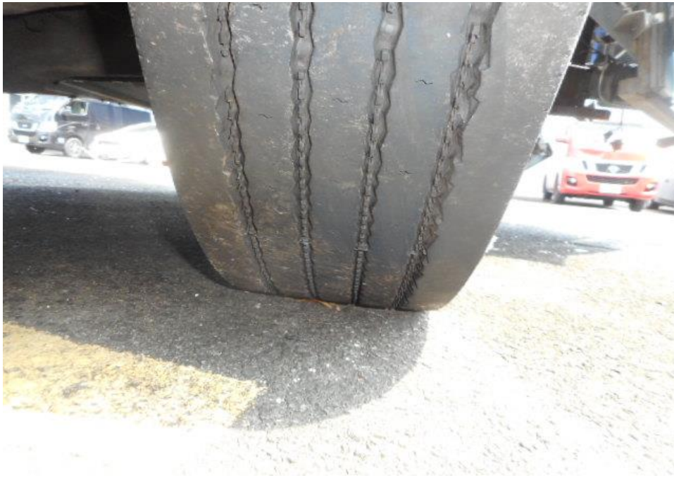
Photo 10 shows the condition of the front right tyre of the Motor Bus, which was observed to be in serviceable condition with remaining tread depth of approximately 5.8mm. The tyre, which was wrapped around standard steel wheel rim, was also observed to be sufficiently inflated for vehicular operation. There was no tear, cut or burst mark(s) on the outer and the inner sidewalls as well as across the tread of the 6 tyres that were fitted on the Motor Bus.
