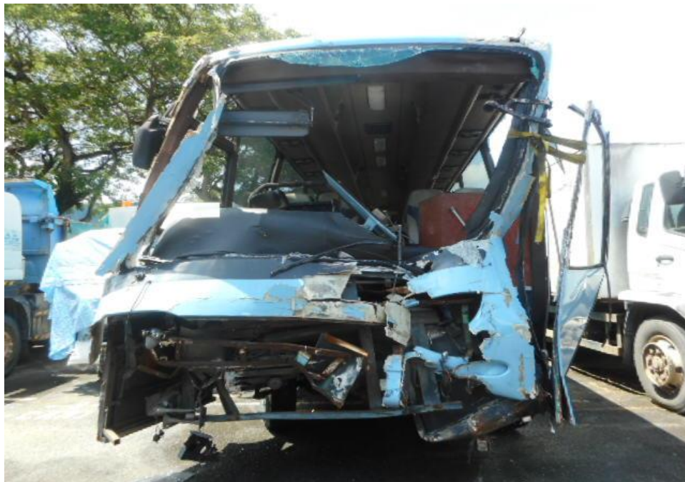
Photo 3 shows a general view of the front body of the Motor Bus at the time of my inspection. The Motor Bus was observed to sustained damage at its front portion. Its front cabin structure, front windscreen, front bumper, front body panel, front door was damaged as a result of the accident.
