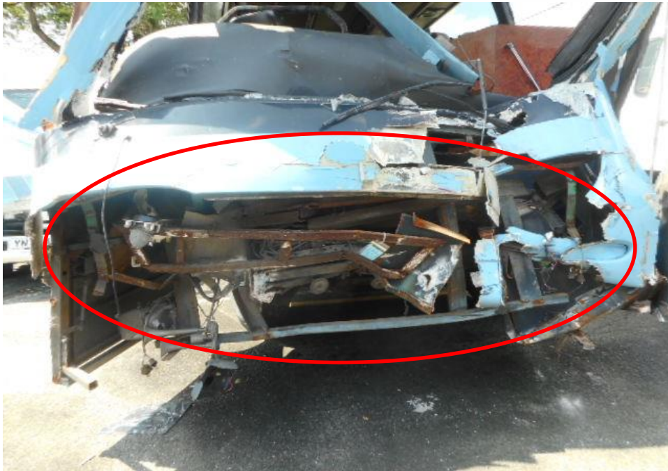
Photo 6 shows a close up view of the front body of the Motor Bus at the time of my inspection. The Motor Bus was observed to sustained damage at its front portion. Its front bumper and front body panel (circled) were damage at the time of my inspection as a result of the accident.
