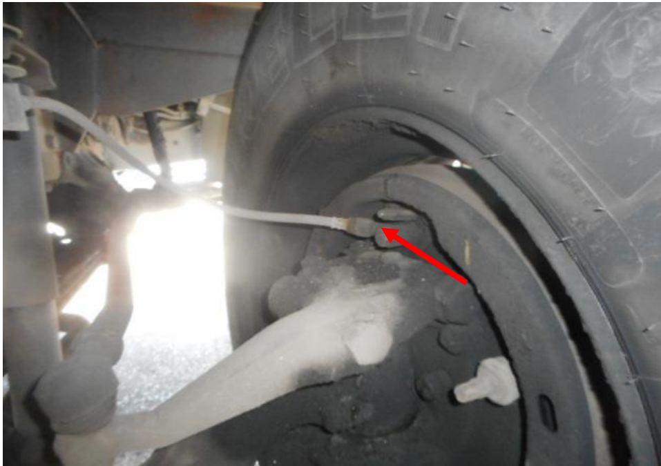
Photo 20 shows the brake pipe (arrowed) at the front right wheel of the Motor Bus. I did not observe any leakage of brake fluid at the time of my inspection of the Motor Bus. My visual examination of the various mechanical components of the braking system where generally intact and unaffected by the accident.
