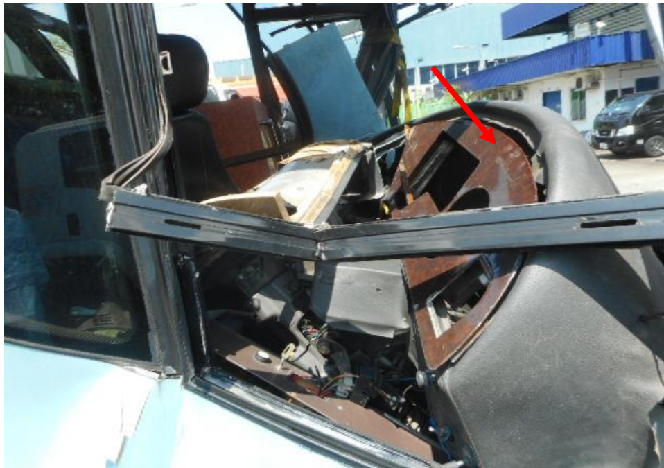
Photo 1 shows the damaged instrument cluster (arrowed). Therefore no mileage is recorded at the time of our inspection.
