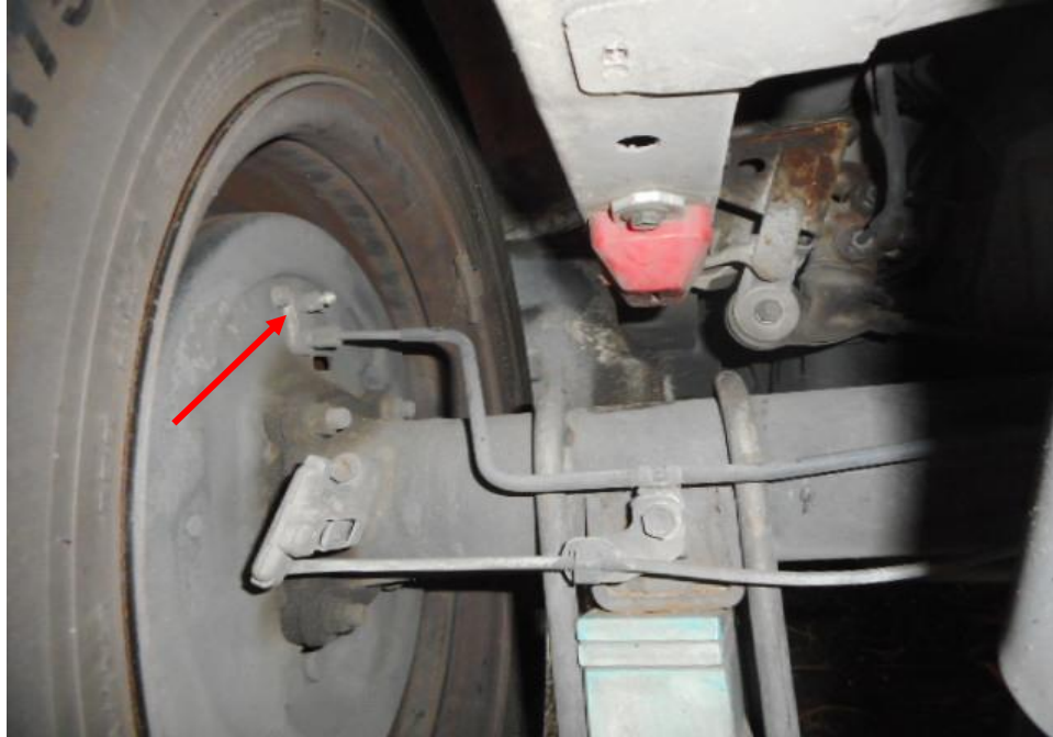
Photo 22 shows the brake pipe (arrowed) at the rear left wheel of the Motor Van. I did not observe any leakage of brake fluid at the time of my inspection of the Motor Van. My static tests of the Motor Van's braking system, along with my visual examination of the various mechanical components in the braking system had indicated that there was no internal leakage of pressure/vacuum. Hence the braking system of the Motor Van was likely to be in serviceable condition at the material time of accident.
