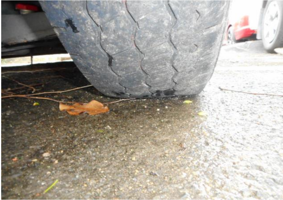
Photo 12 shows the condition of the rear right tyres of the Motor Van, which were observed to be in serviceable condition with remaining, tread depth of approximately 2.5mm. There was also no tear, cut or burst mark(s) on the outer and the inner sidewalls as well as across the tread of the 4 tyres that were fitted on the Motor Van.
