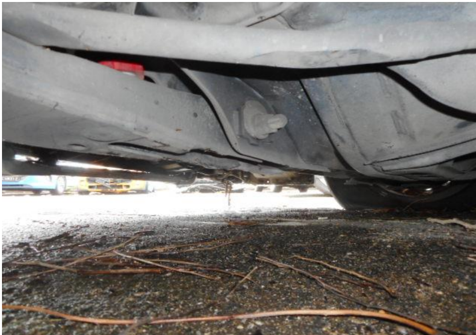
Photo 18 shows the undercarriage of the Motor Van, at the area where the engine housing and transmission housing are located. I did not find any sign(s) or indication(s) of fluid leak and/or fluid stain(s) on the underside of the Motor Van.
