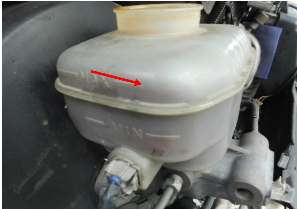
Photo 14 shows the brake fluid reservoir of the Motor Van at the time of my inspection. The brake fluid was observed to be of sufficient level (arrowed) and without any visible contamination.
