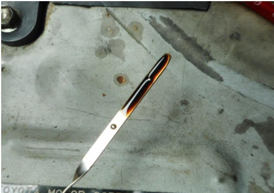
Photo 16 shows the engine oil dip stick of the Motor Van at the time of my inspection. The engine oil was observed to be of sufficient level and without any visible contamination.
