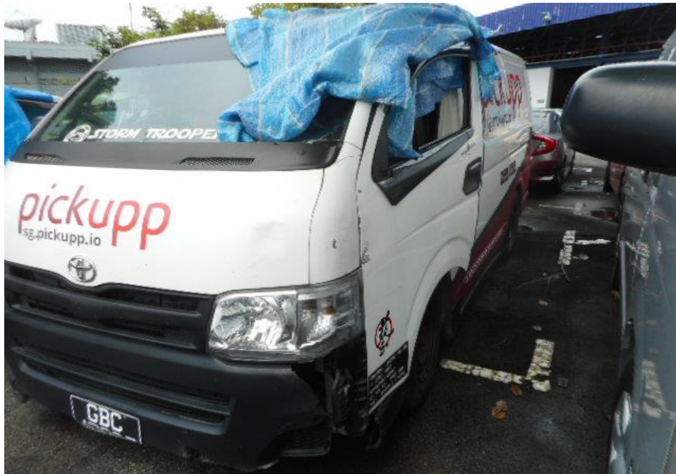
Photo 5 shows a general view of the left body of the Motor Van at the time of my inspection. The Motor Van was observed to sustained damages to its left door windscreen and left rear view mirror due to the accident.
