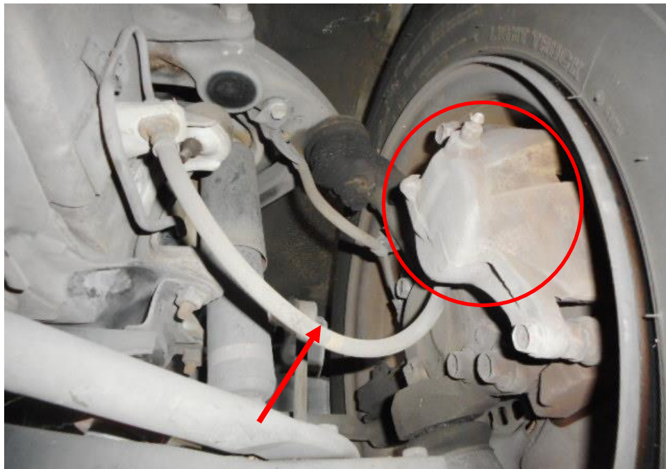
Photo 23 shows the brake hose/pipe (arrowed) at the front right wheel of the Motor Van. No leakage of brake fluid was observed. Visual examination of the various components of the braking system like the brake caliper (circled), brake booster, brake pedal etc had revealed all to be intact and without visible damage at the time of accident. There was also no sign of fluid stain(s) observed on the various undercarriage components.
