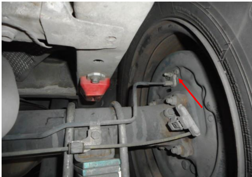
Photo 21 shows the brake pipe (arrowed) at the rear right wheel of the Motor Van. I did not observe any leakage of brake fluid at the time of my inspection of the Motor Van. My static tests of the Motor Van's braking system, along with my visual examination of the various mechanical components in the braking system, had indicated that there was no internal leakage of pressure/vacuum. Hence the braking system of the Motor Van was likely to be in serviceable condition at the material time of accident.
