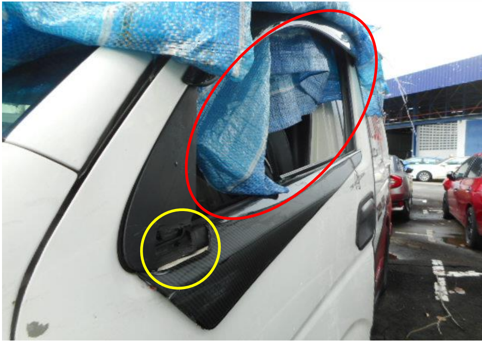
Photo 6 shows a close up view of the left body of the Motor Van at the time of my inspection. The Motor Van was observed to sustained damages to its left door windscreen (red circle) and left rear view mirror (yellow circle) due to the accident.
