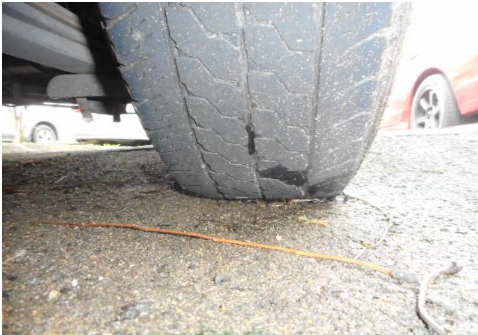
Photo 11 shows the condition of the rear left tyres of the Motor Van, which was observed to be in serviceable condition with remaining tread depth of approximately 1.9mm. The tyres, which were wrapped around standard steel wheel rim, were also observed to be sufficiently inflated for vehicular operation. There was also no damage found on all 4 steel wheel rims of the Motor Van.
