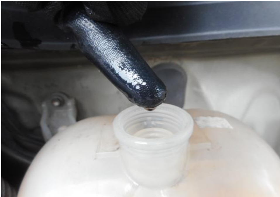
Photo 15 shows the engine coolant of the Motor Van at the time of my inspection. The engine coolant was observed to be of sufficient level and without any visible contamination.
