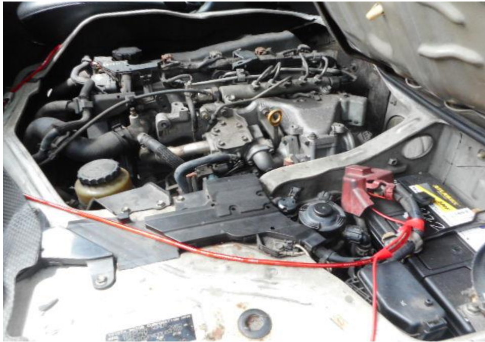
Photo 13 shows a general view of the Motor Van's engine compartment, which was accessed by lifting the front cabin of the Motor Van. The various parts and components inside the engine compartment were unaffected by the accident. There was also no sign(s) or indication(s) of fresh fluid leakage and/or fluid stain within the engine compartment
