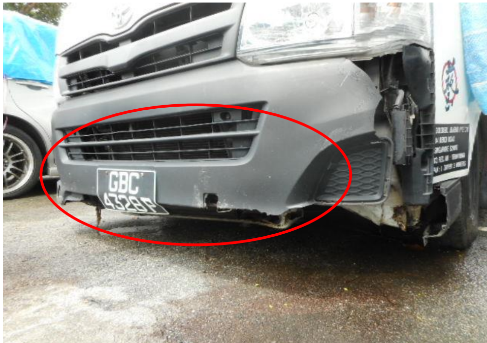
Photo 3 shows a close up view of the Motor Van's frontal portion at the time of my inspection. It appeared to have sustained damage at its frontal portion. Its front bumper (circled) was damage at the time of my inspection as a result of the accident.
