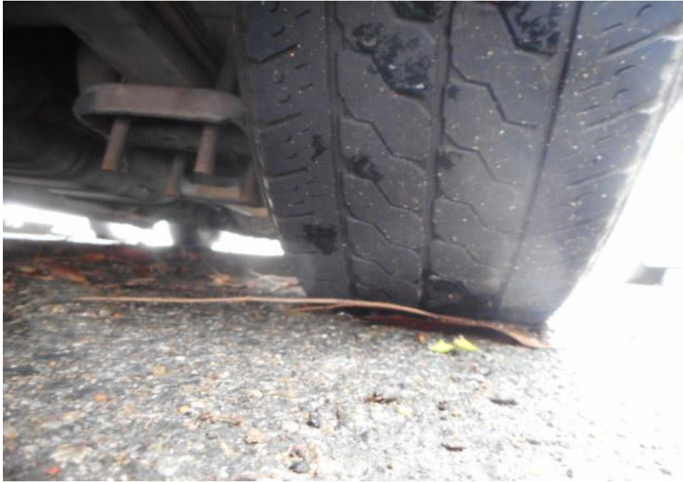
Photo 10 shows the condition of the rear right tyre of the Motor Van, which was observed to be in serviceable condition with remaining tread depth of approximately 6.4mm. The tyre, which was wrapped around standard steel wheel rim, it was observed to be sufficiently inflated for vehicular operation.
