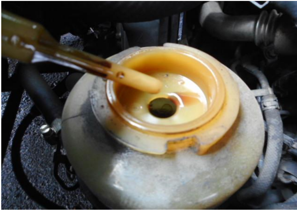
Photo 17 shows the power steering fluid dip stick of the Motor Van at the time of my inspection. The steering fluid was observed to be of sufficient level and without any visible contamination.
