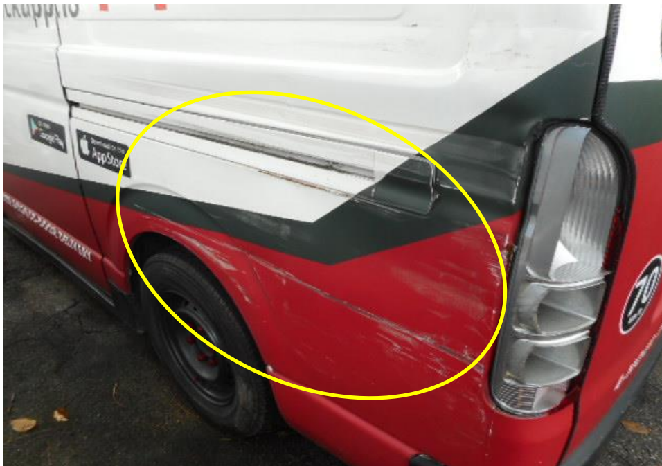
Photo 7 shows a close up view of the left body of the Motor Van at the time of my inspection. The Motor Van was observed to sustained damages to its left body panel (circled) due to the accident.
