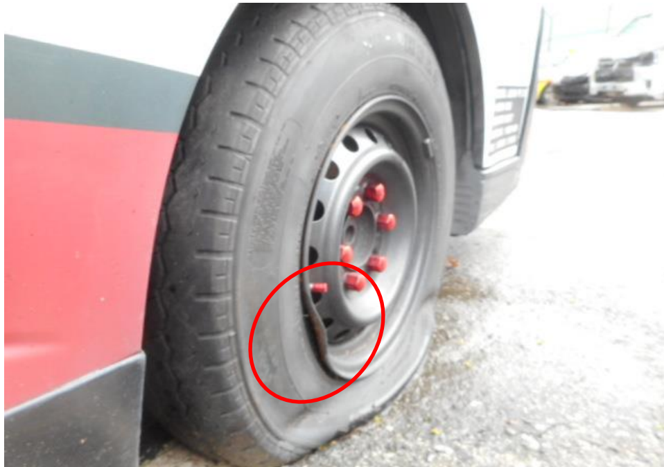
Photo 9 shows the condition of the front right tyre of the Motor Van, which was observed to be deflated as the rim had been damaged (circled) as a result of the accident with remaining tread depth of approximately 3.4mm. The tyre, which was wrapped around standard steel wheel rim, was also observed to be sufficiently inflated for vehicular operation. There was no tear, cut or burst mark(s) on the outer and the inner sidewalls as well as across the tread of the 4 tyres that were fitted on the Motor Van.
