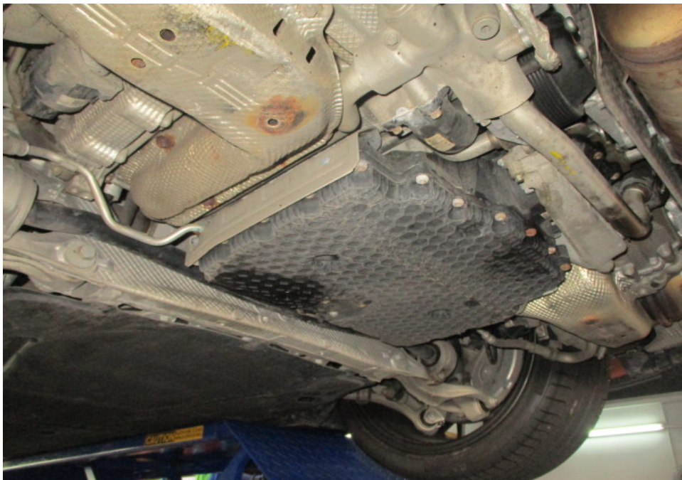
Photo 25 shows a general view of the Motor Car's engine compartment. The engine compartment was at the rear underside of the Motor Car. The various parts and components inside the engine compartment were all observed to be intact and properly fitted. There was also no sign(s) or indication(s) of fluid leak and/or fluid stain found inside the engine compartment.
