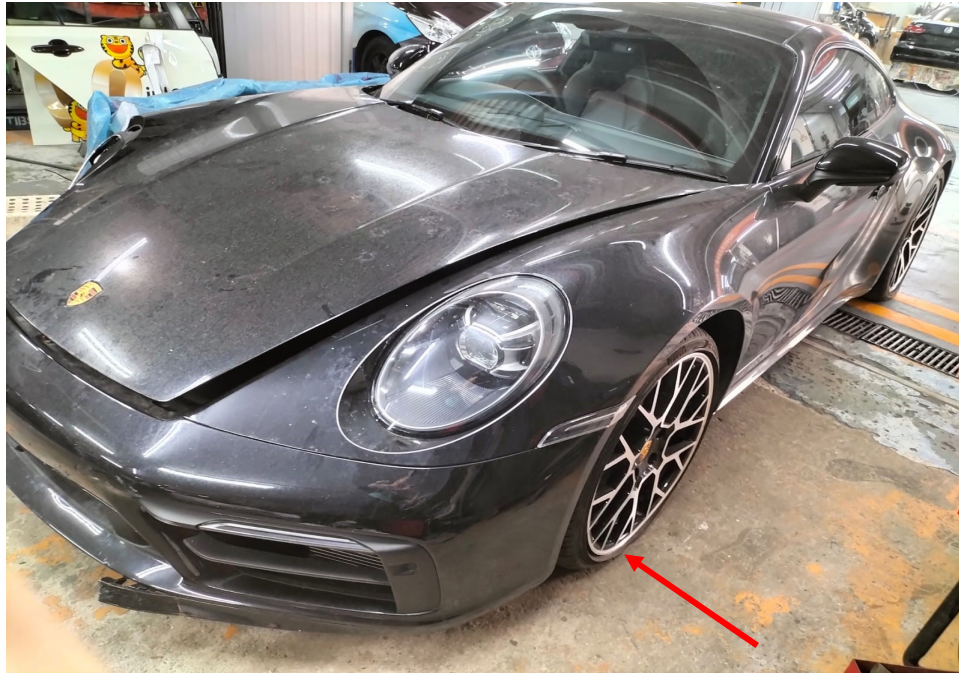
Photo 3 shows the front left body of the Motor Car (photograph provided to me). Apart for the front right portion, there was no physical damage observed to other areas of the Motor Car. The front left wheel (arrowed) and front right wheel (refer to photograph 2 above) were both orientated in a slightly inward direction, which suggests damage to the Motor Car's front right undercarriage parts.
