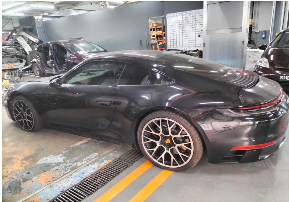
Photo 4 shows the left side body of the Motor Car (photograph provided to me). Apart for the front right portion, there was no physical damage observed to other areas of the Motor Car. The airbag(s) was not deployed as seen from the photographs that were provided to me.
