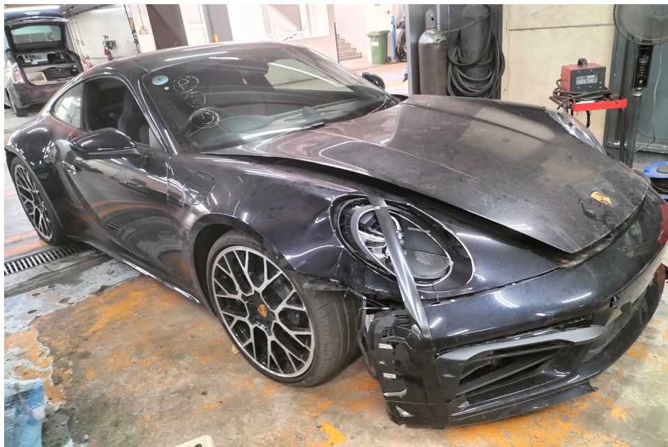
Photo 1 shows the front right body of the Motor Car (photograph provided to me). The photographs provided to me had showed damage to the front right portion of the Motor Car. The front bumper, front bumper lower moulding, front bumper right bracket, front bumper right lower grille, front right fender, front right fender inner shield, front right wheel rim, front right headlamp, front right radiator, right signal lamp and front bonnet were amongst the body parts that were observed to have been damaged.
