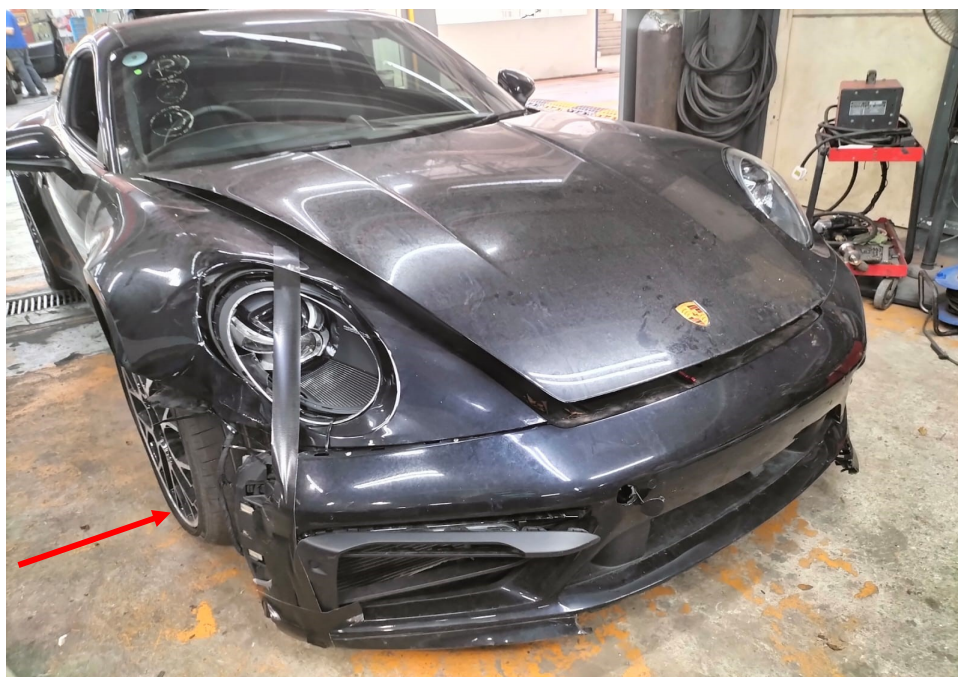
Photo 2 shows another view of the damage at the front right body of the Motor Car (photograph provided to me). The front right wheel (arrowed) and front left wheel (refer to photograph 3 below) were both orientated in a slightly inward direction, which suggests damage to the Motor Car's front right undercarriage parts.
