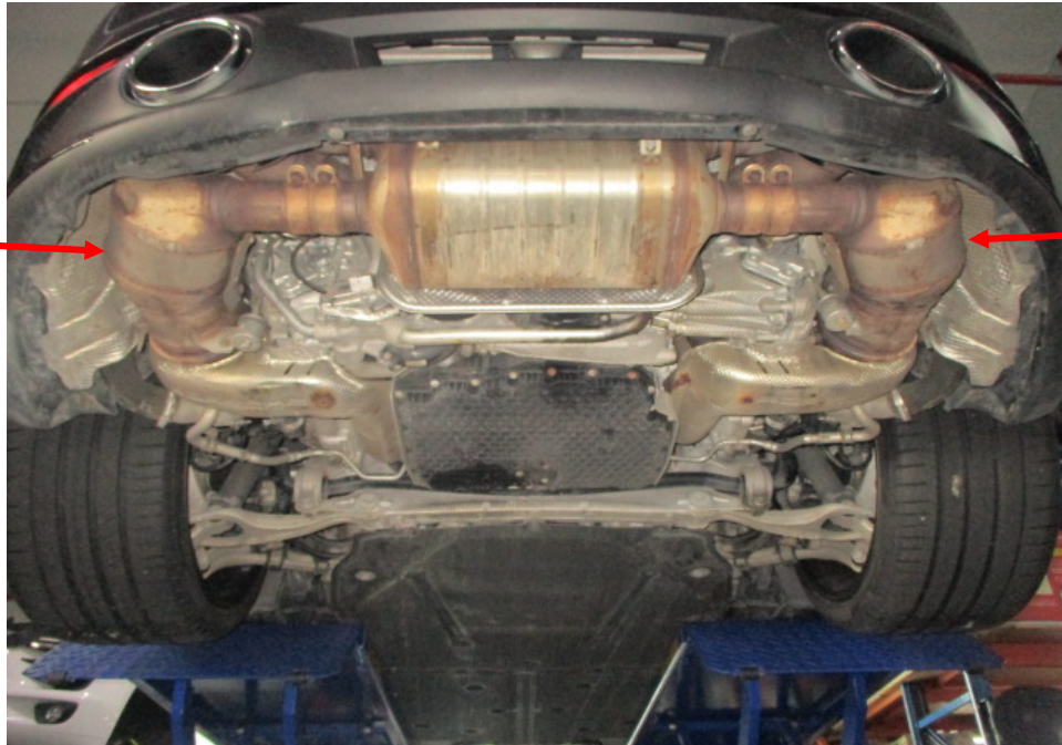
Photo 24 shows the Motor Car's exhaust system. My examination of the Motor Car's exhaust system revealed no sign(s) or indication(s) of any cut or weld marks along its exhaust pipes, on its catalytic converters (arrowed) and on its rear muffler.
