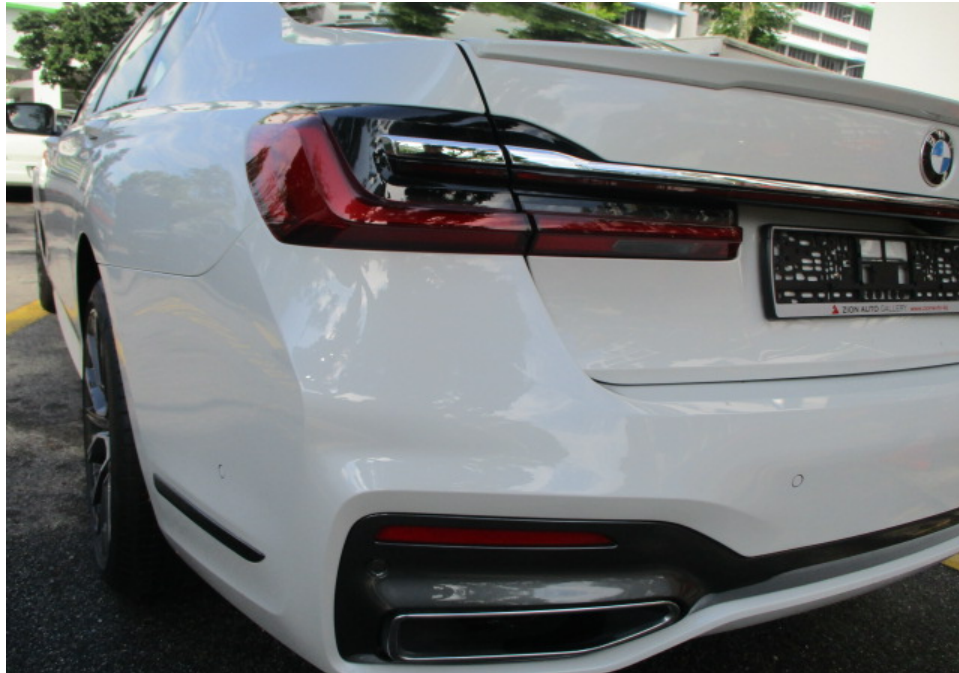
Photo 8 shows a closer view of the Motor Car's rear bumper, rear bootlid, rear bootlid chrome moulding and rear left taillamp at the time of my inspection. The body parts at the rear left portion of the Motor Car were visually examined and it was observed that the repair/restoration works carried out to the damaged area of the Motor Car (refer to photograph 1 above) were reasonably adequate and in order.
