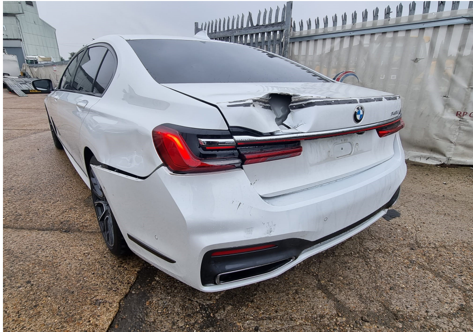
Photo 1 shows the rear left body of the Motor Car (photograph provided to me). The photographs provided to me had showed damage to the rear left portion of the Motor Car. The rear bumper, rear bootlid, rear bootlid chrome moulding, rear bootlid top spoiler, rear left taillamp and rear left fender were amongst the body parts that were observed to have been damaged.
