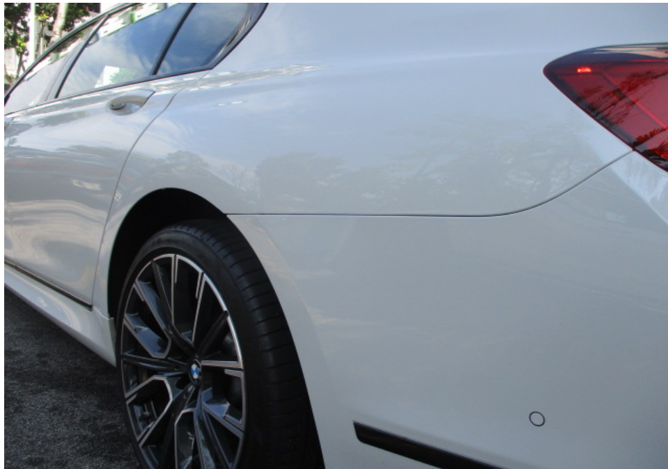
Photo 9 shows a closer view of the Motor Car's rear bumper, rear left fender and rear left wheel rim at the time of my inspection. The body parts at the rear left portion of the Motor Car were visually examined and it was observed that the repair/restoration works carried out to the damaged area of the Motor Car (refer to photograph 1 above) were reasonably adequate and in order.
