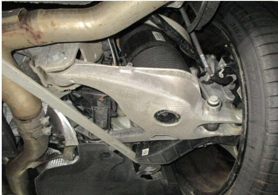
Photo 19 shows a general view of the control arms and linkages at the rear right wheel of the Motor Car. I did not observe any fluid leak and/or fluid stain on the underside of the Motor Car. All of the Motor Car's undercarriage components were observed to be intact and secured in an appropriate manner.
