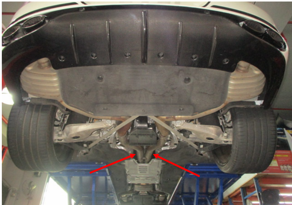
Photo 23 shows the rear section of the Motor Car's exhaust system. My examination of the Motor Car's exhaust system revealed no sign(s) or indication(s) of any cut or weld marks along its exhaust pipes (arrowed), on its rear mufflers, on its centre resonator box and on its catalytic converters.
