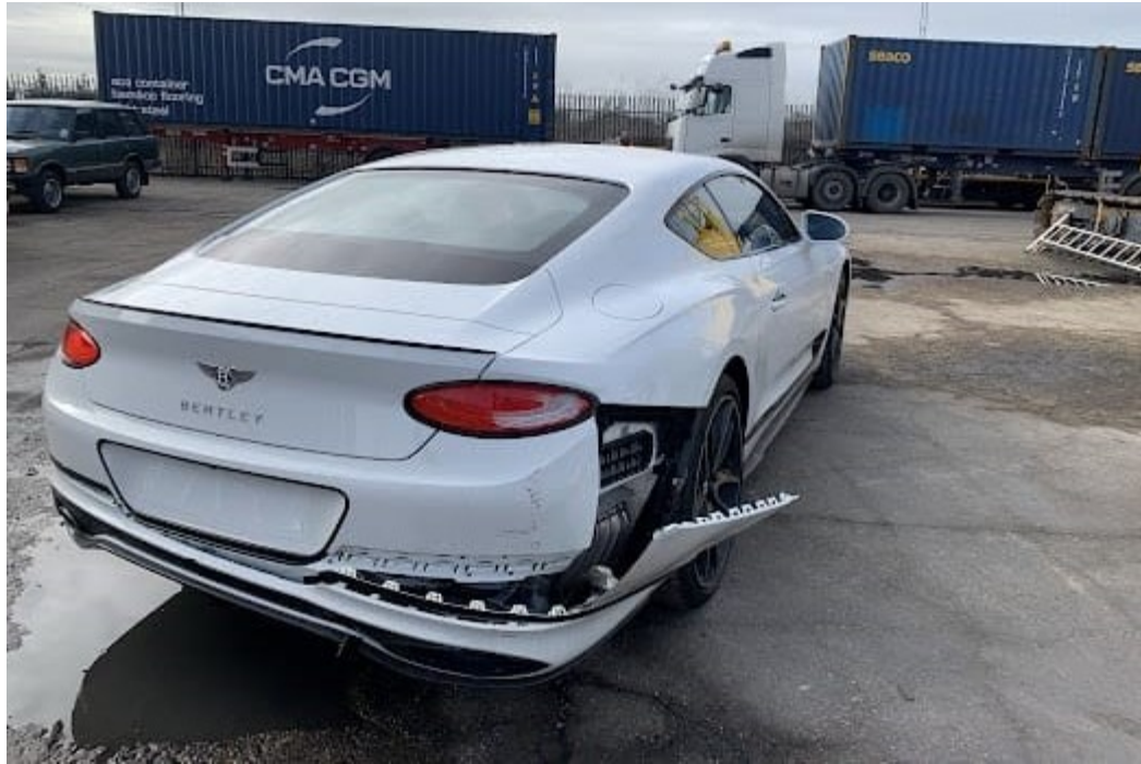
Photo 1 shows the rear right body of the Motor Car (photograph provided to me). The photographs provided to me had showed relatively minor damage to the rear right portion of the Motor Car. The rear bumper and rear right taillamp were observed to have been damaged.
