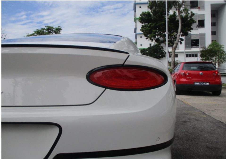
Photo 8 shows a closer view of the Motor Car's rear bumper, rear bootlid and rear right taillamp at the time of my inspection. The body parts at the rear right portion of the Motor Car were visually examined and it was observed that the repair/restoration works carried out to the damaged area of the Motor Car (refer to photograph 1 above) were reasonably adequate and in order.
