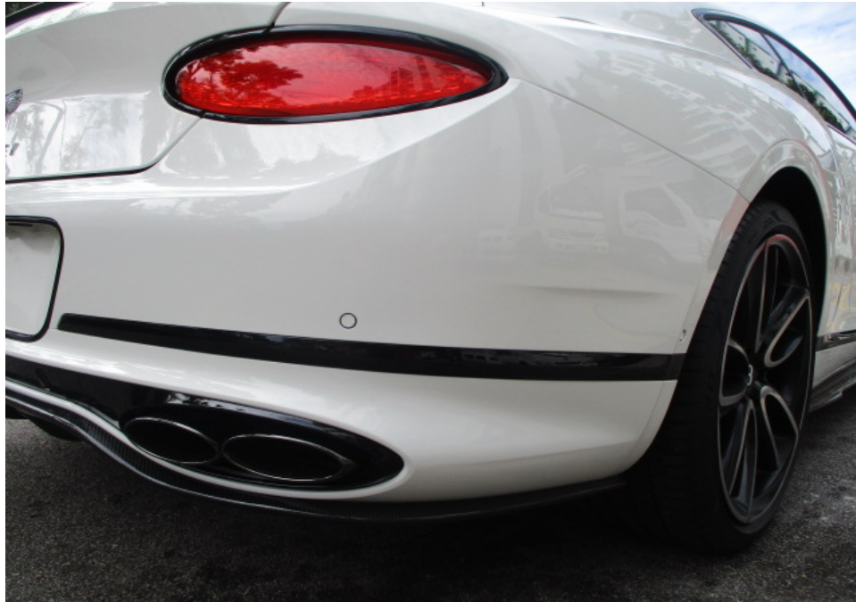
Photo 6 shows a closer view of the Motor Car's rear bumper, rear bumper right lower moulding and rear bumper sensors at the time of my inspection. The body parts at the rear right portion of the Motor Car were visually examined and it was observed that the repair/restoration works carried out to the damaged area of the Motor Car (refer to photograph 1 above) were reasonably adequate and in order.
