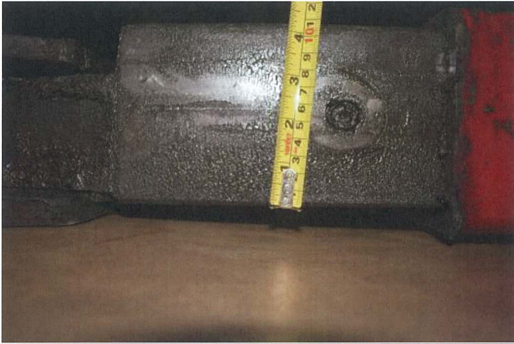
Photo 8 - Measurement on the Tow Truck lifting Inner Boom height reads 10.9cm
