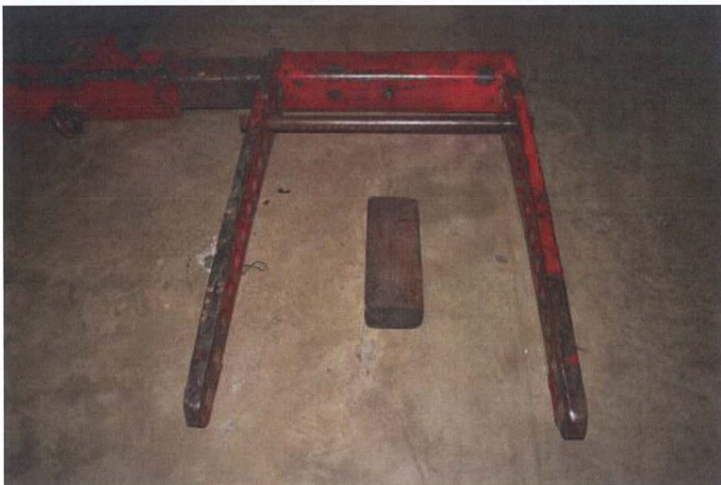
Photo 13 – The proper way to unload a low floor clearance vehicle by using 2 wooden blocks in between each fork
