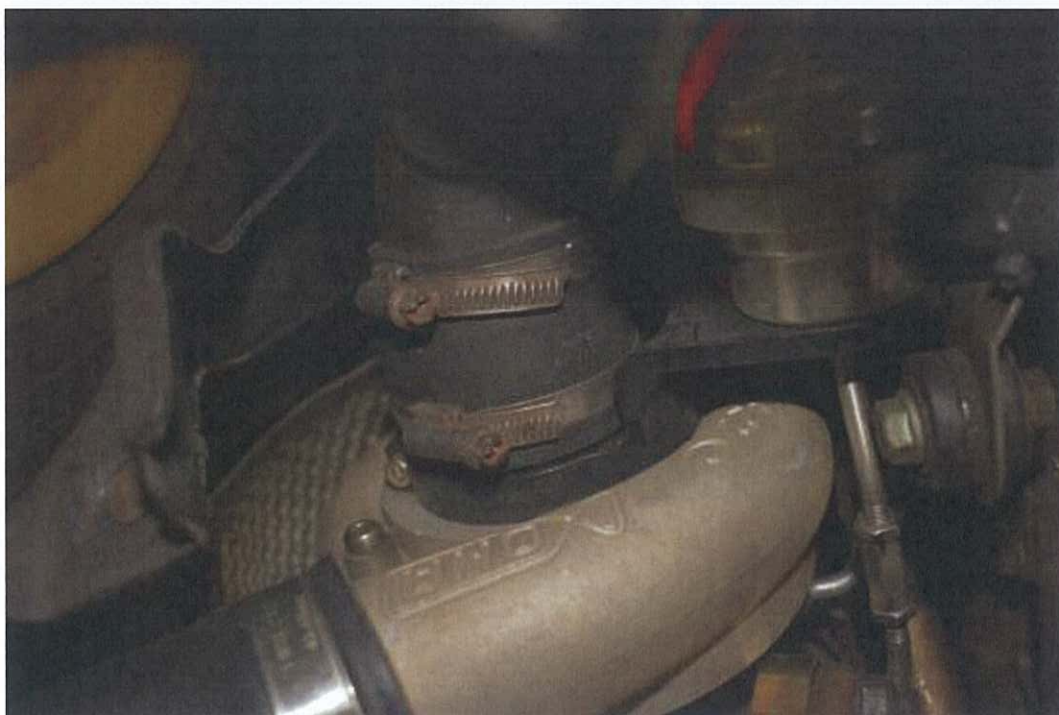
Photo 42 – Right Turbo not replaced -rusty screw and rusty secure bracket. BLACK SOOT MARK SAME AS LKK REPORT PHOTO 19
