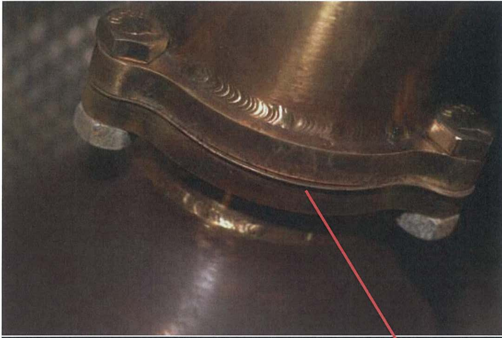
Photo 33 – PV Left Exhaust Muffler to Catalytic Converter Joint with Exhaust Gasket
