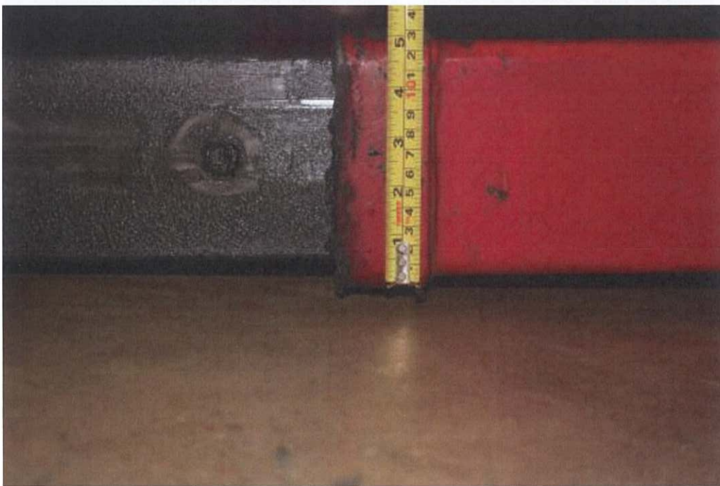
Photo 5 - Measurement on the Tow Truck lifting boom housing height reads 12.5cm
