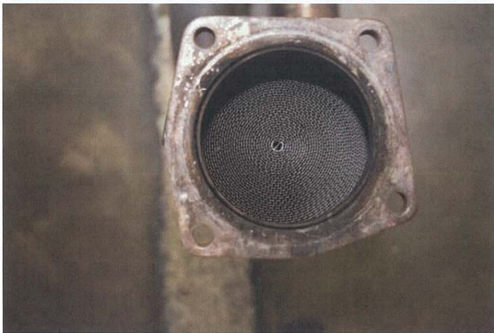
Photo 76 – The honey comb in the Catalytic Convertor is in good condition
