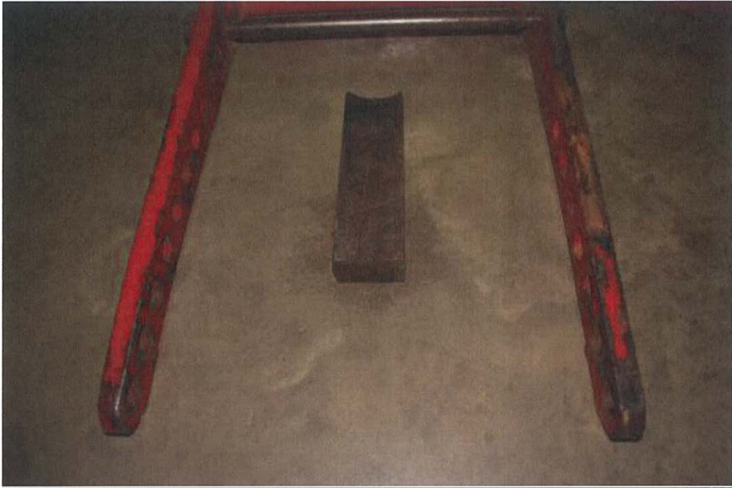
Photo 16 – The proper way to unload a low floor clearance vehicle by using 2 wooden blocks in between each fork
