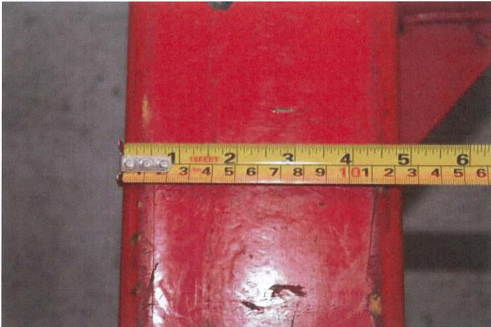
Photo 4 - Measurement on the Tow Truck lifting boom housing reads 12.3cm
