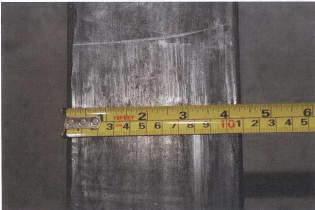
Photo 7 - Measurement on the Tow Truck lifting Inner Boom reads 10.8cm
