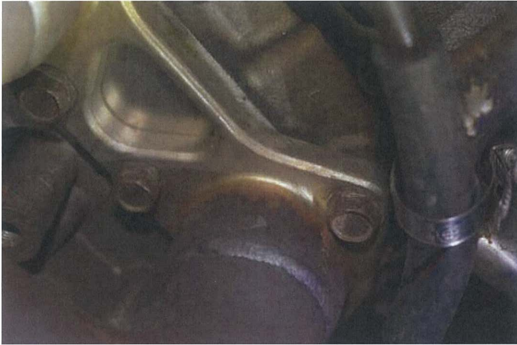
Photo 47 – Left Exhaust Manifold rusty untouched bolt
