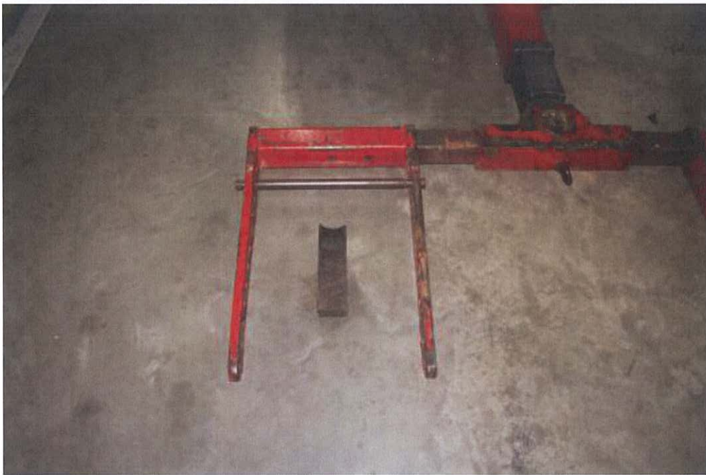
Photo 15 – The proper way to unload a low floor clearance vehicle by using 2 wooden blocks in between each fork
