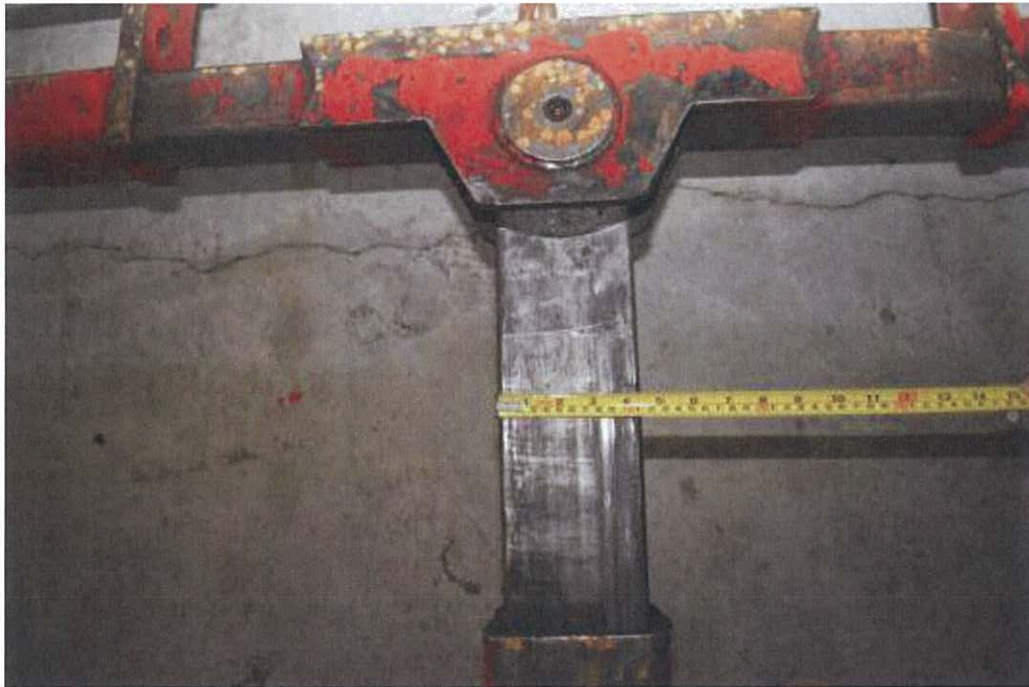
Photo 6 - Measurement on the Tow Truck lifting Inner Boom
