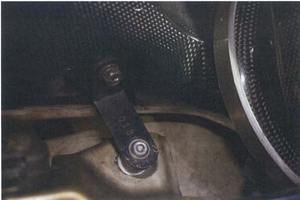
Photo 22 - The Air Duct is secured by a L Bracket
