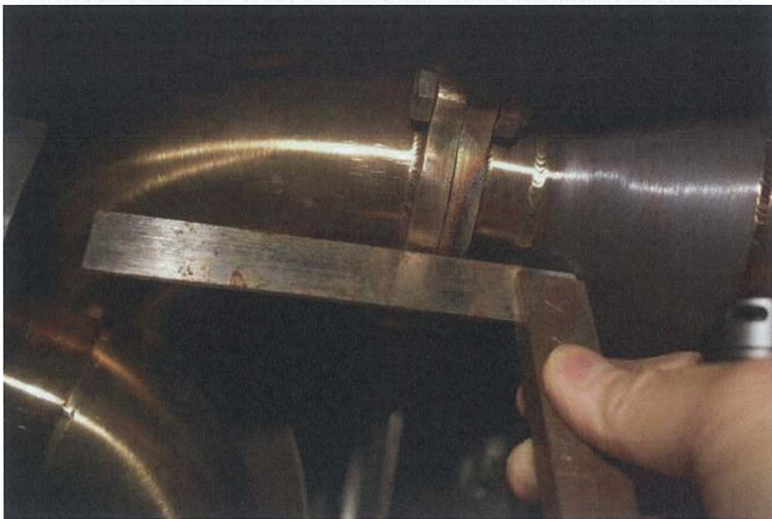
Photo 34 – Measuring the Joint of the right Exhaust Muffler to Catalytic Converter
