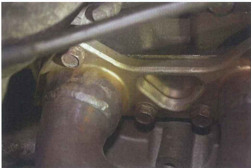
Photo 46 – Left Exhaust Manifold rusted untouched and rusty bolt
