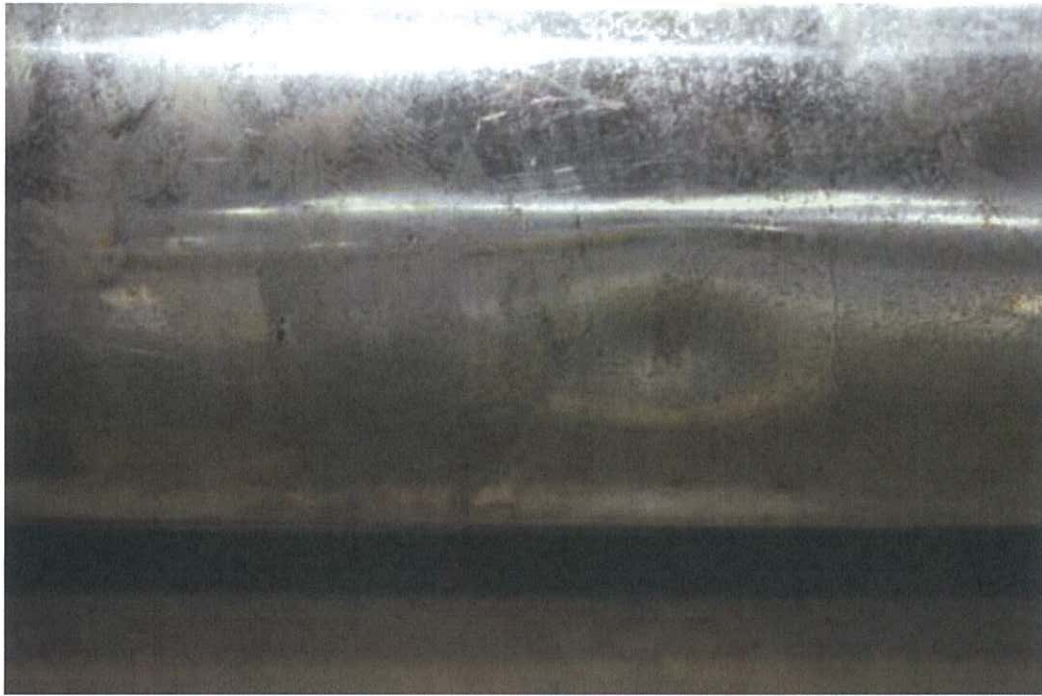
Photo 71 – Rear Exhaust Muffler dent damage, not related to the reported incident
