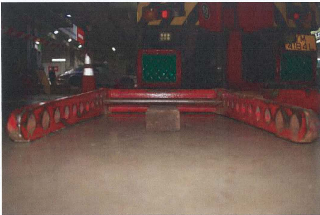
Photo 17 – The proper way to unload a low floor clearance vehicle by using 2 wooden blocks in between each fork
