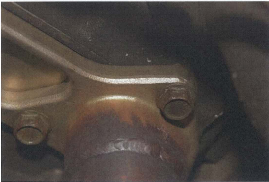
Photo 40 – Right Exhaust Manifold not replaced and untouched rusted bolt
