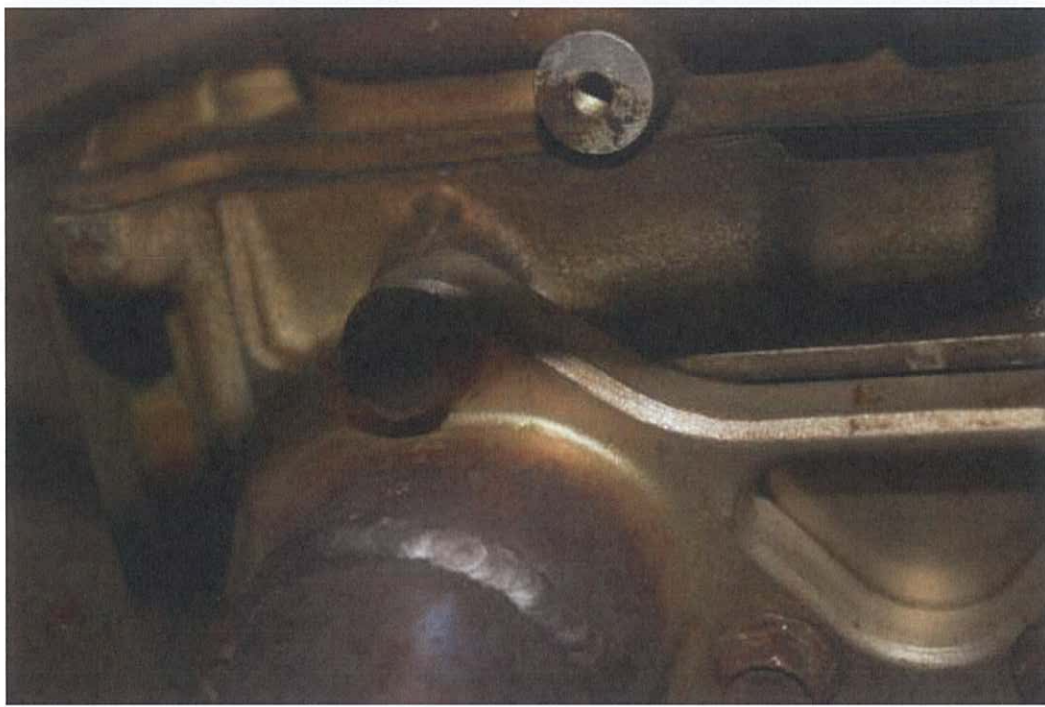
Photo 38 – Right Exhaust Manifold not replaced and untouched rusted bolt
