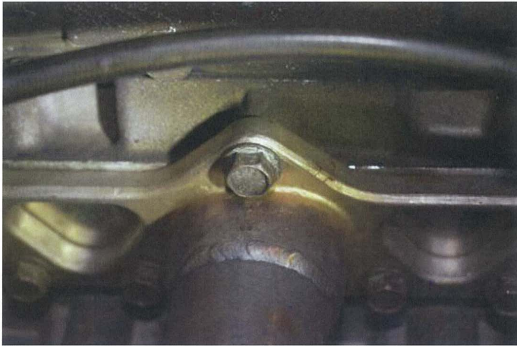
Photo 45 – Left Exhaust Manifold rusty untouched bolt
