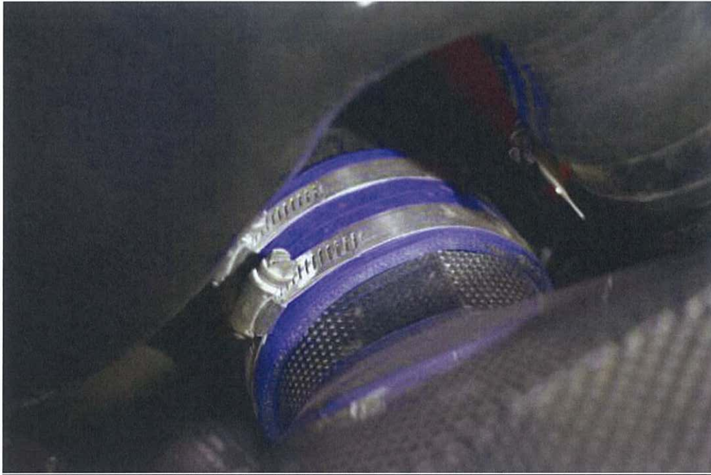
Photo 21 – The Air Duct is secured by hose and clips
