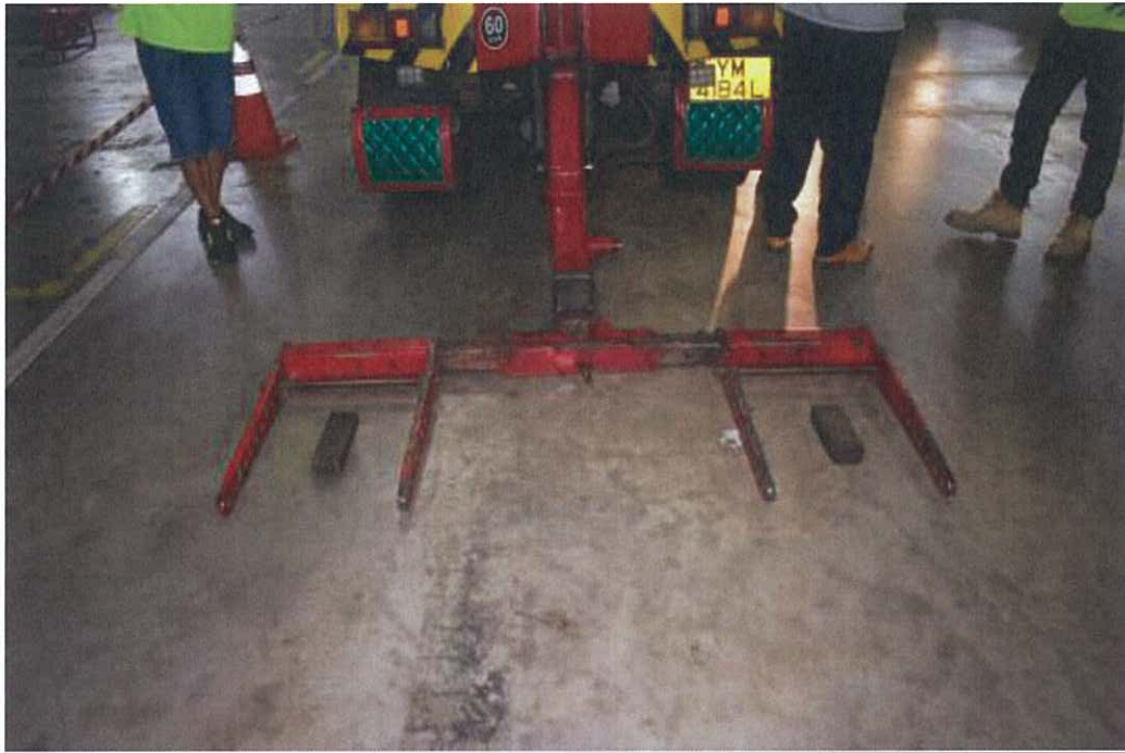
Photo 12 – The proper way to unload a low floor clearance vehicle by using 2 wooden blocks in between each fork
