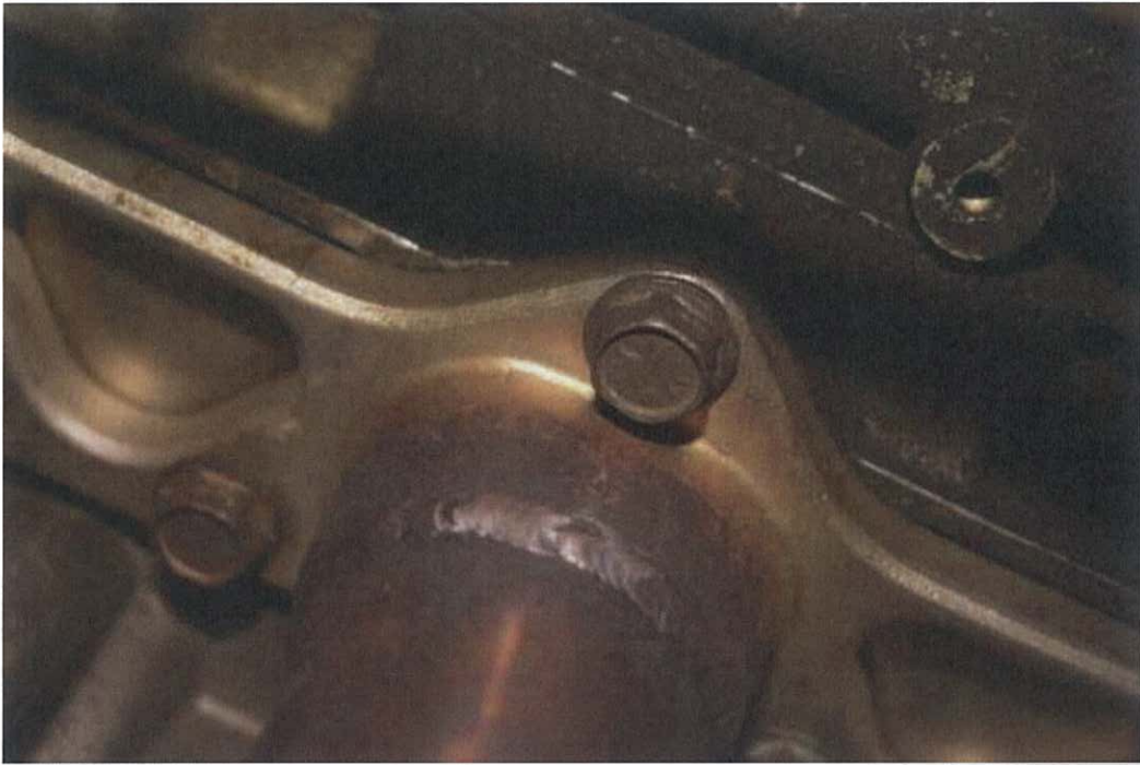
Photo 39 – Right Exhaust Manifold not replaced and untouched rusted bolt
