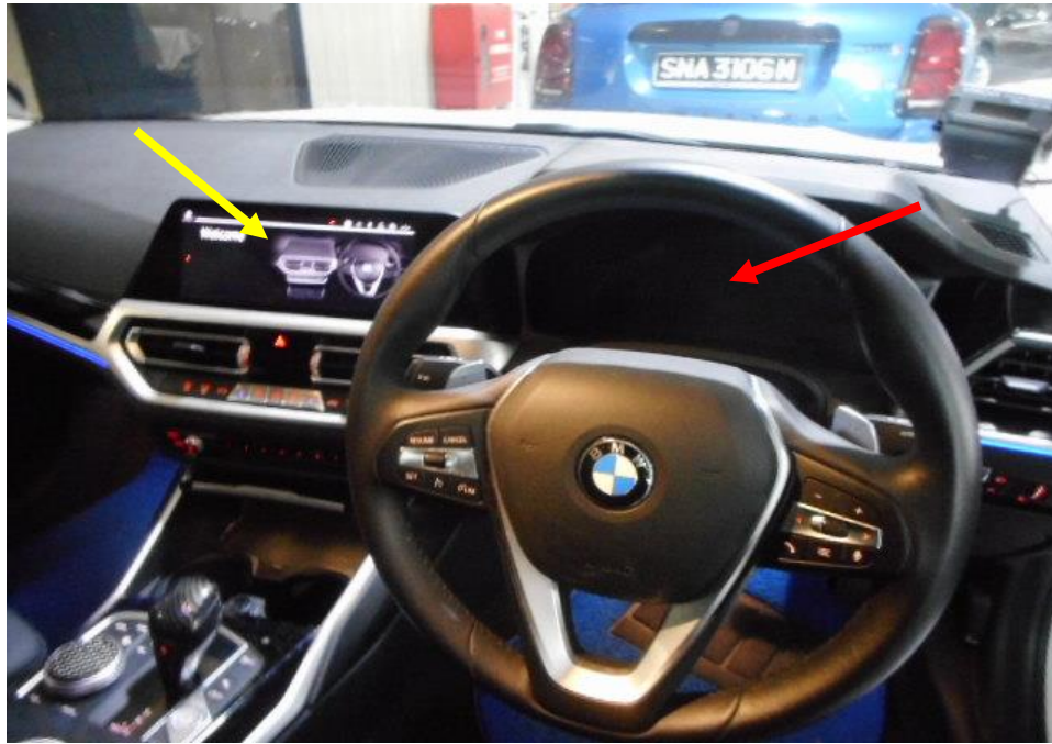
Photo 6 shows the close up view of the vehicle instrument portion of the Insured Vehicle at the time of our inspection. The driver's instrument display (red arrowed) remained turned off even when the vehicle's engine is turned on as compared to the centre display panel (yellow arrow).
