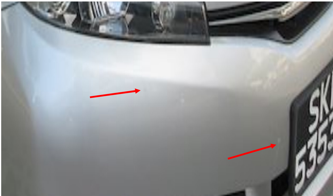
Photo 12 shows a zoomed in view of the relatively faint grazed mark and semi-circular imprint mark on the right side of the Insured Vehicle's front bumper (arrowed). This was at the time when the Singapore Accident Statement was lodged by the driver of the Insured Vehicle on 07 December 2021, which was 10 days before my inspection of the Insured Vehicle on 17 December 2021.
