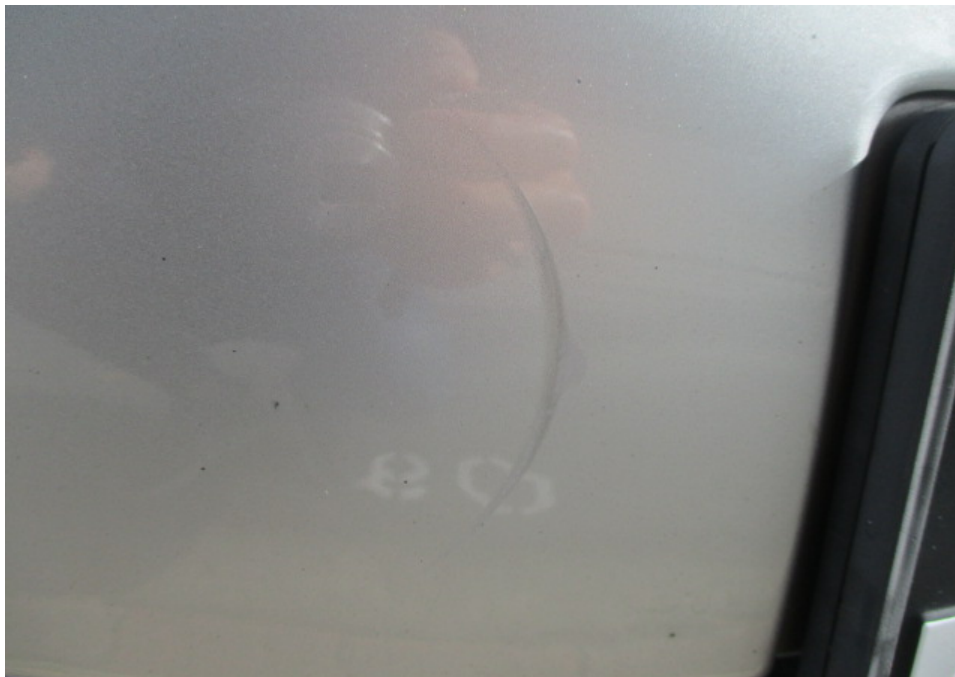
Photo 11 shows a close up view of the semi-circular imprint mark that was found on the front bumper of the Insured Vehicle, at the area towards the right side of the front number plate.
