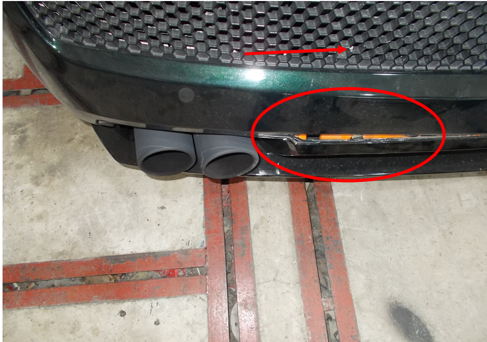
Photo 3 shows another view of the damage to the Third Party Vehicle's rear bumper and rear bumper lower spoiler (circled) at the time of physical inspection by LKK Auto Consultants Pte Ltd. The damage to the rear bumper grille of the Third Party Vehicle is shown by the red arrow.
