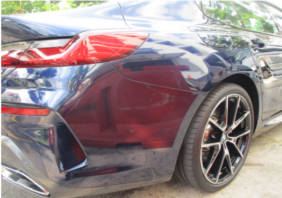
Photo 10 shows a closer view of the Motor Car's rear bumper, rear right taillamp and rear right fender at the time of my inspection. The body parts at the rear right portion of the Motor Car were visually examined and it was observed that the repair/restoration works carried out to the damaged area of the Motor Car (refer to photograph 1 - 3 above) were reasonably adequate and in order.
