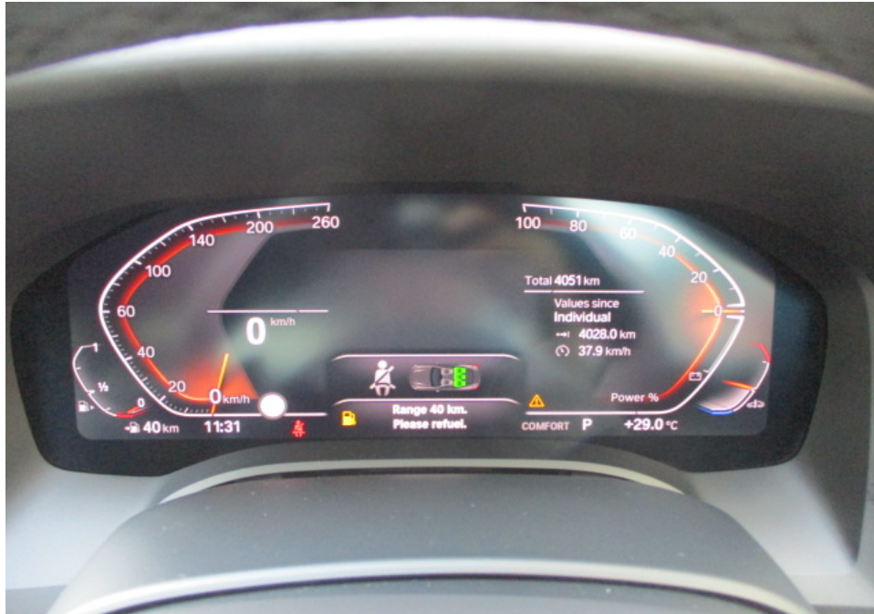
Photo 20 shows the respective warning lights no longer illuminated, indicating that there is no fault detected to the ABS, SRS, IAS, TPM and DSC systems of the Motor Car during the self-test. These electronic systems were hence in working condition at the time of my inspection.
