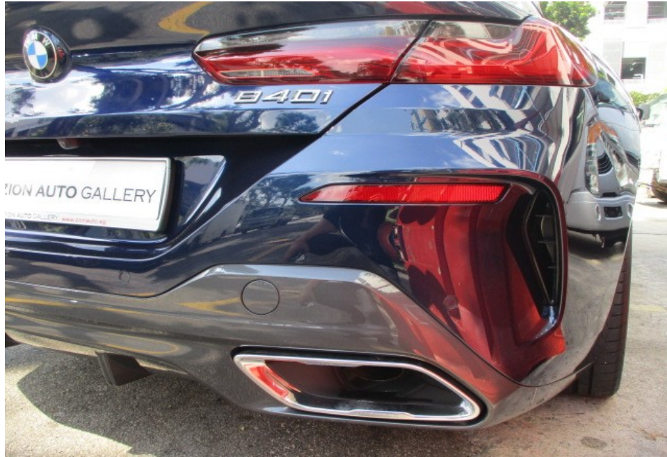
Photo 8 shows a closer view of the Motor Car's rear bumper, rear bumper lower cover, rear bumper tow hook cover, rear bumper right reflector and rear right exhaust chrome garnish at the time of my inspection. The body parts at the rear right portion of the Motor Car were visually examined and it was observed that the repair/restoration works carried out to the damaged area of the Motor Car (refer to photograph 1 - 3 above) were reasonably adequate and in order.
