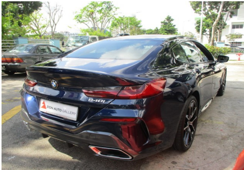
Photo 7 shows a general view of the rear right body of the Motor Car at the time of my inspection. The Motor Car was observed to be in a relatively good general condition with no loose exterior fittings observed. The body parts at the rear right portion of the Motor Car were visually examined and it was observed that the repair/restoration works carried out to the damaged area of the Motor Car (refer to photograph 1 - 3 above) were reasonably adequate and in order.
