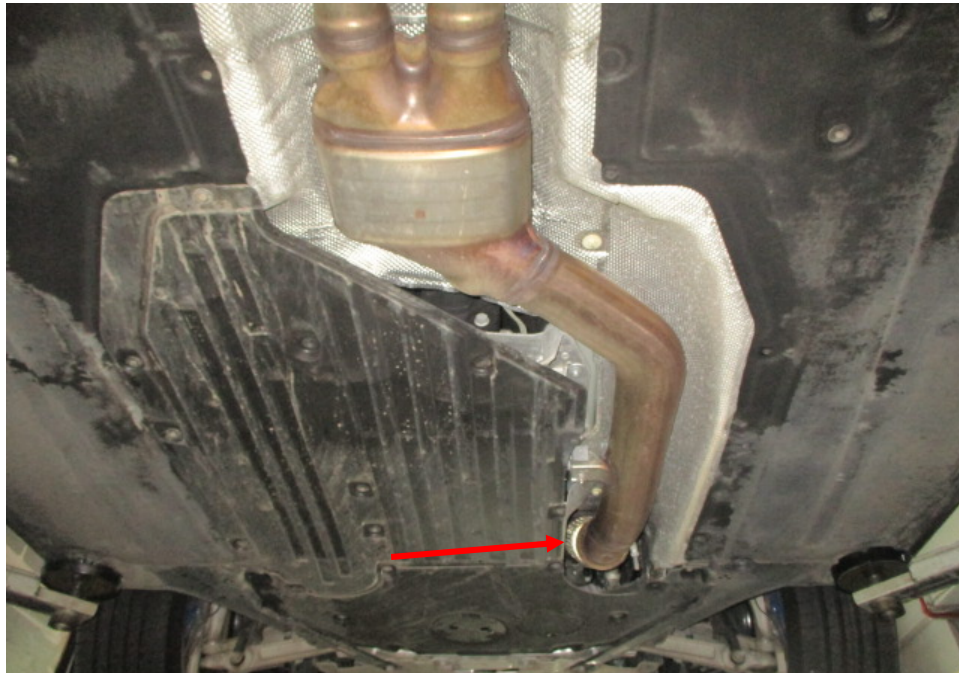
Photo 27 shows the front section of the Motor Car's exhaust system. My examination of the Motor Car's exhaust system revealed no sign(s) or indication(s) of any cut or weld marks along its exhaust pipes, on its rear muffler, on its centre resonator boxes and on its catalytic converter (arrowed).
