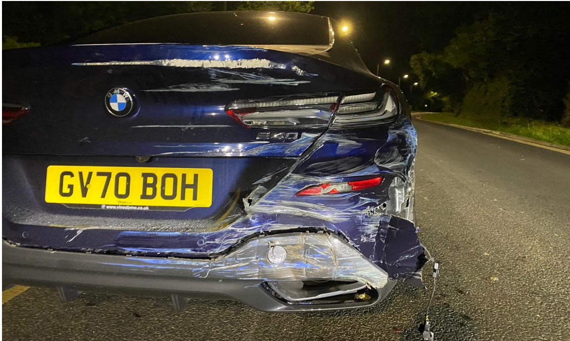
Photo 1 shows the rear right body of the Motor Car (photograph provided to me). The photographs provided to me had showed damage to the rear right portion of the Motor Car. The rear bumper, rear bumper lower cover, rear bumper tow hook cover, rear bumper sensors, rear bumper right reflector, rear right exhaust chrome garnish, rear bootlid, rear right bootlid lamp and rear right taillamp were amongst the body parts that were observed to have been damaged.
