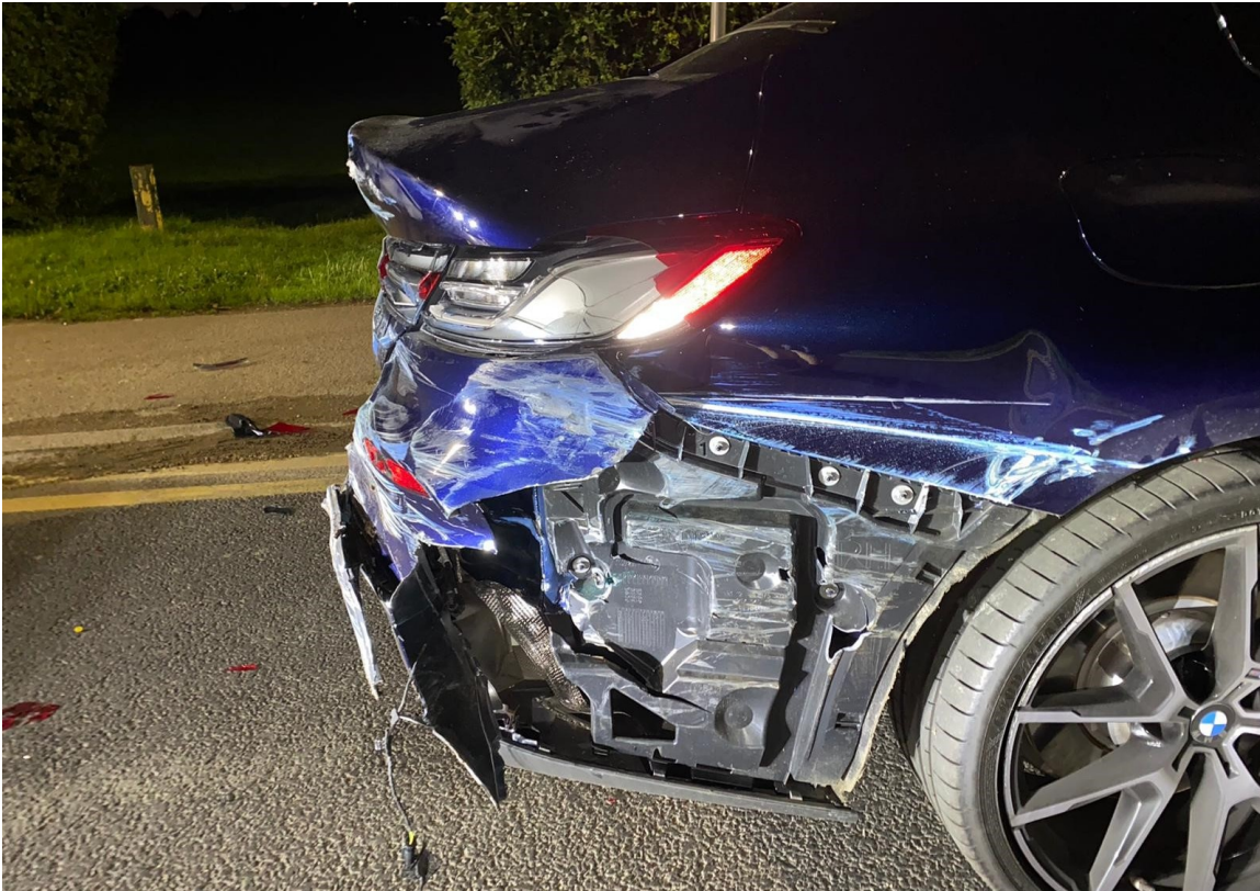
Photo 3 shows the right side rear portion of the Motor Car (photograph provided to me). The rear bumper, rear bumper lower cover, rear bumper sensors, rear bumper right corner air vent, rear bumper right bracket, rear right exhaust heat shield, rear right taillamp and rear right fender were amongst the body parts that were observed to have been damaged.
