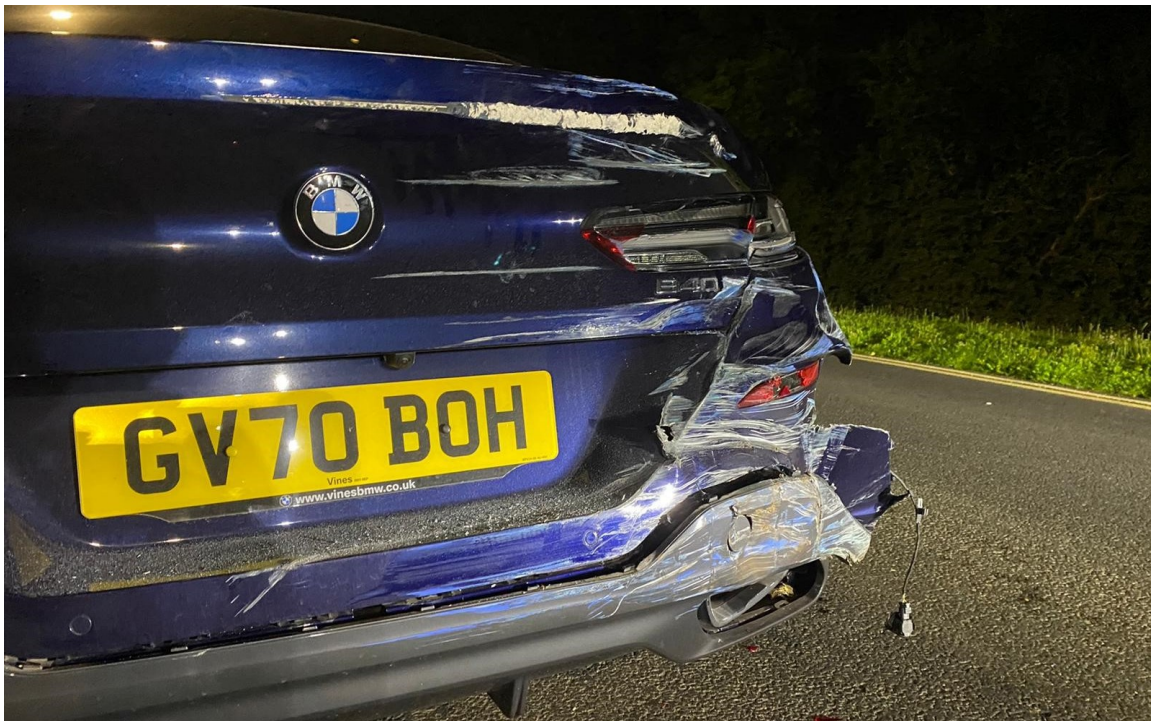
Photo 2 shows another view of the damage at the rear right portion of the Motor Car (photograph provided to me). The rear bumper, rear bumper lower cover, rear right exhaust chrome garnish, rear bootlid and rear right bootlid lamp were amongst the body parts that were observed to have been damaged.
