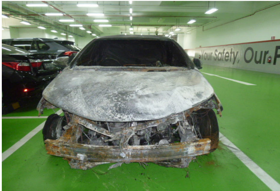
Photo 3 shows the general view of the frontal portion of the Insured Vehicle at the time of our inspection. The fire damage to the Insured Vehicle was confined to its frontal portion. The entire engine compartment of the Insured Vehicle was observed to be severely burnt while the interior compartment was observed to be severely affected by the fire.
