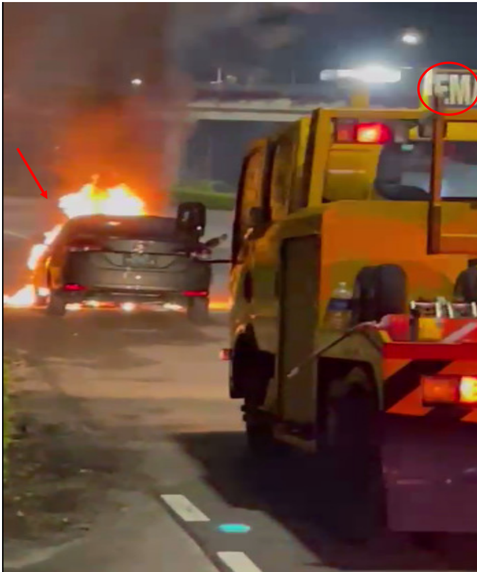
Photo 10 shows the Insured Vehicle on fire before the arrival of the SCDF. In general, the information that could be gathered from this photograph had corresponded to the events that were related to us by Ms Ng which is the fire had started from the frontal portion of the Insured Vehicle (arrowed) and that EMAS Recovery Services were first to arrive at the incident scene (circled).
