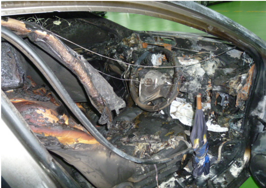
Photo 7 shows the interior compartment of the Insured Vehicle, which was severely affected by the fire.
