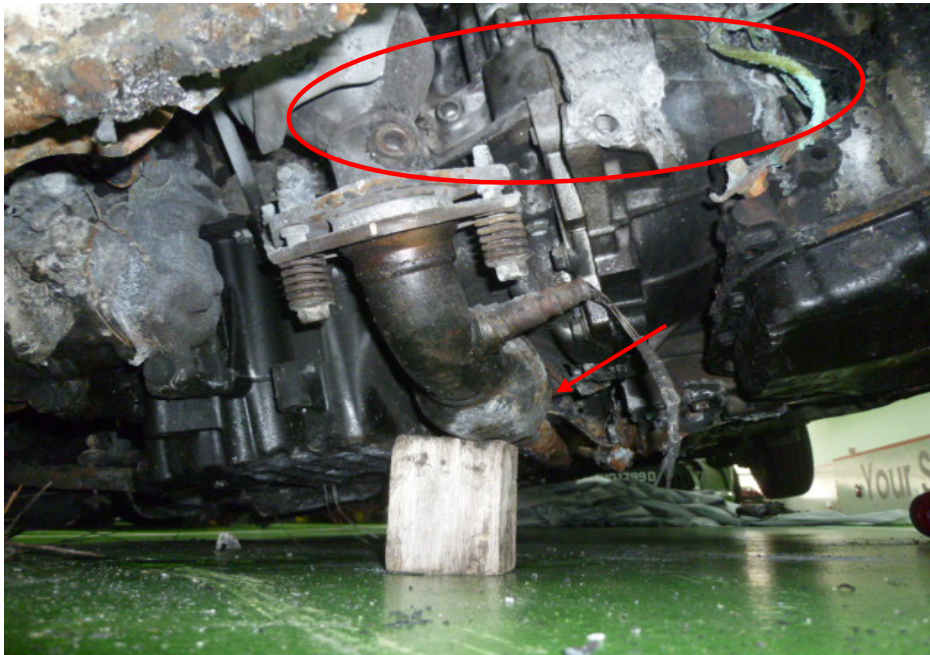
Photo 8 shows the fire damage at the exterior portion of the front undercarriage of the Insured Vehicle. The high heat intensity burn marks (whitish burn marks) found on the exterior surface of its engine components (circled) and rust that had developed on the front undercarriage (arrowed) indicates that the fire to the Insured Vehicle had originated from the exterior of the Insured Vehicle.
