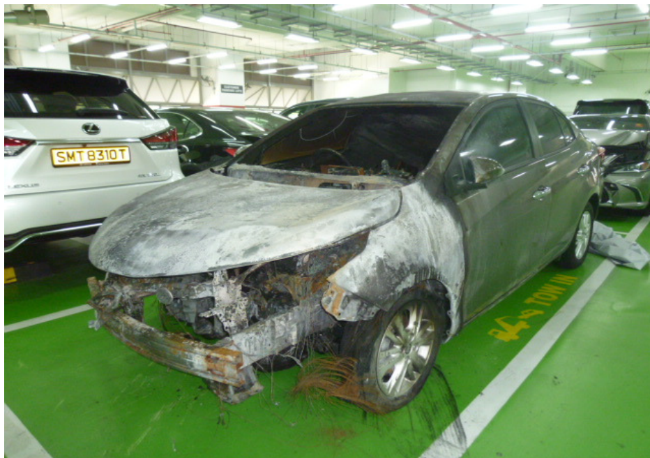
Photo 2 shows the closer view of the left front body of the Insured Vehicle at the time of our inspection. The fire damage to the Insured Vehicle was confined to its frontal portion. Its front windscreen, front bumper, front bonnet, front support panel, front grille, left headlamp, left front wheel rim, left front fender and left front tyre were amongst the body parts that were found to have been affected by the fire.
