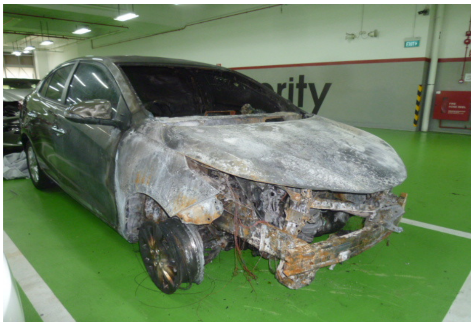
Photo 4 shows the closer view of the right front body of the Insured Vehicle at the time of our inspection. The fire damage to the Insured Vehicle was confined to its frontal portion. Its front windscreen, front bumper, front bonnet, front support panel, front grille, right headlamp, right front wheel rim, right front fender and right front tyre were amongst the body parts that were found to have been affected by the fire.
