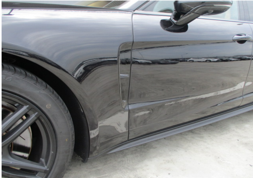
Photo 8 shows a closer view of the Motor Car's front left fender, front left door and left side rocker panel garnish. The body parts at the left side front portion of the Motor Car were visually examined and it was observed that the repair/restoration works carried out to the damaged area of the Motor Car (refer to photograph 1 above) were reasonably adequate and in order.
