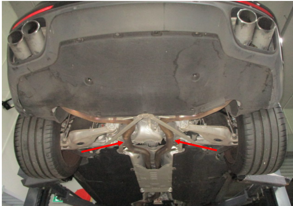
Photo 23 shows the rear section of the Motor Car's exhaust system. My examination of the Motor Car's exhaust system revealed no sign(s) or indication(s) of any cut or weld marks along its exhaust pipes (arrowed), on its rear mufflers and on its catalytic converter.
