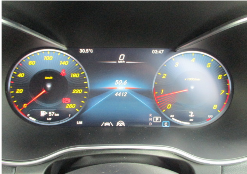
Photo 18 shows the respective warning lights no longer illuminated, indicating that there is no fault detected to the ABS, SRS, EPS, TPM and TCS systems of the Motor Car during the self-test. These electronic systems were hence in working condition at the time of my inspection.
