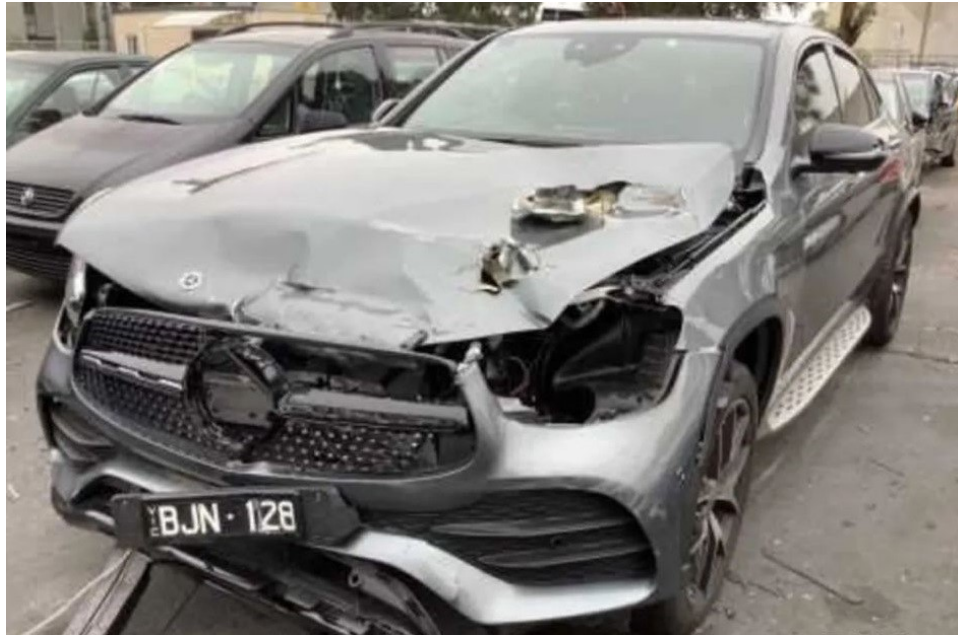
Photo 1 shows the front left body of the Motor Car (photograph provided to me). The Motor Car was observed to have sustained damage at its frontal portion. The front bumper, front bumper left lower grille, front bumper centre lower grille, front bumper number plate garnish, front bumper sensors, front bonnet, front bonnet hinges, radiator grille, radiator grille emblem, front left headlamp and front left fender were amongst the body parts that were observed to have been damaged. The airbag(s) appears to be not deployed as seen from the photographs that were provided to me.
