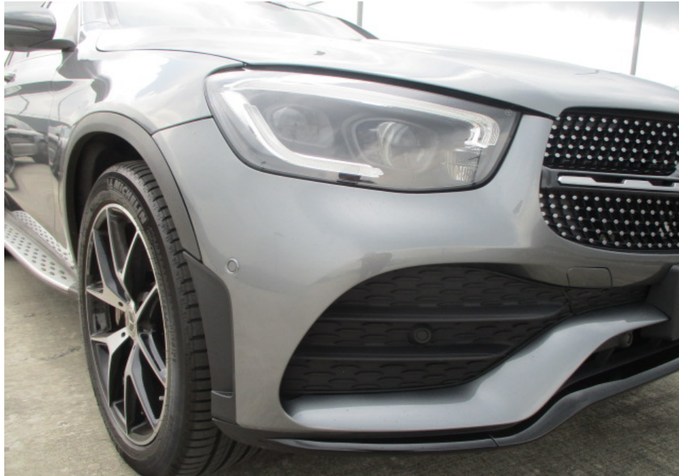
Photo 10 shows a closer view of the Motor Car's front bumper, front bumper right lower grille, front bumper right corner garnish, front bumper right sensor, front right fender wheel arc garnish and front right headlamp. The body parts at the frontal portion of the Motor Car were visually examined and it was observed that the repair/restoration works carried out to the damaged area of the Motor Car (refer to photograph 1 & 2 above) were reasonably adequate and in order.
