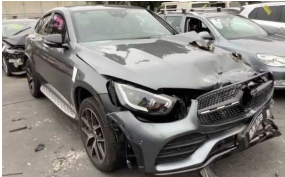
Photo 2 shows the front right body of the Motor Car (photograph provided to me). The Motor Car was observed to have sustained damage at its frontal portion. The front bumper, front bumper right lower grille, front bumper centre lower grille, front bumper lower lip, front bonnet, radiator grille and front right headlamp were amongst the body parts that were observed to have been damaged. The airbag(s) appears to be not deployed as seen from the photographs that were provided to me.
