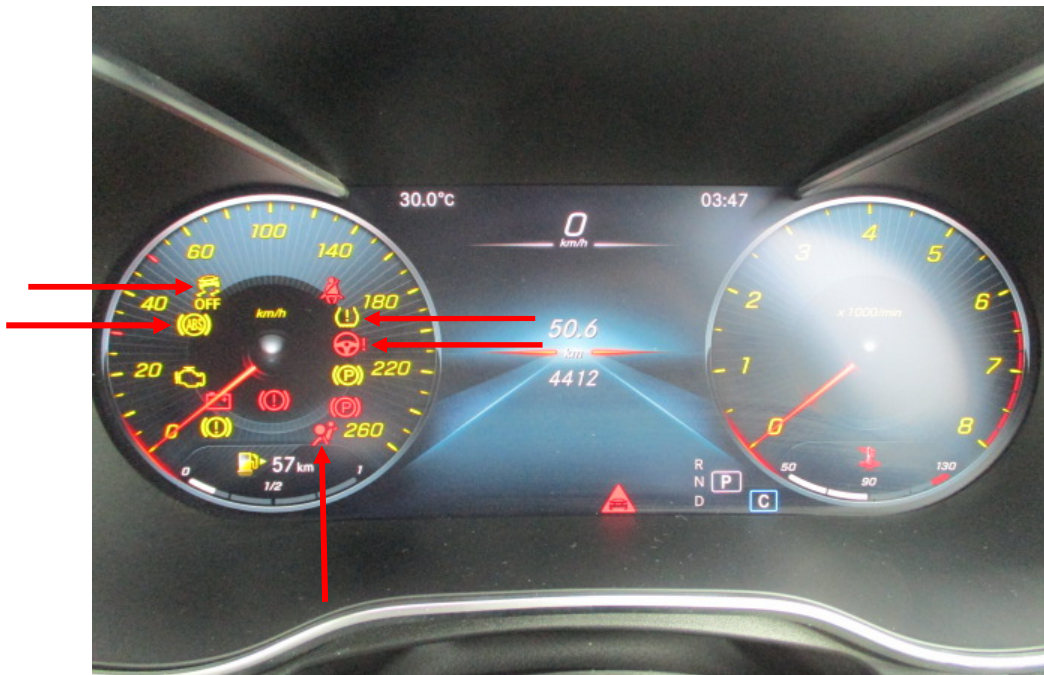
Photo 17 shows the warning lights for the various electronic safety features appearing on the instrument panel of the Motor Car during its self-test when the engine is cranked, in particular the ABS, SRS, EPS, TPM and TCS lights (arrowed).
